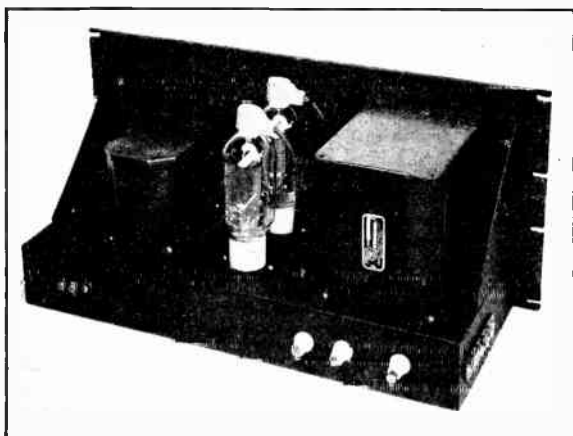
Fig. 1115—A conventional chassis arrangement for low- and medium-power Class B modulator stages. The mechanical layout in general follows the typical circuit diagrams given in Fig. 1113.
