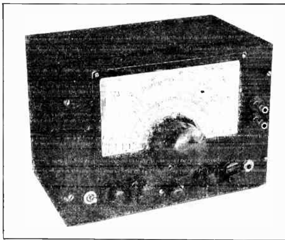
Fig. 1901 — Heterodyne frequency meter with built-in harmonic amplifier, crystal calibrator, and detector, usable on all amateur bands up to 141 Mc. Controls along the bottom of the panel are, from left to right, crystal-oscillator on-off switch, 100-1000-ke. crystal-selector switch, calibration range switch, drift compensator, harmonic-amplifier range switch, output control, headphone jack. The two output terminals are along the right-hand edge.
