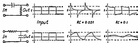
Fig. 359 — With square wave input, the voltage wave-shapes across R and C respectively in an RC circuit have the shapes shown. Note the variation in wave-shapes for different time constants. (Time constant values given are in terms of fractions of the period of the input wave.)
