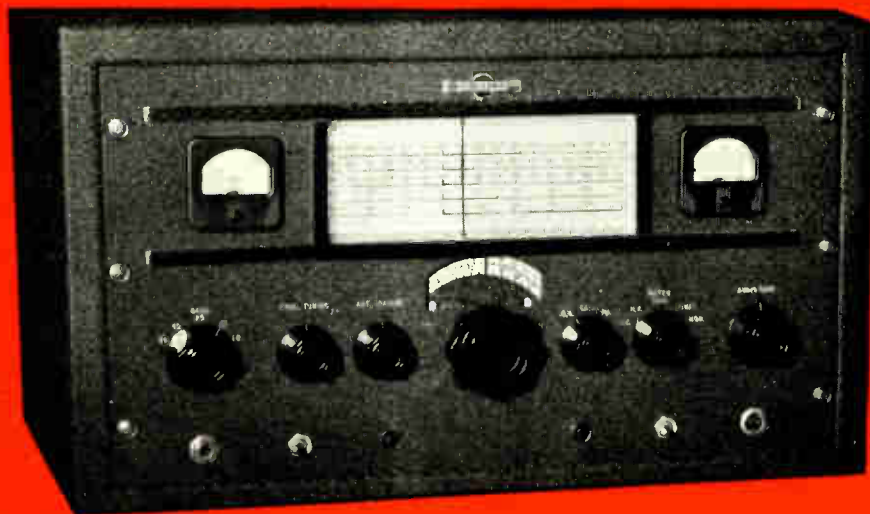
The Collins 32V-1 150 watt Transmitter
