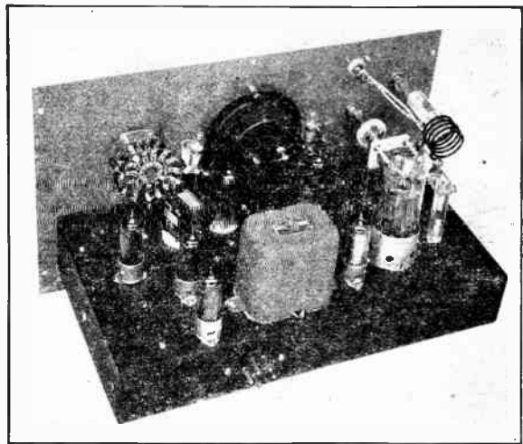
◆ Fig. 1619 — The plate circuit of the final stage of the mobile transmitter is the only r.f. circuit above the chassis. The three tubes at the left are the driver and audio stages, with the oscillator and multiplier tubes directly in back of the meter. The tube to the right of the modulation transformer is the 0A2 voltage regulator. Chassis size is 7 × 13 × 2 inches. ◆
