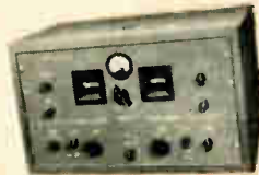
HAMMARLUND SP-400-X SUPER PRO Outstanding communications receiver for professional and amateur use, covering frequency range .54-30.0 mc.
