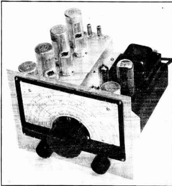
Fig. 1221 — A 28-Mc. converter that uses fixed-tuned r.f. stages and thus eliminates the ganging problem. The knob at left is for the "send-receive" switch, and the right-hand knob is for gain control.
