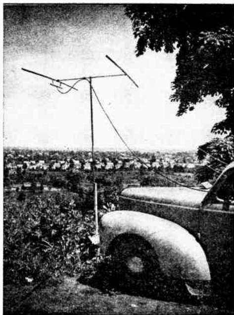
Fig. 1711 — A 2-element collapsible array for 50-Mc. portable use.
