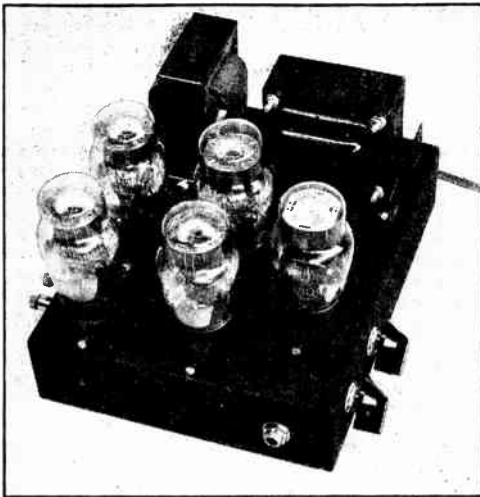
Fig. 1379 — A vacuum-tube keyer, built up on a 7 X 9 X 2-inch chassis with space for four or less keyer tubes and the power-supply rectifier. The resistors and condensers which produce the lag are mounted underneath, controlled by the knobs at the right. The jack is for the key, while terminals at the left are for the keyed circuit.
