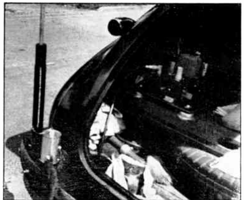
Fig. 20-32 — The base loading coil and tuning condenser mounted on the rear apron of W2NKK's car.
