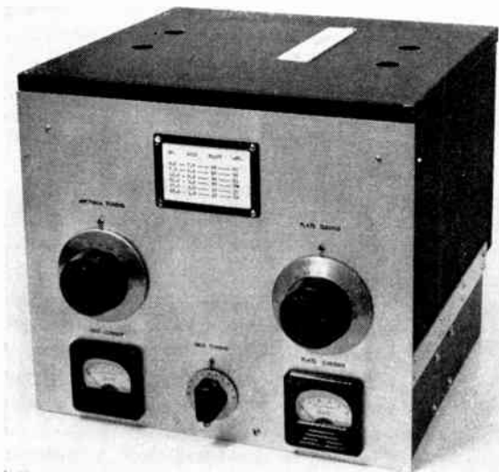
Fig. 6-95 — A multiband push-pull 807 amplifier and antenna tuner with no plug-in coils or switching. The aluminum strip on top covers the harmonic-trap adjusting holes. The other holes are for ventilation. The panel is a sheet of ⅜-inch aluminum 12¼ inches wide and 10½ inches high.
