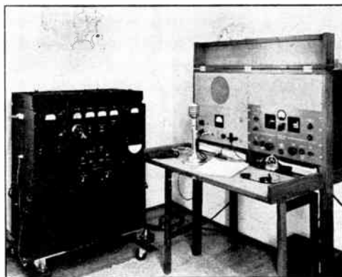
In this example of a compact high-power station, the operating table folds up when not in use and covers the receiver and speech amplifier. Special furniture, like this homemade operating table, goes a long way toward solving the space problem for many amateurs. (W1HAV, Fort Thomas, Ky.)
