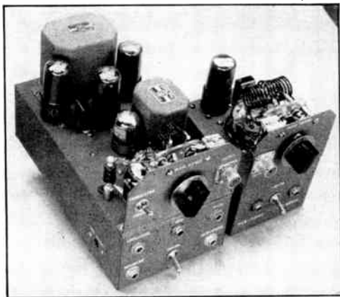
Fig. 17-22 — A 2-band set-up for mobile or low-powered fixed-station operation on 50 and 144 Mc. At the left is the 2-meter unit, complete with modulator. The smaller is the 50-Mc. r.f. section. Toggle switches permit use of the modulator with either r.f. section.
