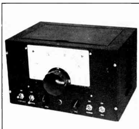
Fig. 21-3 — Additive frequency meter with self-contained power supply. The small knobs are for correction of drift so that both the 100-ke. crystal oscillator and VFO can be set to exact frequency. Dial calibration is in 1000-cycle intervals. This unit can be used for high-accuracy frequency measurement at all frequencies from 100 ke. through 30 Mc.
