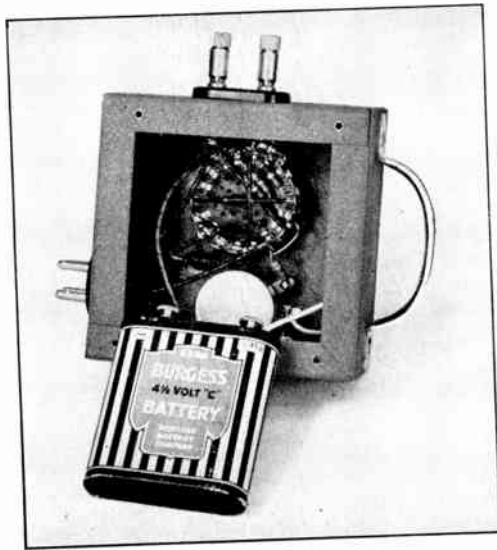
Fig. 21-19 — A rear view of the volt-ohm-milliammeter. The range-selector switch is mounted above the zero-adjustment potentiometer, and the shunts and multipliers are connected across the switch terminals. A four-prong male plug, for connection to the meter box, is shown at the left of the cabinet. The ohmmeter battery fits inside the case; the battery terminals should be insulated with tape or paper before the battery is installed in the box.
