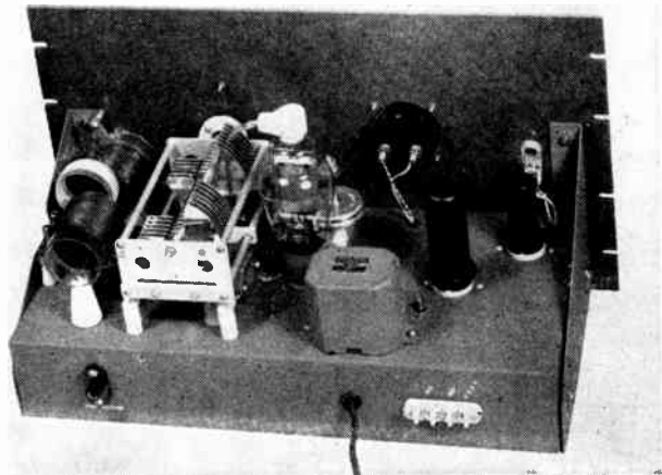
Fig. 6-80 — Rear view of the 1.8-Mc. transmitter. The construction of the amplifier plate coil and its swinging link is shown at the left. The plate r.f. choke and the plate by-pass condenser are mounted underneath the main tuning condenser, which is supported by 1-inch stand-off insulators. An insulated coupling is used between the rotor shaft of the condenser and the panel control. The neutralizing condenser is visible behind the amplifier tube.
