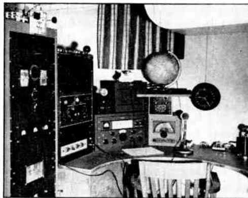
One of the most convenient station arrangements is to build a semi-circular operating table as shown here. All operating controls are readily available, and considerably more equipment can be grouped around the operator than when an ordinary desk is used. (W2SA1, Riverton, N. J.)
