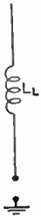
Fig. 20-31 — Placing the loading coil at the center of the whip antenna, instead of at the base, increases the radiation resistance, although a larger coil must be used.
