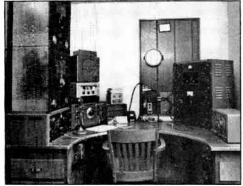
One of the most convenient station arrangements is to build a semicircular operating table as shown here. All operating controls are readily available, and considerably more equipment can be grouped around the operator than when an ordinary desk is used. ( W2S41, Riverton, N. J. )
