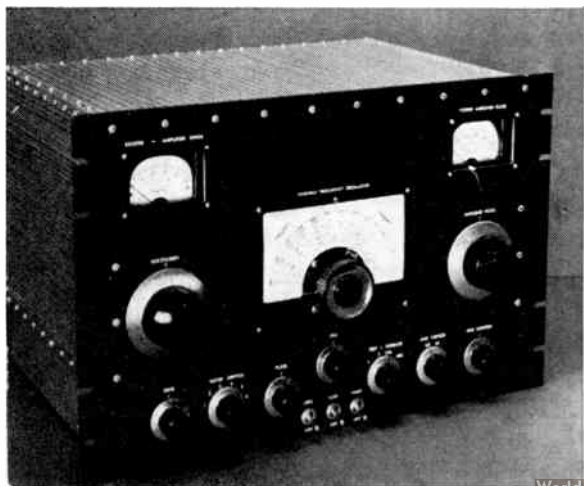
Fig. 6-53 — The standard-rack panel is 12\frac{1}{4} inches high. Controls (National HRS) along the bottom, centers spaced at intervals of 2\frac{3}{8} inches either side of center, are, left to right, for C_4 , S_3 , C_5 , C_2 , S_1 (Centralab 1405), S_2 and C_{10} . Power toggles are below at the center, spaced 1 inch apart. The calibrated VFO dial (National SCN) for C_1 is at the center, with the excitation control (National P dial) to the left, and the dial (National AM) for C_3 to the right. National CFA chart frames outline the rectangular openings for the recessed meters, 50-ma. to the left, 500-ma. to the right. The shielding enclosure is built up using aluminum angle, perforated sheet (also used for the bottom plate), and self-tapping screws.
