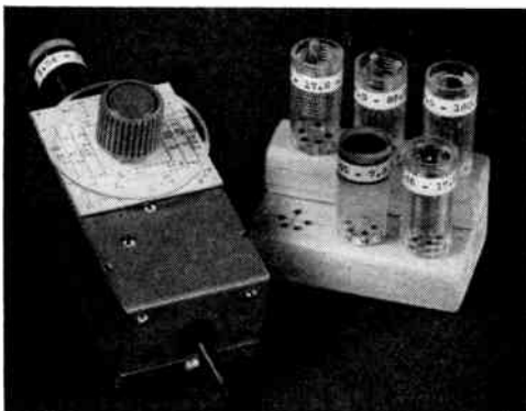
Fig. 21-20 — A compact and light-weight grid-dip meter for one-hand operation. It is built in a 1 5 / 8 × 2 1 / 4 × 4-inch "Channel-lock" box and uses six plug-in coils to cover the range 1600 kc. to 160 Mc. The power supply and milliammeter for reading grid current are in a separate unit.
