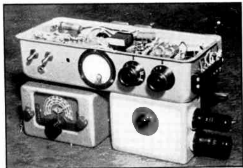
Fig. 12-16 — The crystal-filter SSB exciter, as designed for mobile work, complete with receiver converter and VFO. The top dish is the exciter (with cover removed). The meter reads cathode current to a pair of 807s driven by the unit, and the two knobs handle carrier reinjection and 6AG7 plate tuning. (WJFO/9, Nov., 1950, QST.)
