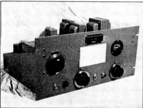
Fig. 6-75 — A beat-frequency exciter built by W6RZL. The dial at the left controls the frequency of the VFO and thereby the frequency of the exciter output. The other two dials are for the crystal-oscillator and amplifier-output tanks.
