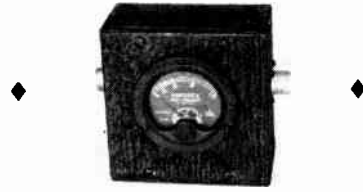
Fig. 21-28 — R.f. ammeter mounted for connecting into a coaxial line for measuring power. A "2-inch" instrument will fit into a 2 \times 4 \times 1 metal box. The shunt capacitance of an ammeter mounted in this way has a negligible effect on the accuracy at frequencies as high as 30 Mc. if the instrument has a bakelite case. Metal-cased meters should be mounted on a bakelite panel which can in turn be mounted in a cut-out which clears the meter case by about \frac{1}{4} inch.
