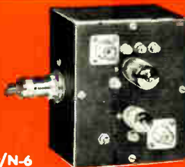
S/N-6 CASCODE 2-METER PRE-AMPLIFIER G-E Ham News, Nov.-Dec., 1952
