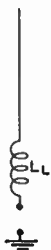
Fig. 20-28 — The capacitive reactance at frequencies lower than the resonant frequency of the whip can be canceled out by adding an equivalent inductive reactance in the form of a loading coil in series with the antenna.
