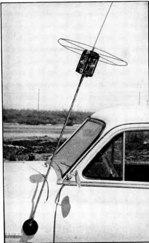
Fig. 20-32 — The top-loaded 4-Mc. antenna used by W6SCX. The loading coil is a B & W transmitting coil. The coil can be tuned by the variable link which is connected in series with the two halves of the coil.
