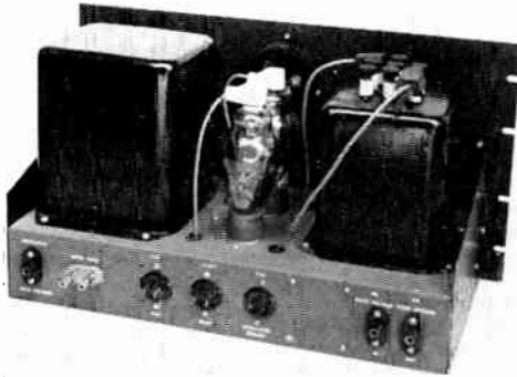
Fig. 9-28 — A typical Class B modulator arrangement. This unit uses a pair of 811As, capable of an audio power output of 340 watts, and includes a splatter filter. The modulation transformer is at the left and the splatter choke at the right. All high-voltage terminals are covered so they cannot be touched accidentally.
