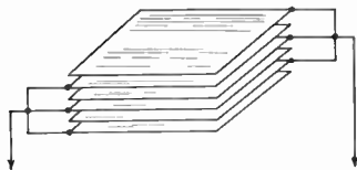
Fig. 2-9 — A multiple-plate condenser. Alternate plates are connected together.
