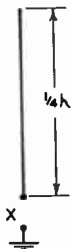
Fig. 20-26 — The quarter-wave whip at resonance will show a pure resistance at the feed point X.
