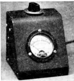
Fig. 21-23 — Power supply and milliammeter for the grid-dip meter are contained in a meter case. The control on top is for varying the plate voltage to maintain the grid current in the proper region.
