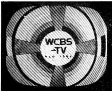
Fig. 23-8 — "Cross-hatching," caused by the beat between the picture carrier and an interfering signal inside the TV channel.
