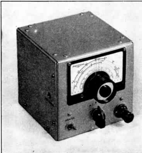
Fig. 20-10 — A bandswitching converter for 6, 10 and 11 meters. The pilot light at the lower right has an adjustable beam, for convenience in mobile work.
