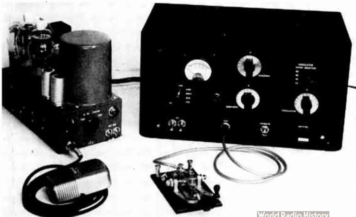
Fig. 9-16 — The 40-watt modulator alongside the 75-watt transmitter described in the transmitting chapter. It is completely self-contained, with power supply and control circuits, on a 5 × 10 × 3-inch chassis.
