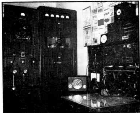
In this arrangement, the two receivers (with separate loudspeakers) and the transmitter VFO are all within easy reach of the operator, while the monitoring oscilloscope on the left-hand transmitter rack can be easily seen from the operating position. ( W7JU, Boulder City, Nev. )
