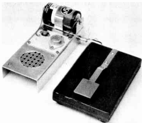
View of the code-practice set. The speaker mounts under the chassis and is protected by a piece of aluminum screening. Ordinary window screen will work here. The circuit board is mounted over a cut-out area in the chassis. Allow a ¼-inch overlap on all sides of the circuit board for mounting purposes. Four 4-40 bolts hold the board in place. The battery holder is a Keystone No. 175.
