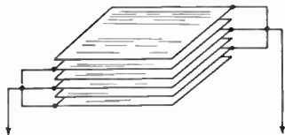
Fig. 2-9—A multiple-plate capacitor. Alternate plates are connected together.
