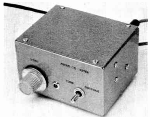
Fig. 7-9—This electronic speed keyer is 100 percent solid state and uses both integrated circuits and bipolar transistors. It operates over a speed range of 10 to 50 w.p.m. and contains its own built-in monitor.
