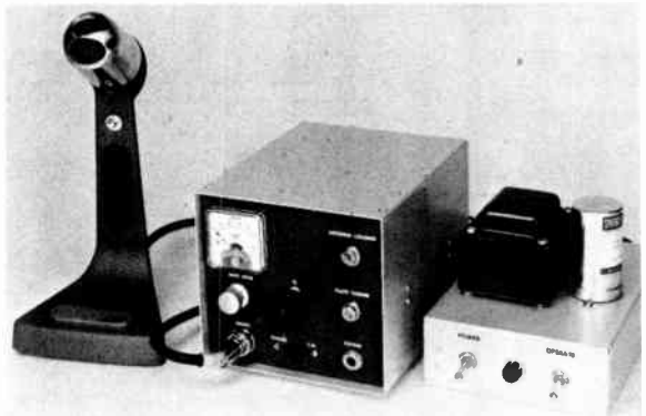
Fig. 6-55—The midget-size 160-meter phone/c.w. transmitter is dwarfed by the microphone next to it. A minimum number of controls are used; all are located on the front panel. A low-cost power supply for fixed-station use is shown at the right of the transmitter.
