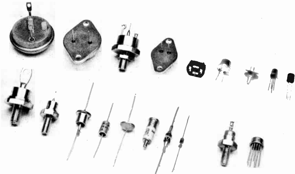
Representative semiconductor types. Various styles of transistors are shown in the back row. High-power types are at the left, medium-power types are at the center, and small-signal types are at the far right. At the extreme right in the back row is an epoxy-encapsulated field-effect transistor. The eight components at the left (in the front row) are silicon and germanium diodes in various package styles. The device at the extreme lower-right (with many leads) is an integrated-circuit assembly. Immediately to the left of it is a varactor diode.
