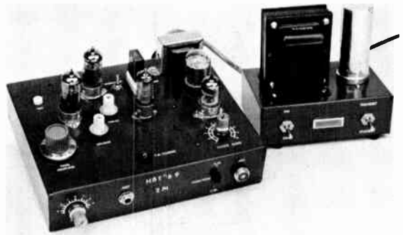
Fig. 17-12—Top-chassis view of the exciter and its power supply. The equipment is finished in dark gray enamel. The controls and jacks are identified by means of decal labels.
