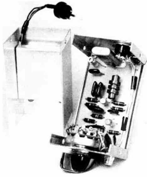
Fig. 21-14—Inside view of the frequency marker. The etched circuit board is mounted under the top of the case, allowing the adjustment screw on C_6 to be reached through a hole in the top. The bottom piece, left, has the battery supply mounted under a homemade aluminum clamp. Two penlite cells are wired in series for the 3-volt supply by soldering wires to the positive post and exposed negative container at the bottom. This wiring must be insulated from the case. The 9-volt supply is a transistor battery with clip-on connector.
