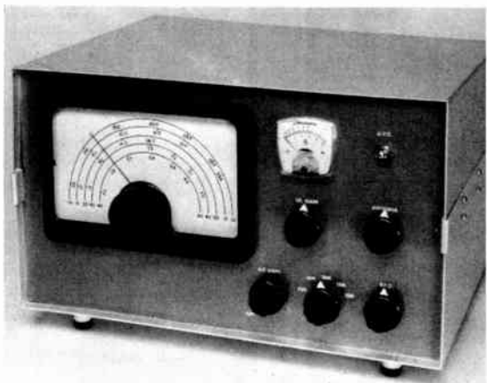
Fig. 5-56—This is a five-band receiver featuring a mechanical filter for selectivity. A two-speed dial (Miller MD-8) is fast enough for quick jumps around the band and slow enough for ease in tuning s.s.b. Audio-derived fast-attack slow-decay a.g.c. also contributes to ease of tuning.
