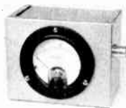
Fig. 21-31—R.f. ammeter mounted in a Minibox, with u.h.f. style connectors for placing meter in series with a coaxial line. The meter can be used for r.f. power measurements ( P = I^2 R ) when connected between a transmitter and a nonreactive load of known resistance.
