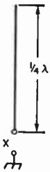
Fig. 19-29—The quarterwave whip at resonance will show a pure resistance at the feed point X.
