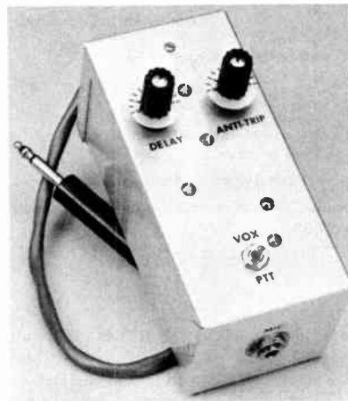
Fig. 9-22—The completed VOX unit. It goes between the microphone and the transmitter. The miniature knobs are Johnson Collet type 116-603.
