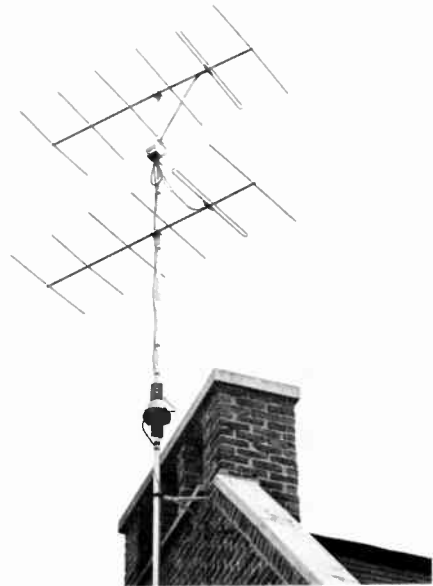
A stacked array for 144 Mc. (W1AW) which uses \frac{3}{8} -wavelength spacing. The phasing lines and the \frac{1}{2} -wavelength balun are joined in a weatherproof box. Element lengths for such an array can be taken from table 18-1. Element spacing is 0.2 wavelength.
