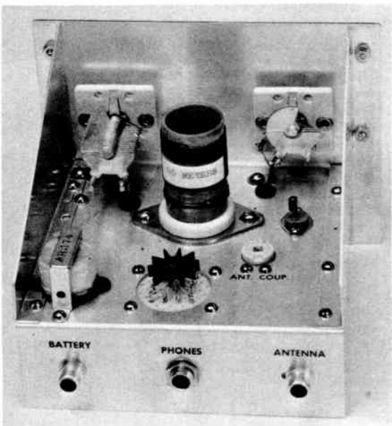
Fig. 5-48—Top-chassis view of the receiver. Q_1 is visible at the upper right, in front of the bandspread capacitor. The plug-in coil is at the center of the chassis, just to the left of Q_1 . C_3 , the main tuning capacitor, is at the left of the coil form. Output transformer T_2 is at the lower left of the chassis. AR_1 is just to the right of T_2 , crowned by is radial-fin heat sink. J_1 , J_2 , and J_3 are on the rear lip of the chassis. C_1 is visible in the right foreground, ahead of, but between, the plug-in coil and Q_3 .
