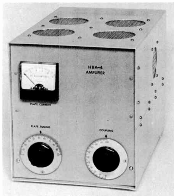
Fig. 6-60—The amplifier has one vent hole on each side of the home-made cabinet, and four holes on the top. Each hole, and the back side of the cabinet, is enclosed by means of perforated aluminum. The cabinet was formed by making two U-shaped sections of \frac{1}{16} -inch thick aluminum and mating them. They are held together by means of two 1-inch wide aluminum strips (inside) and 4-40 hardware.
