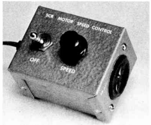
Fig. 20-B—Small enough to fit in the palm of your hand, the SCR motor-speed control is housed in a small Minibox.
