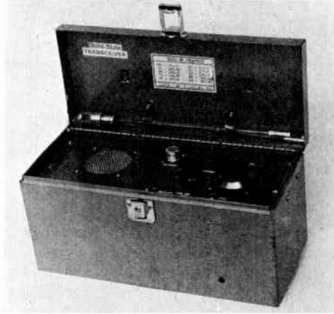
Fig. 19-19—The 2-meter transceiver is housed in a legal-bond box. A home-made dial-calibration chart for the receiver is pasted on the inside of the lid. Two plastic cable clamps serve as holders for the two-section \frac{1}{4} -wavelength whip antenna (inside lid) when the unit is not in use. The antenna is held together at the center by a home-made \frac{1}{4} -inch diameter threaded coupling.
