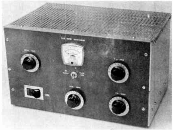
Fig. 9-38—The transceiving converter is housed in a homemade aluminum cabinet which measures 8 × 8 × 12 inches. Perforated aluminum is used for the top and back sides of the cabinet to assure good ventilation.
