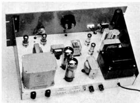
Fig. 8-15—A look at the top of the modulator chassis. The power supply is located on the right, the speech amplifier tubes are at the upper left, and the modulation transformer is at the lower left. The control relay, K_1 , is at the center of the chassis, just behind the meter.
