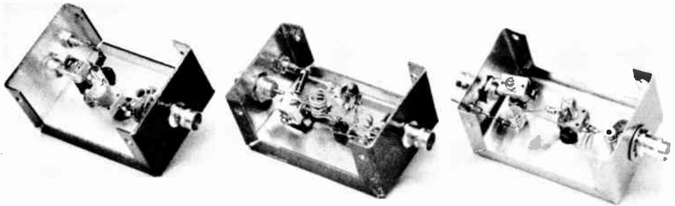
Fig. 16-22—Interiors of the FET preamplifiers, in the same order as in Fig. 16-20. The input end is toward the left in each unit.
