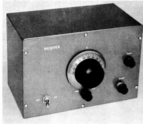
Fig. 5-51—The large vernier dial at the center of the panel is the main-tuning control. The on-off switch is at the lower left, the band switch at the lower center, and the gain control is at the lower right. A peaking control is directly above the gain control.
