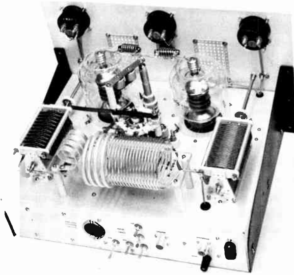
Fig. 6-67—Top view of the 3-500Z amplifier. The plate-tuning control is at the far left, the tank inductor is at the lower center of the photo, and the loading capacitor is to the right of the tank coil. The two paralleled plate-blocking capacitors are mounted on the copper strap which is attached to the top of the plate r.f. choke (between the two 3-500Zs). Each tube uses a heat-dissipating anode connector and a glass chimney. Metal cans enclose the backs of the panel meters, but these were removed for the photo.
