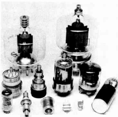
Transmitting tubes are in the back and center rows. Receiving tubes are in the front row (l. to r.): miniature, pencil, planar triode (two), Nuvistor and 1-inch diameter cathode-ray tube.
