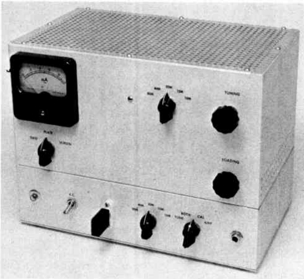
Fig. 6-41—The five-band 50-watt transmitter is a two-tube unit much superior to the "simple 1-tube" transmitters often recommended for newcomers to amateur radio. The cabinet combines a chassis and an aluminum "utility box."
