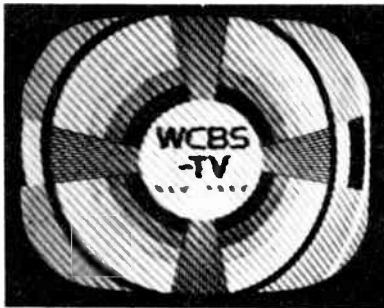
Fig. 23-5—"Cross-hatching," caused by the beat between the picture carrier and an interfering signal inside the TV channel.
