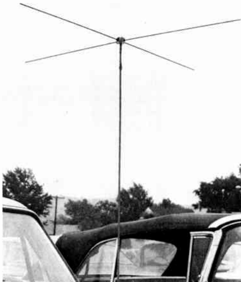
Two-meter turnstile antenna shown mounted on the front of an automobile. The miniature coax cable which feeds the antenna is taped to its \frac{1}{4} -inch diameter steel supporting rod. The ends of the antenna elements should be flattened, or rounded, to make them safer in the event of accidental contact with the human body.
