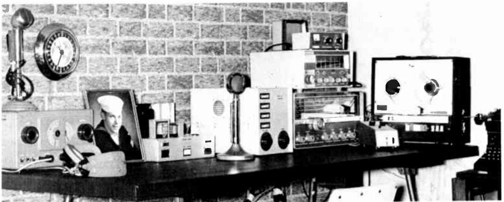
A convenient and inexpensive operation position can be made by purchasing an unfinished door panel, attaching wooden or wrought iron legs, and finishing the surface of the table with a coat of spar varnish or similar heavy-duty material. This station is owned by W1CKK and WN1HTY of Meriden, Conn.
