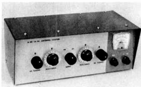
Fig. 18-19—This 6- and 2-meter antenna coupler has a built-in s.w.r. bridge and permits power levels up to 500 watts. This unit will work with balanced or unbalanced feeders.
