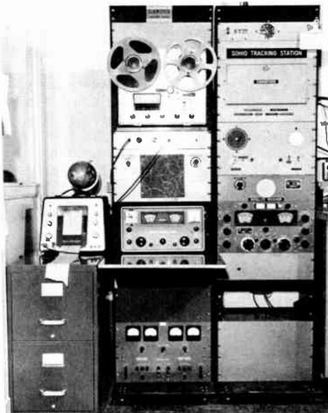
This modern-day satellite-communications station is used by the Sohio Moonbounce group. This photo, submitted by W8FKC, shows a pen recorder at the left, a tape deck at the right of the pen recorder. This rack-and-panel installation is neat and functional, placing all of the equipment within easy reach of the operator.
