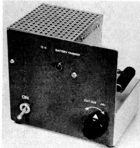
Fig. 12-35—This battery charger is built on a 4 x 5 x 6-inch aluminum chassis and has a home-made panel. The power transformer is enclosed (left side of the chassis) to lessen shock hazard. The small parts are mounted on perforated board and the assembly is located under the chassis. R_1 is visible at the far right.
