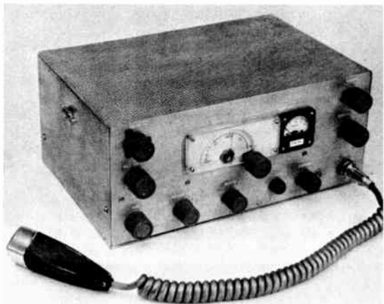
Fig. 9-26—This model was constructed by W5RQJ. The dial is homemade, but may be replaced by a conventional type. At the left-hand end of the panel are the loading and tuning controls of the pi-network output circuit; at the right-hand end are controls for receiver and transmitter audio. Along the bottom, from left to right, are receiver r.f. trimmer, mobile power relay switch, buffer tuning control, and modulator balance control.
