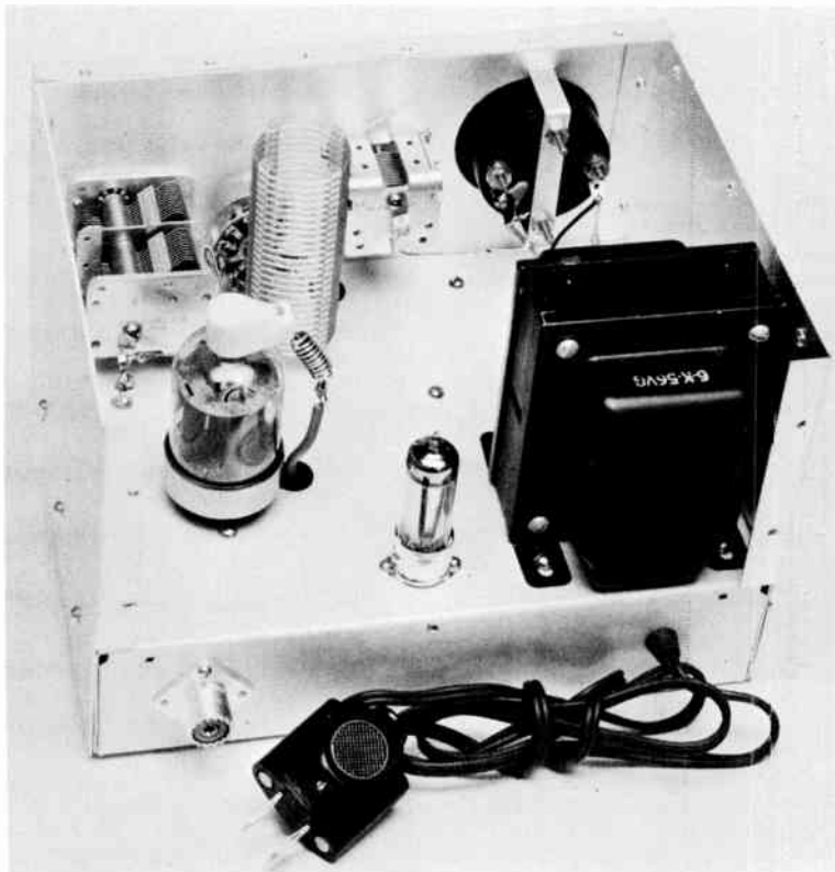
The tank-circuit components are grouped in the front left corner, just in front of the 6146. M_1 is at the upper right on the panel. At the rear is the power transformer with the regulator tube mounted just to the left of T_1 .
