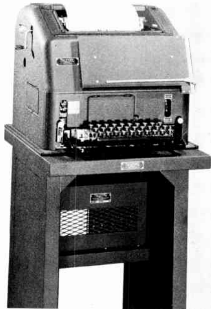
The Model 15 page printer, shown here with table, is used in a great many RTTY stations.
