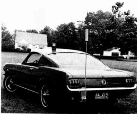
Fig. 19-35—A field-strength meter is placed on the car roof and is used to indicate maximum output when tuning the antenna to resonance. In this installation, a telescoping antenna section is used above the loading coil. The length of the top section is varied until its capacitance provides resonance in combination with the fixed-inductance, weatherproof-loading coil. This photo shows a temporary mobile mount made from 1/8-inch thick steel plate which has been bent to catch on the top lip of the bumper. The lower portion attaches to the car body with two 1/4-inch diameter bolts.
