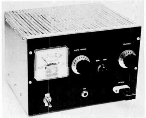
The one-tuber makes a neat package. The plate-tuning capacitor is just to the right of the meter. The loading capacitor is at the far right. Across the bottom from the left are the a.c. switch, key jack, and crystal socket, in that order.
