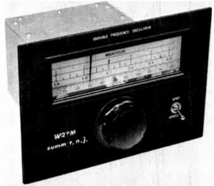
Fig. 6-46—The FET v.f.o. The panel is 1/8-inch aluminum, 7 by 10 inches. (Designed and built by G. D. Hanchett, W2YM.)
