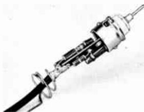
Fig. 21-37—Close-up of the inside of the probe. The 1N34A crystal diode rectifier, calibrating resistor, and input capacitor are mounted tight to the terminal strip with shortest leads possible. Spaghetti tubing is placed on the diode leads to prevent accidental short circuits. The tube-shield spring and flexible-copper grounding lead are soldered to the cable braid (the cable is RG-58/U coax). The tip can be either a phone tip or a short pointed piece of heavy wire.
