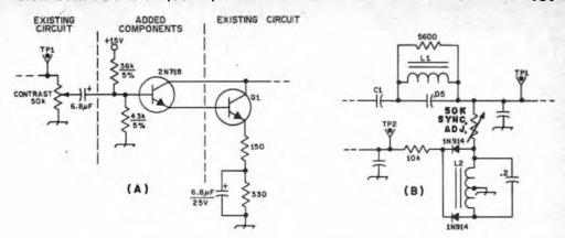
Fig. 2 — At A, a circuit which may be added to increase the contrast of the SSTV adapter, and at B, an alternative circuit using surplus 88-mH toroidal inductors for L1 and L2. If the circuit of A is used, the 18,000- and 22,000-ohm resistors shown connected to the base of Q1 in Fig. 1 are unnecessary.
