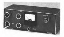
Exterior view of the QRP Transmatch. The cabinet is homemade from solid sheet and perforated aluminum stock. The two controls at the far left are 365-pF variables, as is the one at the lower left of the Simpson meter. At the upper left of the meter is the variable-inductance control. Directly under the meter is the meter-sensitivity potentiometer. The bridge function switch is visible at the upper right of the panel. Kurz-Kasch aluminum knobs are used on the controls,
