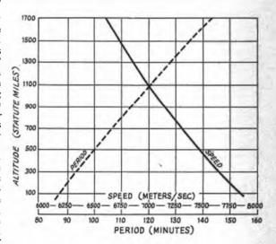
Fig. 15E-4 — Satellite altitude versus its period (time for one revolution) and speed.
