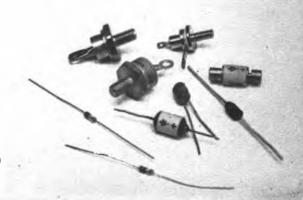
Typical silicon and germanium diodes of the present era. The larger units are designed to handle high current.
