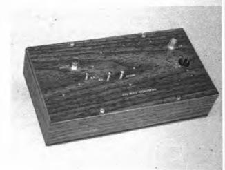
Fig. 1 — The 432-MHz converter is built on the cover plate of a standard aluminum chassis. The "cigar-box effect" results from application of contact paper with simulated wood-grain finish to all exposed surfaces.
