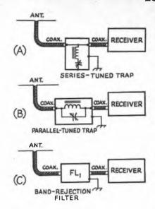
Fig. 8-31 — Examples of series- and parallel-tuned single-frequency traps (installed) are shown at A and B. At C, FL1 represents the band-rejection filter described in the text. If possible, the filter used should be bolted to the chassis or case of the receiver. The receiver should have a good earth ground connected to it.
