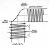
Fig. 14-12 — Representation of limiter action. Amplitude variations on the signal are removed by the diode action of the grid- and plate-current saturation.
