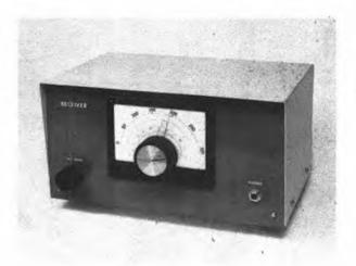
Exterior view of the three-band beginner's receiver. The dimensions are 11×5-1/2×7 inches. The vernier dial is calibrated for 10 kHz per division. The front panel is finished in dark blue. White press-on decals are used to identify the gain control and phone jack. The receiver was built by WA1CQW.
