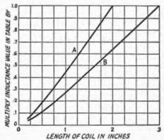
Fig. 2-15 — Factor to be applied to the inductance of coils listed in the table below, as a function of coil length. Use curve A for coils marked A, and
