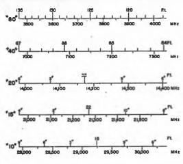
Fig. 21-4 — The above scales, based on Eq. 21-B, can be used to determine the length of a half-wave antenna of wire.
