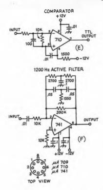
Fig. 4-34 — Some typical applications of operational amplifiers. The pin numbers shown are all for the metal can (TO-99) package.
