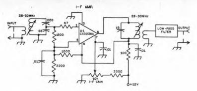
Fig. 4 — Circuit for an IC i-f amplifier that has manual gain control, and which can be used between the converter of Fig. 1 and the tunable i-f receiver. See the text for a discussion of this circuit. This amplifier can provide an additional 25 dB of gain.
