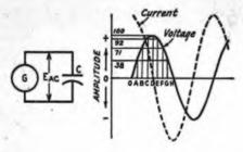
Fig. 2-26 — Voltage and current phase relationships when an alternating voltage is applied to a capacitor.
