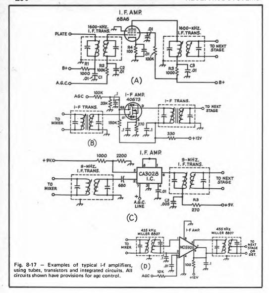
device reduces the gain of the stage. To realize maximum gain when no age voltage is present, it is necessary to apply approximately 3 volts of positive dc to gate 2. Neutralization is usually not required with a MOSFET in i-f amplifiers operating up to 20 MHz. Should instability occur, however, gate 1 and the drain may be tapped down on the i-f transformer windings.
