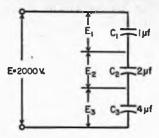
Fig. 2-11 — An example of capacitors connected in series. The solution to this arrangement is worked out in the text.
