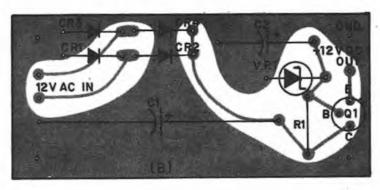
C3 must reach past the ground hole and connect to the foil. R3 is not used on the six-meter converter.
