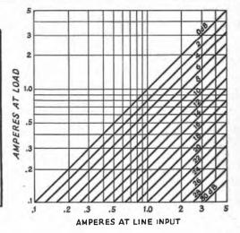
Fig. 20-9 — Graph for calculating losses in transmission lines with an SWR of 1.
