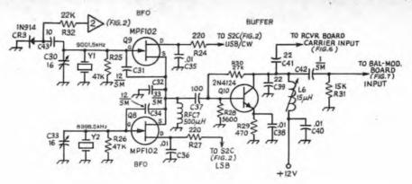
Fig. 5 – Carrier oscillator board.
