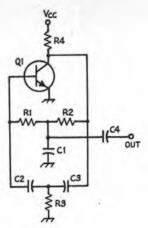
Fig. 17-23 — Twin-T audio oscillator circuit. Representative values for R1-R2 and C1 range from 18k  $\Omega$  and .05  $\mu$ F for 750 Hz to 15k  $\Omega$  and .02  $\mu$ F for 1800 Hz. For the same frequency range, R3 and C2-C3 vary from 1800 ohms and .02  $\mu$ F to 1500 ohms and .01  $\mu$ F. R4 should be approximately 3300 ohms. C4, the output coupling capacitor, can be .05  $\mu$ F for high-impedance loads.
