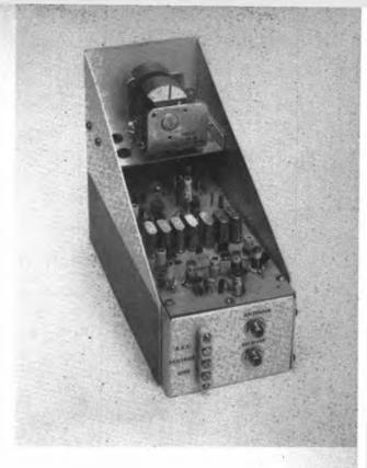
Fig. 8-51 — The front-end tuning capacitor, C1, is mounted on a small shelf just above the toroid coils. The rear section of the main circuit board contains the crystal oscillator. The crystals are soldered directly into the board. The capacitors that go with the oscillator-tank coils are connected across the terminals of the pc-mount coil forms. Most of the chokes and resistors are mounted vertically to save space.
