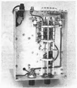
The bottom view of the VFO shows only the two switches and the output transformers — other components are mounted on the etched circuit boards "topside."
