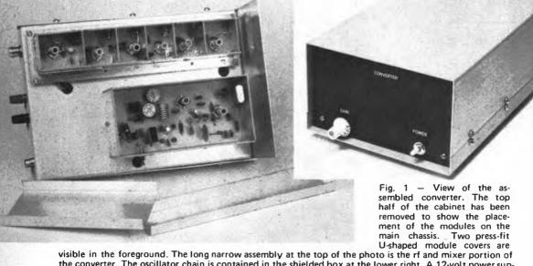
visible in the foreground. The long narrow assembly at the top of the photo is the rf and mixer portion of the converter. The oscillator chain is contained in the shielded box at the lower right. A 12-volt power suply or IC i-f amplifier (see text) can be built in the vacant space at the lower left of the chassis. The completely assembled unit is shown in the inset.
