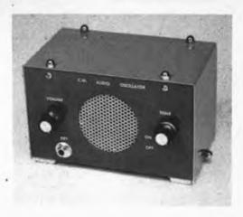
A cw code-practice oscillator along with a speaker may be mounted inside a homemade aluminum box. If desired, the battery could be mounted inside the enclosure also, thereby allowing easy portability of the unit.
