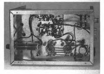
The bottom view of the chassis, the sockets for the 6146B tubes are at the lower center. The etched-circuit board is above the final amplifier tube sockets and the T-R relays at the upper right. The different supply voltages are obtained from the associated transceiver.
