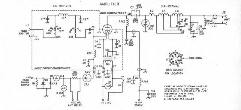
Fig. 1 — Circuit diagram of the 2-kW amplifier. Component designations not listed below are for text reference. The values for C1, C2, and L1 are given in Table 1.
