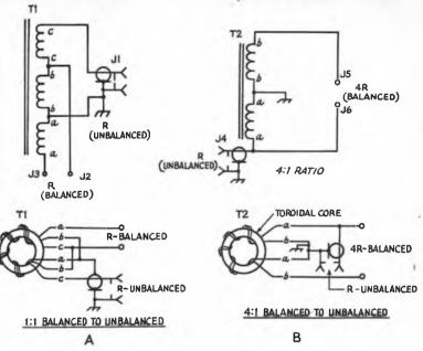
Low-loss high-frequency ferrite core material is used for T1 and T2.1.3 The cores are made from Q-2 material and cost approximately \$5.50 in single-lot quantity. They are 0.5 inches thick, have an OD of 2.4 inches, and the ID is 1.4 inches. The permeability rating of the cores is 40. A packaged one-kilowatt balun kit, with winding instructions for 1:1 or 4:1 impedance transformation ratios, is available, but uses a core of slightly different dimensions.<sup>2</sup>
