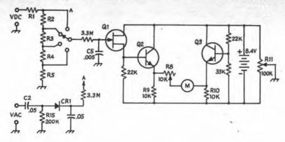
Fig. 17-9 — Electronic voltmeter using field-effect transistor for high input resistance. Components having the same functions as in the VTVM circuit of Fig. 17-8 carry the same designations. (Circuit is
