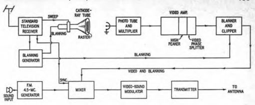
Fig. 15B-1 - Block diagram of the television system used by W2BK, formerly W2LNP. (From QST, June, 1950.)
