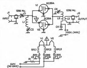
Fig. 7-43 — Representative circuit of the 1296-MHz cavity amplifier. The plate cavity and tuning device are indicated by L2,C3, the cathode inductance and tuning capacitor by L1,C2. Note that the heater supply must not be grounded.
