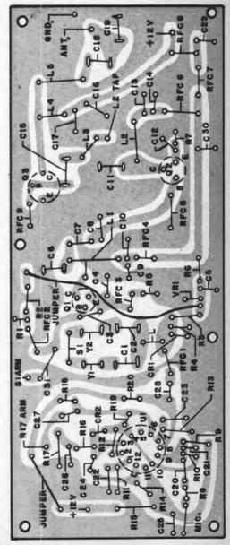
Foil-side view parts layout for the transmitter drawn to full scale. Template and
