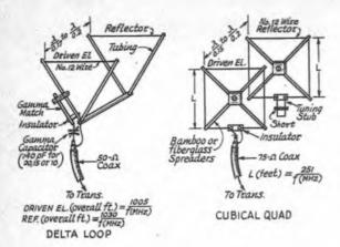
capacitance required is usually 140 pF at 14 MHz and proportionately less at the higher frequencies.
