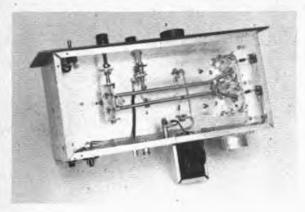
Fig. 7-33 — The principal feature of the bottom view is the half-wave grid circuit. Its split-stator capacitor, C2, is at the left end of the line, L2. The differential balancing capacitor, C3, is also across the line, just to the right of C2. Isolating resistors in the grid circuit, R1, and R2, are near the middle of the picture. The screen isolating resistors, R3 and R4, run to tie points on the right wall of the chassis.
