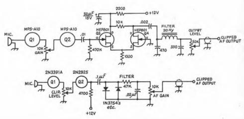
Fig. 13-19 — This drawing illustrates use of JFETs or silicon diodes to clip positive and negative voice peaks.
