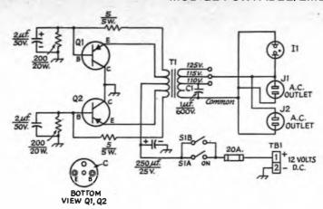
Fig. 10-30 — Schematic diagram of the inverter. Capacitance is in  $\mu$ F. Polarized capacitors are electrolytic. Resistance is in ohms.
