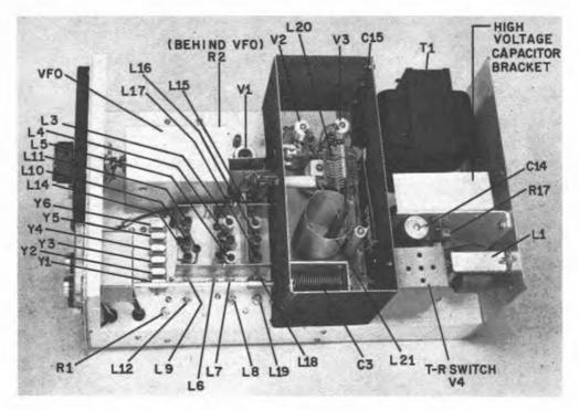
Fig. 3 - Top view of the cw transmitter.
