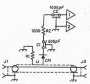
Fig. 22-25 — Circuit diagram for the line sampler.
