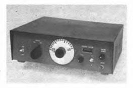
Exterior view of the two-band 10-watt transmitter. A homemade aluminum box is used to house the circuit. The cover has been sprayed with black paint. The panel is gray. White press-on decals are used to identify the controls. A small LED is used as a panel lamp. It is located just above the on-off switch.
