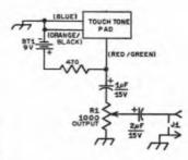
Fig. 14-34 — Typical connections to use a Touch-Tone pad for repeater control. Resistances are in ohms. R1 is a linear-taper composition control and J1 is a panel-mounted phono jack. Capacitors are electrolytic; color coding on the wire leads from the pad is shown in parentheses.
