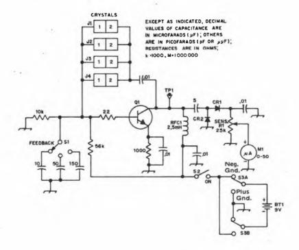
Fig. 1 — Schematic diagram of the No. 2 tester. Capacitors are disk ceramic. Fixed-value resistors are 1/2 or 1/4-watt composition. Estimated cost for this tester (all new parts) is \$13.
