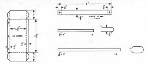
Fig. 7-36 — Flashing-copper parts used in the 2-meter amplifier, Broken lines indicate 90-degree bending required. The surfaces of the C4 rotor are soldered together after bending, for rigidity. The anode clamps, upper right, wrap around the tube cooling ring, and hold the brass tabs (Fig. 7-35) firmly in place. L1 and L4 are shown in the approximate shape, after bending, at the right.
