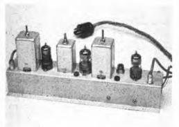
Fig. 14-20 — The fm adapter, wired for connection to a Collins 75A2.
