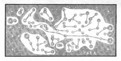
Fig. 6- Scale-size layout for the pc board. The same pattern is used for either band. Foil side shown here.
