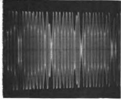
Fig. 3 — Waveform displayed at the output of a Kenwood TS-520 transceiver. The word "hello" is being spoken in each case. (A) Unprocessed signal with the TS-520 set for maximum amplitude display. (B) TS-520 output under fully limited conditions set by the Quasi-Logarithmic Limiter Processor. (The TS-520 was provided by Henry Radio, Inc.)
