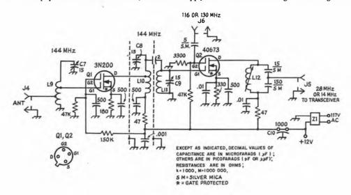
Fig. 7-10 — Diagram of the converter section. Resistors are 1/4-watt composition and capacitors are disk ceramic, except as noted otherwise. C7-C9, incl. — Air variable, pc mount (Johnson
