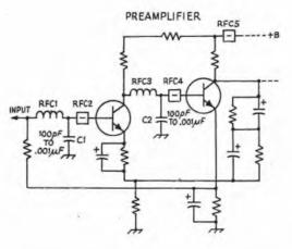
Fig. 16-4 — Typical circuit of a solid-state preamplifier.
