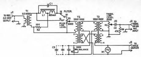
Fig. 1 — Schematic diagram of the phone-patch circuit. Resistances are in ohms, k=1000. Fixed resistors may be 1/2 watt, 10 percent tolerance. Capacitance is in microfarads. Components not listed below are identified for text reference.
