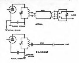
Fig. 16-19 — The stray capacitive coupling between coils in the upper circuit leads to the equivalent circuit shown below, for vhf harmonics.
