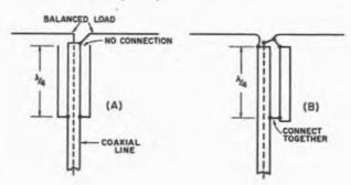
Fig. 22-3 — The balun conversion function, with no impedance change, is accomplished with quarter-wave lines, open at the top and connected to the coax outer conductor at the bottom. Coaxial sleeve, A, is the preferred type.
