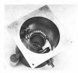
Fig. 7-47 — Interior of the plate circuit assembly, showing the center conductor with its ring of finger stock, the output-coupling loop, left, and the disk-type tuning capacitor, right.
