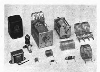
Inductors for power and radio frequencies. The two iron-core coils at the left are "chokes" for power-supply filters. The mounted air-core coils at the top center are adjustable inductors for transmitting tank circuits. The "piewound" coils at the left and in the foreground are radio-frequency choke coils. The remaining coils are typical of inductors used in rf tuned circuits, the larger sizes being used principally for transmitters.
