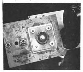
Fig. 7-37 — View of the top of the assembled amplifier. Teflon bushings hold the square capacitor plate in place on the wall of the cavity. One bushing is not shown. The high voltage and rf choke connect to that bushing's screw when it is in place. Plate-tuning adjustments are made from the bottom of the cavity. The shaft for C3 is accessible on the bottom wall of the cavity. This amplifier was designed and built by H. E. Holshouser, Jr., K4QIF.
