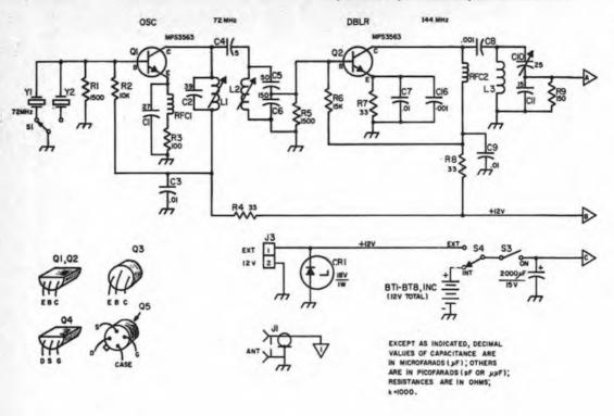
Fig. 3 - Schematic of the 2-meter transceiver, Fixed-value capacitors are disk ceramic except those with polarity marking, which are electrolytic. Resistors are 1/2-watt composition. Component numbering is for identification of parts on the circuit-board templates. Significant parts are listed below in the usual manner.
