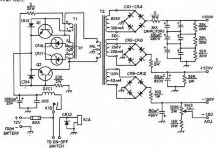
Fig. 10-28 — Circuit diagram of the mobile power supply. Polarized capacitors are electrolytic, others are paper or mica. Resistances are in ohms. Component designations not listed below are for text reference.
