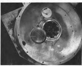
Fig. 7-41 — Inside view of the K4QIF amplifier cavity. The stationary capacitors, C2 and C4, are located on either side of the 4CX250 socket.
