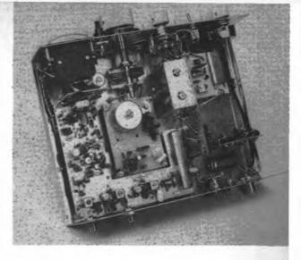
preamplifier, the gain of which has been compromised purposely by tapping the gate down on the output of FL2. This stage, Q4, compensates for the insertion loss of FL2 and establishes the noise figure of the i-f strip. An MPF102 was selected because of its low-noise characteristics. It is unconditionally stable without being neutralized, because the gate is tapped down at low impedance. A single-tuned 455-kHz i-f transformer is used to couple the output from Q4 to the input of U1.
