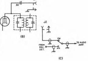
switch. to the fm adapter and adjust the discriminator transformer for best suppression of the noise pulses. If the alignment with the signal generator has been completed properly, only a half a turn or so of the slugs will be needed to complete the phase tuning of the discriminator.
