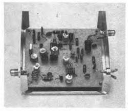
Fig. 1 — The 220-MHz converter is mounted in a box made from sheet aluminum. A phono jack at the lower left is the input connection. Another jack at the upper right is the output to the receiver. The i-f output coil shown here is for use with a low-band receiver. Changes necessary to work into a 2-meter receiver are explained in the parts list and text.
