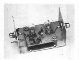
The 2-meter preamp, may be mounted in a small Minibox or connected directly inside an fm receiver.
