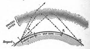
Fig. 19-4 — Refraction of sky waves, showing the critical wave angle and the skip zone. Waves leaving the transmitter at angles above the critical (greater than A) are not bent enough to be returned to earth. As the angle is decreased, the waves return to earth at increasingly greater distances.
