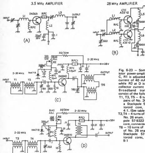
Fig. 6-23 - Some typical transistor power-amplifier circuits. At C. R1 is adjusted for a collector current of 40 mA with no drive. while R2 at D is set for 20 mA collector current with no input. Broadband transformers used consist of the following:
