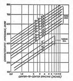
Fig. 20-7 — Chart showing the characteristic impedance of spaced-conductor parallel transmission lines with air dielectric. Tubing sizes given are for outside diameters.
