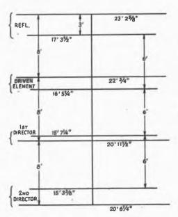
Fig. 21-44 — The element lengths shown are for the phone sections of the bands. Table 21-II provides the dimensions for cw frequencies.
