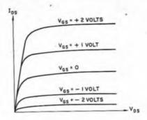
Fig. 4-21B-Typical MOSFET characteristic curves.
