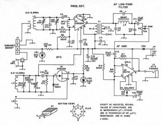
Fig. 2 — Schematic diagram of the tunable if portion of the receiver. Capacitors with polarity marked are electrolytic. Fixed-value capacitors are disk ceramic unless otherwise noted. Numbered parts not appearing below are so identified for pc-board layout purposes only.
