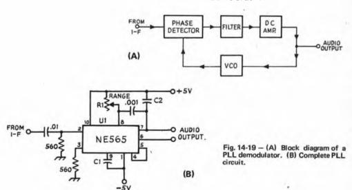
out of lock. The NE565 has an upper frequency limit of 500 kHz; for higher frequencies, the NE561, which is usable up to 30 MHz, can be employed.
