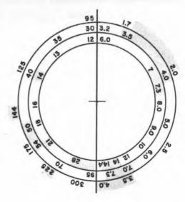
Fig. 17-45 — This dial chart may be copied full size and used as shown in Fig. 17-42 provided the tuned-circuit parts are exactly as specified in Fig. 17-43 and the construction duplicates Fig. 17-44.
