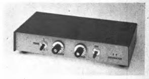
Fig. 17-33 — The two-tone audio test generator. Subminiature controls and switches are used on the front panel. The box is homemade; it consists of two U-shaped pieces of sheet aluminum, one forming the chassis, the other the cover. Overall size is 7 1/2 X 4 1/4 X 1 1/4 inches. For appearance's sake, the top cover overhangs the front panel by 1/4 inch. The controls adjust the output level and balance the relative tone levels.
