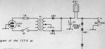
Fig. 1 — Schematic diagram of the 117-V ac charger.
