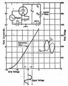
Fig. 3-8 — Amplifier operation. When the plate current varies in response to the signal applied to the grid, a varying voltage drop appears across the load,  $R_{\mathbf{p}}$ , as shown by the dashed curve.  $E_{\mathbf{p}}$ .  $I_{\mathbf{p}}$  is the plate current.
