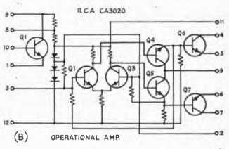
Fig. 4-24 — At A, a representative circuit for a typical differential IC. An Operational Amplifier IC is Illustrated at B, also in representative form.
