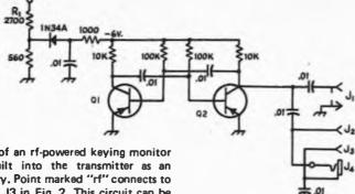
Fig. 5 — Circuit of an rf-powered keying monitor that may be built into the transmitter as an operating accessory. Point marked "rf" connects to the antenna jack, J3 in Fig. 2. This circuit can be used with any transmitter simply by selecting an input resistor, R1, that gives about —6 volts at the point shown. Only the desired output jacks need to be included.
