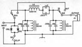
when designing this filter. The attenuation of 120-Hz power supply hum is in excess of 50 dB. Hum resulting from 60-Hz pickup in the receiver audio system is attenuated by more than 70 dB.
