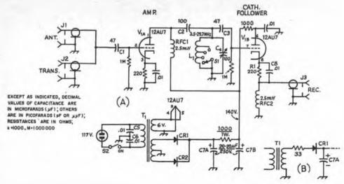
Fig. 2 — Circuit diagram of the T-R switch. Unless otherwise specified, resistors are 1/2 watt; decimal value fixed capacitors are disk ceramic, others are mica with the exception of C7, which is electrolytic. B — method of using a half-wave transformer for T1. Circuit designations not listed below are for text reference.
