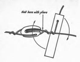
Fig. 21-61 — Using a lever for twisting heavy guy wires.
