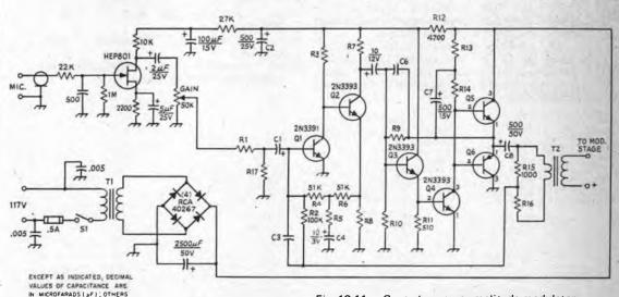
Fig. 12-11 — General-purpose amplitude modulator for 3 to 20 watts of audio power. Capacitors with polarity indicated are electrolytic. See Table 12-1 for parts not listed below.
