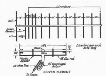
Fig. 22-12 — High-performance long Yagi for 144 MHz, from experimental work by W2NLY and W6QKI. Dimensions are for maximum galn between 144 and 145 MHz.
