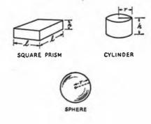
Fig. 2-64 — Forms of cavity resonators.
