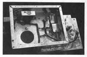
Fig. 7-38 — Inside view of the amplifier. The grid circuit and filament transformer are inside the chassis. Plate and output-tuning adjustments are made from the bottom of the cavity (far right).
