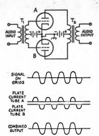
Fig. 3-13 — Class B amplifier operation.
