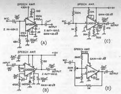
Fig. 13-13 — Typical speech amplifier using integrated circuits.
