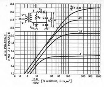
Fig. 5-18 — Dc output voltages from a full-wave voltage-doubling circuit as a function of the filter capacitances and load resistance. For the ratio R<sub>s</sub>/R and for the RC product, resistances are in ohms and capacitance is in microfarads. Equal resistance values for R<sub>s</sub> and equal capacitance values for C are assumed.
