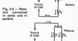
In the lower drawing the current flows to the common connection point at the top of the two resistors and then divides, one part of it flowing through R1 and the other through R2. At the lower connection point these two currents again combine; the total is the same as the current that flowed into the upper common connection. In this case the two resistors are connected in parallel.
