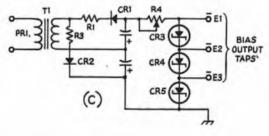
Fig. 5-29 — Circuits of typical bias supplies using solid-state rectifiers. The circuit at B is preferred if the bias is to be supplied to a Class C amplifier stage. Zener-diode regulation is shown at C.
