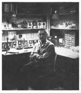
This modern-day operating position was built by KØGKB, of Boulder Colorado. Installing a desk in a corner allows a large amount of table-top area, to be within reach of the operator. Shelves mounted above the operating position provide convenient storage space for books and station accessories.
