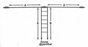
Fig. 21-17 — Practical arrangements of a shortened antenna. When the total length, A + B + B + A, is the same as the antenna length plus twice the feeder length of the center-fed antennas of Table 21-1, the same type of coupling circuit will be used. When the feeder length or antenna length, or both, makes the sum different, the type of coupling circuit may be different but the effectiveness of the antenna is not changed, unless A + A is less than a quarter wavelength.
