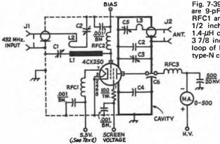
Fig. 7-39 — Schematic of the amplifier. C1 and C2 are 9-pF miniature variables (Johnson 160-104). RFC1 and RFC2 are each 8 turns of No. 16, enam, 1/2 inch diameter and 1 inch long. RFC3 is a 1.4-µH choke. L1 is a brass strip, 1/16 inch thick, 3 7/8 inches long, and 1 1/4 inches wide. L2 is a loop of No. 12 wire, 6 inches overall. J1 and J2 are type-N chassis connectors. B.M. = button mica.
