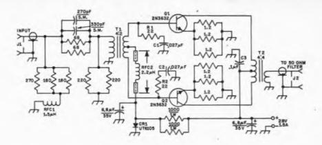
output transformer, and the series 1041 toroids are used for the input transformer.<sup>2</sup> In order to reduce flux leakage the center winding of the primary of the output transformer (and the secondary of the input transformer) should be made of braid similar to the shield-diameter of small coaxial cable. A broadband match to a low-impedance termination is readily achieved with these transformers.
