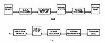
Fig. 4 — Test setups for checking varactor multipliers.
