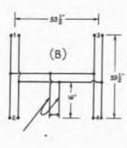
Fig. 22-19 — Large collinear arrays should be fed as sets of no more than 8 driven elements each, interconnected by phasing lines. This 48-element array for 432 MHz (A) is treated as if it were four 12-element collinears. Reflector elements are omitted for clarity. Phasing harness is shown at B.
