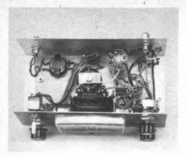
The layout of the phone-patch components is not critical. The two hybrid-network transformers are visible to the right of center, and in the upper left corner of the circuit board the receiver matching transformer may be seen. Two damping capacitors added during modification of the Calectro DI-930A meter are visible atop the meter case; two more are hidden beneath the meter.
