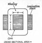
Fig. 5-6 — Cross-sectional drawing of a typical power transformer. Multiplying the height (or
