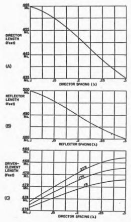
Fig. 21-38 — Element lengths for a 3-element beam. These lengths will hold closely for tubing elements supported at or near the center.
