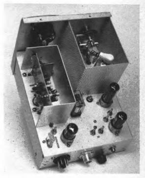
Fig. 7-4 - Top view of the transverter, receiving converter is inside the shield at the left. The 22-MHz crystal oscillator and buffer are in the left rear portion of the chassis. In the right corner is the transmitting mixer. Above it is the first amplifier. The 6146 output amplifier is in the shielded compartment at the left front.
