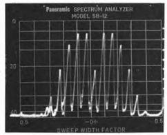
Fig. 14-4 — Output frequency spectrum of a narrow-band fm transmitter modulated by a 1-kHz
