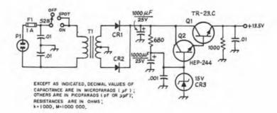
Fig. 4 — Power supply for the solid-state VFO. Capacitors with polarity marked are electrolytic, others are disk ceramic. Resistors are 1/2-watt composition.
