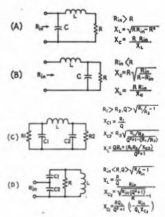
Fig. 2-52 — Impedance-matching networks adaptable to amateur work. (A) L network for matching to a lower value of resistance. (B) L network for matching to a higher resistance value, (C) pi network. (D) Versatile circuit often used in transistor- and antenna-matching networks.
