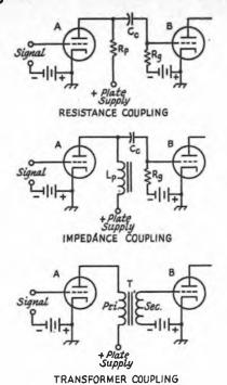
Fig. 3-10 — Three types of coupling are in common use at audio frequencies. These are resistance coupling, impedance coupling, and transformer coupling. In all three cases the output is shown coupled to the grid circuit of a subsequent amplifier tube, but the same types of circuits can be used to couple to other devices than tubes.
