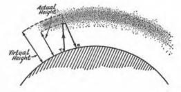
Fig. 19-3 — Bending in the ionosphere, and the echo or reflection method of determining virtual height.
