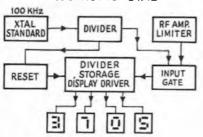
Fig. 6-13 - Block diagram of a frequency counter.
