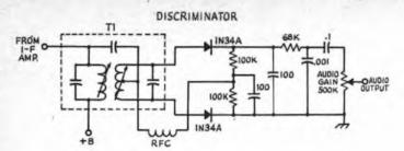
EXCEPT AS INDICATED, DECIMAL VALUES OF CAPACITANCE ARE IN MICROFARADS (μF); OTHERS ARE IN PICOFAROS (pF OR μμF); RESISTANCES ARE IN OHMS; k=1000, M=1000000
