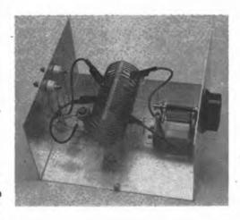
Construction of the coupler. Note method of mounting T1 (seen to the left of the coil L1).
