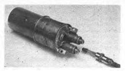
Fig. 10-6 — The automobile ignition coil should be shielded as shown here. A small tin can has been soldered to the metal coil case, and coaxial feed through capacitors have been soldered to the top of the can. The "hot" lead of the coil enters the shield can through a modified audio connector.
