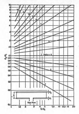
Fig. 20-11 — Impedance transformation ratio, two-conductor folded dipole. The dimensions d1, d2 and s are shown on the inset drawing. Curves show the ratio of the impedance (resistive) seen by the transmission line to the radiation resistance of the resonant antenna system.
