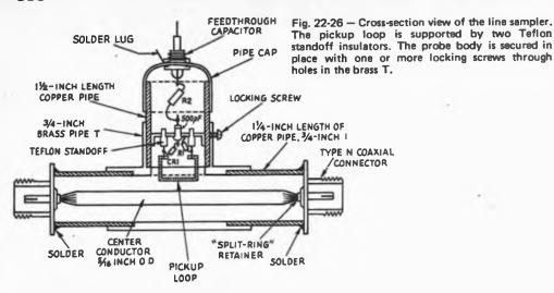
the edge for soldering inside the pipe. The diode, CR1, is connected between one end of the loop and a 500-pF feedthrough capacitor, C1, soldered into the disk. The terminating resistor, R1, is connected between the other end of the loop and ground, as directly as possible.
