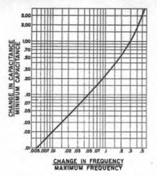
Fig. 8-11 — Minimum circuit capacitance required in the circuit of Fig. 8-10A as a function of the capacitance change and the frequency change. Note that *maximum* frequency and *minimum* capacitance are used.
