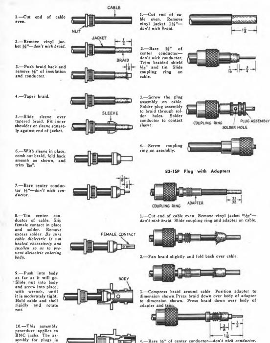
Fig. 18-9 — Cable-stripping dimensions and assembly instructions for several popular coaxial-cable plugs. This material courtesy Amphenol Connector Division, Amphenol-Borg Electronics Corp.
