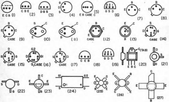
The leads are marked C - collector, B - base, E - emitter, G - gate, D - drain, and S - source.
