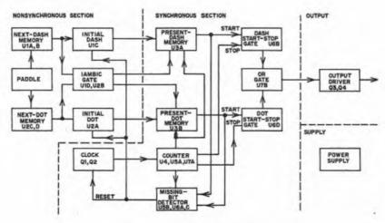
Fig. 1 - Block diagram of the Accu-Keyer.
