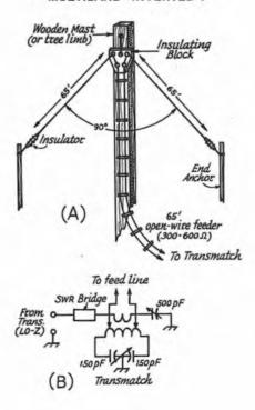
size one quarter wavelength vertical worked against ground. When fed as shown in Fig. 21-14 it serves as an excellent multiband antenna.
