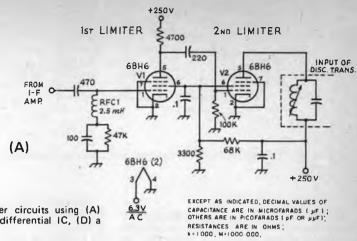
Fig. 14-14 -Typical limiter circuits using (A) tubes, (B) transistors, (C) a differential IC, (D) a high-gain linear IC.
