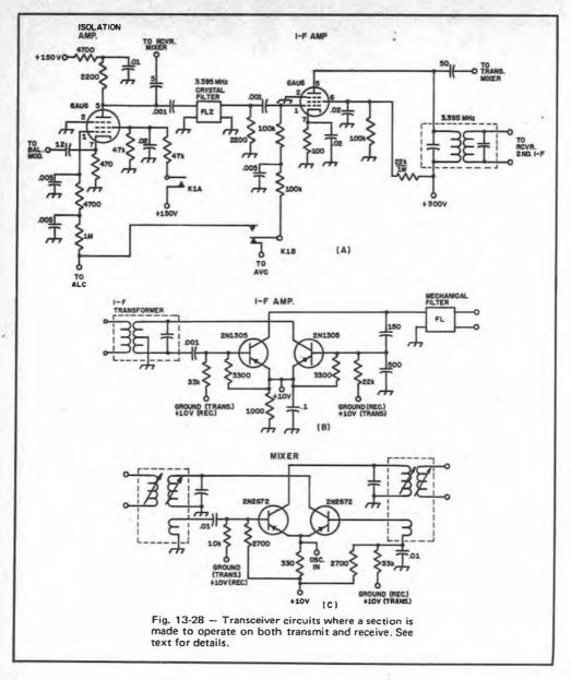
multiple-contact relay, which transfers the antenna if necessary and also shifts the biases on several stages. Most commercial designs offer VOX (voice-controlled operation) and MOX (manual operation). Which is preferable is a controversial subject; some operators like VOX and others prefer MOX.
