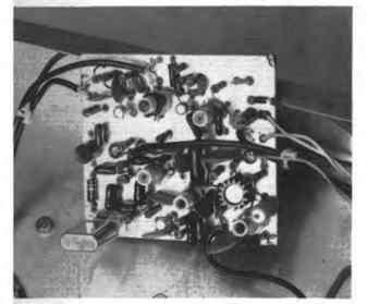
Close-up view of the printed-circuit board. This board has the local oscillator, receiver, and low-level driver stages. The crystal socket and crystal for the LO are shown at the lower left.
