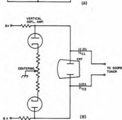
Fig. 13-32 — Modifications to a general-purpose oscilloscope to allow direct input to the vertical deflection plates. A, connection for a scope where centering is done in the B-plus lead and B, where centering is accomplished at the cathodes of the vertical amplifier tubes. The capacitors used for C1 and C2 should have a rating of 1000 volts or more. Connections can be brought out to the front or rear panel of the oscilloscope.
