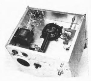
Fig. 7-29 — With the bottom cover removed, a look into the chassis from the rear shows the input circuit, L1,C1, right, the bifilar filament chokes, foreground, filament transformer and control switches. Opening in the rear wall is for air intake.
