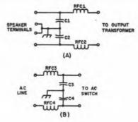
Fig. 16-3 — At A, the method for additional speaker filter, and at B, filtering the ac-line input. In both cases, these installations should be made directly inside the amplifier chassis, keeping the leads as short as possible.
