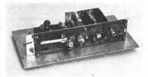
Fig. 3 — The oscillator-multiplier assembly is on a circuit board mounted on a full-length aluminum bracket that provides both support and shielding. The crystal oscillator is at the right end. The strip-line at the left end is L17, the tuned circuit of a 404-MHz filter in the output of the last doubler stage.
