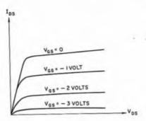
Fig. 4-21 A-Typical JFET characteristic curves.
