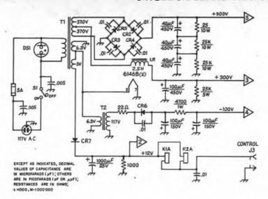
Fig. 2 — Diagram of the power-supply section. Resistors are 1/2-watt composition. Capacitors are disk ceramic, except those with polarity marked which are electrolytic.
