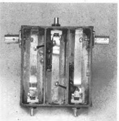
Fig. 14-46 -The 440-MHz preamplifier is constructed in a 3 X 3 1/2 X 1-inch box made of double-sided circuit board. All abutting edges are soldered to complete the enclosure. Two 3 X 15/16-inch shields separate the tuned lines.
