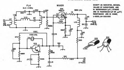
oscillator at 1850 kHz. Tune in this signal and peak the tuned circuits in FL1 for maximum response as heard in the speaker of the homemade receiver. Repeat the peaking process several times until the filter is optimized.
