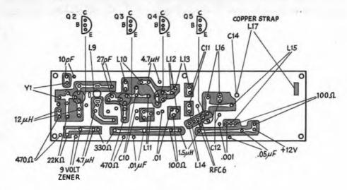
Fig. 9-7 — Half-scale drawing of the injection board, foil side.
