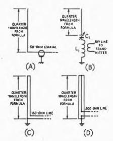
Fig. 21-24 — A quarter-wavelength antenna can be fed directly with 50-ohm coaxial line (A), with a low standing-wave ratio, or a coupling network can be used (B) that will permit a line of any impedance to be used. In (B), L1 and C1 should resonate to the operating frequency and L1 should be larger than is normally used in a plate tank circuit at the same frequency. By using multiwire antennas, the quarter-wave vertical can be fed with (C) 150- or (D) 300-ohm line.
