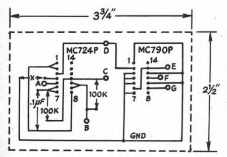
Fig. 17-32 -Wiring plan for the circuit board, component side. Dimensions for placement of parts are exact. jumper. Other letters indicate external connection points, corresponding to similarly lettered connections in Fig. 17-30.
