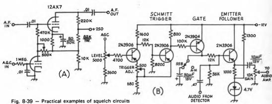
Fig. 8-39 — Practical examples of squelch circuits for cutting off the receiver output when no signal is present.
