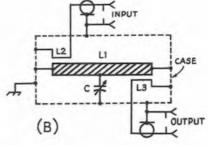
Fig. 16-25 — Equivalent circuits for the strip-line filters. At A, the circuit for the 6- and 2-meter filters are shown. L2 and L3 are the input and output links. These filters are bilaterial, permitting interchanging of the input and output terminals.
