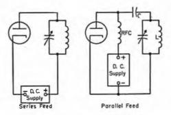
Fig. 2-57 - Illustrating series and parallel feed.
