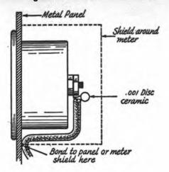
Fig. 16-15 — Meter shielding and bypessing. It is essential to shield the meter mounting hole since the meter will carry rf through it to be radiated. Suitable shields can be made from 2 1/2- or 3-inch diameter metal cans or small metal chassis boxes.
