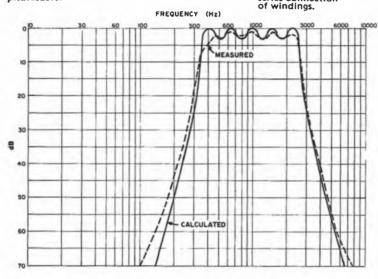
Fig. 2 — Calculated and measured curves for the phone filter.
