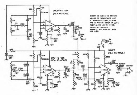
Fig. 17-34 — Circuit diagram of the integrated-circuit two-tone test generator (IC-TT). Resistors are 1/2-watt composition; capacitors with polarity marked are electrolytic, others are disk ceramic. All parts are supplied with the RCA kits, except those marked with an asterisk.
