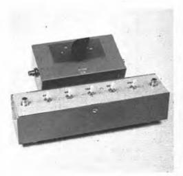
Fig. 8-32 — Two attenuators for receiver front-end protection.
