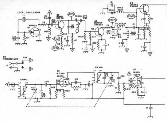
Fig. 1 — Schematic diagram for the transverter. Resistors are 1/2-watt composition and capacitors are disk ceramic, unless otherwise noted.
