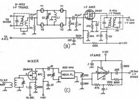
Fig. 8-25 — A half-lattice bandpass filter at A; B shows two half-lattice filters in cascade; C shows a mechanical filter.
