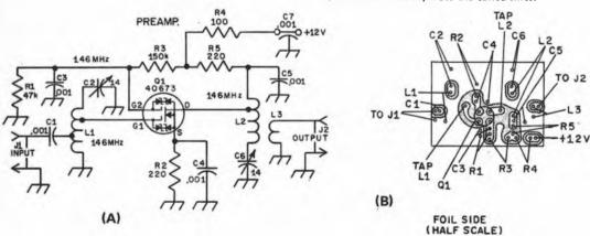
Fig. 14-45 -Circuit diagram (A) and pc-board layout (B) for the 2-meter preamplifier, Resistors are 1/4-watt composition and capacitors are disk ceramic unless otherwise noted. Components not listed below are given designators for circuit-board location purposes.
