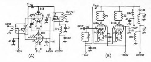
Fig. 6-20 - Typical (A) push-pull and (B) parallel amplifier circuits.
