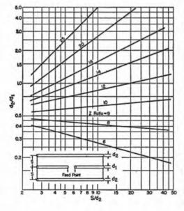
Fig. 20-12 — Impedance transformation ratio, three-conductor folded dipole. The dimensions d1, d2 and s are shown on the inset drawing. Curves show the ratio of the impedance (resistive) seen by the transmission line to the radiation resistance of the resonant antenna system.
