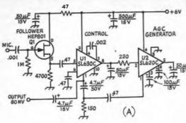
Fig. 13-18 — Typical solid-state compressor circuit.
