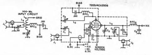
Fig. 7-48 — Schematic diagram of the 432-MHz amplifier, as set up for straight-through operation. An alternate 144-MHz input circuit for tripling is shown at the left.
