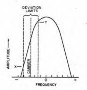
Fm detector characteristics. Slope detection, using the sloping side of the receivers selectivity curve to convert fm to a-m for subsequent detection.
