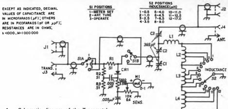
Fig. 1 — Schematic diagram of the Transmatch. Fixed-value capacitors are desk ceramic. Fixed-value resistors are composition types.
