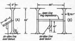
Fig. 22-11 — Stacking details for the 5-element Yagis of Fig. 22-7 and 22-10. The short on the universal stub, and the point of connection of the main transmission line, are adjusted for minimum reflected power in the latter. Balanced line could be connected similarly for the main turn.
