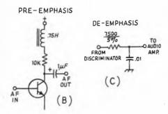
Fig. 14-6 - (A) The phase-shifter type of phase modulator. (B) Pre-emphasis and (C) de-emphasis circuits.
