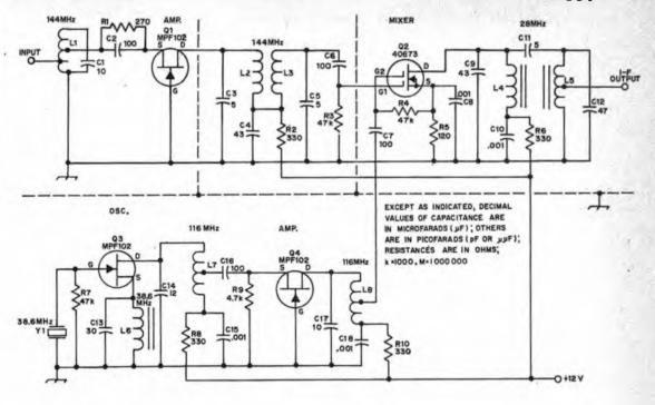
Fig. 3 — Schematic diagram of the two-meter converter. All resistors are 1/4-watt composition. C8, C10, C15 and C18 are .001-μF disk ceramic. All other capacitors are dipped mica units.
