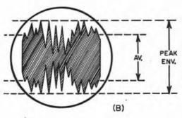
Fig. 13-17 — (A) Typical ssb voice-modulated signal might have an envelope of the general nature shown, where the rf amplitude (current or voltage) is plotted as a function of time, which increases to the right horizontally. (B) Envelope pattern after speech processing to increase the average level of power output.
