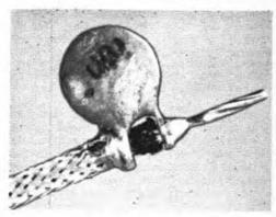
Fig. 16-11 — Proper method of bypassing the end of a shielded lead using disk ceramic capacitor. The .001- $\mu$ F size should be used for 1600 volts or less; 500 pF at higher voltages. The leads are wrapped around the inner and outer conductors and soldered, so that the lead length is negligible. This photograph is about four times actual size.
