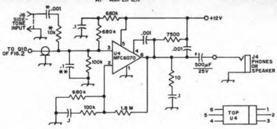
Fig. 3 — Schematic diagram of the MFJ Enterprises 1-watt audio module used in the receiver.
