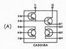
Fig. 4-27 — Transistor arrays offer unlimited application because several circuit combinations are possible. The CA3018A IC at A has a Darlington-connected pair plus two separate transistors. At B, two transistors are internally
