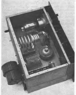
Laboratory tests at Eimac indicate best performance to be at an anode potential of 2700 to 3000 volts. The efficiency runs between 60 and 65 percent.
