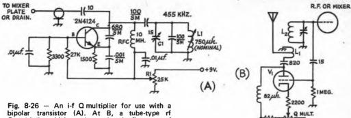
Fig. 8-26 — An i-f Q multiplier for use with a bipolar transistor (A). At B, a tube-type rf Q multiplier which can be used at the first stage of the receiver. The antenna coil is used for feedback to V1, which then introduces "negative resistance" to L2.
