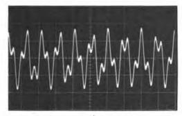
Fig. 17-36 — Proper output waveforms from the generator: (Upper) sine wave, indicating correct adjustment of the FEEDBACK control; (Lower) two-tone output.
