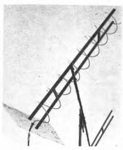
Fig. 22-20 — An 8-turn 432-MHz helical array, wound from aluminum clothesline wire. Left-hand polarization is shown. Each turn is one wavelength, with a pitch of 0.25 wavelength. Feed is with 50-ohm coax, through an 84-ohm Q section.
