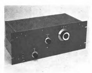
Fig. 7-31 — The 144-MHz amplifier is built in conventional rack-and-panel style, with the entire top of cane metal, to provide free air flow. Controls are grid-circuit tuning, C2, lower left; output loading capacitor, C5, center; and plate-circuit tuning, C4, with vernier dial, right. The slotted end of the Teflon shaft on C1 is visible as a white spot just below the loading control.
