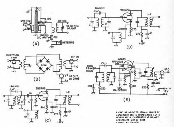
Fig. 9-8 — Vhf and uhf mixer circuits. A diode mixer for 1296 MHz, with a coaxial circuit for the signal frequency, is shown in A. CR1 is a uhf diode, such as the 1N21 series. A balanced mixer, as in B, gives improved rejection of the signal and injection frequencies. If hot-carrier diodes are used for CR2, sorting for matched characteristics is eliminated. Gate and source injection of a JFET mixer are shown at C and D, respectively.
