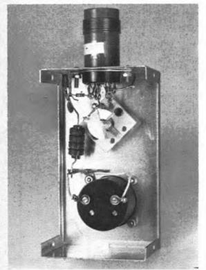
Fig. 17-44 — Inside the absorption frequency meter, showing placement of tuning capacitor and coil socket.
