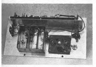
matter if the builder has a 50-MHz receiver. A tuned-line filter, loosely-coupled to the last doubler, helps to suppress unwanted products of the multiplier system.
