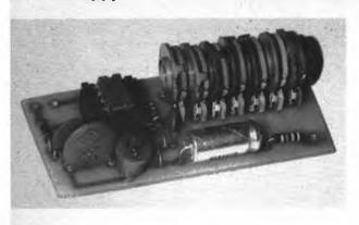
Top view of the circuit board built by Glenn Dickson, WB5BAF. The unit was originally described in April, OST, 1974.
