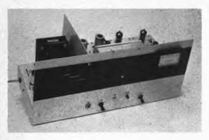
Fig. 7-7 — Panel view of the 2-meter transverter. This version is patterned after a transmitting converter design by K9UIF. The on-off switches for ac and dc sections of the power supply are mounted on the front panel of the unit as are the pilot lamps and plate meter for the PA stage. The tuning controls for the various stages are accessible from the top of the chassis.
