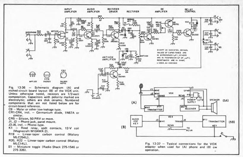
from a 600-ohm speaker lead, or if the receiver has a high-impedance audio output, the Q4 amplifier stage may not be necessary.
