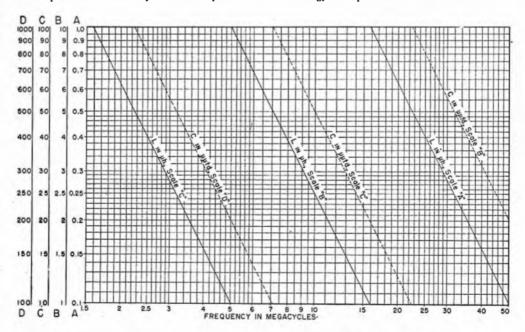
Fig. 17-20 — Chart for determining unknown values of L and C in the range of 0.1 to 100  $\mu$ H and 2 to 1000 pF, using standards of 100 pF and 5  $\mu$ H.
