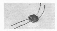
Fig. 4 — Close-up view of the input transformer used in the circuit of Fig. 1.
