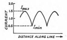
Fig. 20-5 — Measurement of standing-wave ratio. In this drawing,  $I_{\rm max}$  is 1.5 and  $I_{\rm min}$  is 0.5, so the SWR =  $I_{\rm max}/I_{\rm min}$  = 1.5/0.5 = 3 to 1.
