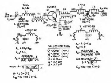
Example: An amplifier stage must deliver 10 watts to a known resistive load. The dc voltage from collector to emitter is 13.6.  $R_L$  is
