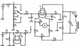
Fig. 17-8 — Vacuum-tube voltmeter circuit.
