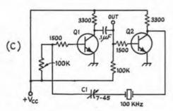
Fig. 17-18 — Three simple 100-kHz oscillator circuits. C is the most suitable of available transistor circuits (for marker generators) and is recommended where solid-state is to be used. In all three circuits C1 is for fine frequency adjustment. The output coupling capacitor, C3, is generally small — 20 to 50 pF — a compromise to avoid loading the oscillator by the receiver antenna input while maintaining adequate coupling for good harmonic strength.
