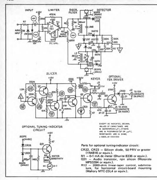
via J3. Typing at the keyboard will then produce local copy on the printer, and will also produce voltages at J1 and J2 for frequency-shift keying a transmitter or an audio oscillator.
