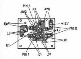
Fig. 9-8  $-\,$   $\,$  Half-scale drawing of the i-f amplifier board, foil side.
