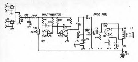
Fig. 11-11 — Circuit diagram of the cw monitor. Unless specified, all resistors are 1/2 watt; resistances are in ohms (K = 1000). All values of capacitors are in microfarads ( $\mu$ F, all .01- $\mu$ F capacitors are disk ceramic). Capacitors marked with polarity are electrolytic.
