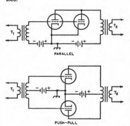
Fig. 3-12 — Parallel and push-pull af amplifier circuits.
