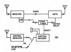
Fig. 14-28 — Simple repeaters. The system at A is for local control. Remote control is shown at B.
