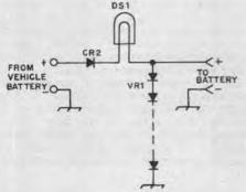
Fig. 2 — Schematic diagram of NiCad battery charger suitable for mobile use. See text for explanation of DS1 and VR1. CR2 protects the components in the event of accidental reversal of input leads. See Fig. 1 for CR2.
