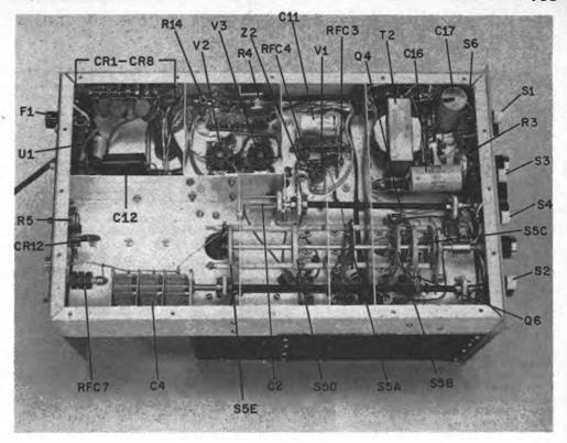
Fig. 5 — Chassis bottom view. The opening next to SSE is needed to make connections to L20 and L21.
