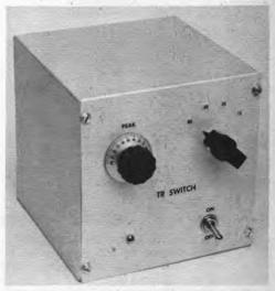
Fig. 1 — The knob at the left is used for peaking the tuned circuit. At the right is the bandswitch. Only four positions are shown; the 15-meter position also covers 10 meters.
