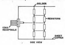
Fig. 17-25 — Using resistors in series-parallel to increase the power rating of a small dummy antenna. Mounted in this way on pieces of flat copper, inductance is reduced to a minimum. Eight 100-ohm 2-watt composition resistors in two groups, each four resistors in parallel, can be connected in series to form a 50-ohm dummy. The open construction shown permits free air circulation. Resistors drawn heavy are in one "deck"; light ones are in the other.
