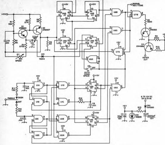
Fig. 2 - Schematic diagram of the Accu-Keyer. Resistances are in ohms; k = 1000. All capacitances are in microfarads. All resistors may be 1/4 watt except R13, which should have a 2-W rating. Capacitors with polarity indicated are electrolytic; all others are disk ceramic. Parts not listed below are for text reference and circuit-board identification.
