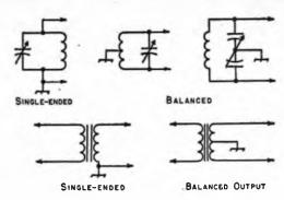
Fig. 2-59 - Single-ended and balanced circuits.
