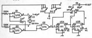
Fig. 17-30 — Marker generator circuit, Pin 4 of both ICs is grounded. Connect pin 11 of U1 to point C, and pin 11 of U2 to point F.
