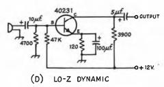
Fig. 13-10 — Speech circuits for use with standard-type microphones. Typical parts values are given.
