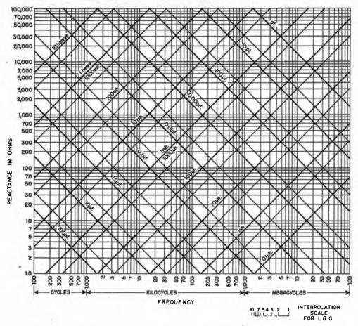
Fig. 2-28 — Inductive and capacitive reactance vs. frequency. Heavy lines represent multiples of 10, intermediate light lines multiples of 5; e.g., the light line between 10  $\mu$ H and 100  $\mu$ H represents 50  $\mu$ H, the light line between 0.1  $\mu$ F and 1  $\mu$ F represents 0.5  $\mu$ F, etc. Intermediate values can be estimated with the help of the interpolation scale.
