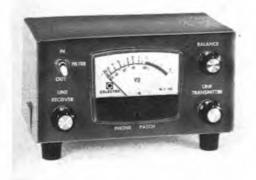
The phone patch unit is built into a homemade aluminum enclosure measuring 3 X 3 X 6 inches. A coating of spray-on enamel, rubber feet, and wet-transfer decal labels plus shiny knobs give the unit a professional appearance. This unit was constructed by W1NPG.
