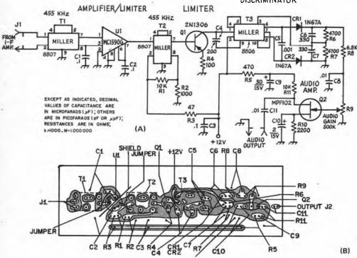
(A) Diagram of the 455-kHz narrow-band adapter. Resistors are 1/4- or 1/2-watt composition and capacitors are disk ceramic, except those with polarity marked, which are electrolytic. Components with reference numbers that are not listed below are noted for circuit-board location.
