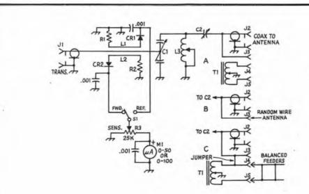
Fig. 20-22 - Circuit diagram of the Transmatch. The .001-µF capacitors used are disk ceramic.
