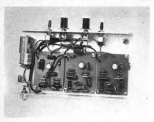
Fig. 17-35 — Interior view of the IC-TT. Interconnections carrying audio signals use subminiature coax to prevent hum pickup. A homemade clip holds the battery in place. Feedback adjustment of each oscillator is made with the controls on the KC-4002 boards.
