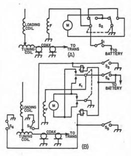
Fig. 10-17 — Circuit of the remote mobile-whip tuning systems.
