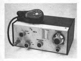
This ssb transceiver is suitable for QRP operation from batteries or as a main frame for fixed-station use. Its circuitry is simple enough to permit easy duplication (or substitution of components where necessary) by proficient builders with only limited experience in solid-state design.
