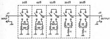
Fig. 8-34 — Circuit diagram of the step attenuator. All reOUTPUT sistors are 1/4-watt composition, 5percent tolerance.
