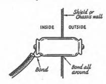
Fig. 16-14 — The best method of using the "Hypass" type feed-through capacitor. Capacitances of ,01 to 0,1  $\mu$ F are satisfactory, Capacitors of this type are useful for high-current circuits, such as filament and 117-volt leads, as a substitute for the rf choke shown in Fig. 16-12, in cases where additional lead filtering is needed.
