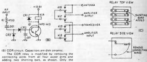
stationary-contact connections are used.
