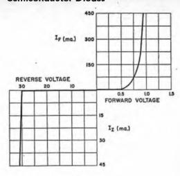
Fig. 4-4 — Typical characteristic of a Zener diode. In this example, the voltage drop is substantially constant at 30 volts in the (normally) reverse direction. Compare with Fig. 4-3. A diode with this characteristic would be called a "30-volt Zener diode."
