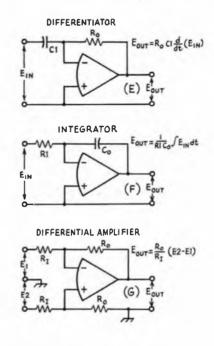
Fig. 4-33 - Basic op-amp circuits.
