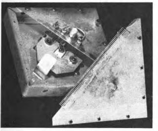
spring bronze to make a snug fit in the heater cup at the end of the tube. The air-wound rf choke is connected directly to this, with the other end running to the feedthrough bypasses. The heaters being brought out separately permits a check on condition of tubes, by turning off the heaters one at a time. Leaving the tube in place, but cold, does not detune the system, and a comparison of the tubes may be made in this way. Note that neither side of the heater circuit can be grounded.
