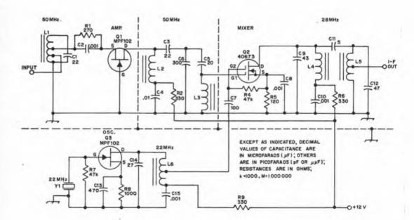
Fig. 2 — Schematic diagram of the six-meter converter. All resistors are 1/4-watt composition. C2, C8, C10 and C15 are .001 $\mu$ F disk ceramic. C4 is .01- $\mu$ F disk ceramic, All other capacitors are dipped mica.
