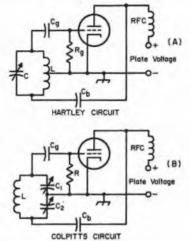
Fig. 3-21 — Basic oscillator circuits. Feedback voltage is obtained by tapping the grid and cathode across a portion of the tuned circuit. In the Hartley circuit the tap is on the coil, but in the Colpitts circuit the voltage is obtained from the drop across a capacitor.
