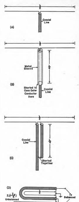
Fig. 20-14 — Radiator with coaxial feed (A) and methods of preventing unbalanced currents from flowing on the outside of the transmission line (B and C). The half-wave phasing section shown at D is used for coupling between an unbalanced and a balanced circuit when a 4-to-1 impedance ratio is desired or can be accepted.
