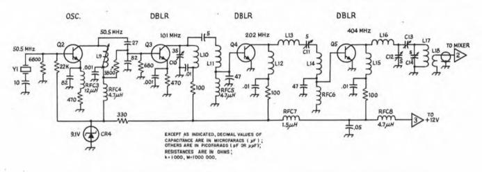
Fig. 5 — Schematic diagram and parts information for the oscillator-multiplier stages of the 432-MHz converter.
