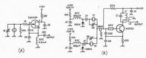
Fig. 6-5 — Two practical crystal-oscillator designs. (A) For low-power output applications such as a conversion oscillator or BFO, (B) an example of diode switching of crystals. The rf choke on the base lead of the transistor is a ferrite bead which prevents which prevents with parasitic oscillation.
