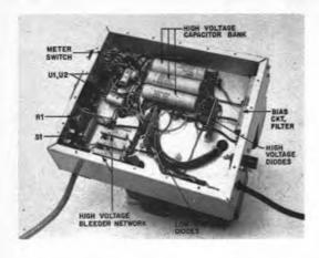
Fig. 3 — Bottom view of the Universal Power Supply.
