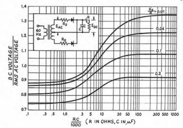
Fig. 5-5 — Dc output voltages from a full-wave rectifier circuit as a function of the filter capacitance and load resistance. R<sub>s</sub> includes transformer winding resistance and rectifier forward resistance. For the ratio R<sub>s</sub>/R, both resistances are in ohms; for the RC product, R is in ohms and C is in  $\mu$ F.
