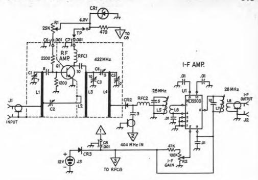
Fig. 4 — Schematic diagram and parts information for the rf and i-f portions of the 432-MHz converter.
