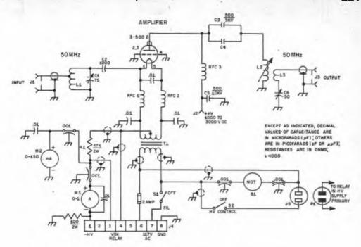
Fig. 7-30 -Schematic diagram and parts information for the 50-MHz grounded-grid ampli-
