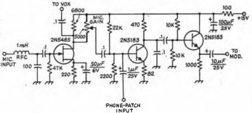
Fig. 13-12 — Typical phase-inverter circuits for transistor amplifier applications.
