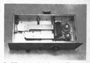
Fig. 7-32 — Interior of the 2-meter amplifier, showing the brass plate-inductor and vane-tuning system. Note the position of RFC1, at the far left, out of the main rf field. The output coupling loop, L4, just below the plate line and barely visible here, is connected to the output jack, J4, on the rear wall with a short section of coax, and to the loading capacitor, C5, on the front panel by means of copper strip.
