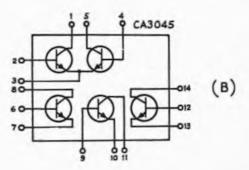
connected in a differential amplifier fashion. Three separate transistors are available for use in other functions. The arrays shown here are useful into the vhf spectrum.
