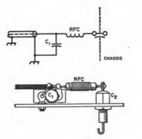
Fig. 16-13 — Additional lead filtering for harmonics or other spurious frequencies in the high vhf TV band (174-216 MHz).
