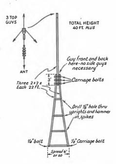
Fig. 21-55 — Details of a simple 40-foot "A"-frame mast suitable for erection in locations where space is limited.
