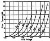
Fig. 3-6 — Grid-voltage-vs.-plate-current curves at various fixed values of plate voltage  $(E_{\rm b})$  for a typical small triode. Characteristic curves of this type can be taken by varying the battery voltages in the circuit at the right.
