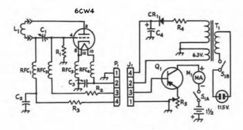
Fig. 17-40 - Circuit diagram of the uhf dip meter.
