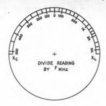
set at 500 in the  $X_{\rm L}$  range, the 0 dial indication is now equivalent to an  $X_{\rm C}$  reading of 500, and the total range of measurement for  $X_{\rm C}$  has been extended to 1000.
