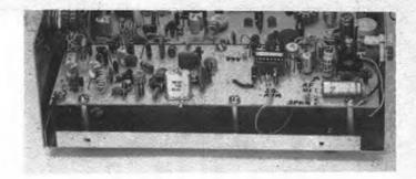
respective tuned circuits. For simplicity s sake only two tuned circuits are used ahead of the mixer, which uses a dual-gate MOSFET. The combination of FETs Q1 and Q2 assures low IMD and provides good immunity to overloading. Output from the mixer is supplied to FL1. This is a four-pole 10.7-MHz i-f filter which is fed from a 900-ohm tap point on tuned circuit C9-C10-L3.
