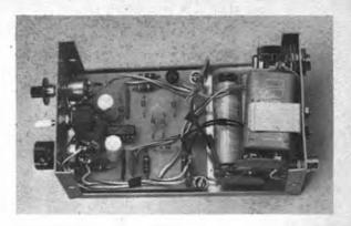
with a single-pole switch is not satisfactory, as current will still flow from the batteries. In the keyer shown in the photographs, S1 is located on the rear of the weight control. When the keyer is energized, the response is almost instantaneous, as there is nothing which must warm up before operation can commence.
