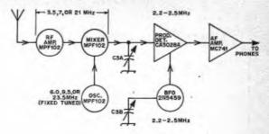
Fig. 5 — Block diagram of the receiver. The arrows indicate the direction of signal travel.
