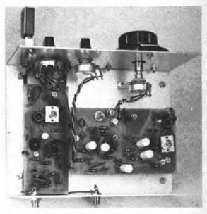
Top view of the W7ZOI and K7TAU 40-meter transceiver built by WA1JLD.
