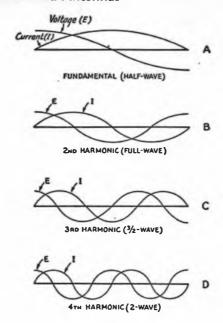
Fig. 21-15 — Standing-wave current and voltage distribution along an antenna when it is operated at various harmonics of its fundamental resonant frequency.
