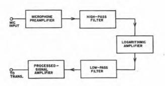
Fig. 1 — Block diagram for the logarithmic processor.
