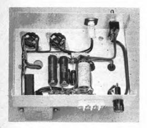
Fig. 10-31 — A look at the underside of the chassis. The resistors and capacitors are mounted between insulated terminal strips. Ac zip cord, paralleled, is used for the heavy-duty primary wiring.
