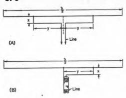
Fig. 20-13 - The "T" match and "gamma" match.
