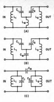
Fig. 2-46 - Three methods of circuit coupling.
