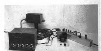
transmitted on the same channel, first by frequency modulating a 4.5-MHz oscillator. The 420-MHz transmitter is modulated simultaneously with this signal and the video, by means of the video-sound modulator.
