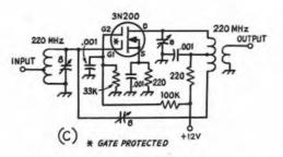
Fig. 9-1 — Typical grounded-source rf amplifiers. The dual-gate MOSFET,A, is useful below 500 MHz. The junction FET,B, and neutralized MOSFET,C, work well on all vhf bands. Except where given, component values depend on frequency.
