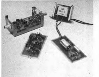
Fig. 1 — Completed six- and two-meter converters (left and center) with power supply.
