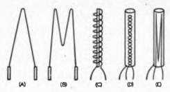
Fig. 3-2 — Types of cathode construction. Directly heated cathodes or "filaments" are shown at A, B, and C. The inverted V filament is used in small receiving tubes, the M in both receiving and transmitting tubes. The spiral filament is a transmitting tube type. The indirectly heated cathodes at D and E show two types of heater construction, one a twisted loop and the other bunched heater wires. Both types tend to cancel the magnetic fields set up by the current through the heater.
