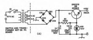
Fig. 7 — Schematic diagram and parts-placement guide for the power supply to the converters. The transformer is mounted external to the board. Pc board size is identical to the one used for the converters.
