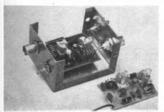
Two versions of the preamplifier. The one in the box is for 2-meter use. Toroids are used in the six-meter version (right) and in the ten-meter preamplifier (not shown). Input is at the right on both units. The extra rf choke and feedthrough capacitor on the right end of the Minibox are for decoupling a crystal-current metering circuit that is part of a 2304-MHz mixer.
