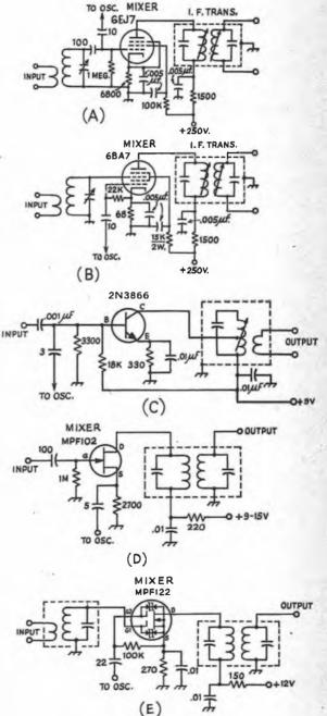
Fig. 8-15 — Typical single-ended mixer circuits.
