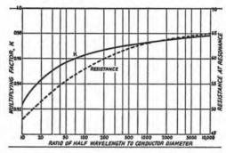
Fig. 21-3 — Effect of antenna diameter on length for half-wave resonance, shown as a multiplying factor, K, to be applied to the free-space half wavelength (Equation 21-A). The effect of conductor diameter on the center impedance also is shown.
