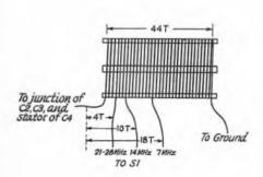
Fig. 3 — L1 and associated taps. L1 is 44 turns of No. 24, 32 turns per inch, 1 inch diameter (Miniductor 3016, Air Dux 832T). To solder the tap leads, indent each turn adjacent to the tap point. This will allow soldering room.
