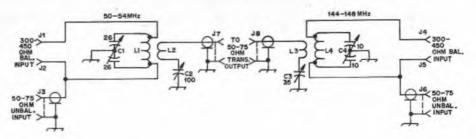
Fig. 22-22 - The schematic diagram of the vhf Transmatches. Capacitance is in pF unless otherwise noted. Resistance is in ohms, k = 1000.
