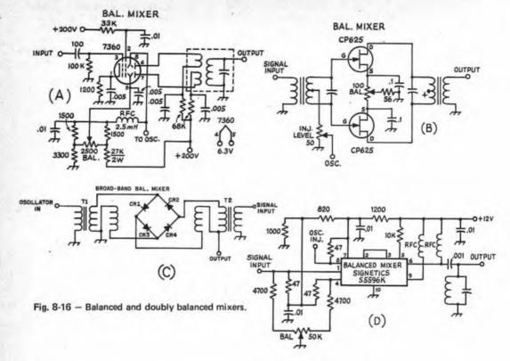
This type of mixer has excellent immunity to cross-modulation and overload. It offers better isolation between the oscillator and input stages than is possible with a JFET mixer. The mixers at D and E have high-Z input terminals, while the circuit at C has a relatively low-Z input impedance. The latter requires tapping the base down on the input tuned circuit for a suitable impedance match.
