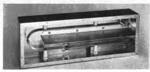
Fig. 16-27 — Interior of the 50-MHz strip line filter. Inner conductor of aluminum strip is bent into U shape, to fit inside a standard 17-inch chassis.
