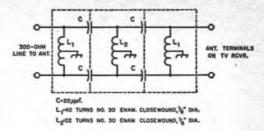
Fig. 16-32 — Another type of high-pass filter for 300-ohm line. The coils may be wound on 1/8-inch diameter plastic knitting needles. *Important*: Do not use a direct ground on the chassis of a transformerless receiver, Ground through a .001-µF mica capacitor.
