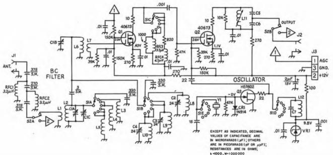
Fig. 8-49 — Schematic diagram of the hf converter. Capacitors are disk ceramic and resistors are 1/2-watt composition, unless otherwise noted. Capacitors with polarity marked are electrolytic. A template is available from the ARRL Technical Department for fifty cents and a large self-addressed stamped envelope.
