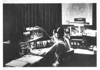
This modern amateur radio station is equipped for use in the hf bands. The gear is neatly arranged to provide the operator (K1ZND) with easy access to the various units. The foundation is made from plywood fashioned in the form of a console. The station belongs to K1THQ.
