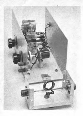
Fig. 13-35 — Interior view of the tuning unit and its pickup box. The variable capacitor is used to adjust the vertical deflection on the scope. The tuning unit should be mounted near the scope so that short interconnecting leads may be used. The pickup box consists of a No. 16 conductor forming a single-turn loop. Next to this loop is placed a two-turn second loop of plastic-covered hookup wire.
