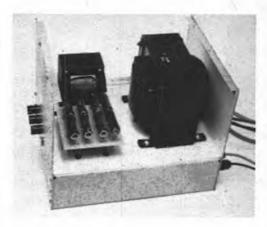
Fig. 1 — Top chassis view of the 3000-volt power supply as constructed by WA1JZC. The circuit board in the foreground holds the bleeder resistors, which are spaced apart and supported a short distance above the board for proper cooling. The large transformer is for the high-voltage supply, and the small transformer provides filament power for the amplifier.
