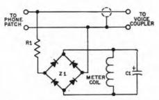
Fig. 2 — Schematic diagram of the modified Calectro DI-930 VU meter and its connections to a phone-patch circuit. Component values are different for early production models. See text for information on identifying a particular meter.
