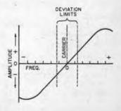
Fig. 14-15 — The characteristic of an fm discriminator.
