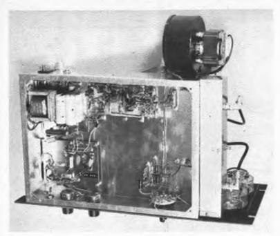
Fig. 7-20 - Looking underneath chassis the 220-MHz transmitter, we see the speech amplifierclipper at the lower left, the exciter circuits across the top. power supply components at the upper left, and meter s witching, lower right.
