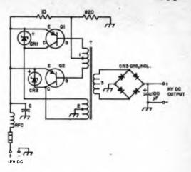
Fig. 10-26 — Typical dc-to-dc converter. Ratings for CR3-CR6, and the 100- $\mu$ F filter capacitor can be selected from data in the power-supply chapter.
