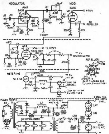
Fig. 3-25 — Schematic diagram and parts information for a power supply and control unit suitable for amateur microwave transceivers. Unless otherwise specified, capacitor values are in  $\mu F$  and resistors are 1/2-watt composition.
