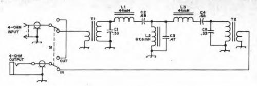
Fig. 3 — Circuit diagram for the ssb CRUD-O-Ject. The capacitors should be of good quality, as mentioned in the text. A complete set of inductors, trimmed and checked, along with two transformers (T1 and T2) are available from New England Engineering.<sup>2</sup>
