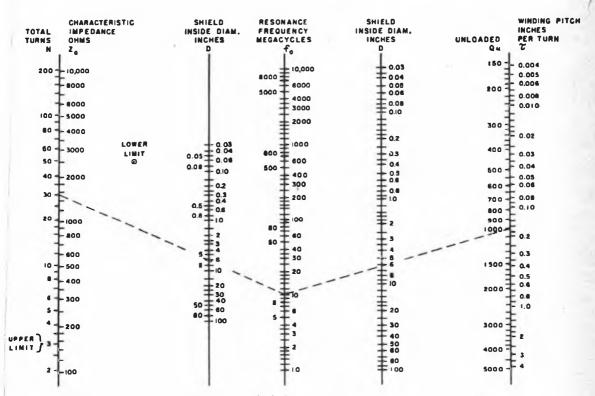
Fig. 9-5 - Design chart for quarter-wave helical resonators.
