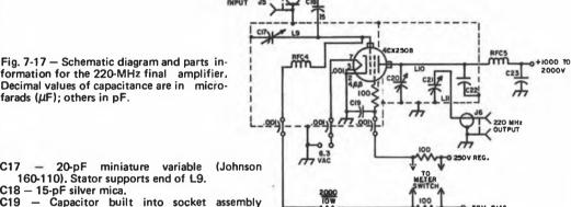
Fig. 7-17 - Schematic diagram and parts information for the 220-MHz final amplifier. Decimal values of capacitance are in microfarads (µF); others in pF.
