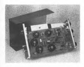
Inside view of the audio processor. A circuit board is used to mount most of the components.
