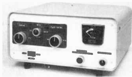
Fig. 75 — Front view of the modified SB-200 linear amplifier. A small false panel covers the original panel holes and adds a contrasting green color to the white front panel. Green Dymo tape labels identify the control functions.
