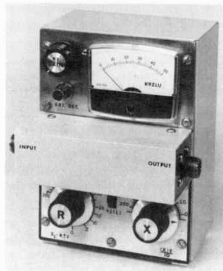
Fig. 73 — The OIB is enclosed in a 7 x 5 x 3-in. (178 x 127 x 76-mm) aluminum chassis. Tinnerman Speed Nuts and machine screws are used to secure the front panel to the chassis flange. Rectangular holes with cover plates in the rear panel permit alignment of the unit while it is fastened to the chassis.
