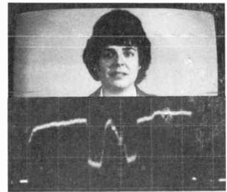
Fig. 39 — A single line of the TV picture at A has its voltage waveform shown at B. (Facilities courtesy of ESPN)
