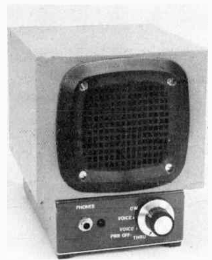
Fig. 84 — Deluxe audio filter with self-contained loudspeaker, built in the ARRL lab by Greg Bonaguide, WA1VUG. The 4-inch speaker is mounted in an enclosure having outside dimensions of 5-1/2 x 6-1/2 x 6-3/4 inches (H x W x D). The chassis measures 2 x 5 x 7 inches.
