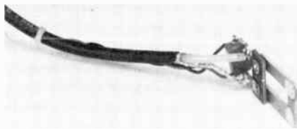
Fig. 41 — The Slipper Dipper, designed and built by Phil Accardi, AJ1N, uses printed circuit-board material as a foundation for its construction, but no etching is required. Q1, the active element, may be seen on edge at the top of the parallel line in this view, with base and collector leads soldered directly to the line conductors. Hookup wire, twisted into pairs, provides for connection to the power source and the external monitor meter, a 50- \mu A dc instrument.
