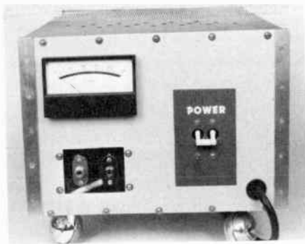
Fig. 51 — Front view of the heavy-duty, 3400-volt power supply.
