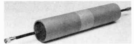
Fig. 5 — This coax shield decoupler is made with steel wool stuffed into an IBM copier tube. This size was selected for photographic purposes, but to be truly effective, the device should be about twice as long.
