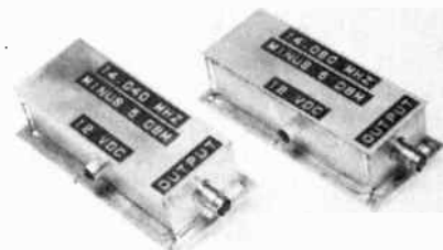
Fig. 81 — Exterior view of the signal generators suitable for use in receiver performance measurements. Each uses an OE-10 oscillator available from International Crystal Mfg. Co., Inc.
