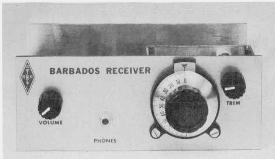
Fig. 55 — A low-cost cw receiver designed by Doug DeMaw, W1FB. The name on the front panel was inspired by the unit's intended purpose — vacation operating.
