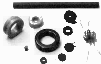
Fig. 50 — An assortment of toroid cores. A ferrite rod is placed at the top of the picture for comparison. The two light-colored, plastic encased toroids at the upper left are tapewound types (Hypersil steel) are suitable for audio and dc-to-dc converter transformers. The wound toroid at the right center contains two toroid cores which have been stacked atop one another to increase the power capability.
