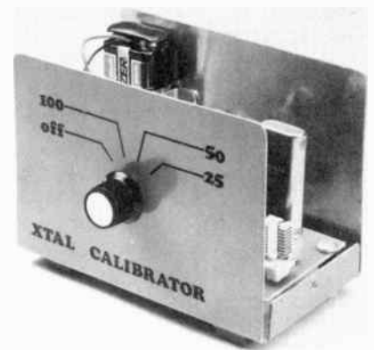
Fig. 25 — The 100, 50 and 25 kHz marker generator is housed in a 4-1/2 x 3 x 2-1/2 inch (114 x 76 x 64 mm) aluminum cabinet. A 9-volt battery makes the instrument completely self-contained.
