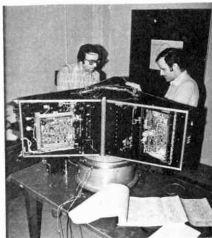
This is one of the Phase III high-orbit AMSAT-OSCAR satellites in the final stages of assembly. Launched in June 1983, this sophisticated yet relatively low-budget spacecraft provides predictable, reliable worldwide amateur communications.
