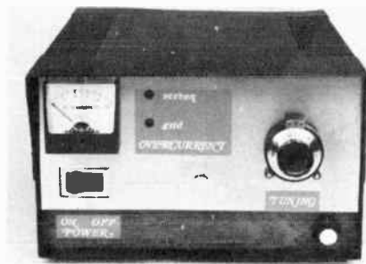
Fig. 21 — A 500-watt amplifier for the 2-meter band, complete with power supply, is housed in this cabinet. The hole plug covers a former location of a control.
