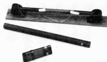
Fig. 52 — A bc-band ferrite rod loop antenna is at the top of the picture (J.W. Miller Co.). A blank ferrite rod is seen at the center and a flat bc-band ferrite loop antenna is in the lower foreground.
