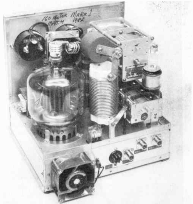
Fig. 58 — Rear view of the 160-meter amplifier with the cover removed. The chassis dimensions are 10 x 12 x 13 inches. Seen here are the plate-circuit components. K1 is the small relay at the rear of the chassis. The large cylindrical object above the tank inductor is the plate-blocking capacitor. Between the tuning and loading capacitors is a 220-pF vacuum capacitor to supplement the variable unit. The loading capacitor is a 5-gang assembly. Behind the tube from left to right are T1, T2 and RFC2. Directly behind the anode cap and parasitic choke is the upper fan.
