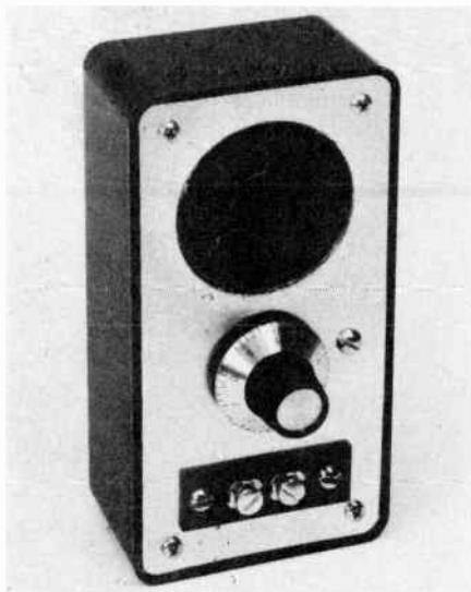
A code practice oscillator that can be constructed from commonly available parts.
