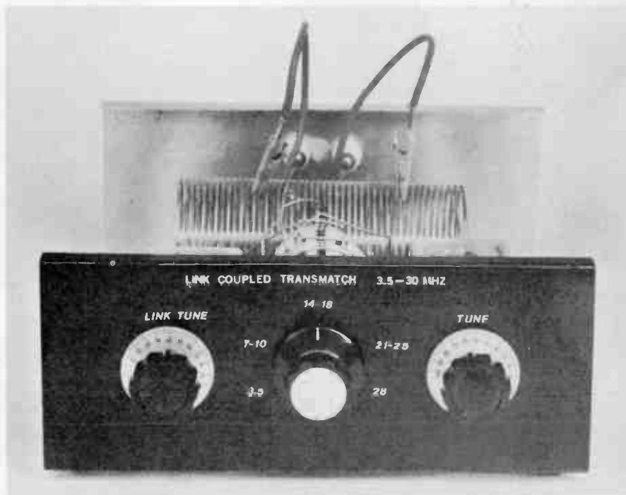
Fig. 26 — Exterior view of the band-switched link coupler. Alligator clips are used to select the proper tap positions of the coil.
