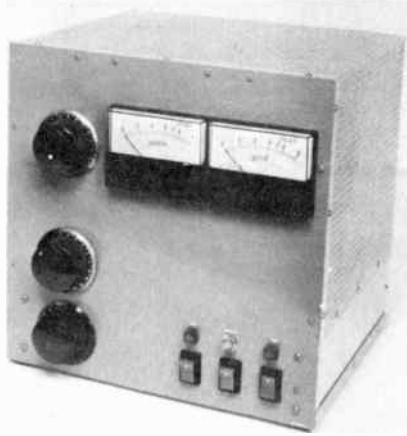
Fig. 54 — A full-power linear amplifier for 160 meters. From top to bottom, the controls are PLATE TUNING, ANTENNA LOADING and INPUT MATCHING. Front panel height is 12 in.
