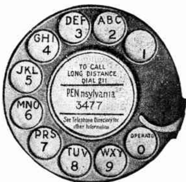
FIG. 7,637.—Multi-central station dial showing central station letters, and numerals.
