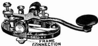
FIG. 7,692.—Fry open circuit key. It has a circuit closer which must be worked like an ordinary key. With circuit closer in closed position, the battery cannot be put to line or short circuited by pressing down on key lever, hence leaving a book or other heavy object on key does not waste the battery, but the relay is always in circuit ready to receive signals.
