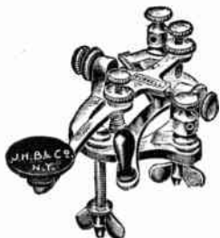
FIG. 7,692.—Fry open circuit key. It has a circuit closer which must be worked like an ordinary key. With circuit closer in closed position, the battery cannot be put to line or short circuited by pressing down on key lever, hence leaving a book or other heavy object on key does not waste the battery, but the relay is always in circuit ready to receive signals.
