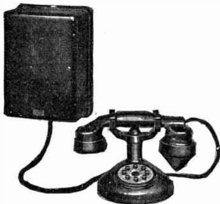
FIG. 7,598.—Graybar selective ringing common talking cradle type inter-phone system. It consists of a hand set with a cradle type mounting having push buttons mounted in the base. The hand set is black moulded bakelite. The interphone set includes an apparatus box containing a bell and a connecting block.
