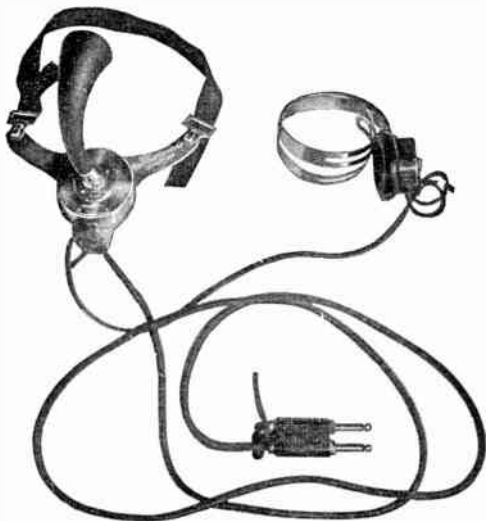
FIG. 7,572.—Operator's equipment showing receiver, transmitter, cut in plug, etc. The chest plate transmitter equipment is shown with cords connecting it to a cut in plug and a head receiver. The horn shaped mouthpiece is made of hard rubber and can be removed. The chest transmitter is held in place by a cloth neck band, the receiver by a head receiver band and the plug is inserted in spring jacks which are connected with the operator's set.
