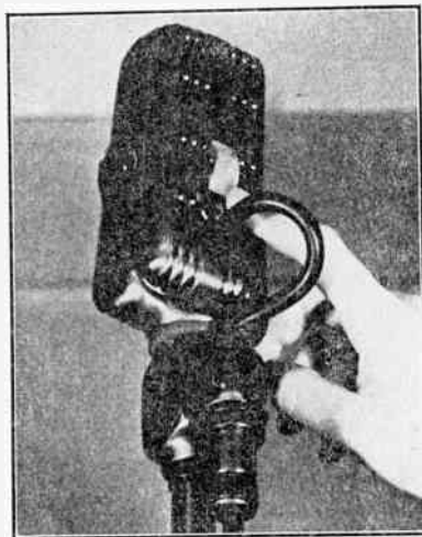
FIG. 26—Illustrating adjustable response type microphone. To increase pitch, push button upward; to lower pitch push button down. This adjustment according to the manufacturer will automatically take place without introducing any peaks or undesirable effects. (Courtesy The Amperite Co.)
