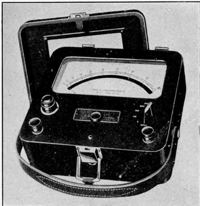
FIG. 17a—Weston Model 622 Thermo A.C.-D.C. Milliammeter.
