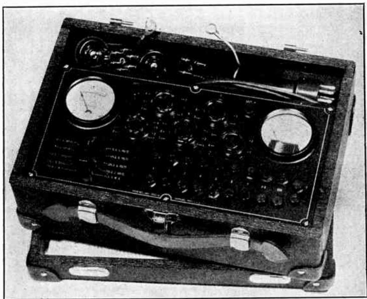
FIG. 32—Panel view of Readrite Model 720-A point to point panel.
