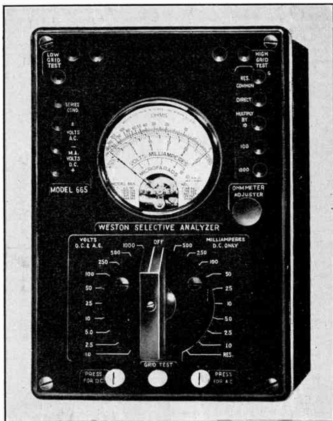
FIG. 13—Typical volt-milliamp-ohmmeter. (Courtesy Weston Electrical Instrument Corp.)
