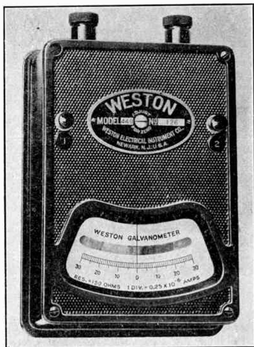
FIG. 4a—Weston model 440 movable coil galvanometer.
