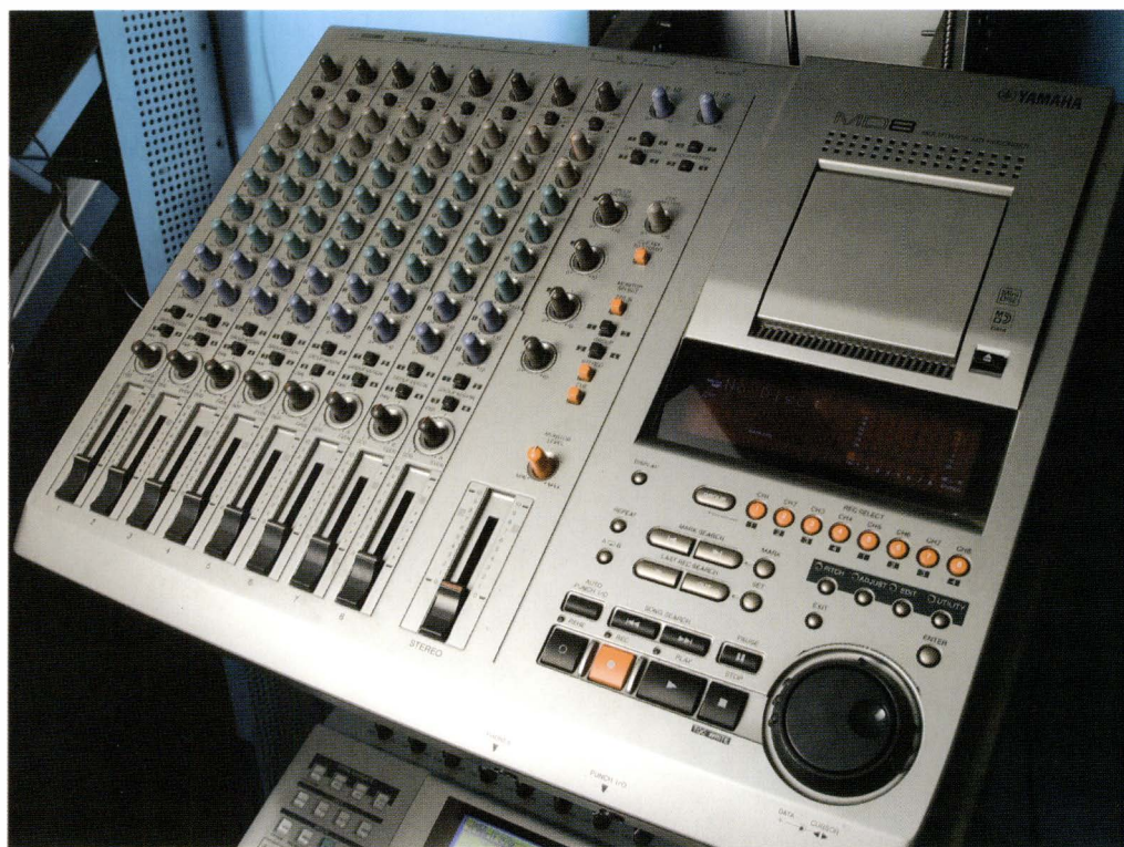
Above: Hot on the trail of some very popular four-track Minidisc (MD) recorders comes the Yamaha MD8, an eight-track version. Merging the convenience of random access with portability makes this a good choice if you want to use MDs. However, data minidiscs can be expensive and unreliable.
