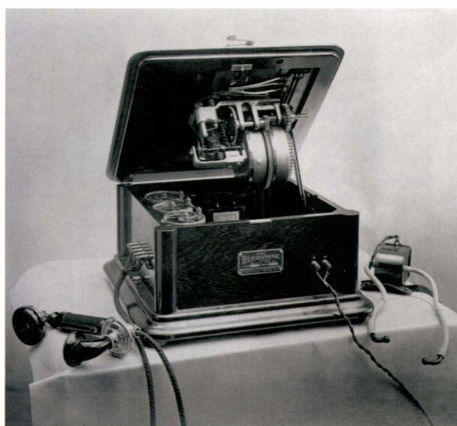
Right: Valdemar Poulsen's Telegraphone was an early ancestor of the tape recorder, recording audio using magnetic flux on a spool of wire. Note the telephone-style headsets.
