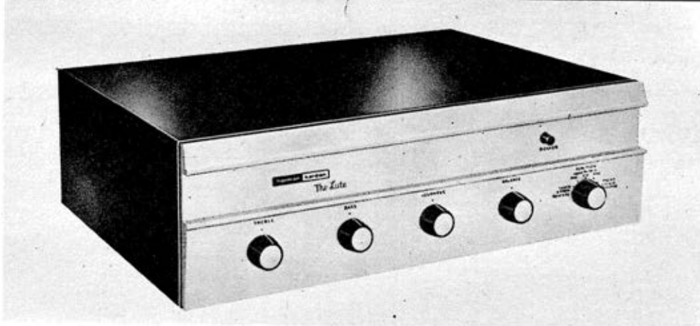
A220 stereo amp by Harman-Kardon gives 10 watts at each channel, has 8 and 16 ohm outputs. Inputs include phonograph, tuner and auxiliary. Crosstalk is below 50 db, hum is -70 db at low volume.
