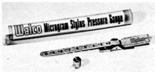
Above are some of the stylus pressure gauges available. At left is one by Cleveite Walco, at right is a Garrard. The Walco gauge is unusual in that it has no springs; it uses movable counterweight.
