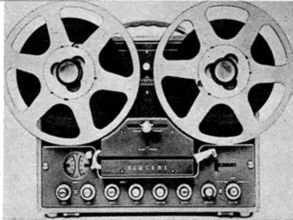
Newcomb stereo model SM-310 has 7½ and 3¾ ips speeds, two record level meters, synchronous motor, weighs 34 lbs. Response at 7½ ips is 30-15,000 cps ± 2 db. signal to noise: 50 db. It has two input jacks (rear view, below) for mike, two high level inputs and three output jacks.
