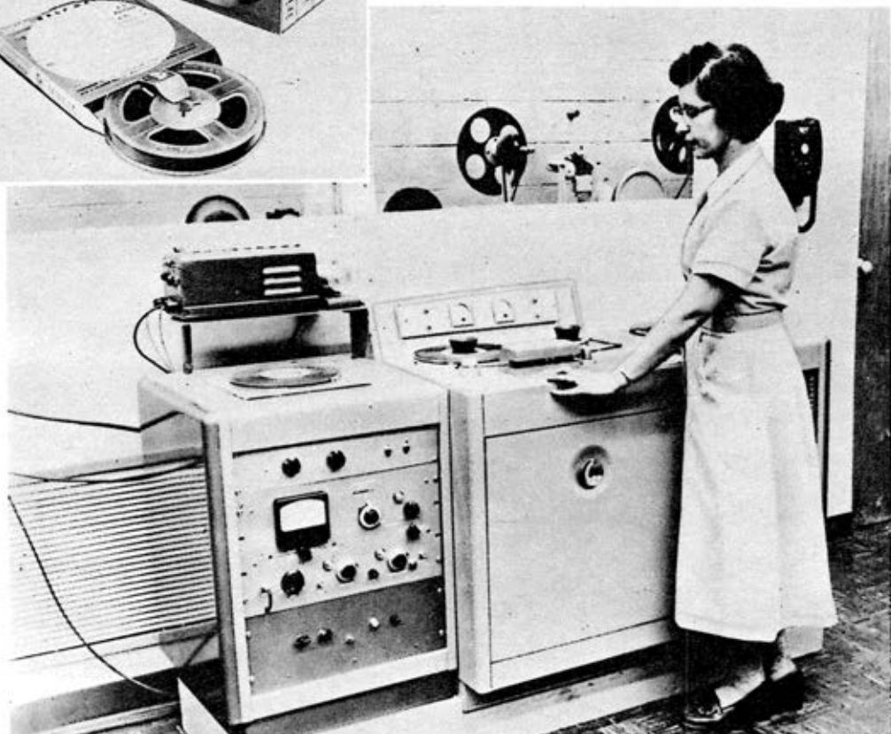
View of Soundcraft factory tape quality control room where tapes are tested against magnetic specs.
