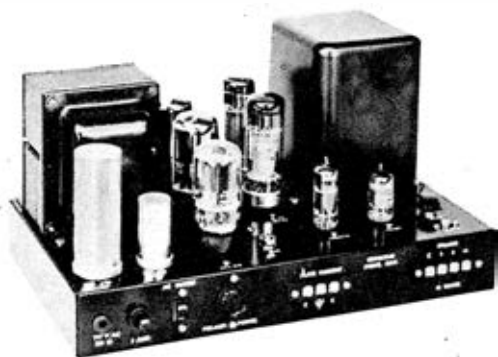
Grommes kit for 60-watt amplifier has damping factor of 15; 4, 8 and 16 ohm outputs. Hum and noise: 90 db below rated power. Feedback: 25 db.
