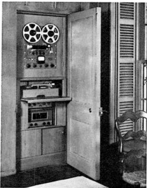
Professional Ampex 350 ($1,284) is featured in this installation. Below is a D&R turntable with a Pickering 190D arm. A Fisher 80C preamp and AM-FM tuner are at bottom above disc storage.
