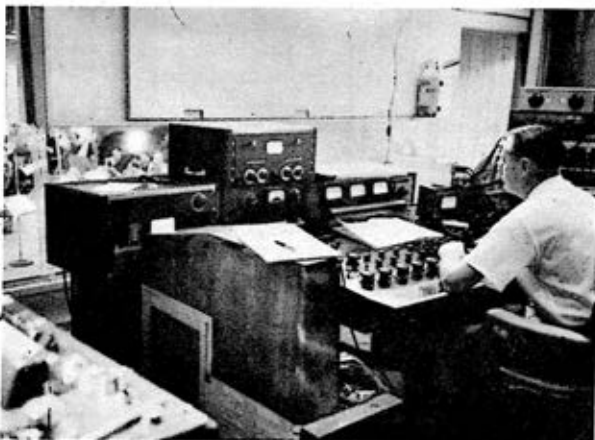
Main console of Columbia Records' New York 30th Street studio control room. All sound is fed through here before going onto the tape machines.
