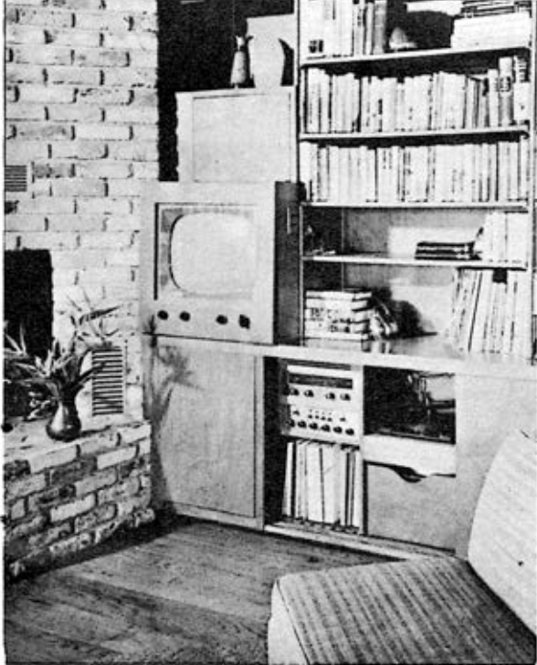
Built-in stereo system includes a Fisher AM-FM tuner and 400-C stereo preamp, two Fisher amps (not shown), Garrard changer, Model RC-88, a JBL 001 speaker system and Ampex 910 stereo deck.
