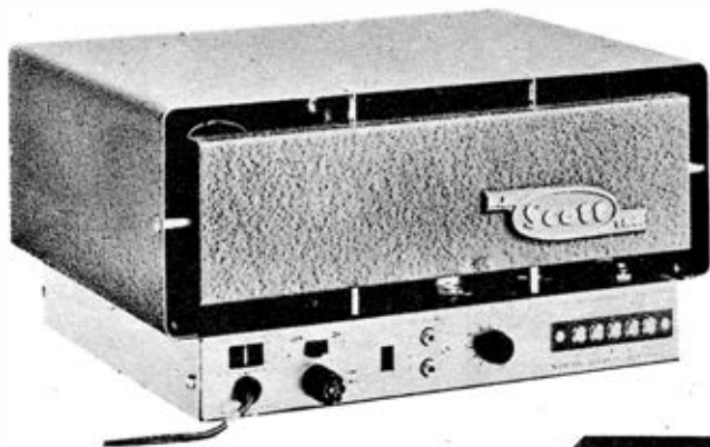
H. H. Scott basic 40-watt power amplifier has flat frequency response from 12-40,000 cps. Speaker outputs available are 4, 8, 16 ohms.
