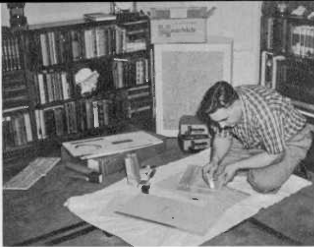
3: Heathkit SS1 is assembled with new fast-drying glue; it is designed to match Model SS1B Range Extender Kit, making 4-way system.
