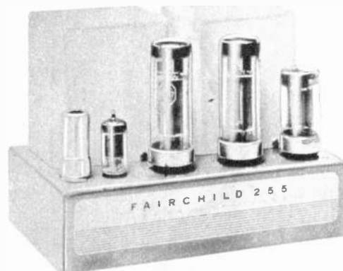
The Fairchild 255 power amplifier has an output of 30 watts, retails for $100.
