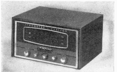
SR-406 Radio Receivers .....$249.95 A combination AM-FM Radio, pre-amplifier, and 20 watt amplifier. Peak power output 32 watts, 20 watts at 1% total harmonic distortion. Sensitivity 5 microvolts for 30 db quieting. Microphone, crystal phono, magnetic phono, auxiliary inputs, 30 to 20,000 cps. Tape recorder output jack. Output taps for 4, 8, 16 ohms. Bass control—15 db boost, 10 db droop at 50 cps. Treble control—10 db boost, 15 db cut at 10,000 cps. U.L. approved. 8"x15½"x11½".
