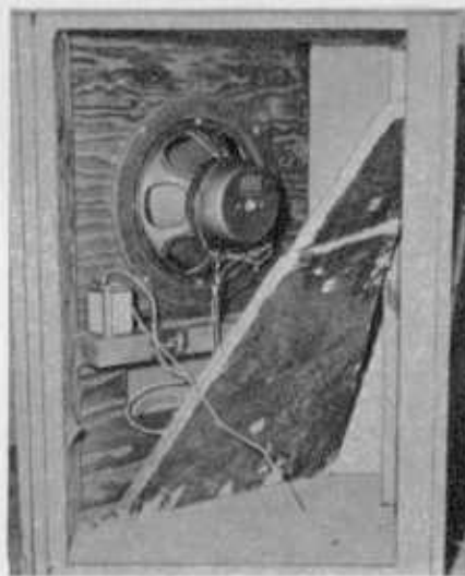
Above, two views of the Altec Lansing 606 corner bass reflex enclosure ($156). Note in cutaway the relationship of the speaker opening to the reflex port below it. Cabinet can be used as multi-speaker setup.
