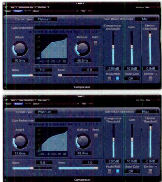
'Hard-knee' (top) and 'soft-knee' (bottom) settings on a plug-in compressor. Notice the difference in the compression curve for each type.
