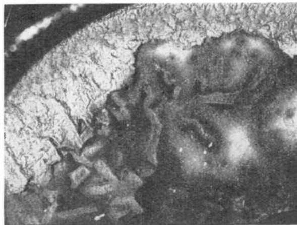
Fig. 20. Photo-micrograph of a portion of the cathode surface of a CV1070 glow-discharge tube after 2,000 hr. continuous operation at a current of 5mA.
