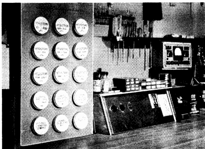
Fig. 80— Rock for storage jars can be made from plywood panel, Masonite, or scrap wood.
