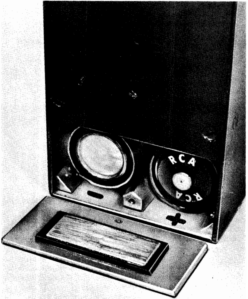
Fig. 166—Battery compartment with batteries installed.
