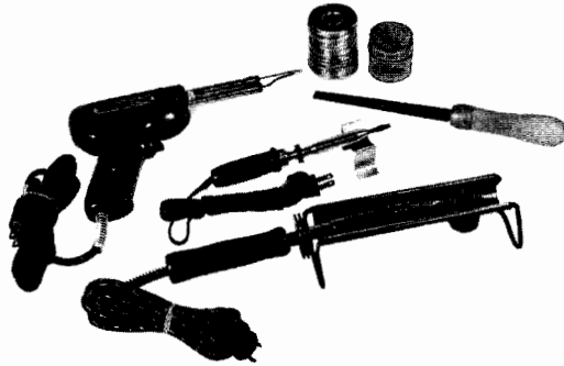
Fig. 3—General-purpose soldering gun of top has built-in spotlight. Small soldering iron of center is useful for printed circuit work and miniaturized projects. Large iron of bottom is suitable for most types of electronic work.
