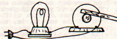
13-1. Counter emf. in an AC Motor.
