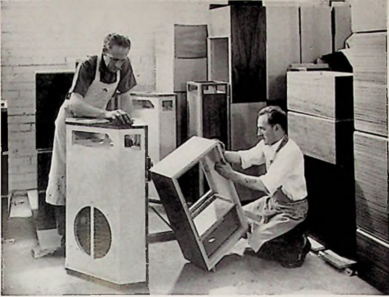
FIG. 7/2. Staining and filling cabinet surfaces in one operation.
