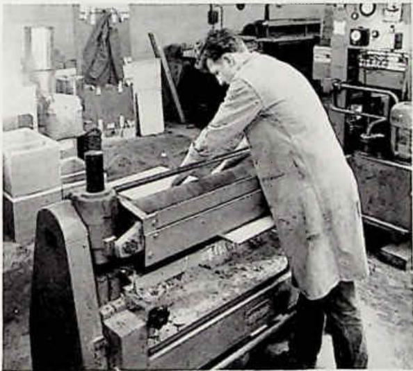
FIG. 4/3. Machine for spreading cold glue by rollers.
