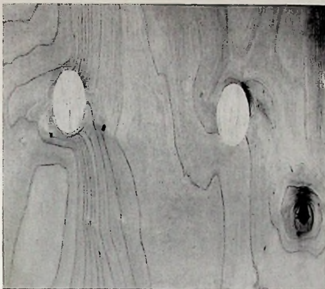
FIG. 2/3. Grade BB birch plywood, showing permitted plugs and small knots.
