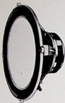
FIG. 10/2. 12" loudspeaker with \frac{3}{4} " thick flat polystyrene diaphragm added to absorb enclosure resonances.
