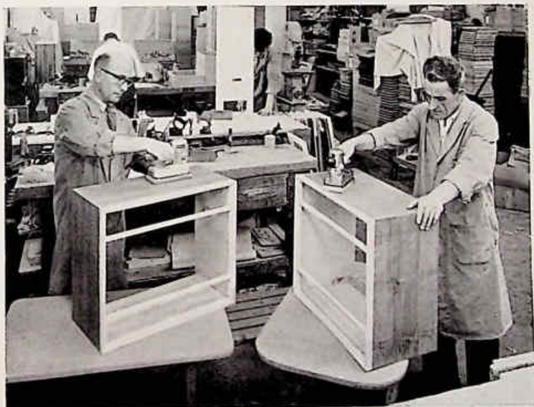
FIG. 7/1. Final sanding of cabinets preparatory to polishing.
