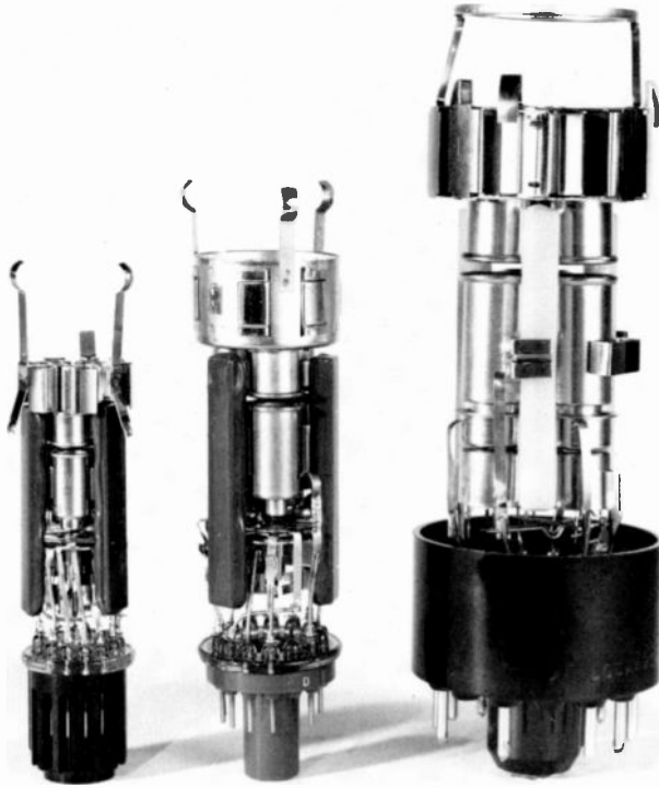
Fig. 5.27. Photograph of electron guns commonly used in 70°, 90°, and 110° shadow-mask color tubes.
