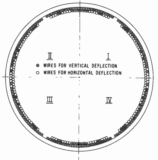
Fig. 5.42. PST winding distribution.
