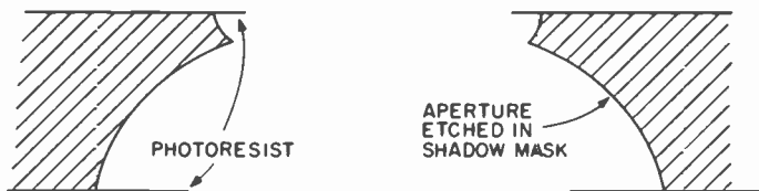
Fig. 5.35. Aperture etched in shadow-mask with photoresist still in place. The surface of the mask with the small opening faces the gun.
