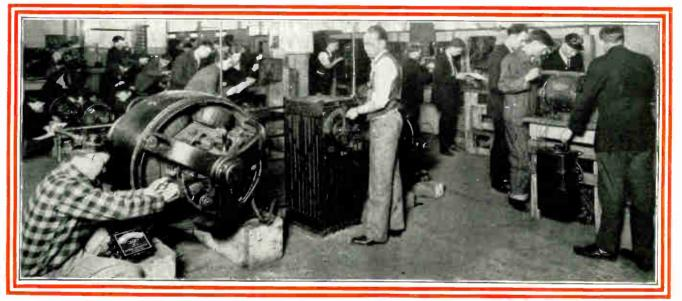
Here you see several students testing and operating D.C. machines. The large machine at the left is used to make practical demonstrations of dynamic braking on large motors. Here you see students doing work on advanced equipment, fellows who a short time ago may have knawn mothing about this work. But this is now easy for them, because they have reached this department step by step.
