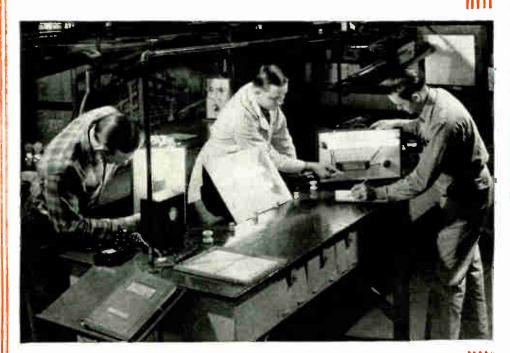
Instructor explaining principles and operation of new type fluorescent lighting units to students, as they perform shop tests on these units. This type of lighting equipment is becoming more popular every day for factories and industrial plants. It is frequently used to provide day-light working conditions to night workers.
