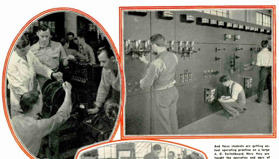
Real practical work overhauling and repairing an A. C. induction motor. When you understand the working parts of such equipment you have confidence in your knowledge of this work. And these students are getting actual operating practice on a large
