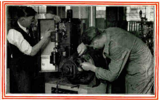
These students are checking the operation of an automatic controller and compound motor. They are making the same test and repairs they may be called upon to make in the field.
