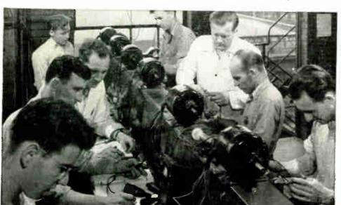
Here you see students getting training and practice in proper procedure in eliminating bearing trouble. The student with the Instructor is using a Line Reamer to align bearings on a Fractional Horsepower Motor. The service man in the field will find this training a mighty valuable feature of this Department.
