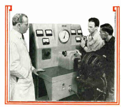
These Coyne students are testing a generator with a modern Dynamometer, a type used extensively in industry for testing A.C. and D.C. motors and generators.
