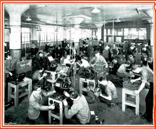
These fellows are connecting up, testing and repairing various types of A.C. motors and controls. When they get the machine running and understand its operation, use, and care, the instructor checks their work, so they know it is right, and when they leave school to take a job on the outside, it's just like changing jobs.
