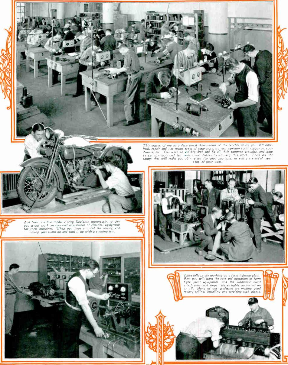
These feelows are using modern garage type test benches for giving final running tests to generations and starters they have overhaued and repaired. Your work on such equipment will help you qualify for the real jobs in this line. And here you see a Packard "& cylinder in line" engine. These men me checking the firing order and connecting ignition wires to the spark plugs properly. Work on such engines as this makes you able to handle the good jobs in ignition work.
