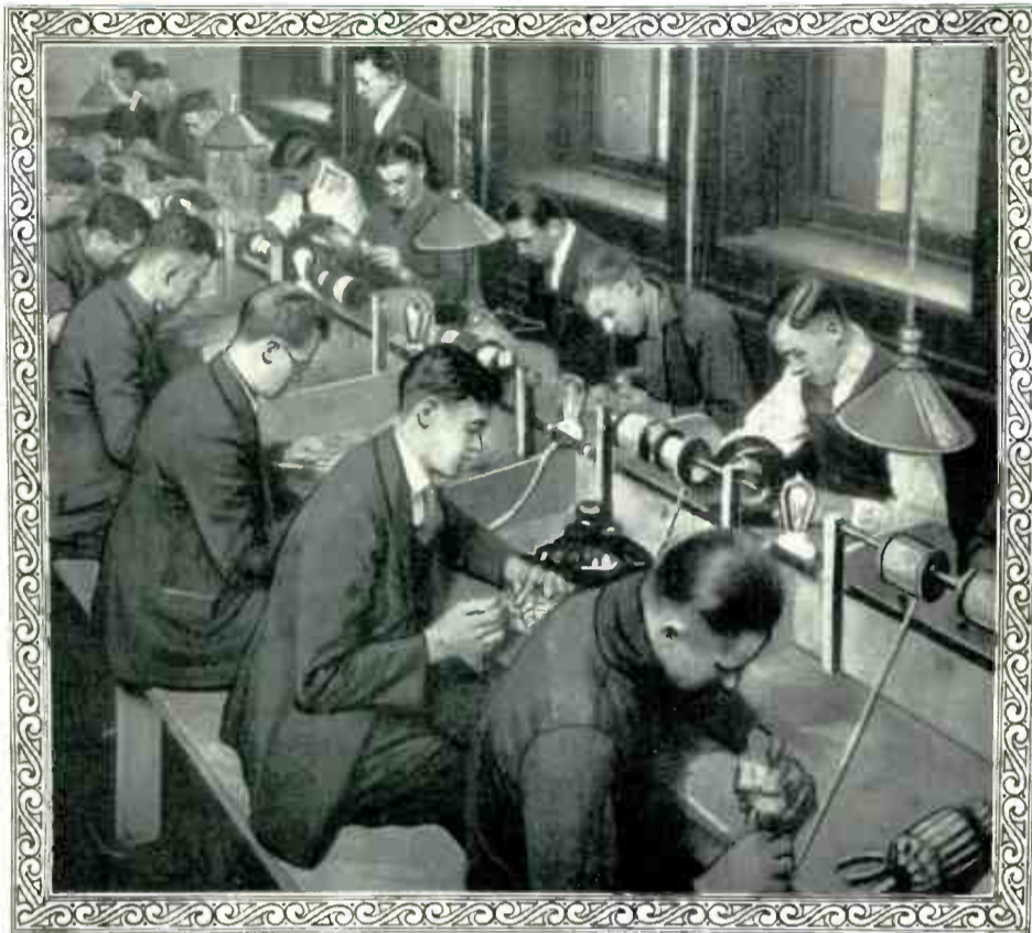
Students Winding Armatures and Stators. Note That This Is Actual Wire Winding
