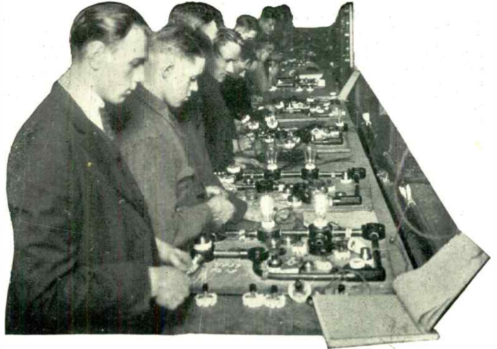
Wiring Up Switches and Fittings on Detail Boards
