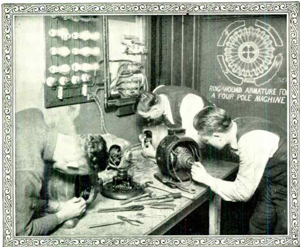
Assembling and Testing Re-wound Armatures
