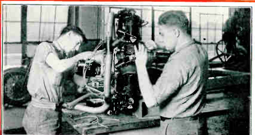
Students in our Aircraft Ignition section assembling and wiring ignition equipment and adjusting magnetos on a radial aircraft engine.
