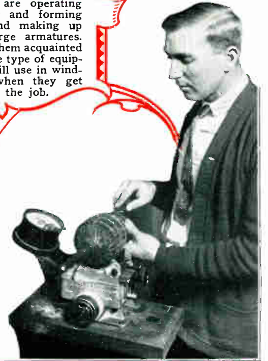
This Student is testing an armature on the growler, a machine for quickly locating trouble and faults in windings. This kind of instruction enables our graduates to get right at the cause of armature troubles without waste of time.
