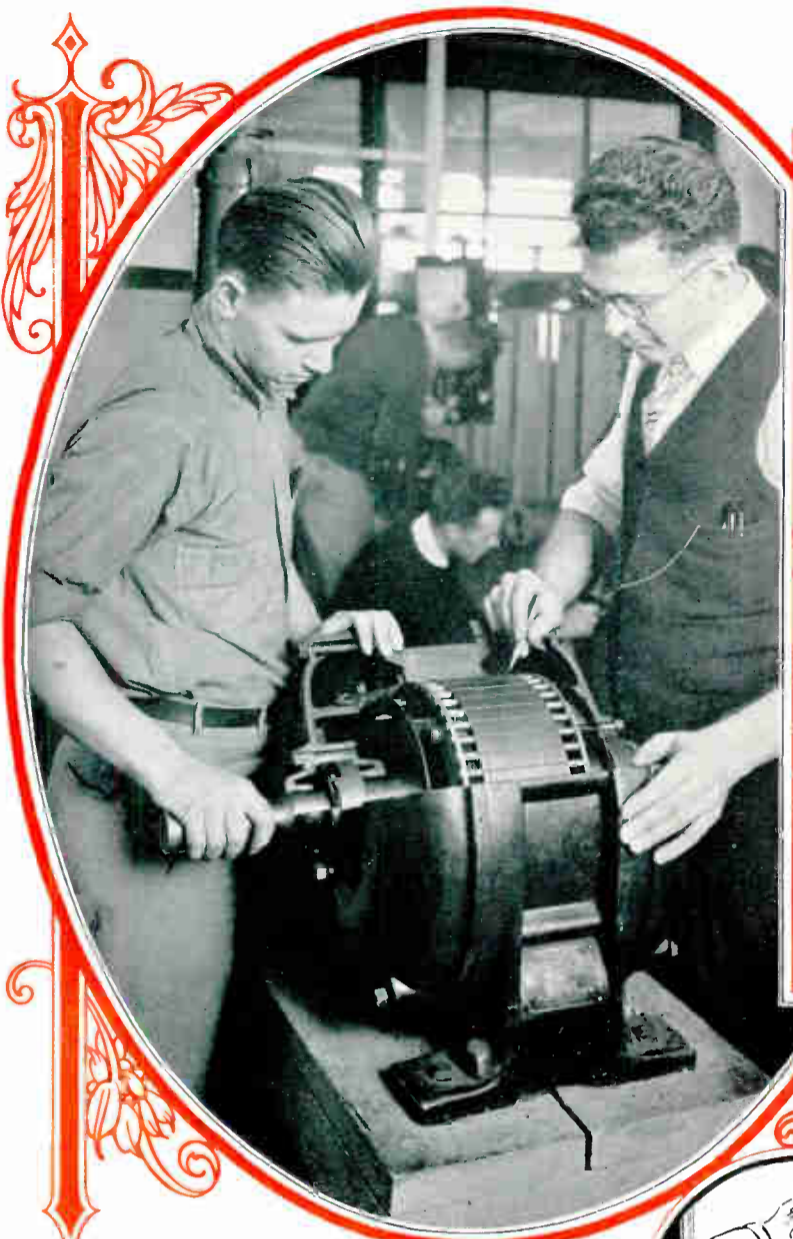
Here an instructor is explaining important principles of an induction motor, on a machine specially cut away, so the student can observe these points both while the motor is idle and when it is running. This is an example of how some of our specially prepared equipment will save your time, and quickly and easily make its operation clear to you.
