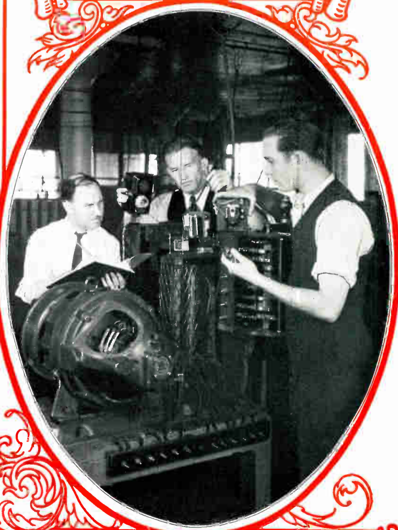
Here you see some students working on a synchronous converter, and making some very interesting connections and tests, under the supervision of the instructor on the right. This machine is used to change Alternating Current to Direct Current. It's the actual work on such equipment as this that gives Coyne graduates ability and confidence.
