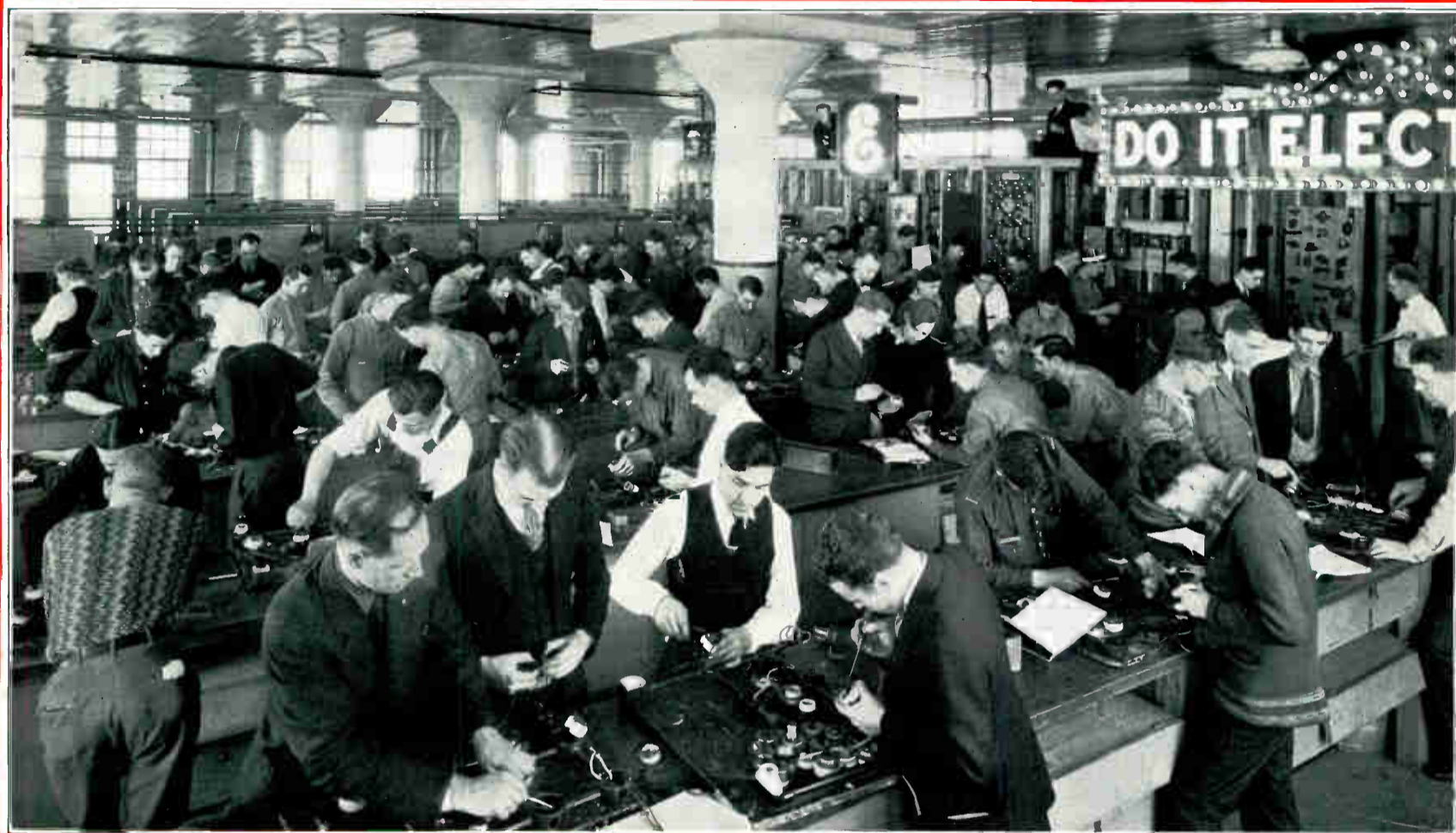
General view of a section of the construction or wiring department. Notice the large and well lighted shop. The men are wiring and testing light control circuits in their first small conduit layout, and getting real practical experience in the handling of tools and different kinds of switches.
