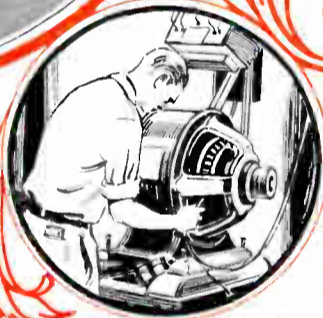
Here an instructor is explaining important principles of an induction motor, on a machine specially cut away, so the student can observe these points both while the motor is idle and when it is running. This is an example of how some of our specially prepared equipment will save your time, and quickly and easily make its operation clear to you.
