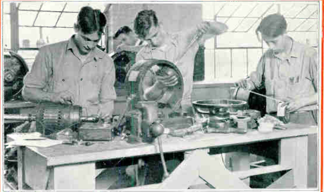
Real practical training. These students are completely overhauling and repairing a D. C. motor, and repairing the field coils, and the commutator and armature.
