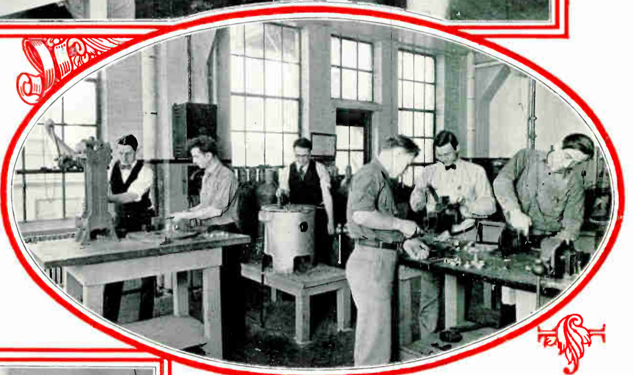
And these students are melting lead in a modern electric melting pot, and moulding lead posts and straps for the batteries they are building. This work gives them excellent practice with tools, and modern equipment.
