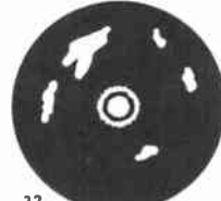
32 TYPE PPI DISPLAY. CIRCULAR SCAN—AZIMUTH, RADIAL DISTANCE = RANGE
