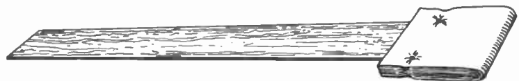
To properly clean a commutator, use a piece of dry canvas or other hard non-linting material which is wound around and securely fastened to a wooden stick, and held against the commutator.
