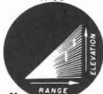
28 TYPE E, SIMILAR TO (27) BUT Y AXIS SHOWS ELEVATION ANGLE
