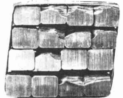
Example of a set of brushes fractured as a result of brush chatter caused by high mica and rough commutator surface.
