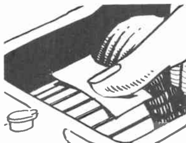
Fig. 1—Sanding a commutator. The best method is to hold the sandpaper with a strip of hard wood.
