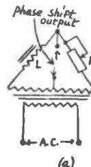
Circuits for phase-shifting an A.C. voltage
