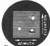
26 TYPE C—RECTANGULAR COORDINATE SCAN, MODULATED AS IN TYPE B
