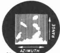
25 TYPE B—RECTANGULAR DISPLAY WITH INTENSITY MODULATED BEAM
