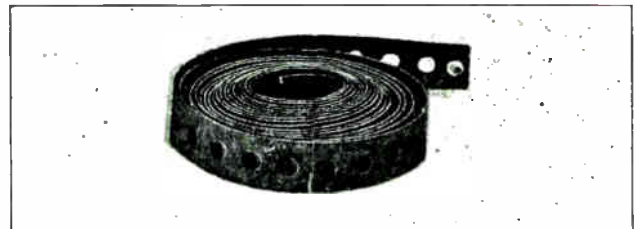
Fig. 74. Copper grounding strip of the type shown above is often used to ground conduit systems to the waterpipes or earth grounds.
