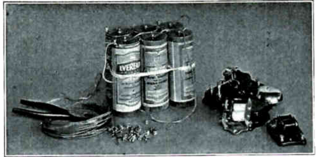
Fig. 12. Six dry cells connected parallel-series, for use in an alarm system.
