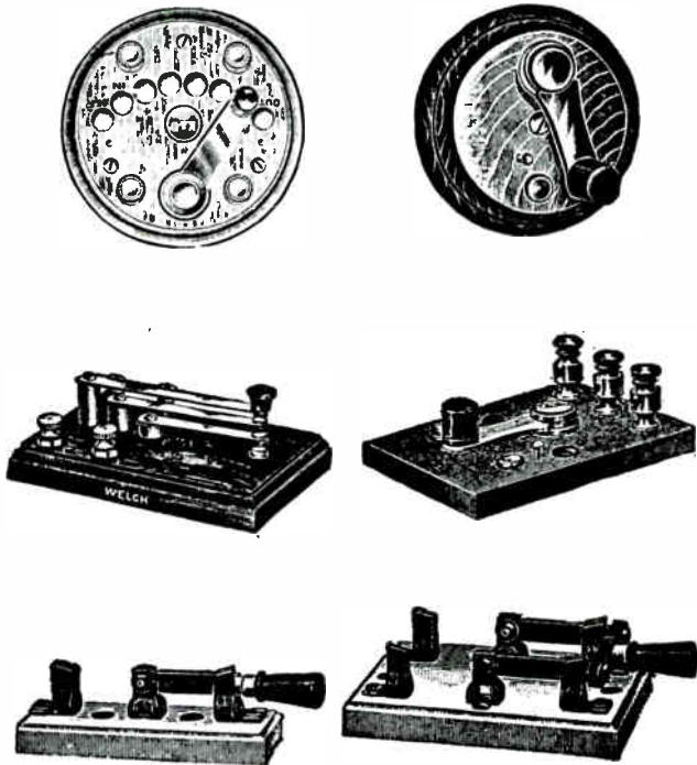
Fig. 27. Several different types of switches used in signal work. The two above are called Lever Switches. In the center on the left is a Multiple Key Switch; at the right double circuit Lever Switch. Below are two Knife Blade Switches.
