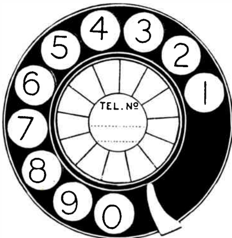
Fig. 152. Front view of dial, showing finger plate, holes, numbers and finger stop.
