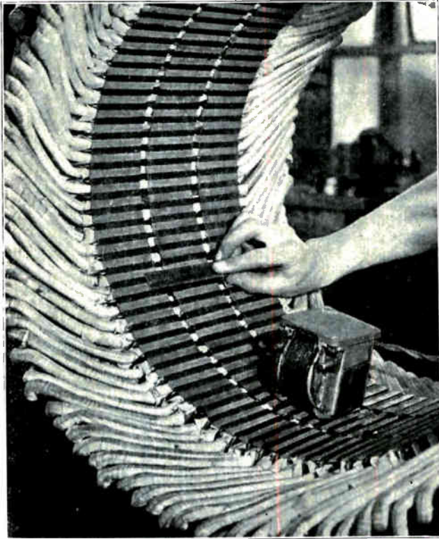
Fig. 95. This photo shows a growler in use in a large stator. Note the size and shape of these coils and the position of the steel strip which is just the width of one coil from the center of the growler.
