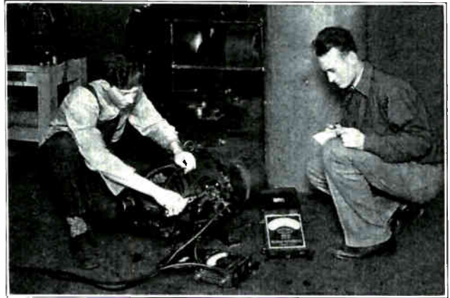
Fig. 8. Using meters right on the job to test a motor. When you know the rating of a machine in volts and amperes, it is easy to determine with meters whether the machine is properly loaded or not.
