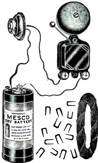
Fig. 1. Materials and parts for a simple doorbell or call system. Note how the dry cell, bell and button are connected.
