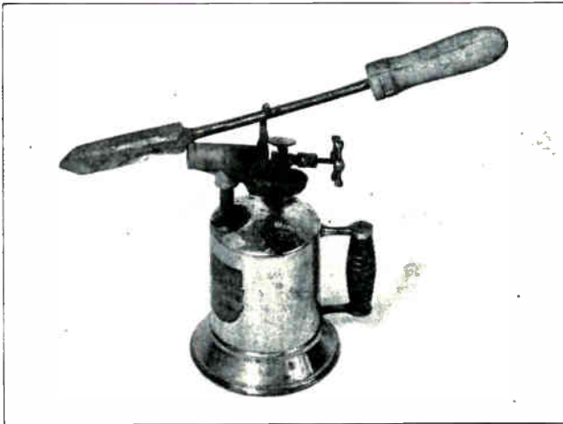
Fig. 21. This photo shows a gasoline blow torch such as commonly used for heating soldering coppers, and splices in electrical conductors.
