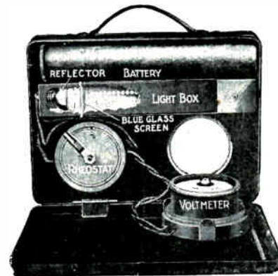
Fig. 166. This view shows the important parts of a foot-candle meter. Note the arrangement of the standard lamp behind the paper screen, and also the rheostat and voltmeter used in making proper adjustments.
