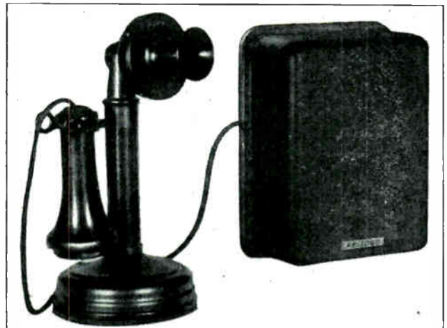
Fig. 134. Common desk type telephone with bell box to be mounted separately.
