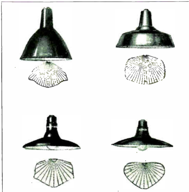
Fig. 171. Above are shown several types of porcelain enameled, metal reflectors. Note how their various shapes give different distribution of the light, as shown by the curves under each reflector.
