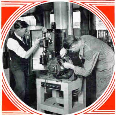
These students are being trained in the operation of an automatic controller and compound motor, and to make the same test and repairs they may be called upon to do in the field.
