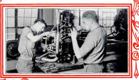
Students in our Aircraft Ignition section assembling and wiring ignition equipment and adjusting magnetos on a radial aircraft engine.
