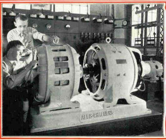
Here you see some students working on a synchronous converter, and making some very interesting connections and tests, under the supervision of the instructor on the right. These machines are used to change Alternating Current to Direct Current. It's the actual work on such equipment that gives Coyne graduates ability and confidence, in their work.
