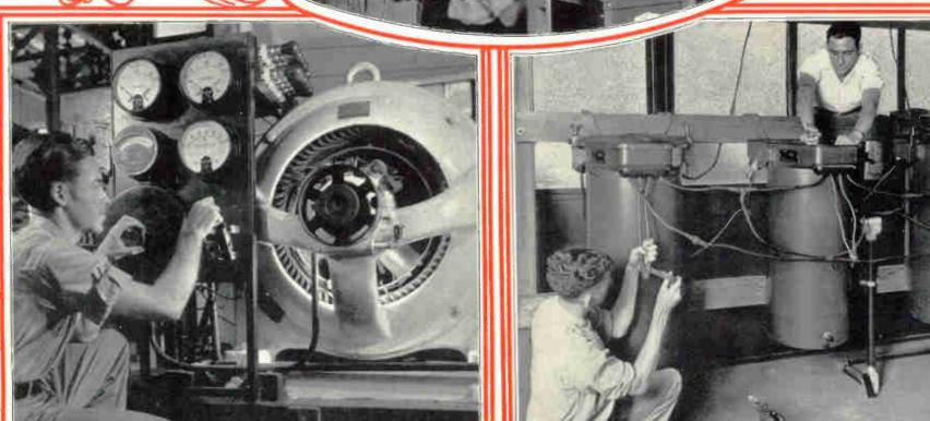
A student preparing to test a large synchronous motor which is used for correcting power factor and saving money on power bills. Every trained electrical maintenance man should be familiar with this type of work.
