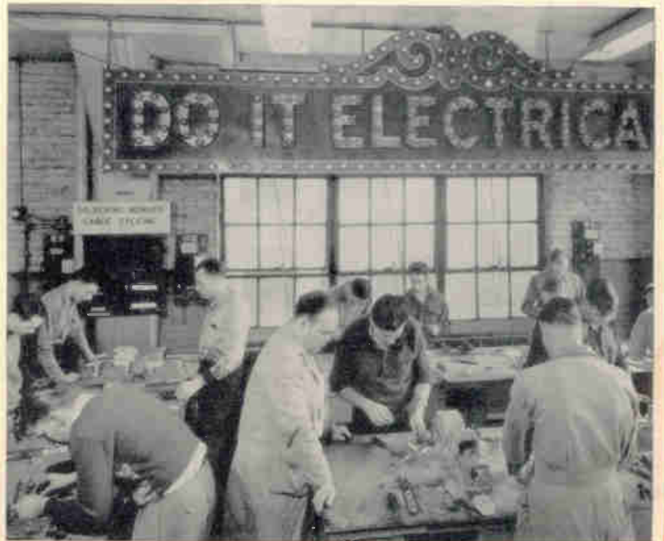
In this picture you see students doing splicing and soldering. The instructor has shown them how to strip the wires and make the common splices. Students then perform this job themselves.
