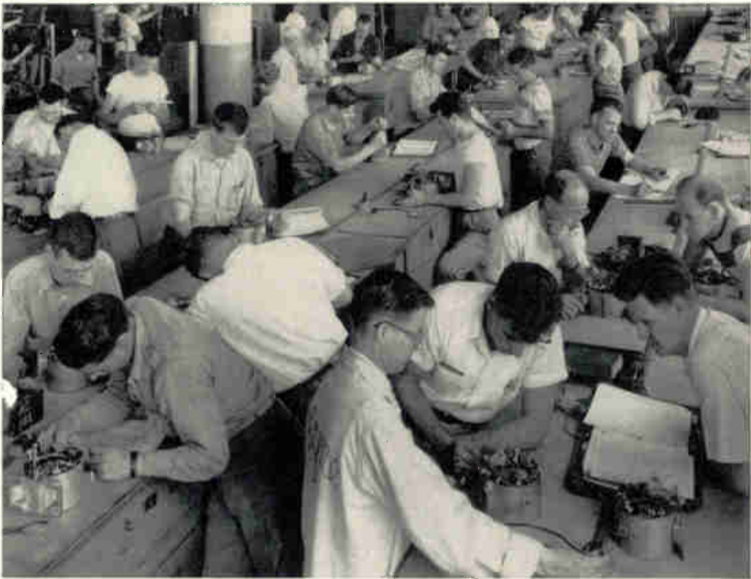
Here you see a view of the Stator Winding section. Notice that real wire is used in winding these stators. Actual winding and testing of Alternating Current motors gives you the practical training you need in this work. Motor repair work of this kind is often necessary in Electrical maintenance jobs in Power Plants, Factories, Stores, Office Buildings and, in fact, wherever Alternating Current motors are used.
