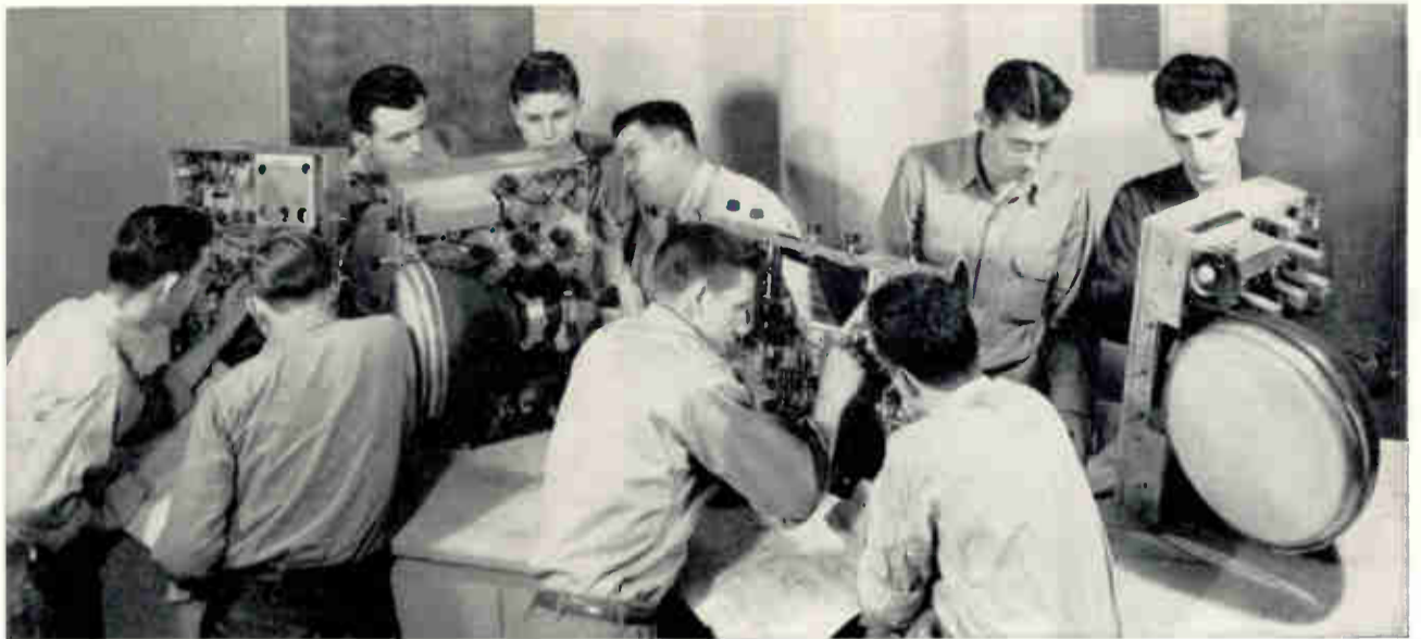
Here you see students checking the wiring and tracing the circuits of Television Receivers. This actual practice and practical experience qualifies them to quickly locate the troubles in Television Receivers they may find in service work out in the field.
