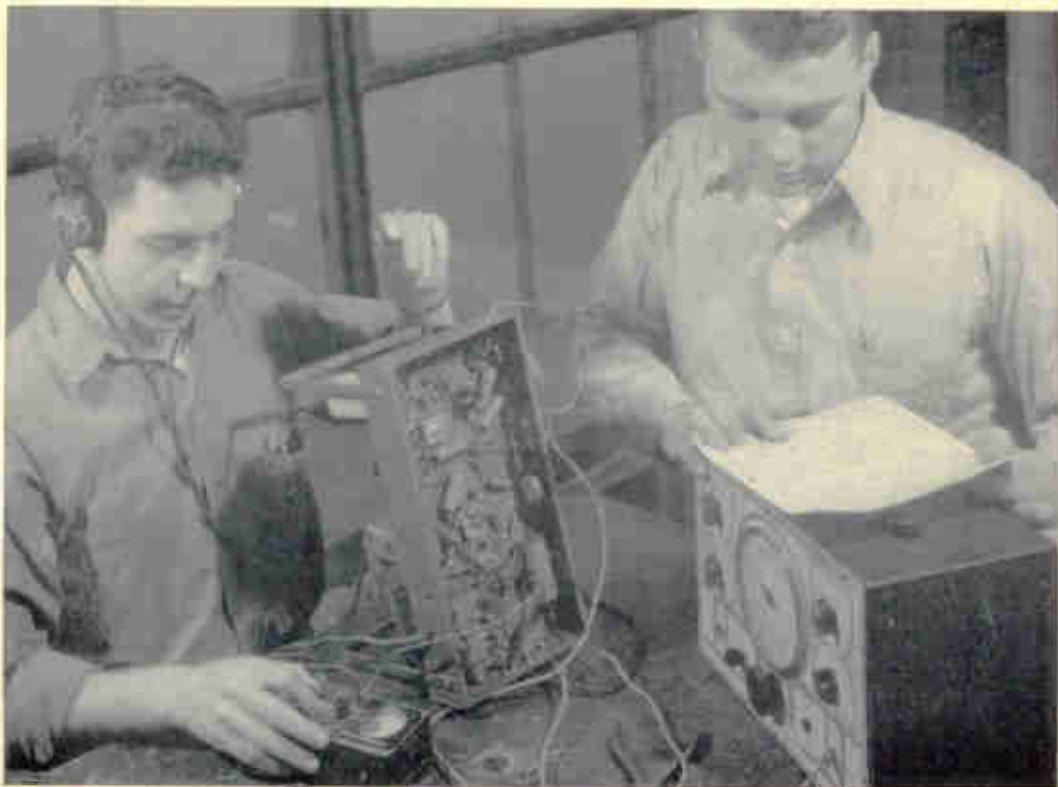
In this department students actually build a T. R. F. Receiver and a Superheterodyne Receiver. They get a chassis and all the parts from the stock room and step-by-step they assemble the receiver. In the above photo these students have completed their receiver and are doing aligning and making tests with various testing instruments. The testing methods learned here are later applied to other types of Receivers.
