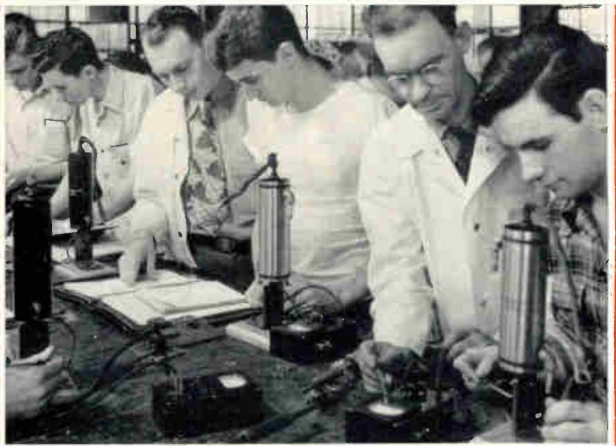
The Ignitron Tube has proved invaluable for use in Electronic Switches, Welding Controls, and many other applications. The photo above shows students getting practical experience and instruction in the operation of this Electronic Tube.
