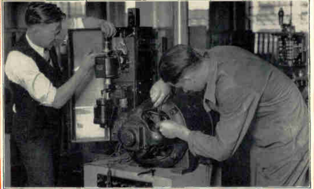
These students are checking the operation of an automatic controller and compound motor. They are making the same test and repairs they may be called upon to make in the field.
