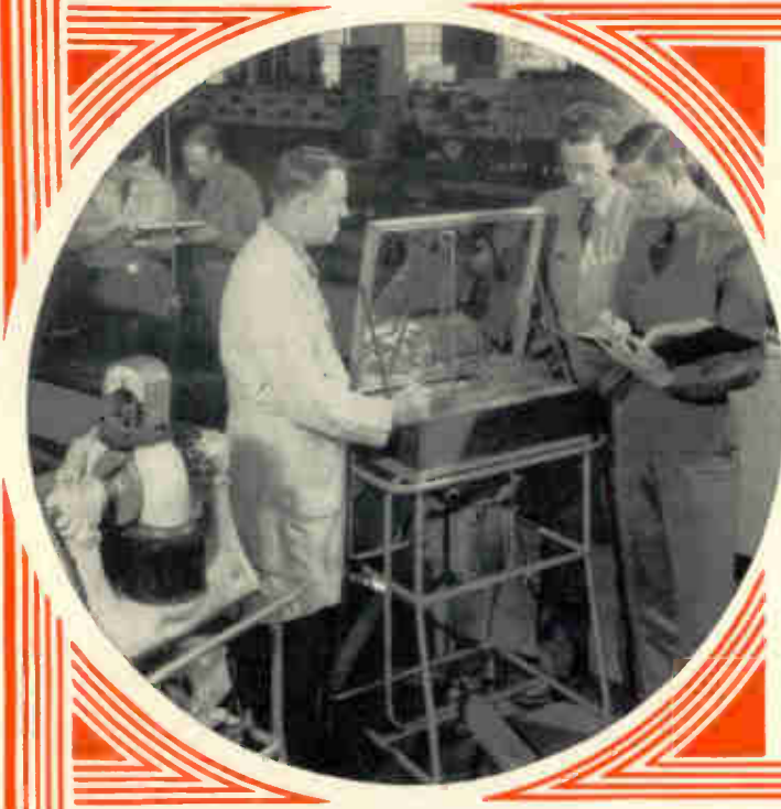
Specially designed demonstration units and personal instruction make the principles of Electricity and Magnetism clear to students. On the left is a unit for demonstrating magnetic fields around conductors and coils.
