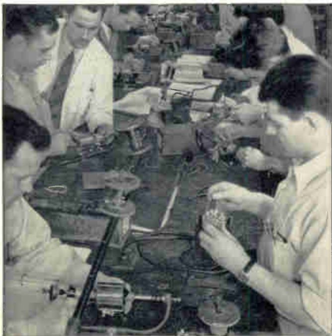
This is a view of a part of the Armature Winding bench. Notice that these students are winding Armatures with actual wire. After they have wound their Armature, it is mounted in a motor housing and checked under actual operating conditions.
