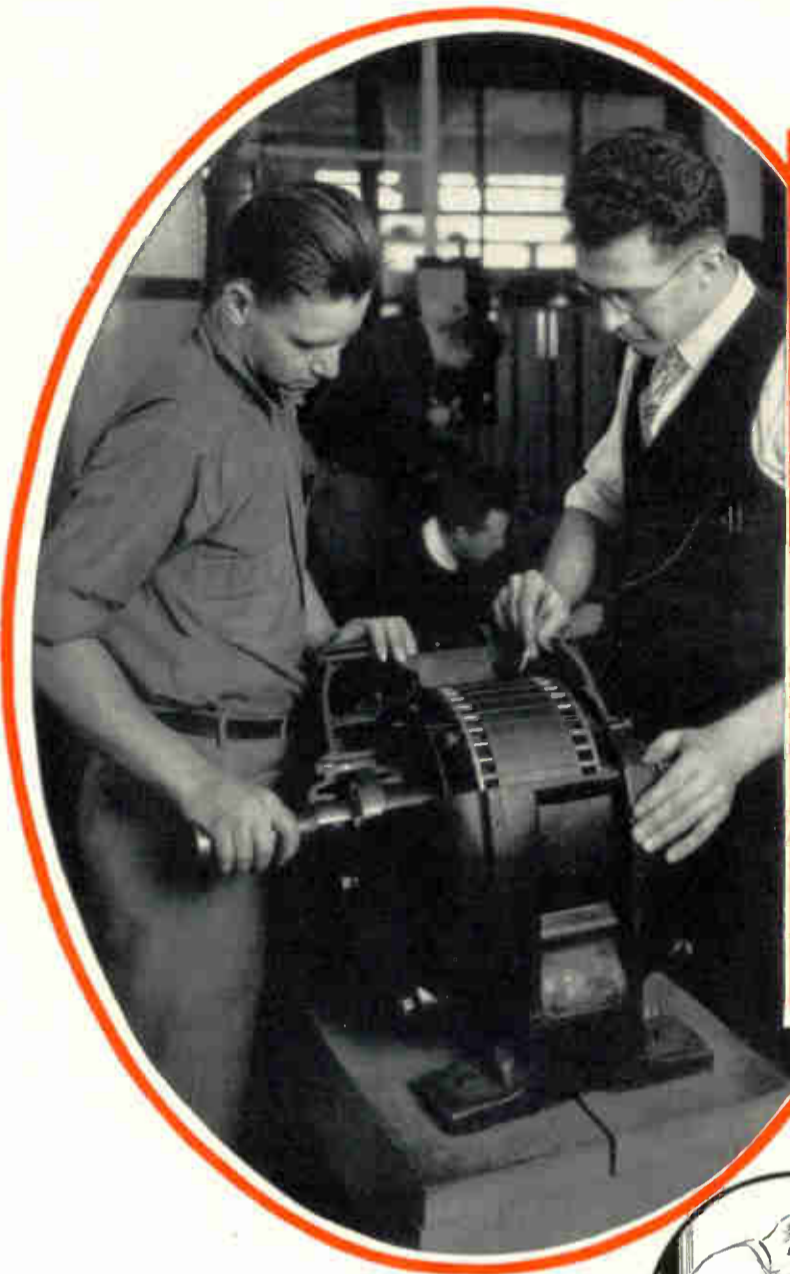
Here an instructor is explaining important principles of an induction motor, on a machine specially cut away, so the student can observe these points both while the motor is idle and when it is running. This is an example of how some of our specially prepared equipment will save your time, and make your training easier.
