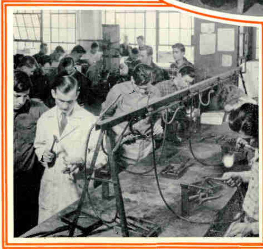
This photo shows the set-up for giving students training and practical experience in cutting and swedging copper tubing. An instructor is always handy to answer questions or make clear any particular operation.
