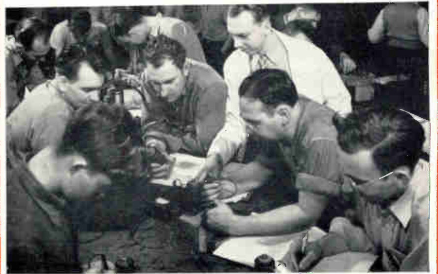
This picture shows a group of Coyne students testing Copper Oxide Rectifiers. This unit is a very important part of a large number of Industrial Electronic Controls, so it is important for the Electrical man to understand the use and application of this equipment.
