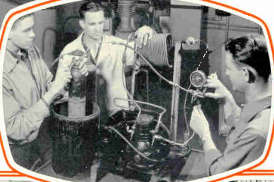
The photo to the right shows students charging a Refrigerator unit under the supervision of an instructor. This type of experience gives students the confidence to do these jobs out in the field.
