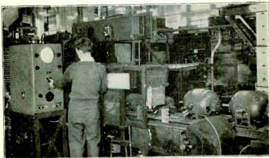
Fig. 296. Testing the insulation of windings with the help of a cathode-ray tube.
