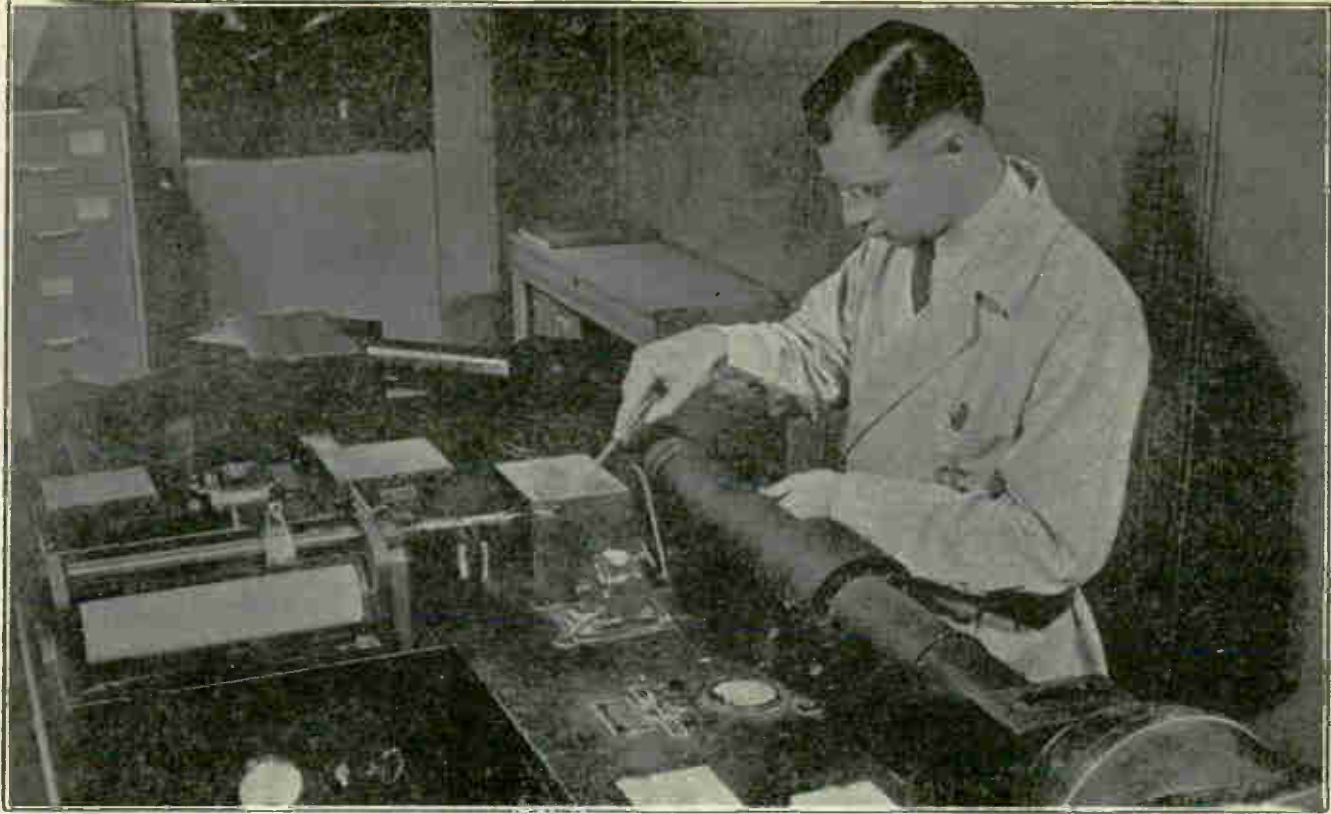
A RECORDING SPECTROPHOTOMETER, a high precision electronic instrument widely used in the paper, textile, chemical and paint industries for analyzing quality and color of product. Radio men and electricians with a knowledge of electronics are needed to install, maintain and operate this as well as other types of electronic equipment.
