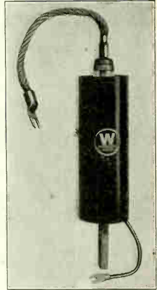
Fig. 316. A welding ignitron WL-652 rated for a maximum demand of 600 kilovolt-amperes.
