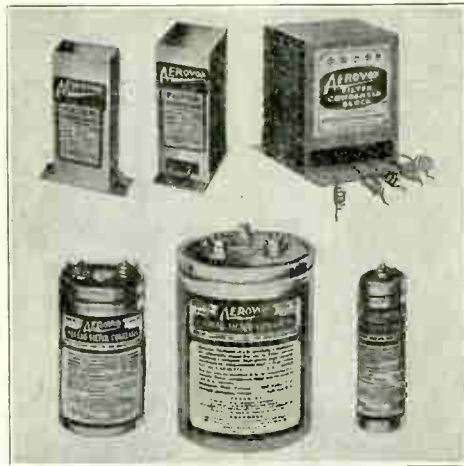
Fig. 65. Paper capacitors (top row) and electrolytic capacitors (bottom row) such as used in filter systems.
