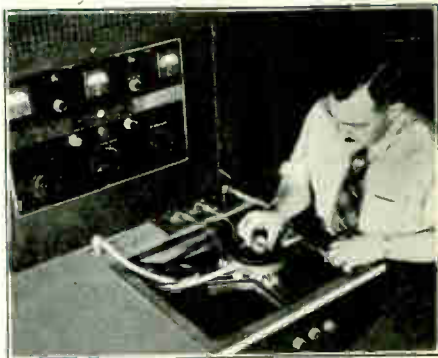
Fig. 243. The operator is placing a small gear in a fixture for induction heating as part of the process of surface hardening. The power oscillator to which connections are made is a 15-kilowatt unit.
