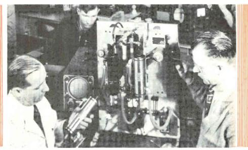
The "IGNITRON TUBE" has proved invaluable for use in Electronic Switches, Welding Controls and various other applications. The above photo shows an Instructor explaining the operation of this Electronic Tube.
