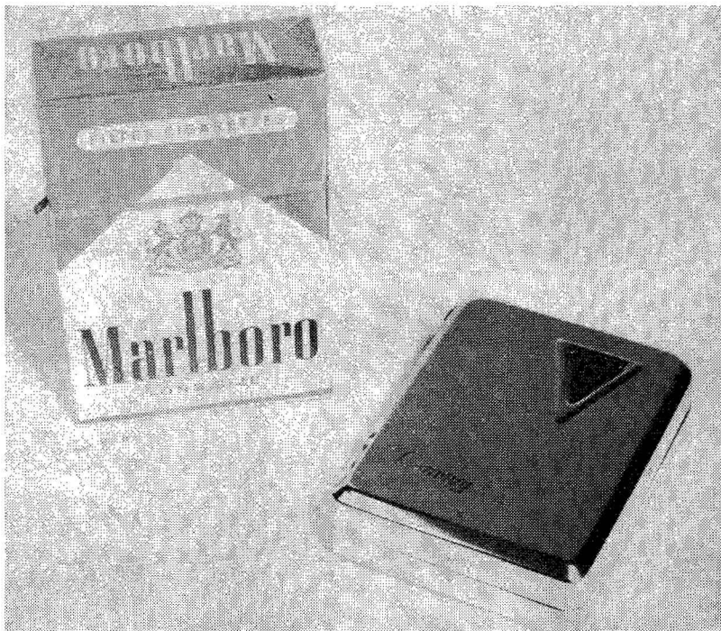
Fig. 2-16: A commercial transistorized Hearing Aid. The unit is smaller than a package of cigarettes. Some Hearing Aids are even smaller and weigh but a fraction of an ounce.
