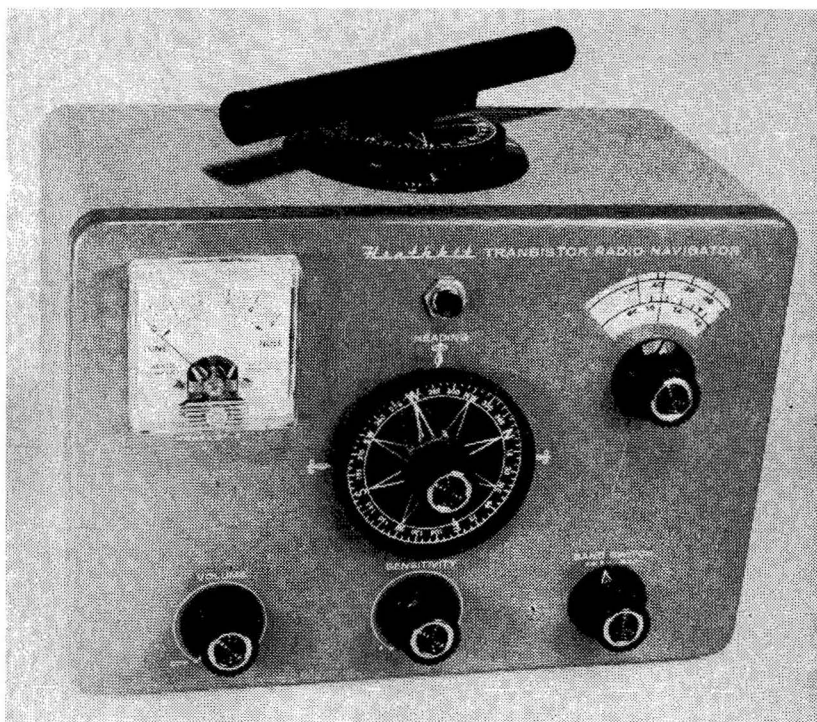
Fig. 9-4: The HEATH Model DF-2 Radio Navigator—basically a two-band transistorized receiver, this type of set is used extensively in marine installations.
