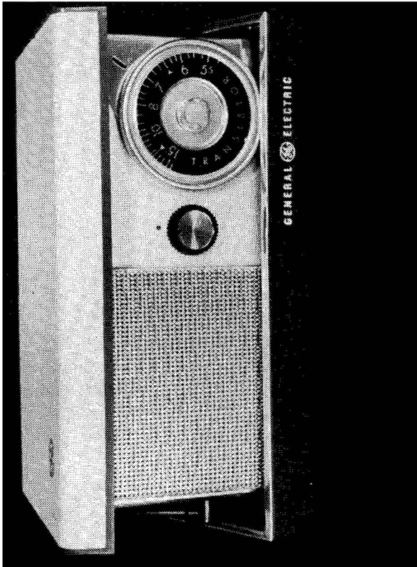
Fig. 5-30: The GE Model P-715D receiver, setting upright in its "travel case." Many portable receivers are designed to serve both as "portables" and as "table model" sets.
