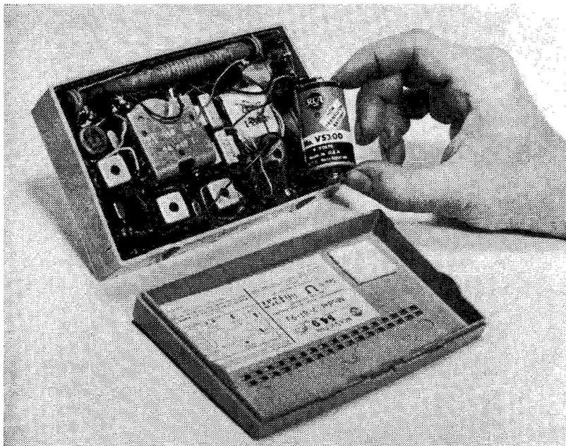
Fig. 5-24: Rear view of the 7-BT-9J receiver with back cover removed. Proper technique for battery replacement is shown.
