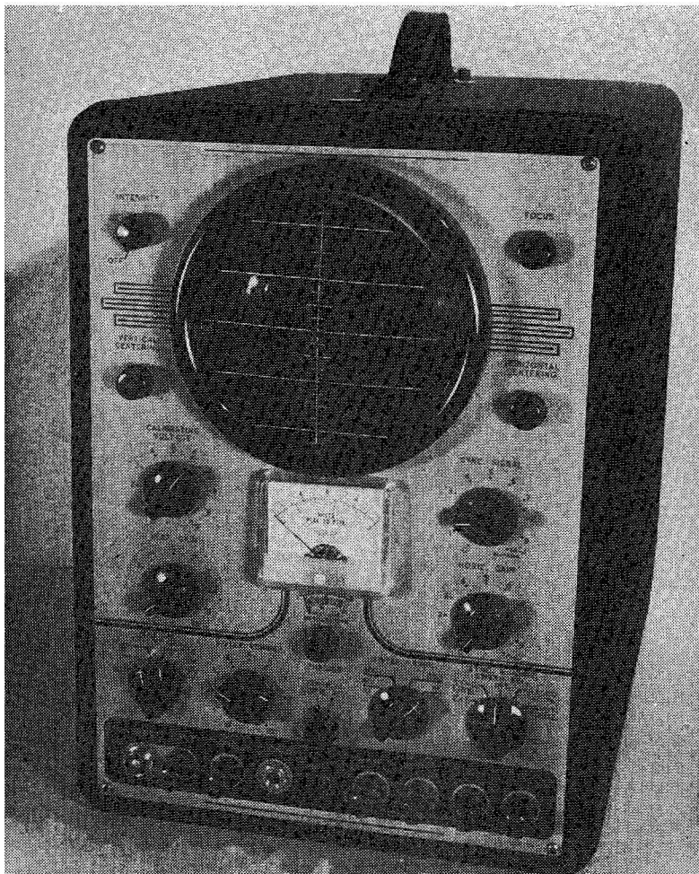
Fig. 1-12: A good general-purpose Oscilloscope, while essential only for a few service jobs, is valuable for signal-tracing and waveform checks in transistorized instruments, TV sets, and similar gear.
