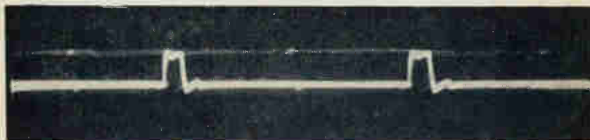
Fig. 9-18-3. These horizontal pulses go to the horizontal afc system, from 3 of Fig. 9-15.
