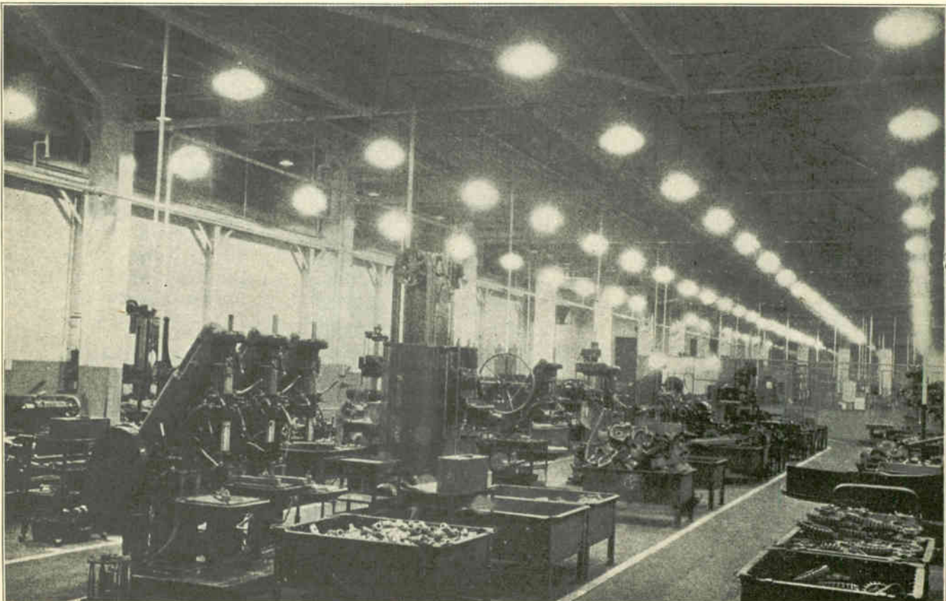
Fig. 188-B. This photo shows a view in a well lighted machine shop. It is easy to understand why production can be increased and greater safety obtained in a shop which is lighted in this manner. (Photo Courtesy Light Magazine).
