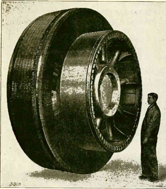
Fig. 13. This large armature shows the size to which D. C. generators can be built. An armature of this size would develop several thousand horsepower.
