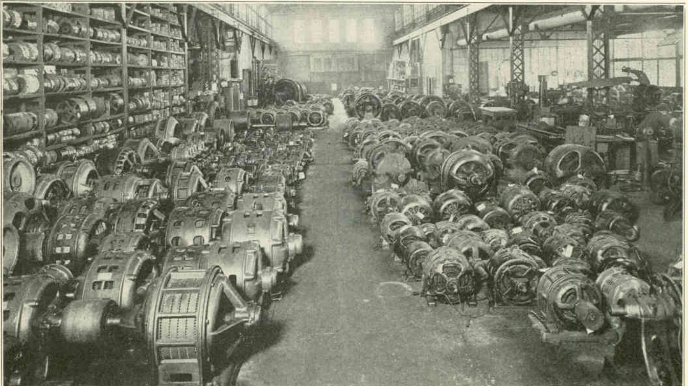
Fig. 1. This photo shows a view in a modern electric repair shop. Note the great number and variety of electrical motors and generators which go through this shop by the thousands each year. They are tested, rewound, reinsulated, and generally repaired before going back in service.
