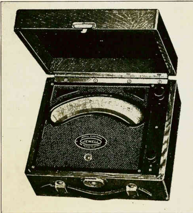
Fig. 83. Portable meters of the above type are very convenient and necessary devices for the practical electrician to use in testing various machines and circuits.
