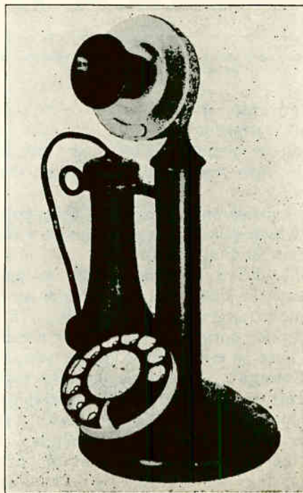
Fig. 148. Desk telephone equipped with dial for use on automatic exchange systems.
