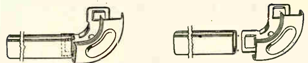
Fig. 93. A common form of elbow used with metal raceways or moldings
