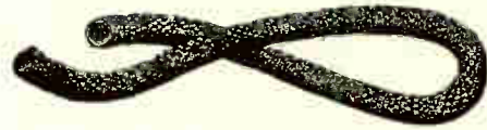
Fig. 37. A piece of "loom" or flexible insulation used to protect wires in certain places in Knob and Tube wiring.
