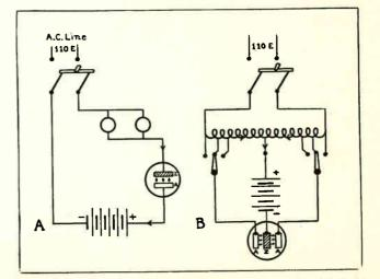
Fig. 226-A. Shows a half-wave, electrolytic rectifier and B shows an electrolytic rectifier of the full-wave type. Current can only pass through these devices in one direction. to the aluminum electrode A and then to the center lead electrode, because the current cannot pass through the rectifier in this direction.
