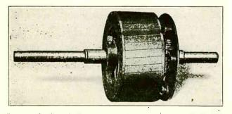
Fig. 164. Small squirrel-cage rotor such as used in single-phase induction motors. Note the centrifugal switch mechanism on the right end.
