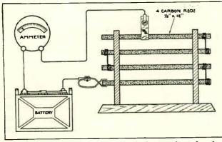
Fig. 23. Diagram showing construction and connections of a simple capacity test discharge resistance, which can be easily and cheaply made of carbon rods supported in an insulating frame of heat resisting material.
