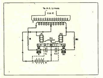
Fig. 225. The above diagram shows the parts and connections of a simple mechanical rectifier of the vibrating type. The synchronous operation of the contacts delivers pulsating D.C. to the battery circuit.
