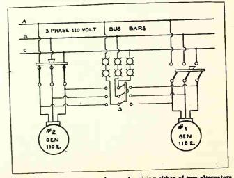
Fig. 95. Connection diagram for synchronizing either of two alternators with the bus bars by means fo a lamp bank and double-throw switch
