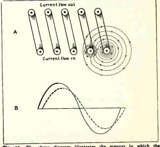
Fig. 16. The above diagram illustrates the manner in which the counter-voltage of self-induction is built up in an inductance coil. more and more until the current reaches maximum value. During this building up of the current and flux, the lines will be cutting across adjacent turns of the coil in the direction shown, and will be inducing a voltage in them.
