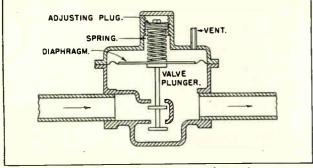
Fig. 18. Automatic pressure control gas valve.
