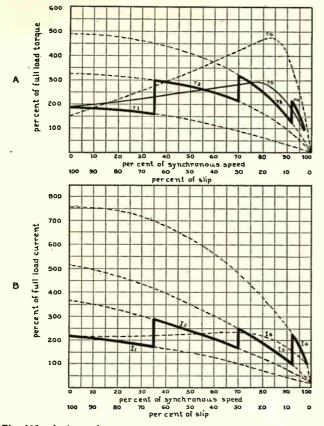
Fig. 185. A shows the torque curves of a slip-ring induction motor as the resistance is cut out of the rotor circuit and the motor comes up to speed. B shows the current curves of the same motor and corresponding to the various steps of the torque curves. Study these curves very carefully with the accompanying explanation.
