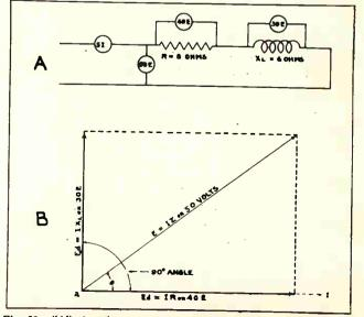
Fig. 22. "A". A resistance coil connected in series with an inductance coil in an A. C. circuit. "B". This sketh shows the method of determining the amount of impedance of the circuit shows at "A". plied would be in phase with the voltage. If the circuit had only inductance, the current which would then flow would be 90° out of phase with the voltage, or lagging 90° behind it.
