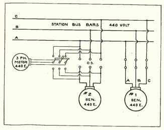
Fig. 94. The above sketch shows the connections and illustrates the metbod for phasing out an alternator by means of a three-phase motor.
