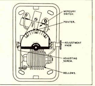
Fig. 7. Thermostat operated with bellows.
