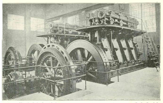
Fig. 306. Oil burning diesel engines of the above type are very commonly used as prime movers for generators in small and medium sized power plants. These engines are very economical in fuel cost and are simple and easy to operate and maintain. They are particularly desirable for use where coal and condensing water are difficult to obtain and where only limited space is available for a generating station.
