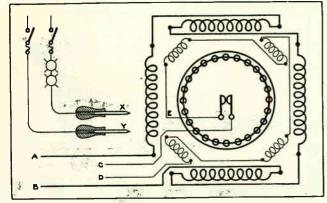
Fig. 467. Diagram illustrating connections and methods for convenient trouble tests on single-phase split-phase A. C. motors.
