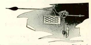
Fig. 46. Moving element of an iron-vane type meter. This view shows the shaft, iron vane, damping vane, pointer, and spring.
