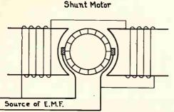
Fig. 110. Diagram of the connections for a simple shunt motor. 127. STALLING TORQUE OF SHUNT
