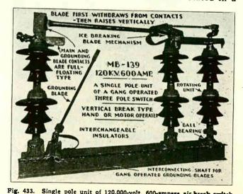
Fig. 433. Single pole unit of 120,000-volt, 600-ampere air-break switch with auxiliary grounding blade. Note the description of the various parts of this figure. (Courtesy of Delta-Star Manufacturing Company.)
