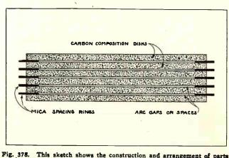
Fig. 375. This sketch shows the construction and arrangement of parts of an auto-valve lightning arrester. The discharge occurs in the abort gaps between the composition disks which are separated by insulating rings.
