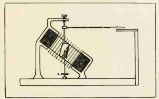
Fig. 47. The above diagram shows the construction and principle of the Thompson inclined-coil meter.
