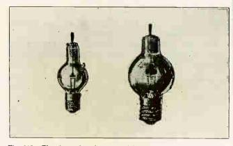
Fig. 228. The above view shows two different sized rectifier bulbs such as commonly used in battery chargers and other small rectifiers.
