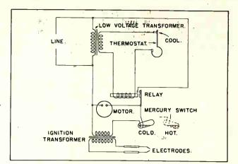
Fig. 13. Control system for an oil burner.
