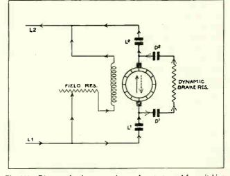
Fig. 142. Diagram showing connections and contacts used for switching a dynamic brake resistance across the armature of a D. C. motor when the line is disconnected.
