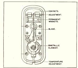
Fig. 1. The working parts of a room thermostat.
