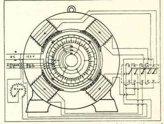
Fig. 260. Wiring diagram showing armature and field connections, and also the field break-up switch and rheostat for a four-pole, threephase converter. Trace out the field circuit both with the switch in the upper and lower positions and note that the polarity reverses when the switch is changed.
