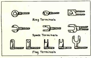
Fig. 147. Above are shown several types of terminals for brash shunts or leads.
