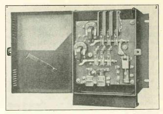
Fig. 274. Automatic controller which uses magnetically-operated contactors to cut the resistance out of the motor circuit in two steps. (Courtesy Cutler Hammer Mfg. Co.).
