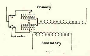
Fig. 136. This diagram shows a method of arranging adjustable connections on the primary of a tap-changing transformer.
