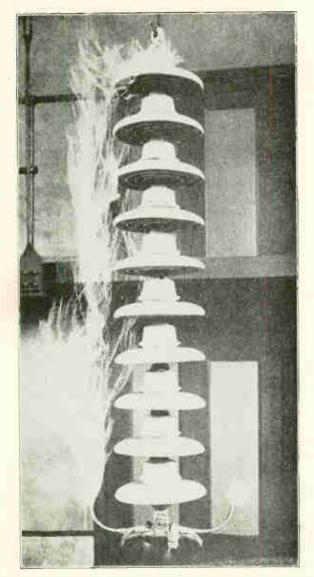
Fig. 341. This very interesting photograph shows an actual flashover or high-voltage arc on a string of 10 suspension insulator units. This flashover was made with 500,000 volts in a test laboratory, but similar flashovers occur on line insulators in service, due to lightning. (Courtesy Ohio Brass Co.)
