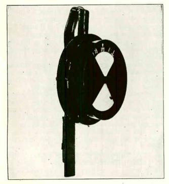
Fig. 112. This photo shows a temperature-indicating device for use with pole type transformers. This device is called a thermotel and indicates both excessive temperatures and overload of a transformer on which it may be installed.
