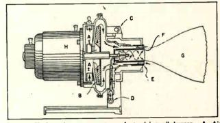
Fig. 11. Horizontal rotary cup type of atomizing oil burner. A. Air path. B. Fan. C. Hinged hanger for burner. D. Oil inlet. E. Air nozzle. F. Rotating automizing cup. G. Flame. H. Electric motor.
