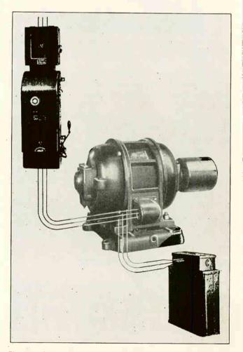
Fig. 218.—Static condensers can be connected direct to the terminals of individual induction motors as illustrated in the above view. The condenser then supplies the magnetizing current to the motor and corrects the lagging power factor at its source. (Courtesy G. E. Company)
