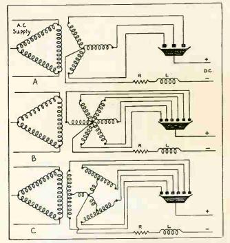
Fig. 245. The above diagrams show three different types of transformer connections which are commonly used with three-phase and six-phase mercury are rectifiers.
