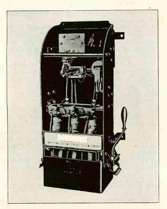
Fig. 282. This photo shows a front view of a three-phase, auto transformer starter or compensator used for starting squirrel-cage motors at reduced stator voltage. (Photo courtesy General Electric Co.).
