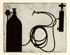
Fig. 39. This view shows the method of connecting a lead burning torch to the gas cylinder and piping, and also shows the mounting of the pressure regulating value on the gas cylinder.
