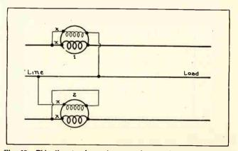
g. 37. This diagram shows the connections to the lower wattmeter reversed to obtain proper readings on circuits with low power factor. Fig. 37.
