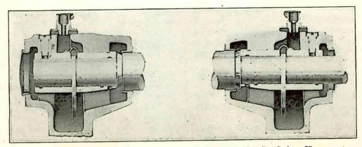
Fig. 453. Sectional views of two sleeve bearings, clearly showing the oil wells, oil rings, filler cups, etc.
