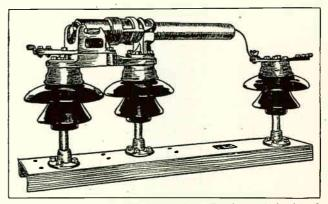
Fig. 435. Expulsion type high-voltage fuse. The fuse strip is violently blown out of the tube or barrel, thus quickly interrupting the circuit when this fuse blows. (Courtesy of Hi-Voltage Equipment Co.)
