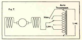
Fig. 7. Auto-transformer Speed Control for a Universal Motor Operated on Alternate Current.
