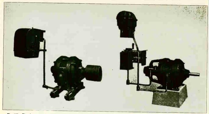
Fig. 300. The above two views show methods of connecting compensators and drum controllers to induction motors by means of rigid and flexible conduit. While in some temporary installations open wires which are properly supported and protected may do very well, in general a neat, permanent installation of the wires in conduit is a much safer and better arrangement.
