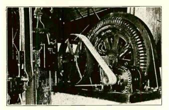
Fig. 192. 150-h. p., 2300-volt, low-speed, synchronous motor and exciter. The speed of the large motor is 144 RPM. (Photo courtesy Allis-Chalmers Mig. Co.)
