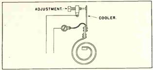
Fig. 3. Insulated spiral bimetallic element.
