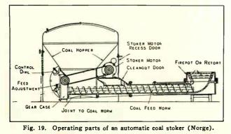
The underfeed stoker takes coal from a hopper or bin and carries it to the retort in the furnace by means of a large screw or by combinations of rams, plungers and screws. The coal-carrying device is driven by an electric motor through gearing or other drive elements which allow adjustment of the rate of feed.
