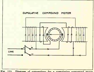
Fig. 113. Diagram of connections for a cumulative compound motor. Note that the series field winding is connected so it will aid the shunt field winding in providing a strong field. to lower the counter-E. M. F. sufficiently to allow enough current to flow to carry the load. The stronger the field of any motor, the lower will be the speed at which it can generate the normal counter-E. M. F.
