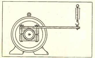
Fig. 115. The above diagram illustrates the method of making a brake-b. p. test on a motor.
