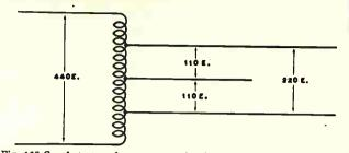
Fig. 138-C. Auto transformer connection for obtaining both 110 and 220 volts from a 440-volt line.
