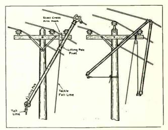
Fig. 369. The above diagrams show the use of live line tools to move live high-voltage conductors safely out of the way for replacing insulators or making other repairs. (Courtesy Johnson Mfg. Co.)
