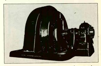
Fig. 212. 5000-kv-a., 2300-volt, enclosed-type, synchronous condenser. The exciter for this machine is shown on the right. (Photo courtesy G. E. Company)
