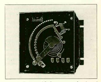
Fig. 125-A. Simple type of D. C. motor starter and speed control. Note the extra sets of contacts for the field resistance used in varying the speed.
