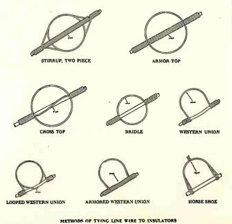
Fig. 335. The above sketches show the methods of making some of the most common types of line ties. Note carefully how the tie wires are wrapped around the insulator cap and around the conductor. (Courtesy Lapp Insulator Company, Inc.)
