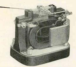
Fig. 59. This photo shows a meter element with part of the magnetic shield in place around it. These shields are made of soft-iron laminations and prevent magnetic flux from other machines or circuits from interfering with the accuracy of the meter. One-half of the shield is shown removed in this view.
