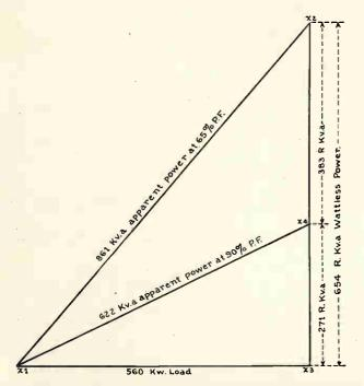
Fig. 221. This diagram also shows the reduction obtained in the apparent power and wattless power by improving the power factor of a system. By carefully measuring the top section of the vertical line in the diagram we can find the size of the condenser required to correct the power factor.
