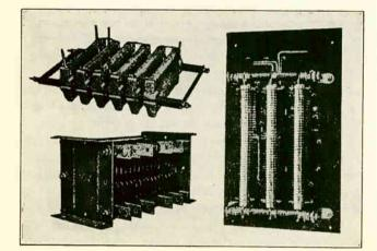
Fig. 271-A. This photo shows several types of resistance units used with A. C. motor starters. On the upper left are shown non-inductive, coil-wound resistors; on the lower left grid type resistors; and on the right edge-wound resistors made of strips of resistance metal wound edgewise around non-combustible cores.
