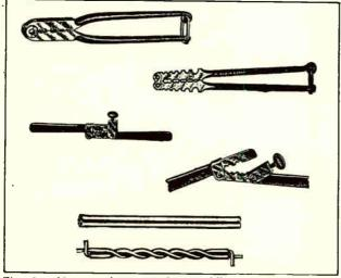
Fig. 361. Above are shown several styles of lineman's splicing clamps, and also a splicing sleeve and completed splice.
