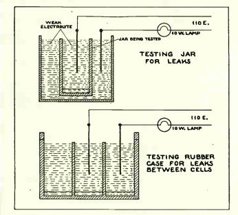
Fig. 33. The above two sketches illustrate the method of testing single cell jars or complete rubber battery cases for possible cracks or leaks.
