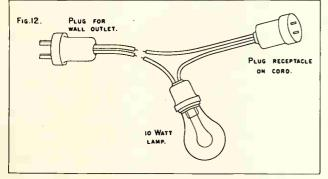
Fig. 12. Test Lamp and Plug Connectors.
