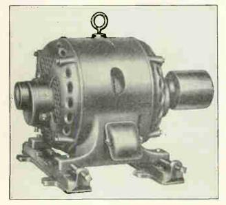
Fig. 105-A. This motor has a frame of the semi-enclosed type. The openings at the ends and around the frame are provided for air circulation and cooling.
