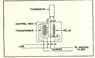
Fig. 8. Internal and external connections of control box with relay.
