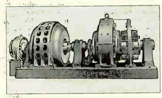
Fig. 406. 1000-kw. motor-generator set with an A. C. synchronous motor and exciter on the left. and the D. C. generator on the right. (Courtesy of Allis-Chalmers Mfg. Co.)
