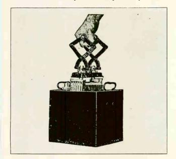
Fig. 36. This view shows a convenient type of cell puller used for lifting plate groups or elements from cell jars when taking down a battery for repairs.
