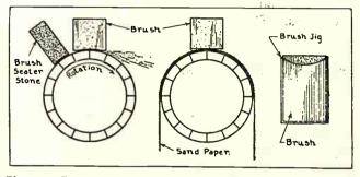
Fig. 149. The above sketches show several methods of cutting brush faces to fit the commutator surface. Each is explained in the accompanying paragraphs.
