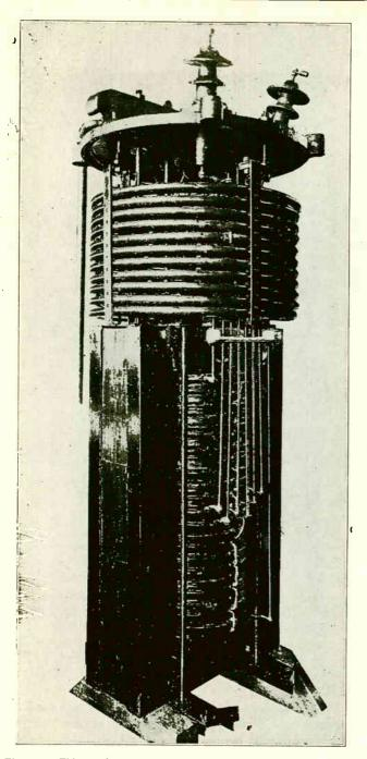
Fig. 110. This view shows a single-phase power transformer equipped with a coil of copper tubing through which water is circulated to cool the transformer and the oil which surrounds it.
