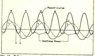
Fig. 13. Voltage, current, and power curves of a single-phase circuit in which the voltage and current are out of phase. The current, represented by the dotted curves, is shown lagging behind the voltage in this case.
