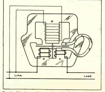
Fig. 65. This diagram illustrates the construction and principles of an induction watthour meter. Note the manner in which the current and potential coils are connected to the line.
