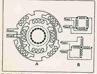
Fig. 175. A. This diagram shows the connections of the stator windings of a two-phase induction motor. At B are shown two schematic diagrams illustrating different methods of connecting two phase windings.
