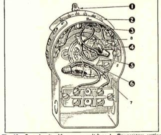
Fig. 17. Control unit with mercury switches: 1. Temperature setting pointer. 2. Temperature dial. 3. Lock screw. 4. Limit switch.
