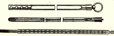
Fig. 156. Convenient thermometers of the above type are used for determining the temperature of the machine windings, by attaching the bulb to the windings with a small amount of putty.
