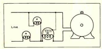
Fig. 31. This sketch shows the method of connecting the meters to measure voltage, current, and power of a single-phase motor.
