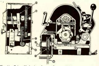
Fig. 11. Drive Mechanism for an Ironer (Kelvinator). 1. Shifter knob. 2. Shilter. 3. Jaw clutch. 4. Worm gear. 5. Worm.
