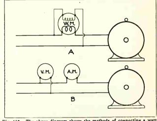
The above diagram shows the methods of connecting a watt-or voltmeter and ammeter, to determine the KW or h. p. Fig. 117. 01 input to a motor.
