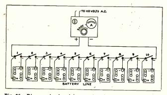
Fig. 26. Diagram showing the connections for charging up to ten batteries in series by means of a bulb type rectifier or the constant current system. Knife switches are used to close the circuit when a battery is removed from the line.
