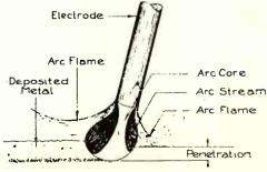
Fig. 1. Diagram of the welding arc.
