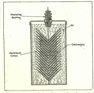
Fig. 386. The above sketch shows the construction and arrangement of parts of an electrolytic or aluminum cell arrester. Note the electrolyte between the aluminum cones and also the inlulating oil surrounding them.
