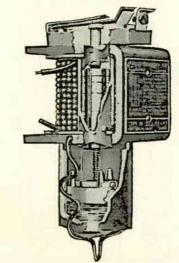
Fig. 280. Sectional view of a magnetic overload-relay and dash pot. When the core is lifted the rod above it forces open the spring contacts which break the circuit to the holding magnet. (Courtesy Allen Bradley Co.).
