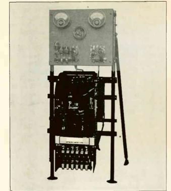
Fig. 283. This photo shows another view of a compensator with both the front cover and the oil tank removed. The contacts which operate under oil can be seen at the bottom of the controller. (Courtesy General Electric Co.).
