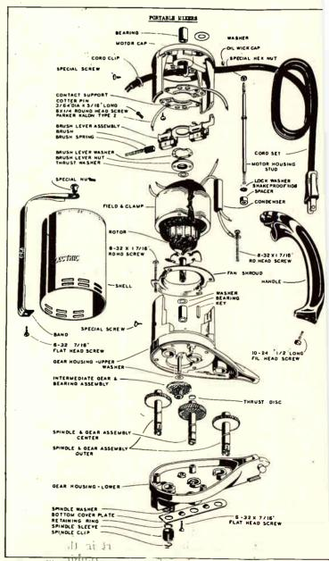
Fig. I. The Parts of an Electric Food Mixer (General Electric).
