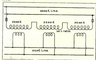
Fig. 123. Transformer primaries are sometimes connected in series to a line of higher voltage as shown above. The secondaries can then be connected for parallel operation.
