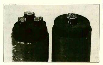
Fig. 325. These views show sections of high-voltage three conductor and single conductor, underground transmission cables. Note the arrangement of conductors and insulation inside of the lead sheath. (Courtesy General Electric Co.)
