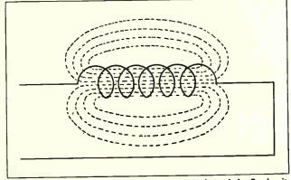
Fig. 15. The alternating flux around colls or wires of A. C. circuits produces voltage of self-induction and inductive reactance in the circuits.
