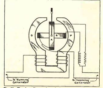
Fig. 75. The above diagram shows the important parts and illustrates the principles of a synchroscope. This diagram also shows the connections of the colls to the "running" and "incoming" generators.
