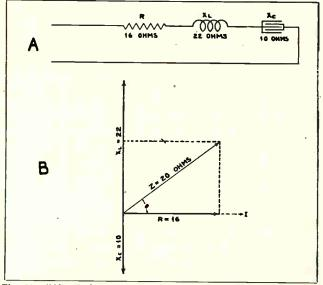
Fig. 24. "A". Resistance, inductance, and capacity connected in series in an A. C. circuit. "B". Note how the capacity reactance is subtracted from the inductive reactance, as the two neutralise each other in the circuit.
