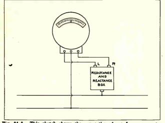
Fig. 74-A. This sketch shows the connections for a frequency meter and the resistance and reactance box which is used with the meter.
