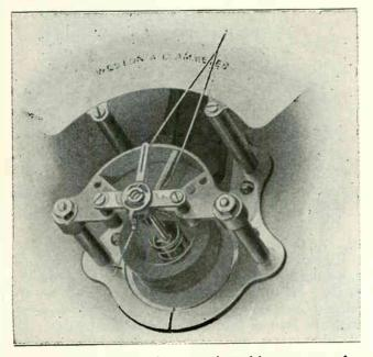
Fig. 45. This photo shows the construction and important parts of an iron-vane meter. Note the position and shaps of the iron vanes within the coil and also note the damping vane and chamber above the coil.
