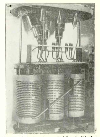
Fig. 113. This view shows the core and windings of a high voltage, three-phase transformer and also the lower ends of the insulating bushings through which the high voltage and low voltage leads are taken from the tank.
