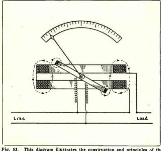
Fig. 53. This diagram illustrates the construction and principles of the dynamometer type instrument. Note the action between the flux of the moving and stationary coils.
