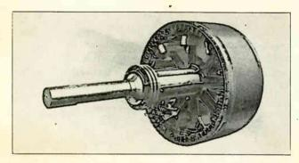
Fig. 181-A. Phase wound rotor of a large slip-ring induction motor. This rotor has heavy bar windings which are not shorted together like those of a squirrel-cage rotor, but instead have connections brought out from each phase to the slip rings.
