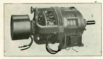
Fig. 204. This photo shows the completely assembled BTA motor. The brush-shifting wheel can be seen on the upper corner of the frame and the slip rings are enclosed in the housing at the left end of the shaft. (Courtesy G. E. Company)
