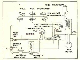
Fig. 16. Complete automatic control system for gas burning plant.
