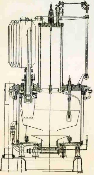
Section through Brown Boveri mercury-arc power rectifier.
