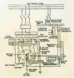
Fig. 246. Wiring diagram of a six-phase rectifier showing transformer connections and auxiliary control circuits. (Courtesy American Browa Boveri Co.).
