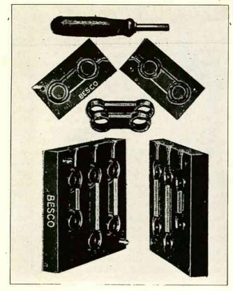
Fig. 44. Above are shown two types of strap or connector molds for molding lead straps of different lengths to be used in connecting together the separate cells of automotive batteries.
