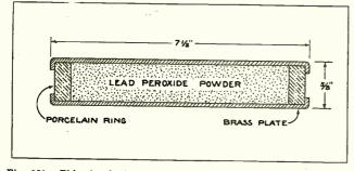
Fig. 382. This sketch shows the construction of one disk or unit of an oxide film lightning arrester.
