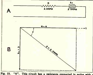
Fig. 23. "A". This circuit has a resistance connected in series with a condenser. "B". The vector diagram shows the method of determining the impedance and angle of lead between the current and voltage for a circuit such as shown at "A".
