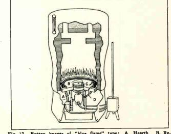
Fig. 12. Rotary burner of "blue flame" type: A. Hearth. B. Revolving tubes. C. Igniter. D. Refractory lining.
