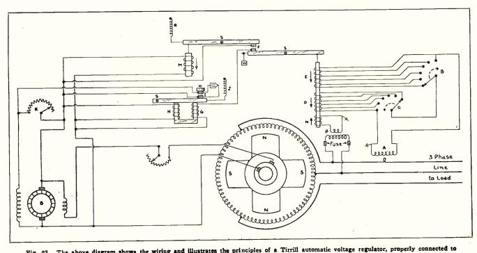
Fig. 92. The above diagram shows the wiring and illustrates the principles of a Tirrill automatic voltage regulator, properly connected to the exciter and line leads of a three-phase alternator.
