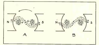
Fig. 141. The above sketch illustrates the principle of dynamic brake action in a motor when its armature is short circuited.
