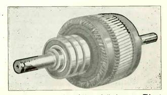
Fig. 181. Wound rotor of a variable speed slip-ring motor. This rotor has windings of insulated copper wire similar to those in D. C. armatures. induced currents to flow from the rotor winding to a control resistance in the external circuit. By varying this resistance the secondary current flow in the rotor can be varied; and this will increase or decrease the amount of torque and slip, and thus vary the speed of the motor.
