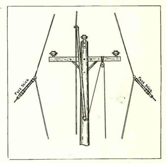
Fig. 370. This view shows the method of using a live line tool known as a "jew claw" to raise the center conductor; and two other tools known as "fuzz sticks" to draw aside the outer conductors and thereby allow a lineman to work safely on any of the three insulators on the pole and cross arm. (Courtesy Johnson Mfg. Co.)
