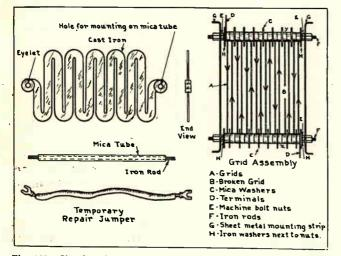
Fig. 460. Sketches showing construction of iron grid type secondary resistors for slip-ring motors. Also note the jumper used for making temporary repairs to open circuited units.
