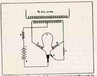
Fig. 238. Circuit diagram of a bulb type mercury arc rectifier used for battery charging purposes. Trace this circuit carefully with the acc.mpanying explanation.
