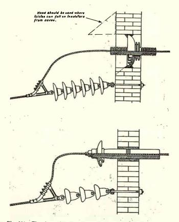
Fig. 344. The above diagrams show methods of using strain insulators to attach line conductors to the walls of substation buildings and keep the strain from the conductor where it enters the building through wall type insulator bushings. (Courtesy Ohio Brass Co.)
