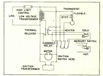
Fig. 14. Control system with safety features.
