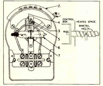
Fig. 6. The bimetallic helix used as a thermostat in bonnets, ducts and stacks: 1. Temperature indicator. 2. Temperature dial.
