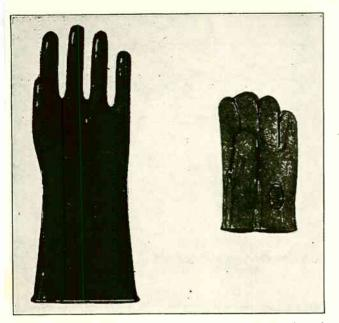
Fig. 367. On the left is shown a lineman's rubber glove and on the right a soft leather protector glove to prevent mechanical injury of puncture of the rubber insulating glove.
