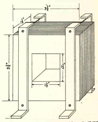
Fig. 153-C. A 50 w. transformer core constructed from strips 1"x23/2". Note the method of binding the strips together.
