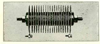
Fig. 233. Single unit of a copper oxide rectifier, consisting of a number of copper disks coated with copper oxide and clamped into one series group. Current can only pass through these devices in one direction. (Courtesy of Westinghouse Elec. & Mfg. Co.).
