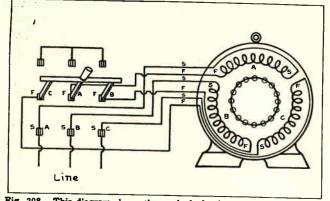
Fig. 298. This diagram shows the method of using a three-pole, doublethrow switch for star-delta starting of squirrel-cage induction motors. gether to form the Y or star connection for starting.
