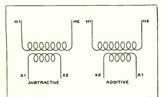
Fig. 117. This sketch shows winhings of two transformers with their leads properly marked for subtractive and additive polarities.
