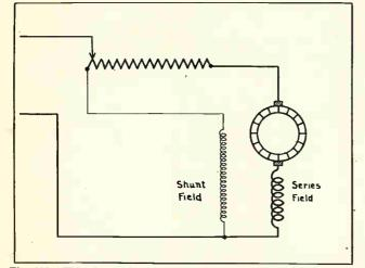
Fig. 118. This simple sketch shows the manner in which a resistance is used in series with the armature when starting a D. C. motor.
