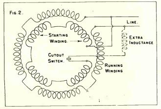
Fig. 2. Connections in a Split-phase Motor.
