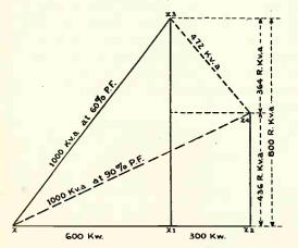
Fig. 222. This diagram shows the graphic solution of a problem in which the synchronous motor is used for mechanical power purposes as well as power factor correction. The figure should be easily understood by referring to the explanations in the accompanying paragraphs.
