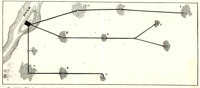
Fig. 322-A. This diagram shows the location of a central station power plant and the layout of a transmission system. The power plant is located at the river where fuel and condensing water are easily available and the transmission lines feed the generated energy to substations located in the various towns.
