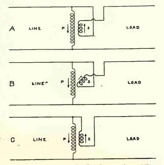
Fig. 140. The above three sketches show the connections and illustrate the principle of an induction voltage regulator. Study carefully each of the three diagrams while reading the explanations given on these pages. mum induced voltage from the primary, and this voltage is in a direction to add to the primary voltage in series and thereby increase the line voltage.
