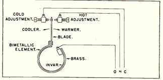
Fig. 2. The bimetallic element and contacts.
