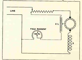
Fig. 119. This diagram shows the armature starting resistance and also a shunt field rheestat for varying the speed of the motor.
