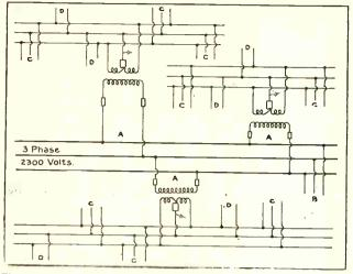
Fig. 397. Sing'e-phase transformers with their primaries properly connected to balance the load on a three-phase distribution line, and their secondaries connected to supply three-wire Edison service to customers. At "B" is shown a connection for three-phase motor service directly from the distribution line.
