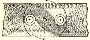
Fig. 107. The above diagram illustrates the manner in which the reaction between the lines of force from the armature and field windings set up the torque or turning effort in a motor.
