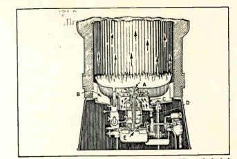
Fig. 10. Rotary centrifugal atomizing oil burner with vertical shaft: A. Atomizer. B. Chamber lines with refractory material. C. Air space. D. Electric motor. E. Hollow shaft.
