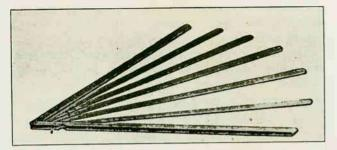
Fig. 459. Common motor air gap gauge, for measuring clearance between the armature or rotor and the field poles or stator. Note the several different "fcelers" or blades which are of different thicknesses.
