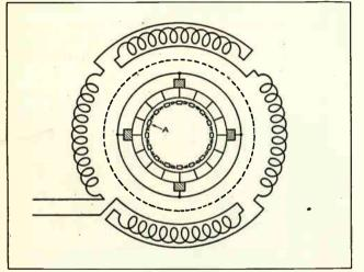
Fig. 172. This diagram shows the connections and arrangement of the short-circuiting device of a repulsion-induction motor. The shortcircuiting mechanism at "A" lays around the inside of the commutator bars and short-circuits them all together when the machine comes up to speed.
