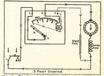
Fig. 121. This diagram shows the connections for a simple 3-point D. C. motor starter. Trace the circuit carefully with the accompanying instructions. to apply the line voltage to the controller and motor.
