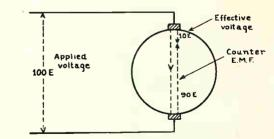
Fig. 109. From the above illustration you will note that the countervoltage is often nearly as high as the applied voltage. This sketch illustrates the extent to which counter-voltage regulates or limits the flow through a motor armature.
