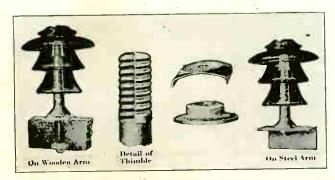
Fig. 332. Above are shown the methods of mounting insulators on pins and attaching the pins to wood and metal cross arms, and also the soft lead thimble which enables the insulator to be securely tightened on the pin without damaging the threads in the porcelain. (Courtesy of Ohio Brass Company.)
