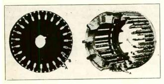
Fig. 199. This figure shows two views of a double squirrel-cage rotor. On the left is a sectional view and on the right the core iron has been eaten out by acid, clearly showing the construction and shape of the double squirrel-cage. (Photo courtesy General Electric Co.)
