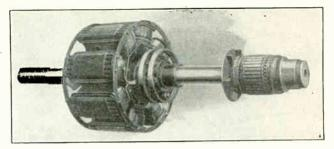
Fig. 81. This view shows the construction of the rotor or revolving field of an alternator similar to the one shown in Fig. 80. Examine its construction carefully and note the position of the collector rings and exciter-armature on the shaft.
