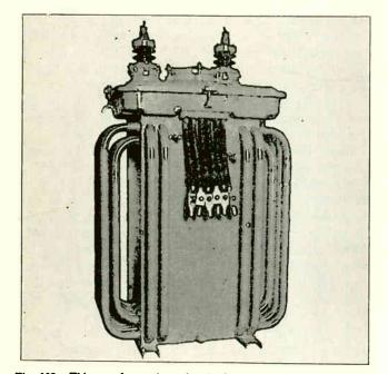
Fig. 108. This transformer is equipped with cooling tubes to allow the oil to circulate outside of the tank and give off its heat more rapidly to air.
