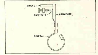
Fig. 4. Permanent magnet for producing snap action as contacts open.
