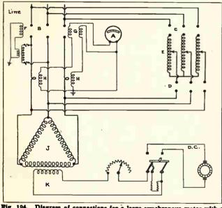
Fig. 194. Diagram of connections for a large synchronous motor with a compensator for starting at reduced voltage. Also note the protective device connected with a circuit-breaker in the line leads.
