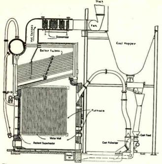
Fig. 308. Diagram of a modern power plant boiler using pulverized coal for fuel. Note the coal hopper, pulverizer, furnace feed tube, and also the economizer which is located above the boiler.
