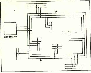
Fig. 395. This sketch illustrates the loop method of connection for distribution systems.
