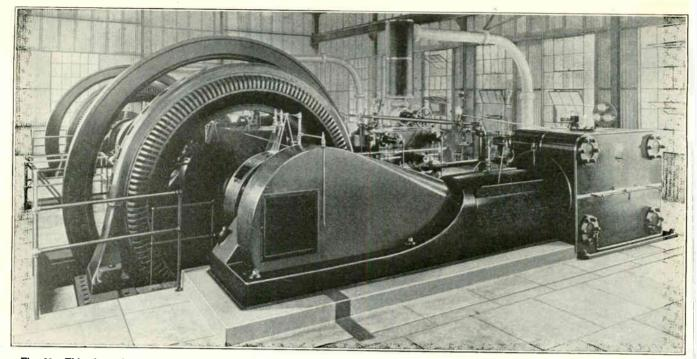
Fig. 83. This photo shows a view in a power plant equipped with horizontal type steam-engine-driven alternators. These alternators are made with large diameters because of the relatively low speed at which they are driven. (Poto Courtesy Allis Chalmers Mfg. Co.)
