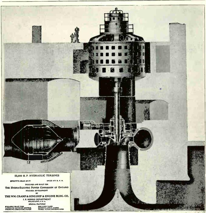
Fig. 318. Excellent sectional view of a large hydro-electric generator unit. Note the casing and runner of the water wheel and also the draft tube through which the water discharges to the tail race. The valve controlling the water flow through the wheel or turbine is shown on the left. The main part of the generator is set down in the concrete so that just the top of the unit and its exciter project above the operating floor. (Courtesy Wm. Cramp & Sons Co.)
