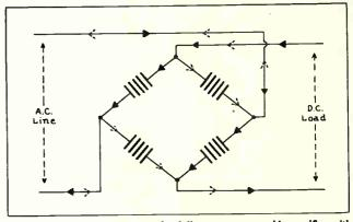
Fig. 235. Connection diagram of a full-wave, copper oxide rectifier with four units connected in a "bridge" type circuit.
