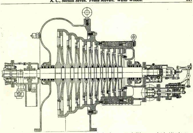
g. 315. An excellent sectional view of a modern steam turbine showing how the steam enters the high pressure end at the right and passes through one set of blades after another as it expands toward the exhaust end on the left. The stationary blades redirect the steam to apply its force against each successive ring of movable blades. (Courtesy of Elliott Company.) Fig. 315.
