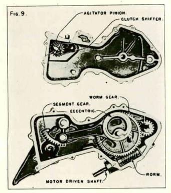
Fig. 9. Gears and Gear Case for a Clothes Washer (Easy).
