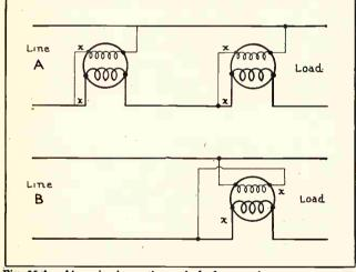
Fig. 35-A. Above is shown the method of connecting wattmeters to a single-phase circuit to locate the proper terminals of the potential and current coils. Fig. 35-B. This sketch illustrates the method of reversing the leads to the potential coil if necessary, to make the meter read properly.
