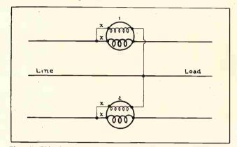
. This sketch shows the connections for using two single-phase wattmeters to measure the power in a three-phase circuit. Fig. 36.
