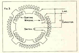
Fig. 3. . Connections in a Capacitor-start Motor.
