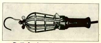
Fig. 473. Convenient trouble lamp with hook, guard, and insulating handle.
