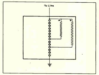
Fig. 377. The above sketch shows the arrangement and connection of parts for a simple series-gap graded-shunt lightning arrester.
