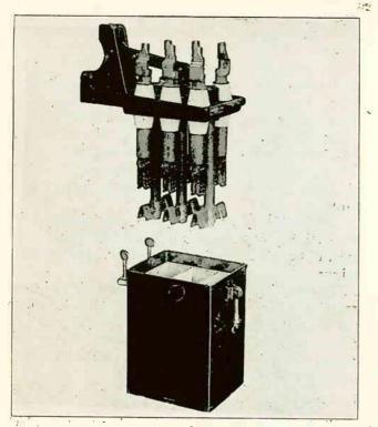
Fig. 422. View of a three-pole, 3300-volt, 200-ampere oil switch with oil tank removed to show contacts. (Courtesy of G. E. Company.)
