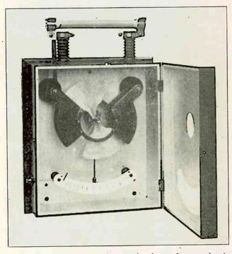
Fig. 63. This photo shows an electro-static voltmeter for measuring the potential of high voltage circuits. The pointer movement is obtained by the attraction between the moving and stationary metal vanes when they are charged with opposite polarity.
