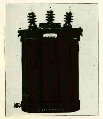
Fig. 107. Three-phase power transformer for high voltage operation. Note the large insulating bushings and also note the manner in which the entire tank is corrugated to provide a greater heatradiating surface.
