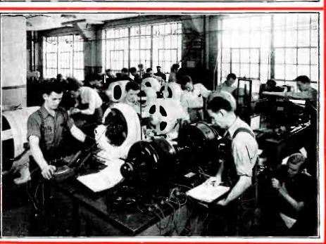
Upper view shows student receiving personal instruction on D. C. meters. Lower view, these men are making generator voltage tests and horse-power and efficiency tests on D. C. motor generators.
