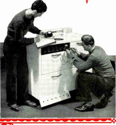
Here are some of the motors the students wire and test in this department. This actual work teaches them how motors and starters must be wired according to the code, and how to test to locate troubles in the wiring, which might cause motors to fail to operate. And it gives them still more practice in the use of tools.
