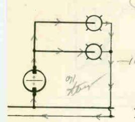
A single-pole switch used to control two lights in parallel.
