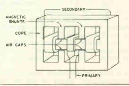
Sign Transformer Having High Leakage Reactance, Showing the Magnetic Shunts Between Winding Sections. Fig.13
