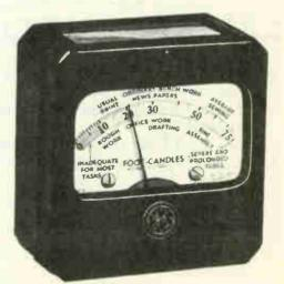
This G-E Light Meter closely resembles a small thin desk clock. It is  $2\frac{1}{4}$  inches square and  $1\frac{1}{8}$ inches thick and can be carried in the vest pocket. The normal scale range of the meter is from 0 to 75 footcandles but each meter is provided with a multiplying shield so that illumination values up to 750 footcandles can be read.
