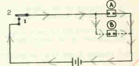
Open circuit switch used to control 2 bells in parallel
