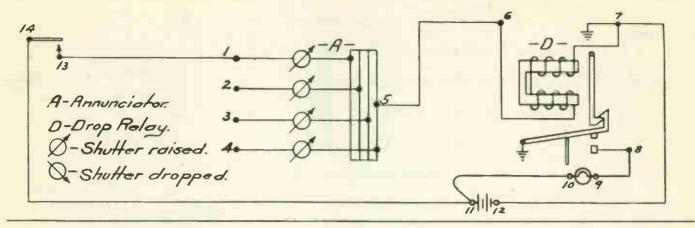
To Find Common Terminal of Annunciator, With Test Leads.
