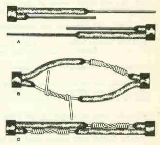
Fig. 4 When making splices in pairs of conductors they should be staggered as shown above so each splice will be close to good insulation on the other wire. Job No. 3
