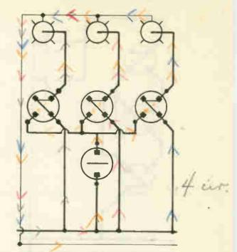
FIG. B This shows 3 lights, each one individually controlled from one place, using a three-way switch as a single-nole switch. The one single-pole switch is used as a master switch When the master switch is on; the other lights cannot be turned off.
