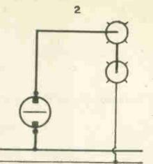
A single-pole switch used to control two lights in series. 5
