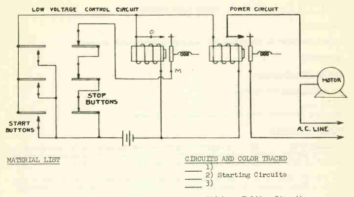
Stick or Holding Circuit Power or Motor Circuit
