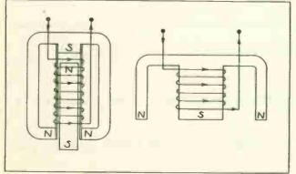
Fig. 10. Plunger type magnet at left. Shell type magnet at right.
