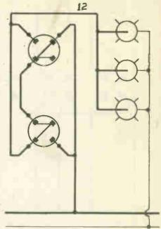
This is the "Carthweise" method used to control lights from 2 places, using two 3-way switches. This system is not approved by the Code for 110E systems, but may be used on 32E systems.
