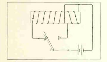
Fig. 12 Electrc magnet with demagnetizing coil for destroying residual magnetism.
