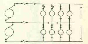
Fig. 4 An unbalanced 3-wire system with an open neutral.
