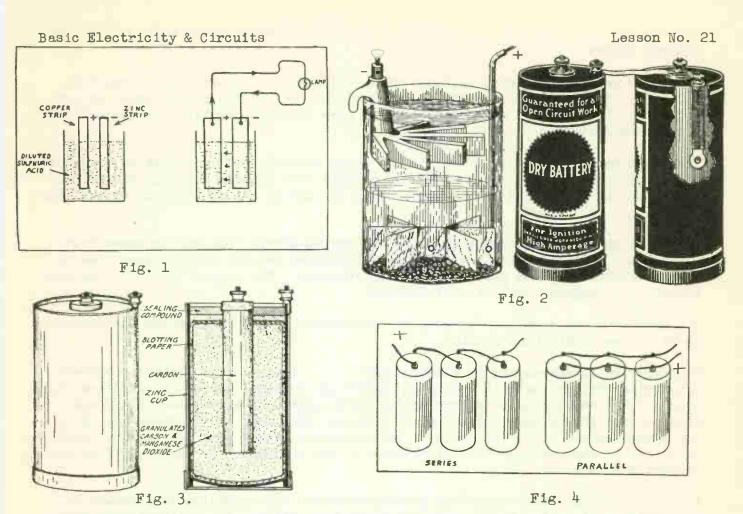
A bichromate cell is a cell having an electrolyte consisting of a solution of sulphuric acid and a bichromate.
