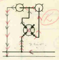
A 4-way switch used to control one light only, or 2 lights in .series.
