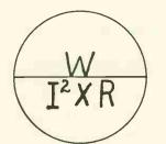
Fig. 3. Simplified formula for use when voltage is unknown.
