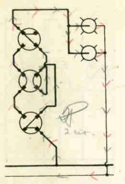
FIG. A Method used to control one or more lights from three places.
