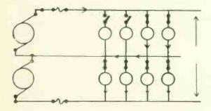
Fig. 3 an unbalanced 3-wire system with a solid neutral.
