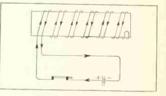
Fig. 13 Non-magnetic winding. One half of the turns oppose the other half, so the core does not become magnetized.
