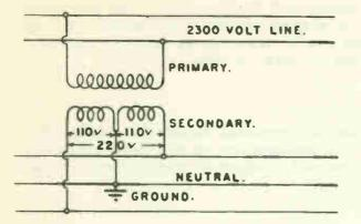
Fig. 1A a 3-wire AC system Fig 1B A 3-wire DC system
