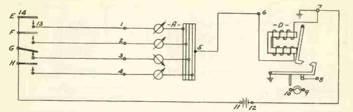
The circuit through battery, relay and annunciator has been completed through the movable contact at signal station G when the annunciator shutter \*3 indicating the station falls and relay trips.
