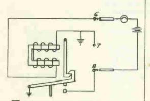
Test leads from 6 to 8. Lamp does not light, Relay does not trip.
