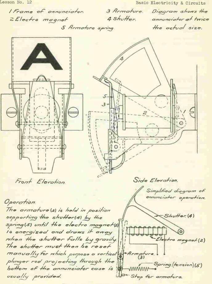
Fig. 1 Gravity drop type annunciator Coyne Electrical School
