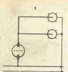
A single-pole switch used to control two lights in parallel. 4
