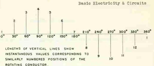
These values are based on the assumption that the conductor moves at constant angular velocity thru a magnetic field of uniform strength.
