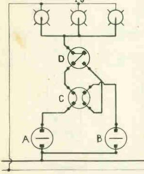
By means of 2 single-pole switches at A and B, it is possible to prevent turning the lights on or off at switches C and D. When switches A and B are closed, the lamps cannot be turned off. When switch A is on and B is off, the lamps may be controlled from switches C and D.
