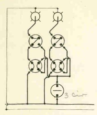
FIG. A When the single-pole switch is open, each of the 2 lights may be controlled from 2 places. When the singlepole switch is closed, all the lamps will remain lighted regardless of the position of the other switches.
