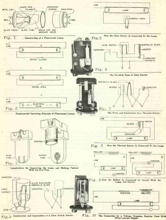
2. Construction and Operation of Ballast - a. A coil having many turns wound on an iron core has high inductance. When current has been flowing in such a coil and suddenly is stopped the magnetic lines of force which have existed around the windings collapse and cut back through the turns. This cutting of the conductor by lines of force induces a voltage which is much higher than that which was sending current through the coil. It is commonly referred to as "inductive kick".
