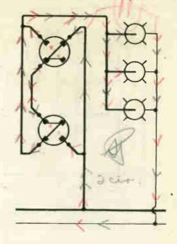
FIG. B This shows another method of controlling lights from 2 places.
