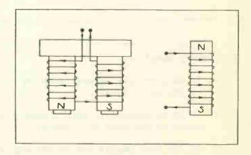
Fig. 11 Double and single electro-magnets.
