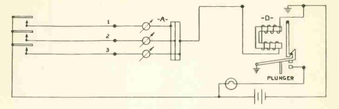
Fig. 6 This is an alarm or signal system using an annunciator A and a drop relay D (drop switch) to provide a continuous alarm until the relay is reset by hand.
