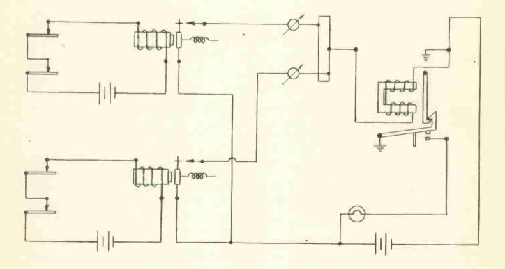
Fig. 7 This is a two-section alarm or signal system. Two or more floors, buildings, or departments can be protected in this manner. The annunciator indicates which floor or building the call comes from and the drop relay gives a continuous indication after the system has been disturbed. A bell can be used in place of the lamp if an audible signal is desired.
