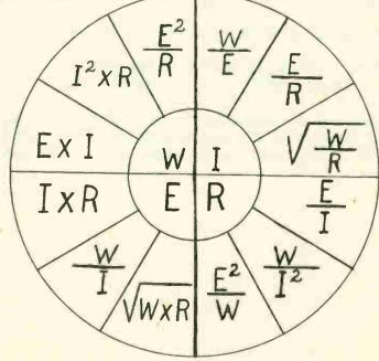
Fig. 5. "WIRE" Wheel. Any of the four values shown in the center--W, I, R, or E, can be found in three different methods, according to which values are known.
