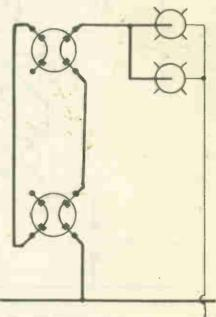
This diagram shows how to control each light alternately from three different places. Possible circuit used to control two lights in parallel from two places using two 4-way switches.
