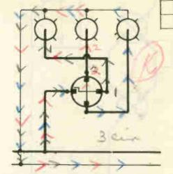
Electrolier switch used to control three separate lights from one place.
