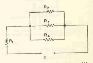
R1 is connected in series with the network TRUE FALSE
