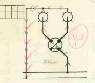
A 3-way switch used to control.2 lights alternately. One or the other will be lighted.
