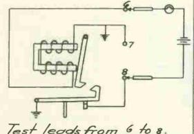
Test leads from 6 to 8. Lamp lights dimly. Relay must be reset manually.
