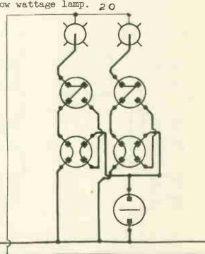
When the single-pole switch is open, each of the 2 lights may be controlled from 2 places. When the singlepole switch is closed, all the lamps will remain lighted regardless of the position of the other switches.
