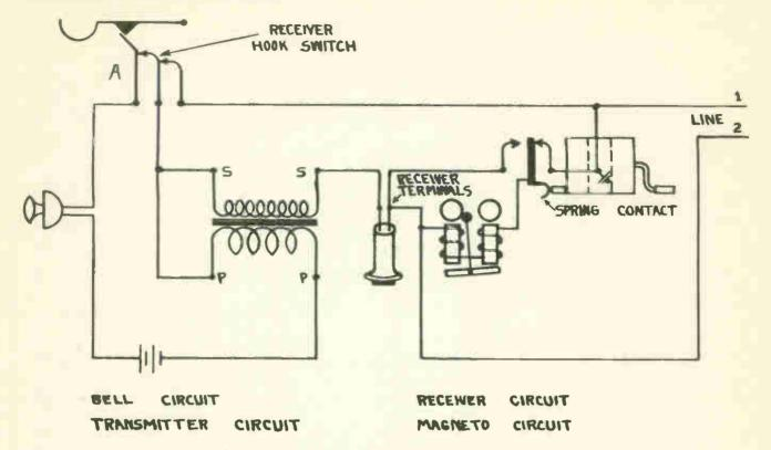
Fig. 1 Local battery type telephone - silent ringing.
