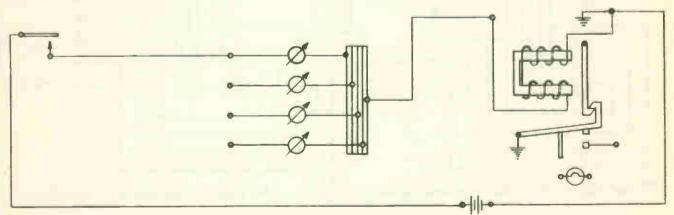
Required wiring connections to battery, annunciator and relay so that station signaling is recorded and relay tripped. For wiring of worning lamp or bell signal eqipment see following sheet.
