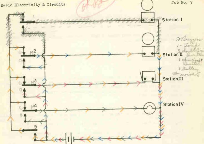
Fig. 1 This selective station call system shows the use of various switches with switch 1 to 4 inclusive calling the corresponding station, while switch 5 calls all stations.
