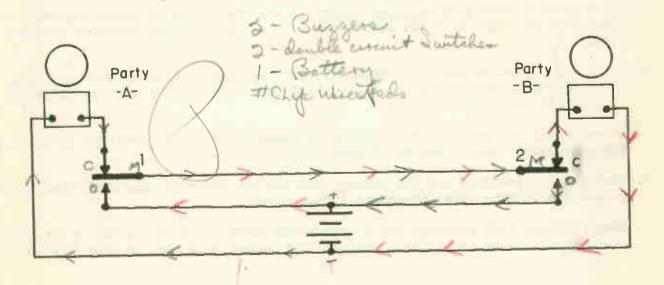
Fig. 2 A return call system using double circuit switches connected so that switch #1 calls party B and switch #2 calls party A.
