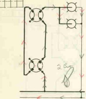
FIG. A Possible circuit used to control two lights in parallel from two places using two 4-way switches.
