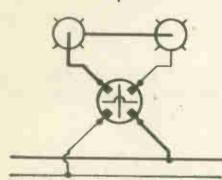
A double-pole switch used to control two lights in series.
