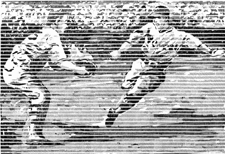
Fig. 114-1.—A picture image is divided into many horizontal lines by scanning.
