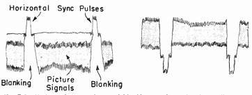
Fig. 7-2.—Horizontol sync pulses and blanking as shown by the oscilloscope.
