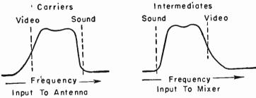
Fig. 8-4.—Where carrier frequencies and intermediate frequencies appear on the frequency response from the video detector.
