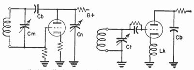
Fig. 95-2.-Circuits connections for modified Colpitts oscillators.
