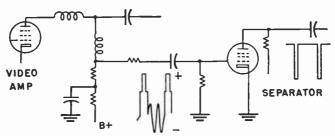
Fig. 116-3.—Sync separator connected to output of a video amplifier.
