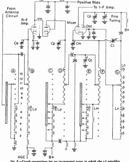
Fig. 9.—Circuit connections for an incremental tuner in which the r-f amplifier is a cascode type, with a pentode-triode for mixer and oscillator.
