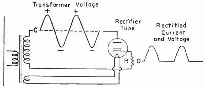
Fig. 110-1.—How alternating voltage causes ane-way current in a half-wave rectifier employing a vacuum tube.
