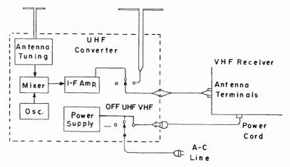
Fig. 138-5.—Circuit orrongements in o uhf converter used os on ottochment to o vhf television receiver.
