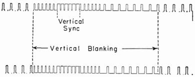
Fig. 118-4.—Sync pulses of the several kinds occurring during vertical blanking periods.
