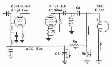
Fig. 43-2.—Circuits for a simple type of automatic gain control.
