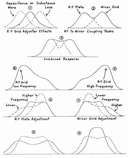
Fig. 21.—Frequency responses which may be observed during r-f olignment
