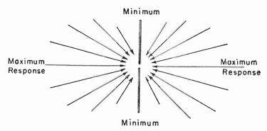
Fig. 9-3.—Directional properties of a simple half-wave dipole antenna.
