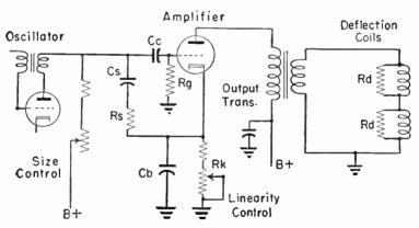
Fig. 5-12.—Typical vertical sweep circuit for magnetic deflection.
