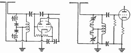
Fig. 63-4.—Trops in r-f grid circuits and ontenno couplings for 300-ohm bolonced tronsmission line.
