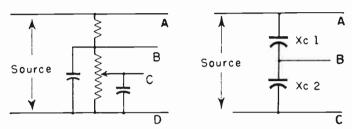
Fig. 32-1.—A resistance voltage divider (left) and a capacitance voltage divider (right).
