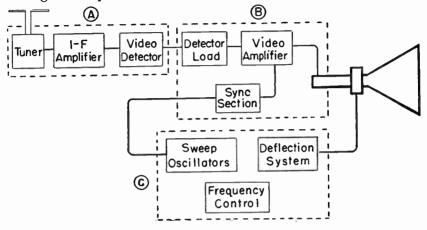
Fig. 99-9.—Woveforms, frequency responses, or both, may be observed from these sections of a television receiver.
