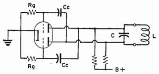
Fig. 95-3.—Push-pull r-f oscillotor with porollel resonant tuned circuit.
