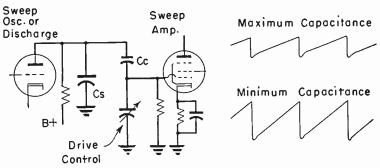
Fig. 34-2.—Capacitor type drive control and its action.
