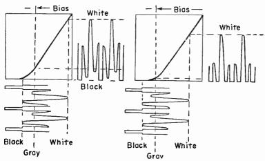
Fig. 11-5.—Left: Brightness and contrast correct for a strong signal.
