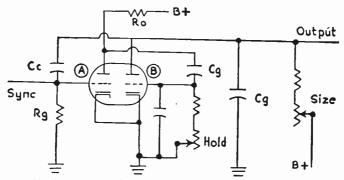
Fig. 96-8.—A capacitor-coupled multivibrator sweep oscillator.
