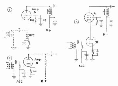
Fig. 137-19.—The principle of the cascode amplifier having the two triodes in series for d-c plate-cathode current.
