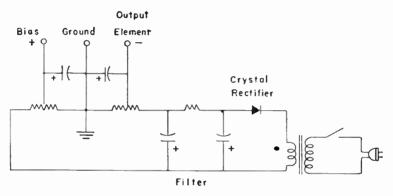
Fig. 17.—The circuit of the d-c power supply used with transistors.
