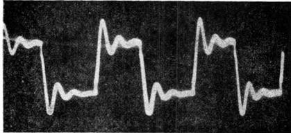
Fig. 99-4.—A square wave valtage is seen to be accompanied by damped ascillation.
