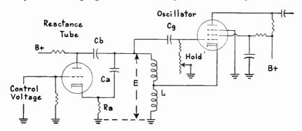
Fig. 2.—The reactance tube controls oscillator frequency by means of a variable capacitive effect.
