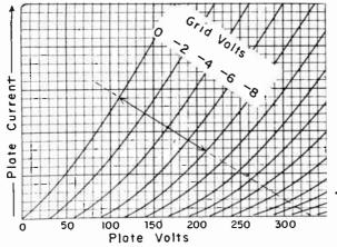
Fig. 44-1.—On the plate and plate load there is change of 100 volts for 8 volts change on the grid, indicating a gain of 12½ times.
