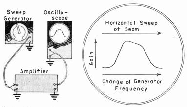
Fig. 51-1.—Connections for a sweep generator and features of the ascillascope trace.
