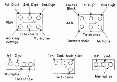
Fig. 12-2.—Meanings of color code dats in various positions on mico capacitors.
