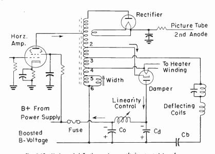
Fig. 5-20.—Horizontal deflection system employing an autotransformer.
