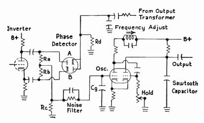
Fig. 97-2.—Phase detector for direct frequency control of a multivibrator oscillator.
