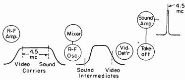
Fig. 8-23.—Frequency responses with an intercarrier sound system.
