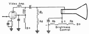
Fig. 11-2.—Brightness control used when signal input is to the picture tube control grid.
