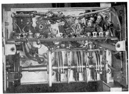
Fig. 17.—Channel selection is by means of three continuously variable oir-dielectric capacitors.
