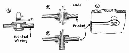
Fig. 2.—Methods of making terminal connections to printed wiring.
