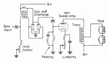
Fig. 5-22.—An autotransformer in a vertical sweep system.
