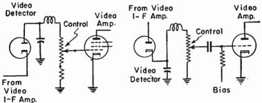
Fig. 18-2.—Controst controls on grid input of video omplifier tubes.
