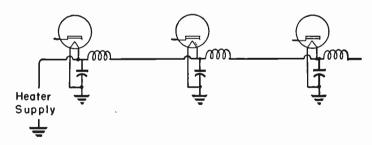
Fig. 8-20.—Decoupling capacitors and chokes in a heater circuit.
