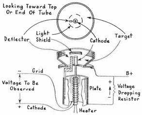
Fig. 1.—The elements in an electron-ray tube.
