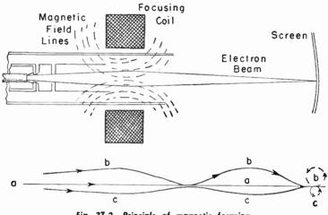
Fig. 37-2.—Principle of magnetic focusing.
