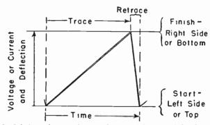
Fig. 69-1.—Relations of sawtooth wave slopes to deflections of the electron beam.
