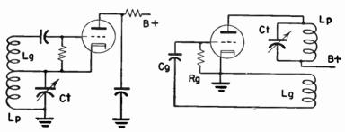
Fig. 91-6.—Tuned plate oscillators with tickler feedbacks.
