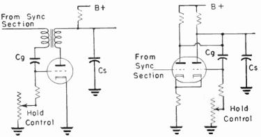
Fig. 55-2.—Hold control connected to a blocking oscillator.
