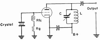
Fig. 46-1.—A simple crystal-controlled oscillator.
