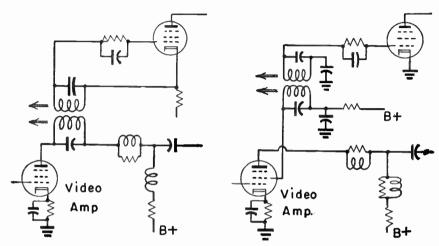
Fig. 62-2.—Intercarrier sound tokeoffs consisting of double-tuned transformers.
