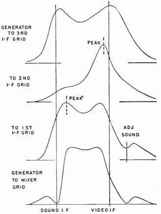
Fig. 128-6.—Frequency responses of various points in the i-f amplifier having trops for occompanying and adjacent sound.
