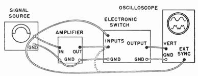
Fig. 121-3.—Electronic switch connected for observing input and output voltages of an amplifier.
