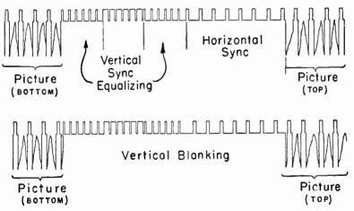
Fig. 118-3.—The television signal during the two vertical blanking periods of one frame.
