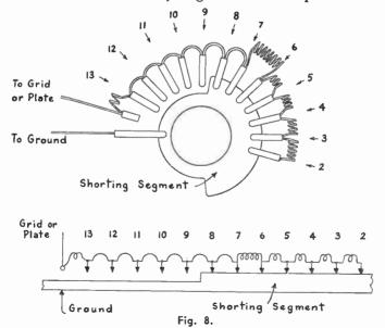
ductor sections on a switch wafer that has a shorting segment
