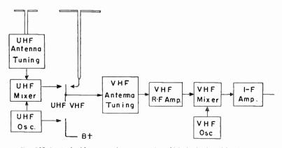
Fig. 138-4.—A double conversion system in which both the uhf mixer and vhf mixer remain in operation for uhf reception.
