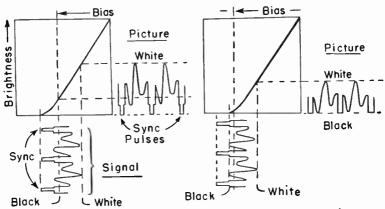
Fig. 11-4.—Left: Brightness control too high or contrast control too low.
