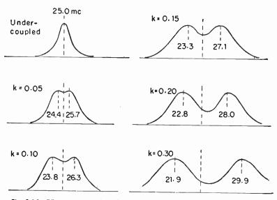
Fig. 8-14.—Effect on separation of resonance peaks when coupling is increased.
