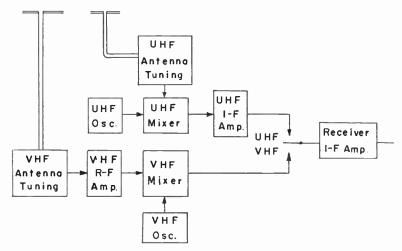
Fig. 138-2.—Tuner circuits in which there is no r-f omplifier for uhf signals.
