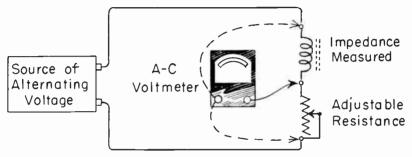
Fig. 56-1.—Measuring impedance with a voltmeter and adjustable resistance.
