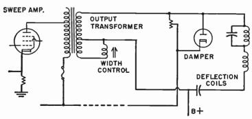
Fig. 119-2.—Width control inductor in porollel with port of the secondary on the horizontal autput transformer.
