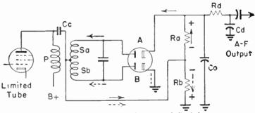
Fig. 31-1.—A typical circuit for a sound discriminator.
