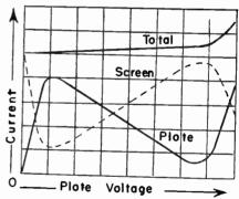
Fig. 93-2.—Currents in a dynatron oscillator tube.
