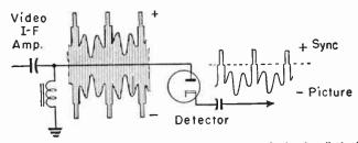
Fig. 7-9.—Sync pulses are positive in the output from the cathode of a diode detector.
