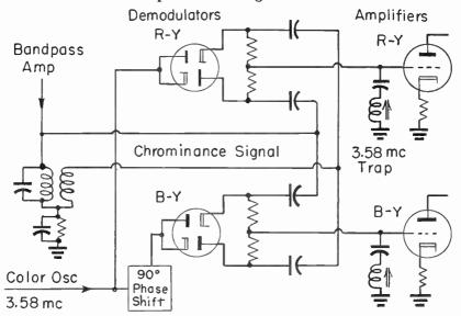
Fig. 15.—Twin-diodes used as R-Y and B-Y demodulators.
