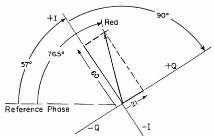
Fig. 13.—How the red color phase results from combining certain praportions of I- and Q-signals.
