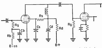
Fig. 23-3.—Separate decoupling for plate, screen, and grid circuits.
