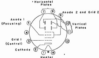
Fig. 7.—Bosing connections for a type 7.1P4 picture tube using electrostatic deflection.
