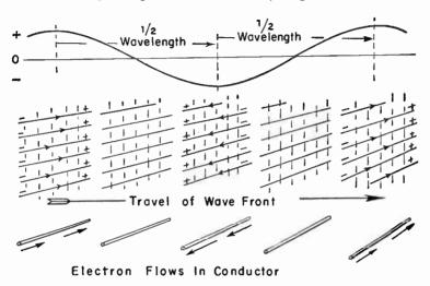
Fig. 9-1.—The electrostatic force of the radio wave causes alternating electron flows in the antenna conductors.
