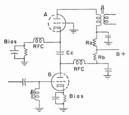
137-21.—Principle of the cascode amplifier with the triodes in series far signals, but not for d-c plate-cathode currents.
