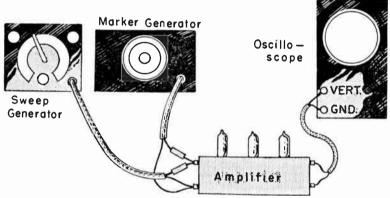
Fig. 47-2.—Connections of marker generator, sweep generator, and oscilloscope to amplifier or receiver.
