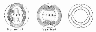
Fig. 25-1.—Arrangement of coils in a magnetic deflection yoke.
