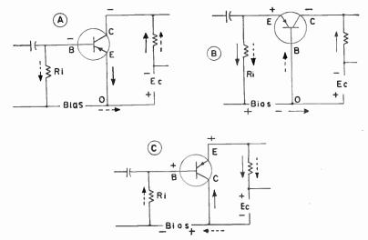
Fig. 9.—Directions of electron flows in transistor circuits.
