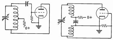
Fig. 91-3.-Modifications of the Hortley oscillator circuit.
