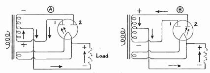
Fig. 110-2.—Current flow in a full-wave rectifier during opposite alternations of applied valtage.
