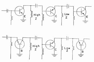
Fig. 14.—Impedances may be matched fairly well by using a grounded collector circuit between two circuits of other types.
