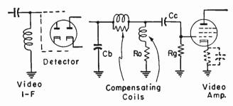
Fig. 29-2.—Features found in couplings between video detector and first video amplifier.
