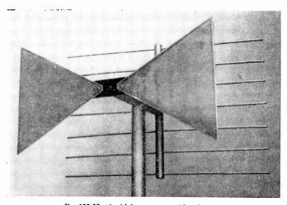
Fig. 138-20.—A uhf fan antenna with reflector.
