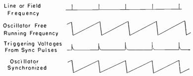
Fig. 55-1.—Sweep oscillator free running frequency is changed to sync frequency by the triggering pulses.
