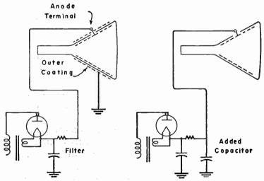
Fig. 134-2.—Using picture tube cootings as a high-voltage filter copocitor (left), ond connections for an added copocitor (right).
