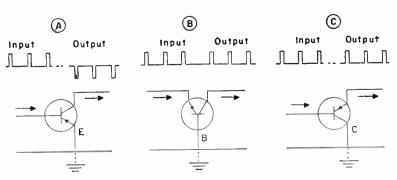
Fig. 15.—Signal polarity is inverted by a grounded emitter circuit, but not by a grounded base or by a grounded collector circuit.
