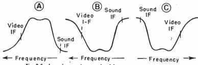
Fig. 8-5.—Inversions and reversals of frequency response curves.
