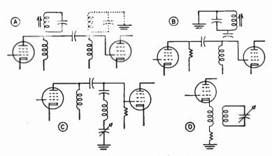
Fig. 128-1.—Interference traps of absorption types.
