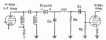
Fig. 29-4.—A crystal diode used as a video detector.
