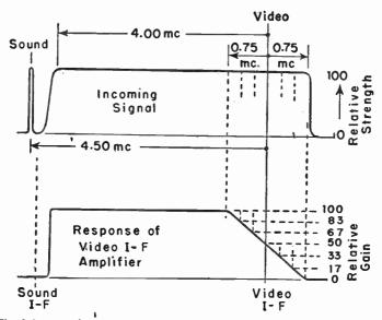
Fig. 8-6.—How the frequency response of the video i-f amplifier is shaped to equalize total amplification at all applied frequencies.
