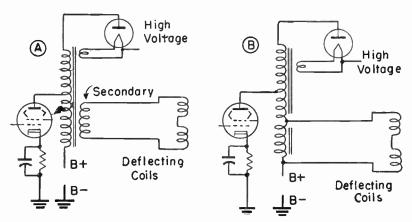
Fig. 5-19.—Insulated winding transformer and autotransformer used in horizontal sweep sections,
