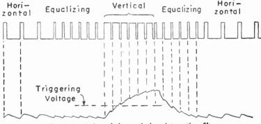
Fig. 35-3.—Action of the vertical or integrating filter.
