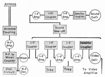
Fig. 1-1.—Ports or circuits of a television receiver in which there are odjustments for alignment.
