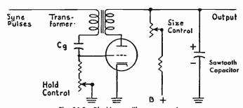
Fig. 96-3.—Blocking oscillator connections.
