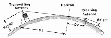
Fig. 108-2.—Factors which affect television and f-m radio reception distance.
