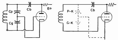
Fig. 95-1.—Colpitts oscillator with external tuning capacitonces (left) and with tuning by tube interelectrode capacitonces (right).
