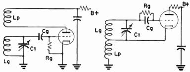
Fig. 91-5.—Tuned grid oscillators with tickler feedbacks.
