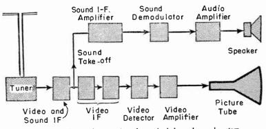
Fig. 120-1.—Scheme of connections for a dual-channel sound system.
