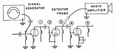
Fig. 125-1.—Connections for testing with a signal tracer.
