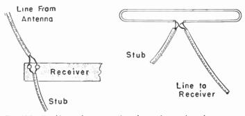
Fig. 68-3.—Matching stubs connected at the receiver and at the antenna.
