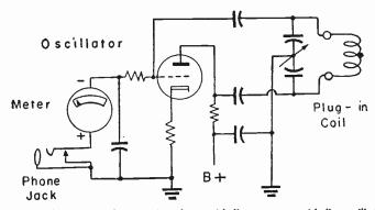
Fig. 76-1.—The ports and connections in a grid dip meter or grid dip ascillator.
