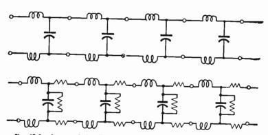
Fig. 68-2.—A transmission line consists, in effect, of many sections in which there is inductance, capacitance, and resistance.
