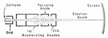
Fig. 6.—Electrostatic focusing is by means of electron lenses between electrodes
