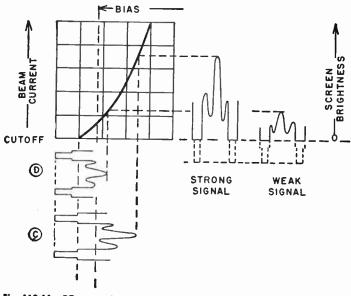
Fig. 113–11.—Effect on picture reproduction of equalizing the sync tip voltages for strong and weak signals.
