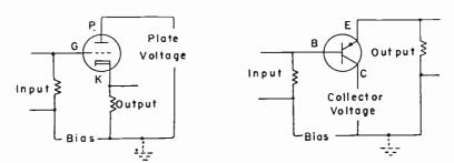
Fig. 7.—Cothode follower circuit for a triade tube (left) and the grounded collector circuit for a transistor (right).
