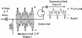
Fig. 7-8.—Picture signals are positive when the detector output is from the diade plate.
