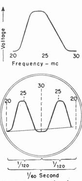
Fig. 1-5.—Appearance of a gain curve or frequency response on the oscilloscope when using the internal sweep.
