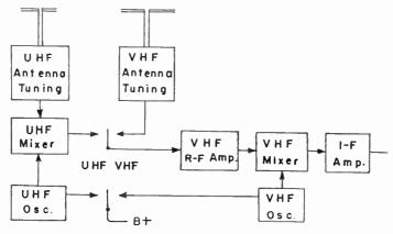
Fig. 138-3.—A system with which the r-f amplifier of the vhf tuner is used as an additional amplifier following the uhf mixer.
