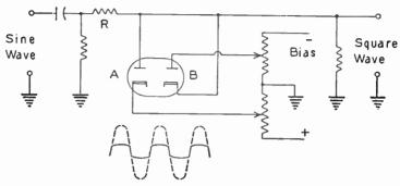
Fig. 50-2.—Square wave clipping circuit with diodes in parallel.
