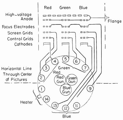
Fig. 5.—Base pin connections of a CBS-Colortron picture tube.
