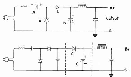
fig. 85-2.—Holf-wove voltage doubler (obove) and holf-wove voltage tripler (below). of the capacitors and limits the current in case of accidental short circuits. This resistor may be on either side of the line.
