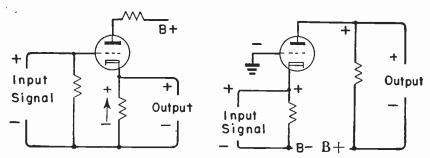
Fig. 64-2.—Tube circuits with which there is no inversion between input and output voltages.
