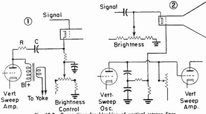
Fig. 10-8.—Connections for blanking of vertical retrace lines.
