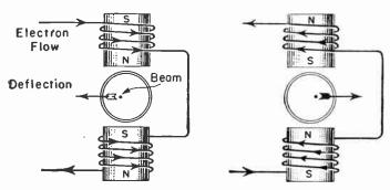
Fig. 13-3.—Effects of steady electron flow or direct currents in the yoke coils of a magnetic deflection system.
