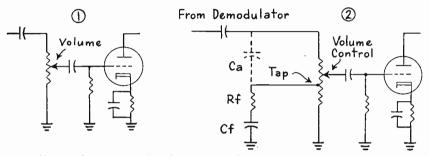
Fig. 2.—A compensated volume control helps maintain equality of low, middle, and high frequency sound at low volume.
