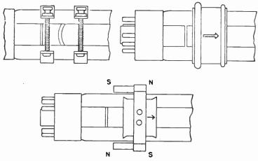
Fig. 129-3.—Methods of mounting double magnet ion traps on the necks of picture tubes.
