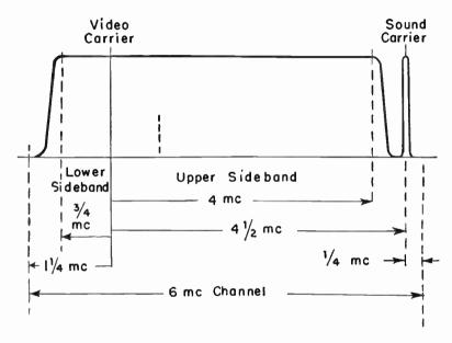
Fig. 127-1.—Distribution of transmitted frequencies within a six megacycle channel.
