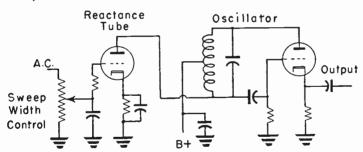
Fig. 51-2.—A reactance tube employed for frequency sweeping.
