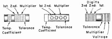
Fig. 12-3.—Color code markings for fixed ceramic and some other cylindrical or tubular capacitors.
