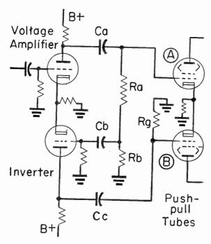
Fig. 3-2.—An inverter employing a resistance voltage divider.
