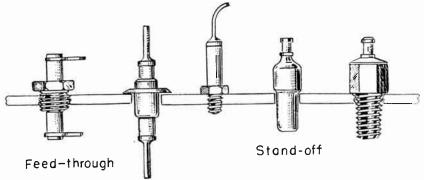
Fig. 12-5.—Copocitors of feed-through and standoff types.
