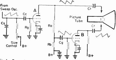
Fig. 4.—Connections for a phase inverter in an electrostatic sweep amplifier.
