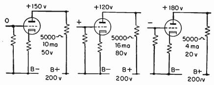
Fig. 64-1.—Inversion or phase reversal of voltages changes at grid and plate.
