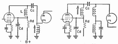
Fig. 8-2.—Tuning inductor locations in video i-f amplifiers.
