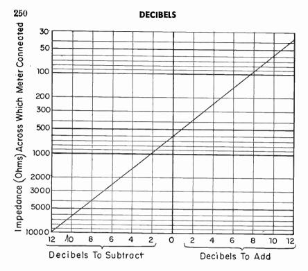
Fig. 3.—Corrections for decibel readings when a meter is across an impedance other than that for which calibrated.
