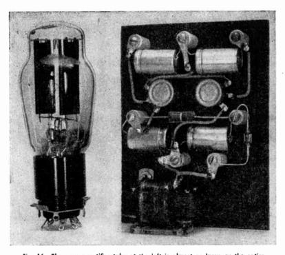
Fig. 16.—The power rectifier tube at the left is almost as large as the entire d-c power supply for transistors at the right.
