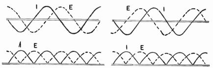
Fig. 67-3.—How standing waves may be represented in diagrams
