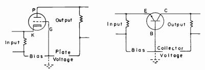
Fig. 6.—Grounded grid triode tube connections (left) and grounded base connections for a transistor (right).
