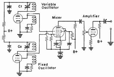
Fig. 89-1.—Circuits in one type of beot-frequency oscillator.
