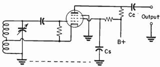
Fig. 90-1.—An electron coupled Hartley oscillator.
