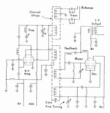
Fig. 5.—Circuit connections in a turret tuner employing a cascode r-f amplifier with another twin-triode as oscillator and mixer.
