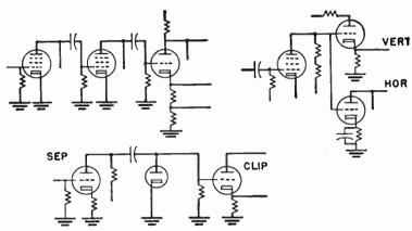
Fig. 122-3.—Connections in sync sections which provide two or more seporate outputs to filters.
