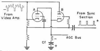
Fig. 43-11.—Keyed agc system in which positive keying pulses for control grids are taken from the sync section of the receiver.
