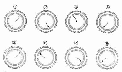
Fig. 37-9.—Permanent magnet centering when only one of the magnets is moved.
