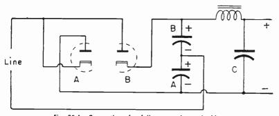
Fig. 85-1.—Connections for full-wave voltage doubler.
