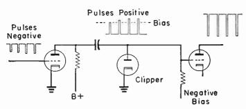
Fig. 15-1.—A diode used as a leveler or clipper for sync pulses.
