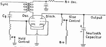
Fig. 96-5.—Discharge tube used with a blocking oscillator.
