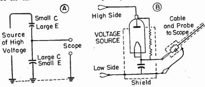
Fig. 107-4.—The principle of a capacitance voltage divider, and its application in a probe for waveform observation at high voltages.
