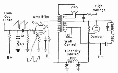
Fig. 5-14.—Typical horizontal sweep circuit for magnetic deflection.
