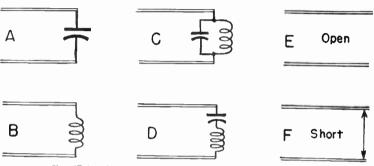
Fig. 67-2.—Line terminations which cause wave reflections.
