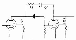
Fig. 26-2.—One method of obtaining voltage feedback.
