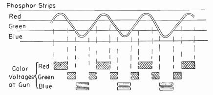
Fig. 30.—How the single electron beam traverses phosphor strips of three primary colors during horizontal traces.
