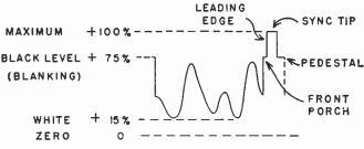
Fig. 118-2.—Voltage levels in a television signal.
