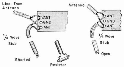
Fig. 63-6.—Transmission line stubs used as interference traps.
