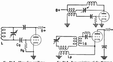
Fig. 91-7.—Ultraudion oscillator circuit.
