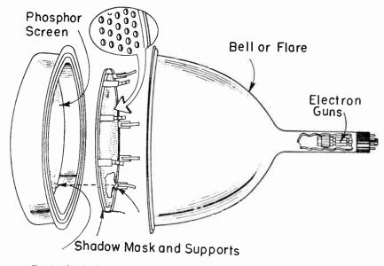
Fig. 4.—The shadow mask is a thin plate supported just back of the face plate which carries phosphor dots.
