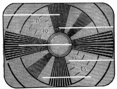
Fig. 63-1.—Effects of spark interference as seen at the picture tube.
