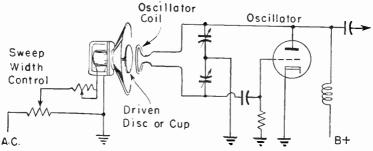
Fig. 51-3.—Electromechanical or electrodynamic method of frequency sweeping.
