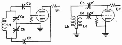
Fig. 91-4.—Colpitts oscillator circuits.
