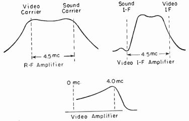
Fig. 2-1.—Typical frequency responses of broad band amplifiers,
