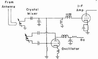
Fig. 80-3.—Connections between o crystol diode mixer, uhf ontenno, and uhf oscillotor tube.
