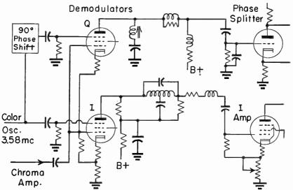
Fig. 16.—A method of demodulating to secure I- and Q-signals.
