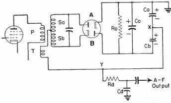
Fig. 28-1.—Typical circuit for a ratio detector used in f-m sound systems.
