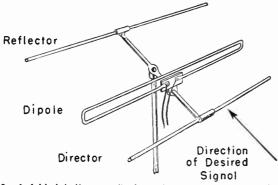
Fig. 9-12.—A folded holf-wove dipole with a reflector element back of it and a director element in front.
