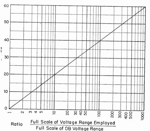
Fig. 4.—Additions for decibel readings when a meter is used on a ronge other than that for which the db scale is colibrated.
