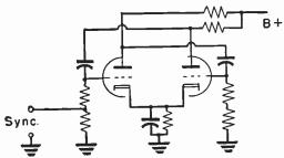
Fig. 94-1.—Connections for a multivibrator oscillator.
