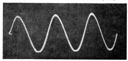
Fig. 99-3.—Three cycles of a sine-wave valtage are shown on the screen of the ascillascape.
