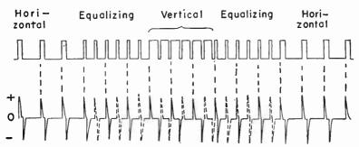
Fig. 35-2.—Action of the horizontal or differentiating filter.
