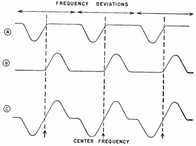
Fig. 120-4.—Audio-frequency voltage pulses produced by frequency deviations.
