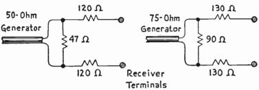
Fig. 100-1.—Motching pods used between signol generators and receiver ontenna terminals.
