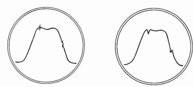
Fig. 1-7.—Frequency identification on traced responses by marker pips (left) and marker dips (right).
