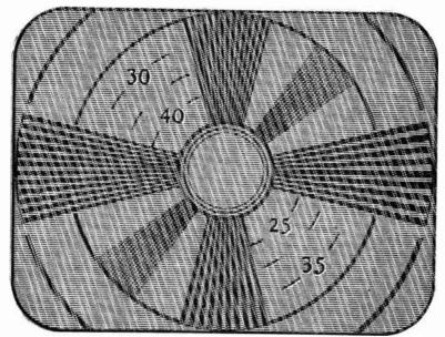
Fig. 63-3.—Radio-frequency interference causes beats which produce narrow lines on the screen pattern or picture.
