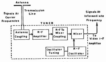
Fig. 1.—Principal parts of the tuner.
