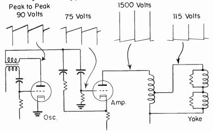
Fig. 10-10.—Waveforms in a vertical sweep section.
