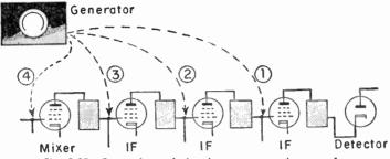
Fig. 8-25.—Connections of signal generator and output for video i-f alianment.
