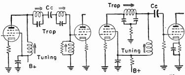
Fig. 8-3.—Porollel resonant trops in interstage couplings of video i-framplifiers.
