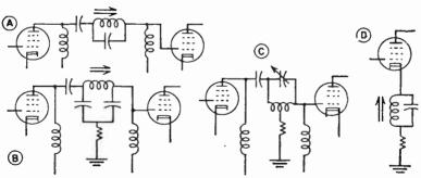
Fig. 128-2.—Interference traps of impedance types.
