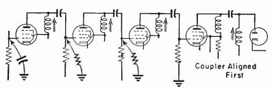
Fig. 8-21.—Grounding of control grids through capacitors or resistors to prevent oscillation during alignment.
