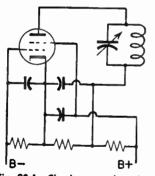
Fig. 93-1.—Circuit connections for a dynatron oscillator.
