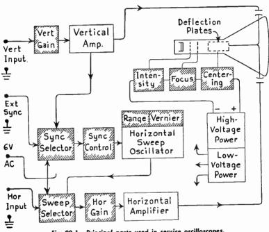
Fig. 99-1.—Principal parts used in service oscilloscopes.
