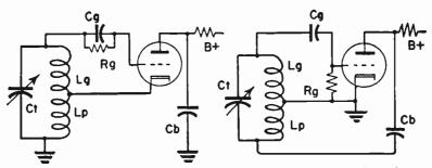
Fig. 91-2.—Hortley oscillotors with grounded tuning copocitor (left) and with grounded cothode (right).
