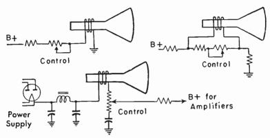
Fig. 37-3.—Control odjustments for current in magnetic focusing coils.
