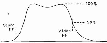
Fig. 8.7.—Typical frequency response of a video i-f amplifier system.
