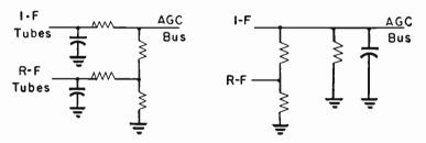
Fig. 43-7.—Methods of lessening the automotic gain control action on r-f amplifiers.
