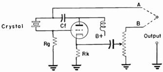
Fig. 46-2.—An untuned crystal-controlled r-f oscillator.
