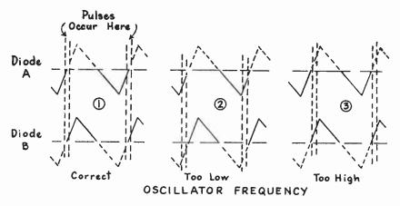
Fig. 97-4.—Conductions in the phase detector diodes.
