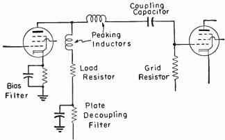
Fig. 2-2.—Ports which offect response of lowest and highest frequencies in video detector and video amplifier couplings.
