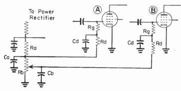
Fig. 10-5.—Fixed bias with decoupling capacitors and resistors.
