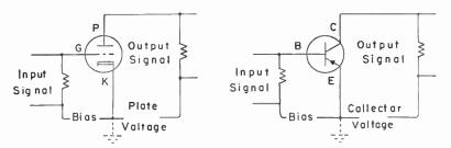
Fig. 5.—Grounded cathode circuit for a triode tube (left) and grounded emitter circuit for a transistor (right).
