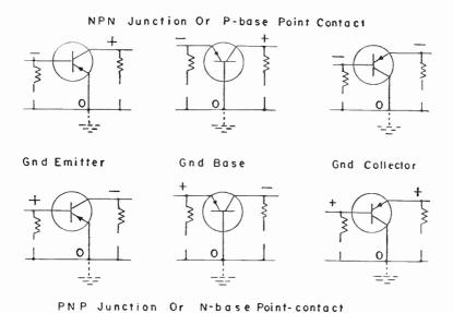
Fig. 8.—Transistor element polarities with reference to the common or grounded element.
