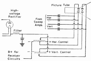
Fig. 5.—Centering controls used with electrostatic deflection.
