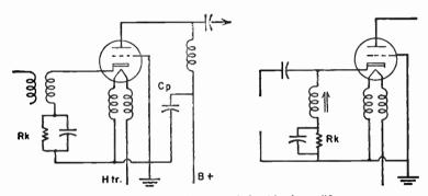
Fig. 133-1.—Circuits for grounded grid r-f amplifiers.
