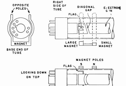
Fig. 129-1.—Ion trap of the type requiring a double magnet.
