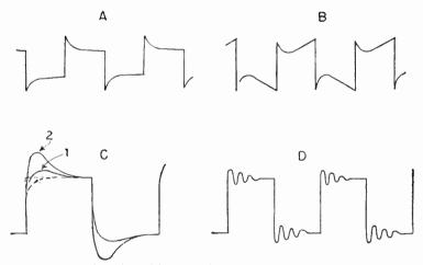
Fig. 50-5.—Faults indicated by traces from square waves. A, phase distortion with current leading. B, phase distortion with current lagging. C, effects of frequency compensation. D, oscillation in amplifier.
