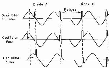
Fig. 97-10.—How sync pulses and a sine wave voltage from the ascillator circuit combine at the discriminator diades.
