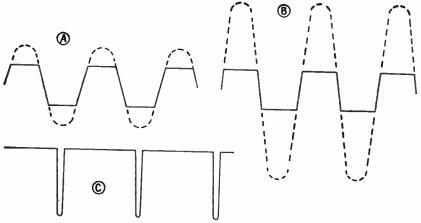
Fig. 3.—With sine-wave voltage applied to agated beam tube, the autput may be made square waves, pulses, or other forms.
