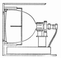
F.g. 134-11.—Picture tube mounted between cabinet front and a cushion on the yoke ossembly.
