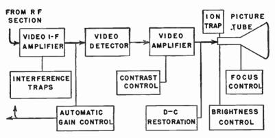
Fig. 124-3.—The video section with its accessories and controls.
