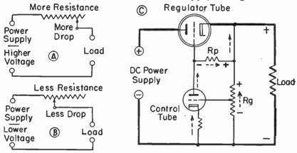
Fig. 111-2.—A method of automatic voltage regulation by variation of resistance in series between source and load.
