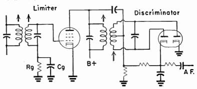
Fig. 66-1.—A limiter with its biasing resistor and capacitor in the grid return connection to ground.
