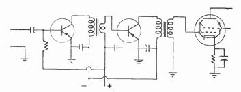
Fig. 12.—The two transistors are used in grounded emitter circuits. The first coupling transformer has a step-down turns ratio for matching of transistar impedances.
