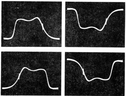
Fig. 99-8.—The same frequency response may appear in any of these positions on the oscilloscope screen.
