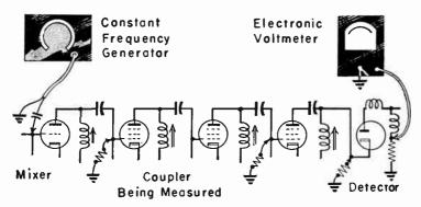
Fig. 8-34.—Determination of frequencies at which individual couplers are peaked.
