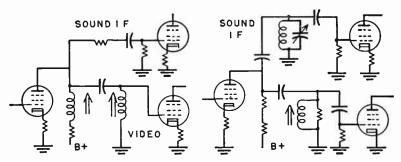
Fig. 120-2.—Sound takeoff connections for dual-channel sound systems.
