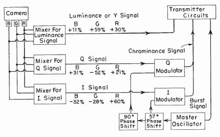
Fig. 7.—How color signals are formed at a transmitter.
