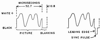
Fig. 118-1.—Television signal valtages during one line period.
