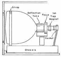
Fig. 134-9.—Picture tube mounted on chassis.
