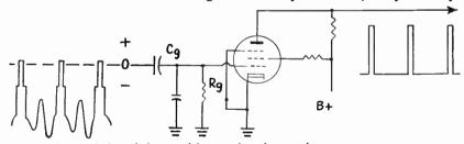
Fig. 2.—Action of the gated beam tube when used as a sync separator.
