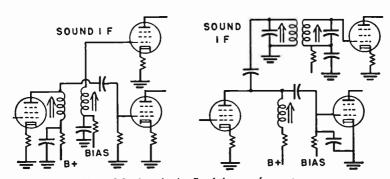
Fig. 120-3.—Sound takeoffs of the transformer type.
