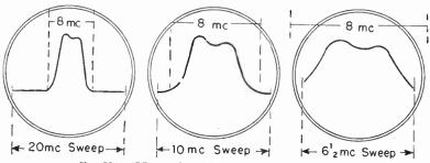
Fig. 51-4.—Effects of varying o sweep width control.
