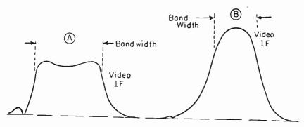
fig. 8-9.—How i-f response curves are affected by increasing the gain.
