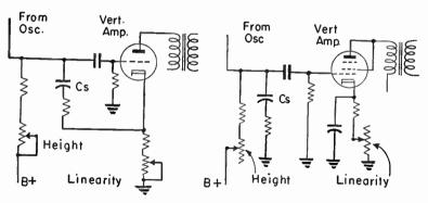
Fig. 69-5.—Linearity controls on output amplifiers in a vertical deflection system.
