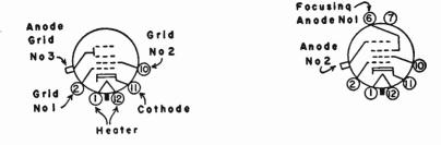
Fig. 134-5.—Base pin positions and element connections for magnetic deflection picture tubes.
