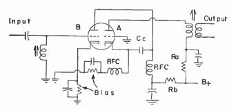
Fig. 137-22.—The second style of cascode r-f amplifier may be shown in this general manner on circuit diagrams.
