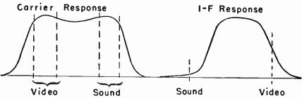
Fig. 62-4.—Typical frequency responses for receivers having intercarrier sound systems.
