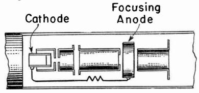
Fig. 37-7.—Position of an electrostatic focusing anode in the electron gun.
