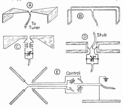
Fig. 9-19.—Various styles of built-in antennas.
