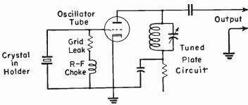
Fig. 20-1.—The circuit for a simple crystal-controlled oscillator.
