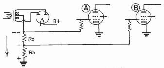
Fig. 10-4.—The principle of fixed bias.
