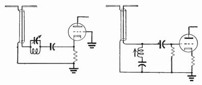
Fig. 63-5.—Parallel and series resonant traps shown connected to inputs from coaxial transmission line.
