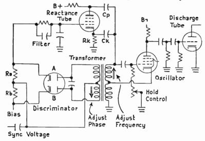
Fig. 97-9.—The discriminator furnishes correction voltage to the reactance tube grid, and reactance tube plate current varies the oscillator frequency
