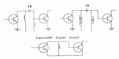
Fig. 13.—Resistance and impedance couplings have equal output and input impedances for signal voltages and currents.
