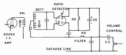
Fig. 120-7.—Ratio detector in a sound system whose cathode line supplies plate and screen voltages to other tubes.
