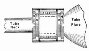
Fig. 25-2.—Positions of the yoke and deflecting coils on the neck of a picture tube.
