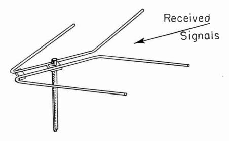
Fig. 9-9.—A V-type antenna for broad band reception.
