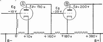
Fig. 3- .—Elementary principle of the direct-coupled amplifier.
