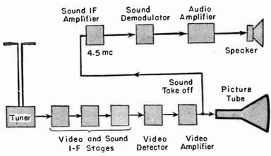
Fig. 62-1.—Signal paths in a receiver employing intercarrier sound.
