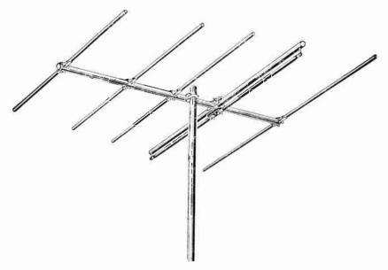
Fig. 9-15.-A five-element Yagi antenna.
