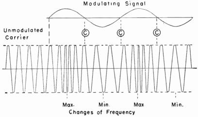
Fig. 82-1.—The principle of frequency modulation.
