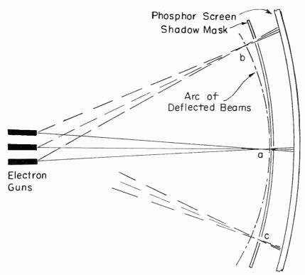
Fig. 23.—Points of beom convergence will not remain at the shodow mask when the beams are deflected, unless corrections are applied.
