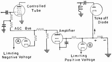
Fig. 43-8.—Two woys in which diodes may be used as noise limiters.
