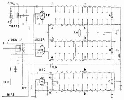
Fig. 13.—Shorted quarter-wave resonant lines in a tuner.
