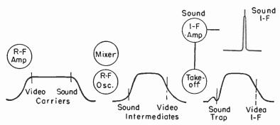
Fig. 8-22.—Frequency responses when the sound system operates at the sound intermediate frequency.
