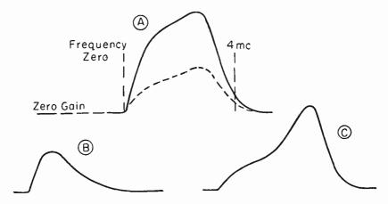
Fig. 7-7.—Frequency response curves of a video amplifier.
