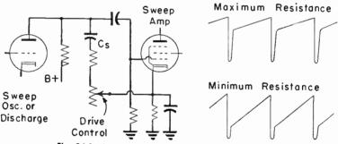
Fig. 34-1.—Resistor type drive control and its action.
