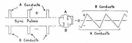
Fig. 97-3.—Sync pulses and a sawtooth voltage as applied to opposite sides of a phase detector.
