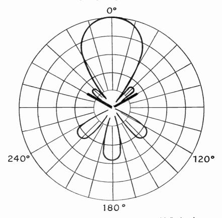
Fig. 9-8.—How response labes are combined by forward inclination of antenna conductors.
