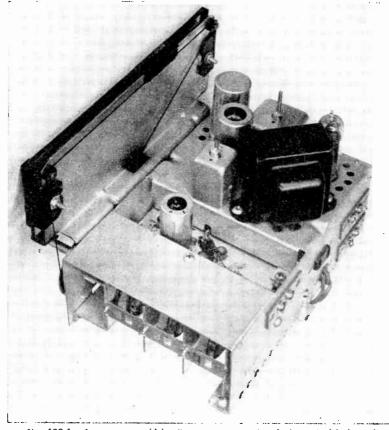
Fig. 138-1.—A converter which allows reception of unf channels 14 through 83 on television receivers designed for channels 2 through 13.
