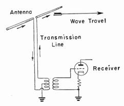
Fig. 9-2.—Connection of a dipole antenna through a transmission line ta the receiver.
