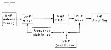
Fig. 138-17.—To the uhf mixer is applied a harmonic of the fundamental frequency at which the vhf oscillator operates.
