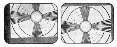
Fig. 13-1.—The pattern or picture may be off center in one or more directions.
