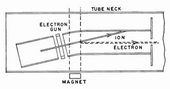
Fig. 129-4.—Operating principle of the bent-gun ion trop employing a single magnet.
