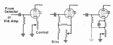
Fig. 18-5.—Contrast controls consisting of adjustable cathode bias on video amplifier tubes.
