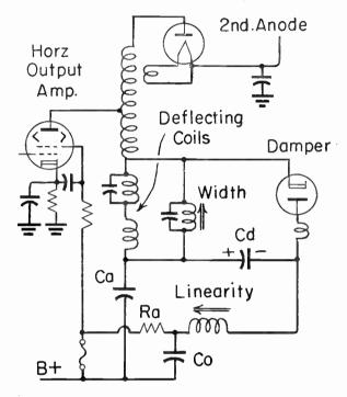
fig. 5-21.—Deflecting coils of the yoke form a secondary for this autotransformer. tube is not of a type which safely will withstand heater-cathode voltages much in excess of 2,000, the value of peak potential often found in horizontal yoke circuits.
