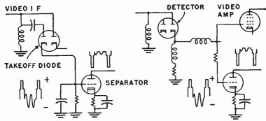
Fig. 116-1.—Sync takeoff from the final amplifier in the video i-f section.
