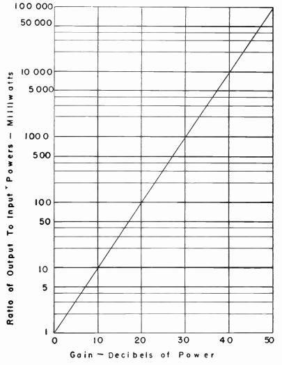
Fig. 10.--Relations between gains measured in decibels of power and in ratios of output to imput milliwatts
