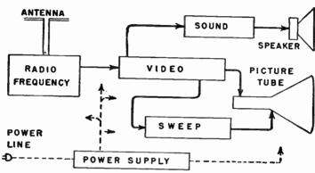
Fig. 124-1.—The principal sections of a television receiver.
