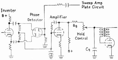
Fig. 97-5 —Sweep atc system employing an amplifier between a phase detector and a blocking occurator.
