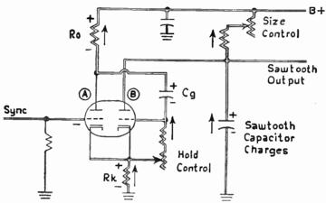
Fig. 96-6.—A cathode-coupled multivibrator sweep oscillator.
