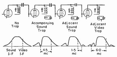
Fig. 8-24.—How various traps affect frequency responses in the video i-f amplifier.
