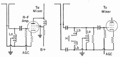
Fig. 4-1.—Untuned coupling between antenna and r-f amplifier.
