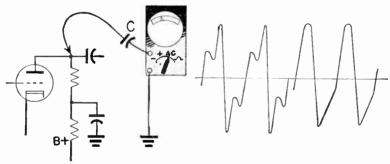
Fig. 74-2.—Protecting the voltmeter against high direct potential.
