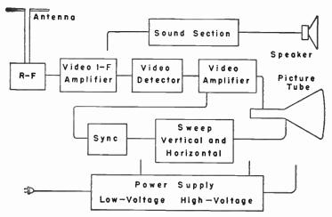
Fig. 130-1.—Sections of receiver to be considered during location of troubles.
