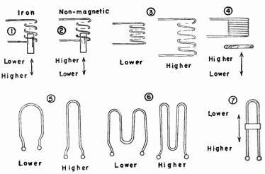
Fig. 20.—How resonant frequency is affected by various methods of adjusting inductors used in tuners.
