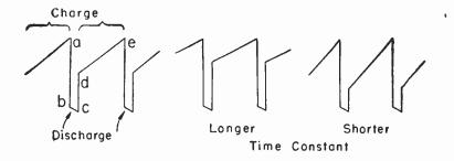
Fig. 5-11.—How the negative pulse is added to the sawtooth voltage.
