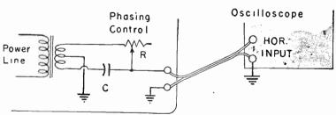
Fig. 51-10.—A phase shifting circuit for synchronized sweep voltage.
