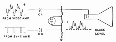
Fig. 113-12.—Black level control system in which sync pulses are removed to leave only the pedestals of the signal.
