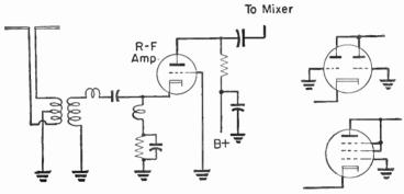
Fig. 4-3.-Connections used for grounded grid r-f amplifiers.
