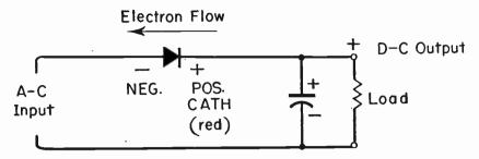
Fig. 110-3.—A selenium rectifier in a half-wave circuit.
