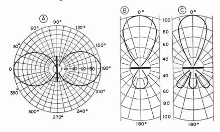
Fig. 9-4.—Polar diagrams showing directional responses of antennas.
