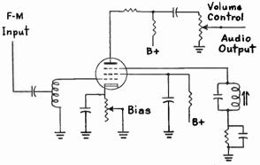
Fig. 1.—The gated beam tube in on f-m sound demodulator circuit.
