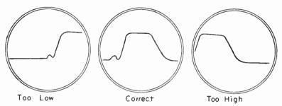
Fig. 51-6.—Effects of altering the center frequency of the sweep generator.
