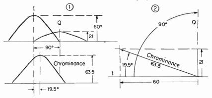
Fig. 11.—I- and Q-signals combine in this manner to form a chrominance signal corresponding to red.
