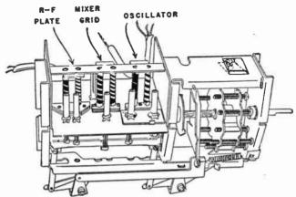
Fig. 16.—A variable inductorice tuner in which inductor cores are moved within the windings by the channel selector shaft.
