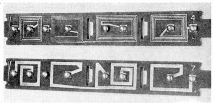
Fig. 7.—An incremental tuner with which channel selection is by means of rotary switch sections.
