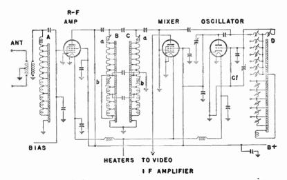
Fig. 10.—Addition of antenna tuning with shorting connections made through a rotary selector switch.
