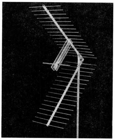
Fig. 138-22.—A carner reflector who antenna with a plain dipole as the active element.
