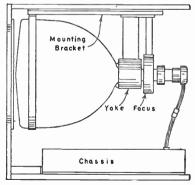
Fig. 134-10.—Picture tube mounted in top of cabinet.
