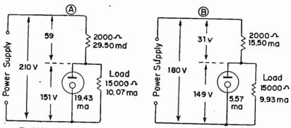
Fig. 111-4.—Performance of a glow tube regulator when there are fluctuations of power supply voltage.
