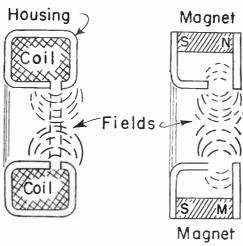
Fig. 37-4.—Magnetic fields are alike for electromagnetic and for permanent magnet focusing.
