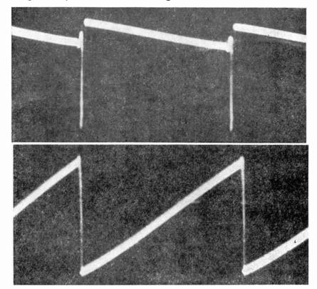
Fig. 99-13.—The voltage waveform at A is quite different from the current waveform at B, a though both are taken from the same circuit camponents.
