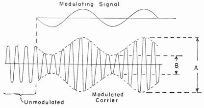
Fig. 81-1.—The principle of amplitude modulation.
