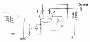
Fig. 137-20.—How the cascode a-f amplifier may be shown in television receiver diagrams.
