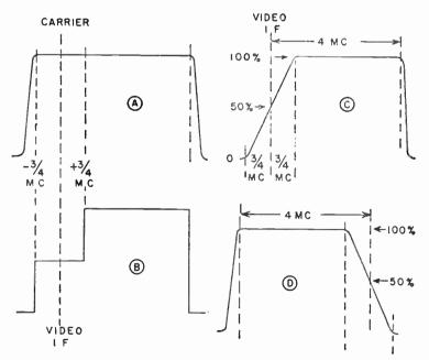
Fig. 127-2.—How receiver attenuation compensates for double transmission of some signal modulation frequencies.
