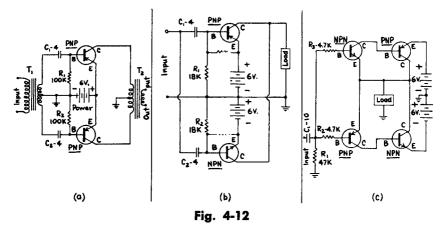
**PUSH-PULL CIRCUITS** — (a) Conventional; (b) Complementary Symmetry; (c) Cascaded Complementary Symmetry. Circuit (a) is a conventional transformer-coupled push-pull amplifier employing transistors of the same type. The general arrangement is quite similar to its vacuum tube counterpart. D.C. stabilization is not provided in the circuit shown, although it is recommended in power applications (see Fig. 4-4).
