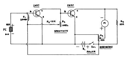
Fig. 9-25.—A very Sensitive Light Meter circuit featuring a cascaded complementary amplifier.
