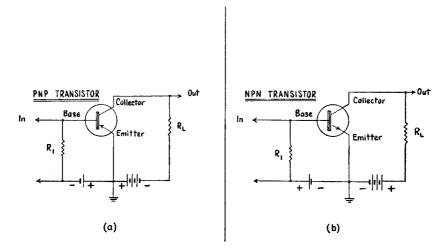
Fig. 1-6.—The schematic symbols and D.C. power supply connections for PNP and NPN transistors are shown here. The only difference in the schematic symbols is in the direction in which the arrowhead points on the line representing the emitter electrode.
