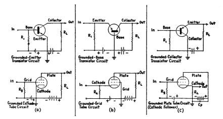
Fig. 1-7.—The three basic transistor circuit configurations with the roughly equivalent vacuum tube circuit arrangements. Power supply polarities shown are for PNP transistors . . . polarities would be reversed for NPN units. See TABLE A for a comparison of their basic electrical characteristics.
