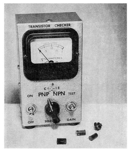
Fig. 9-19.—Author's model of the Transistor Checker.
