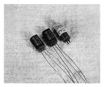
Fig. 1-5.—As this photograph shows, point-contact transistors are no larger than junction units. The cylindrical unit is an early point-contact transistor, the other two are junction units. All three are produced by the same manufacturer—RAYTHEON.
