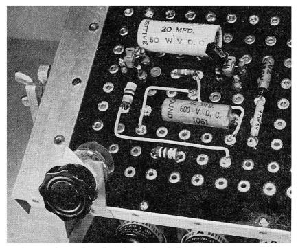
Fig. 13-6.—An experimental transistor circuit wired on a commercial "Breadboard" Chassis. Photo Courtesy The Electratomic Company, Wheaton, Md.
