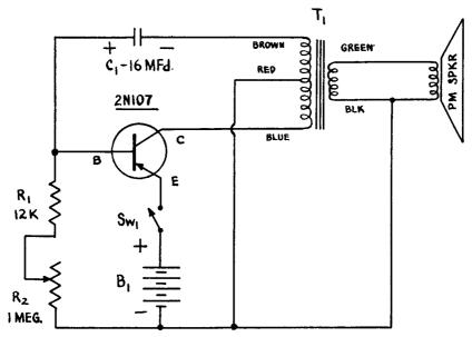
Fig. 10-16.-Schematic diagram of a transistorized Metronome.
