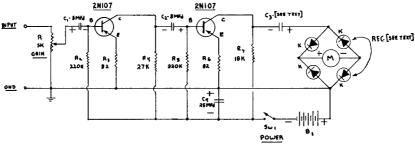
Fig. 9-26.—Schematic of an easily built Audio Level Meter.
