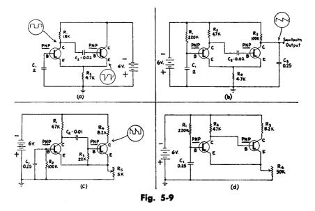
**EMITTER-COUPLED MULTIVIBRATORS** – (a) Basic Emitter-Coupled circuit; (b) Sawtooth waveform circuit; (c) Adjustable stability circuit; (d) Directcoupled circuit. The emitter-coupled transistor multivibrator is roughly analogous to the cathode-coupled vacuum tube multivibrator.
