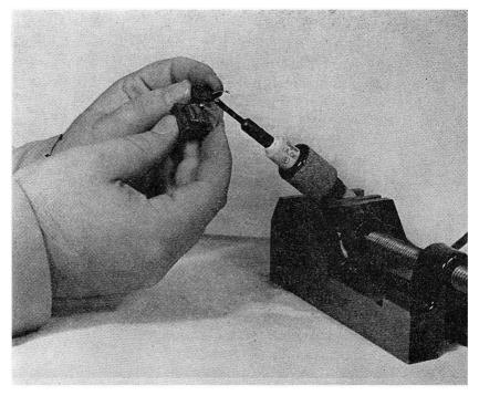
Fig. 2-3.—Some technicians prefer to clamp their soldering instrument in a vise.
