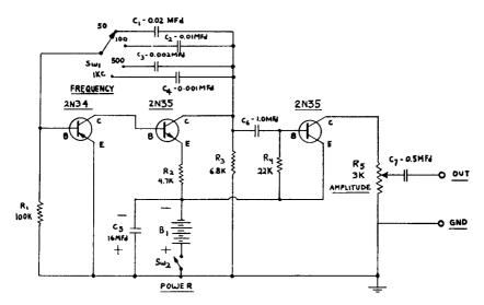
Fig. 9-10.—Schematic of a simple 4-frequency Square-Wave Generator.
