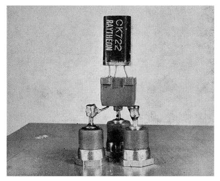
Fig. 2-5.—Detail of transistor socket mounting.
