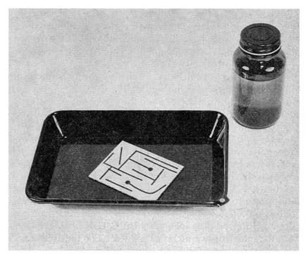
Fig. 13-4.—After the desired layout has been transferred to the copper-clad laminate as a pattern of resist, the board is etched in an enamel or plastic tray.
