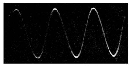
Fig. 9-3.—The nearly perfect sine wave signal obtained from the Audio Generator.
