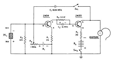
Fig. 10-15.—Circuit for a Light Beam Receiver or Audio Photometer.
