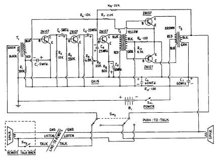
Fig. 7-13.-- A transistorized two-station Intercom.
