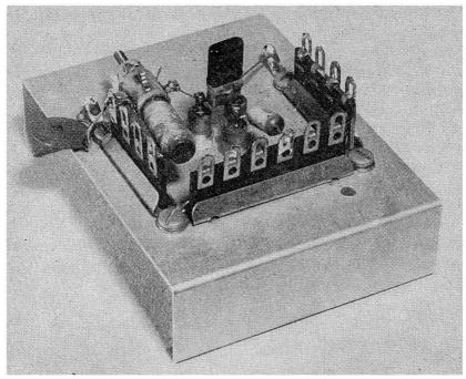
Fig. 8-25.-Breadboarded Frequency Doubler.
