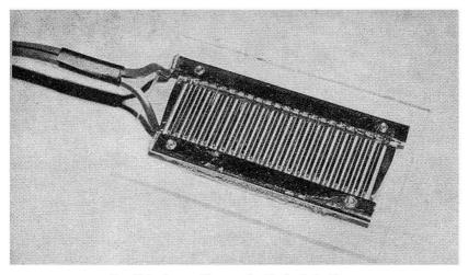
Fig. 10-5.—Sensor Plate used with the Rain Alarm.
