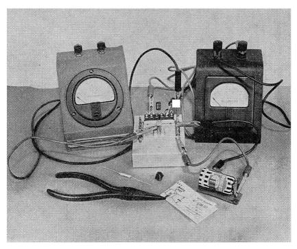
Fig. 2-6.—A typical experimental set-up for checking a breadboarded transistor circuit.
