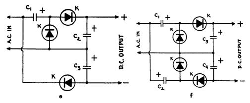
Fig. 10-20.—Basic semiconductor diode Rectifier circuits: (a) Half-Wave; (b) Full-Wave; (c) Full-Wave Bridge; (d) Voltage-Doubler; (e) Voltage-Tripler; (f) Voltage-Quadrupler.
