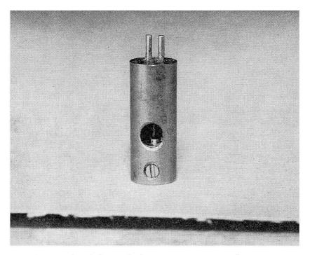
Fig. 1-4.—Enlarged photograph of a point-contact transistor. The two cat'swhiskers and the small block of semiconductor material are clearly visible.
