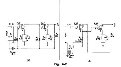
A.C. TYPE DIRECT-COUPLED AMPLIFIERS — (a) Two-stage amplifier made up of cascaded grounded-emitter stages; (b) Two-stage amplifier made up of a grounded-collector stage direct-coupled to a grounded-emitter stage. Of the two circuits shown, circuit (a) has by far the greater gain, but circuit (b) has a higher input impedance.
