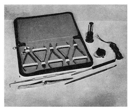
Fig. 2-1.—Hand tools useful when working with transistor circuits.
