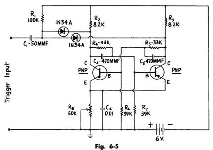
**BISTABLE CIRCUIT** — This circuit represents a transistorized version of a familiar vacuum tube binary counter. In essence, it is a non-oscillating collector-coupled multivibrator which has two stable states, and which can be transferred from one state to the other by the application of an appropriate trigger pulse. In operation, one or the other of the two transistors starts conducting first.
