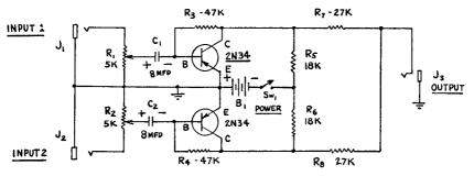
Fig. 7-17.---A transistorized 2-Channel Audio Mixer.
