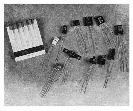
Fig. 1-1.—A collection of typical transistors. A match book is included for size comparison. Transistors shown include units manufactured by RCA, GE, CBS-HYTRON, SYLVANIA, RAYTHEON, RADIO RECEPTOR, AMPEREX, TRANSISTRON, and GERMANIUM PRODUCTS.
