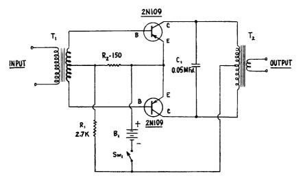
Fig. 7-2.—Basic Push-Pull Power Amplifier.
