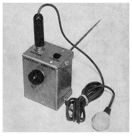
Fig. 7-6.-Exterior view of the electronic "Stethoscope"
