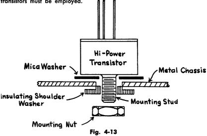
**POWER AMPLIFIERS** — A typical mounting for a "high power" transistor is shown. In order to improve heat dissipation, power transistors are frequently assembled in a metal case which serves as a heat radiator. This case, in turn, may be mounted on a metal chassis to provide a "heat sink".
