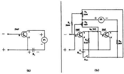
Fig. 9-21.—Circuits for two transistorized Meter Amplifiers—(a) Single Stage and (b) Cascaded Stages.
