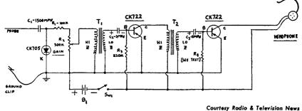
Fig. 9-27.—Schematic diagram of a transistorized Signal Tracer.
