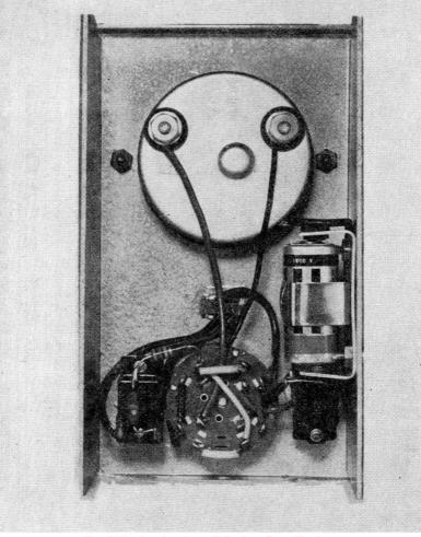
Fig. 9-20.—Interior view of the Transistor Checker.
