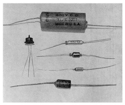
Fig. 3-2.-Subminiature electrolytic capacitors compared to a standard paper unit.
