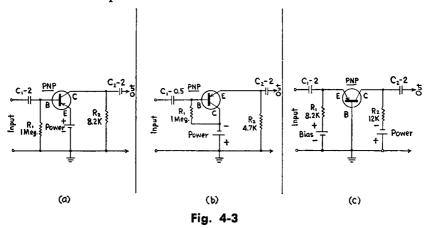
**BASIC AMPLIFIER CONFIGURATIONS** – (a) Grounded-emitter; (b) Grounded-collector; (c) Grounded-base. Resistive loads and capacitive coupling are shown in all three circuits. Signal phase reversal occurs in the grounded-emitter circuit (a), but not in the grounded-collector (b) and grounded-base (c) circuits.
