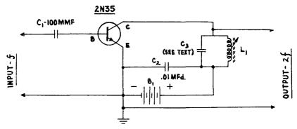
Fig. 8-24.-Diagram of a basic transistorized R.F. Frequency Doubler.
