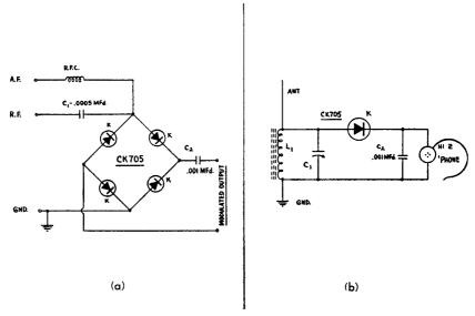
Fig. 10-26.—R.F. Semiconductor Diode applications: (a) Bridge Modulator; (b) Simple Crystal Receiver.
