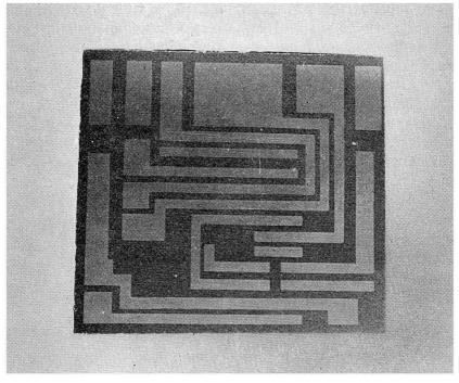
Fig. 13-5.—A typical etched circuit board.
