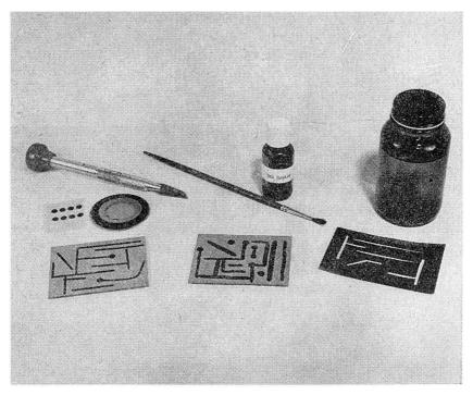
Fig. 13-3.—Three popular techniques used for making up "one-shot" etched circuits in the laboratory. Reading from left to right, the methods shown include tape resist, ink resist, and a photographic negative for a printed circuit layout.
