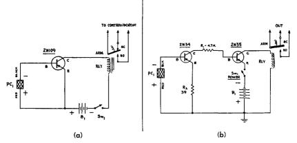
Fig. 10-6.—Two "Electric Eye" relay circuits (a) Basic circuit; (b) Sensitive version.
