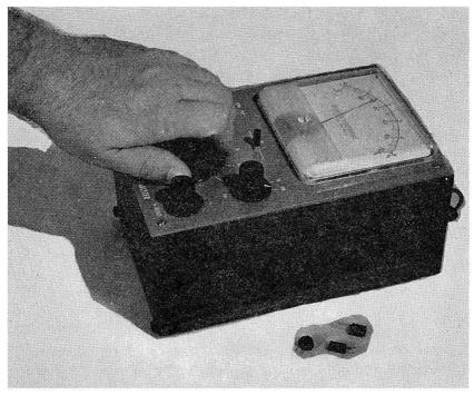
Fig. 13-7.—Using a QUANTUM Junction Transistor Analyzer to check transistors.
