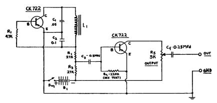
Fig. 9-1.--Circuit for the transistorized Audio Sine Wave Signal Generator.
