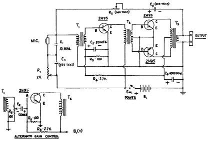
Fig. 7-19.—A transistorized P.A. System.
