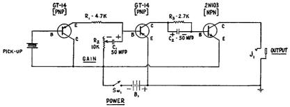
Fig. 7-5.—A transistorized electronic "Stethoscope".
