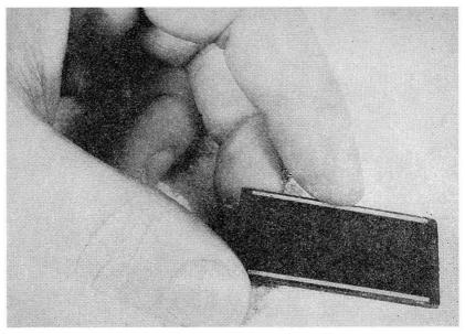
Fig. 10-28.-A single selenium Photocell.
