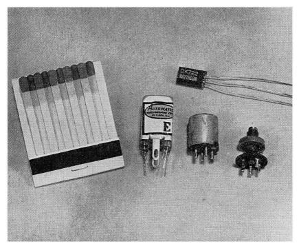
Fig. 3-3.—Subminiature R.F. coils and I.F. transformers.
