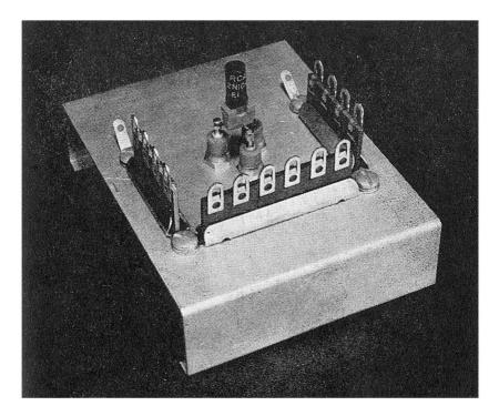
Fig. 2-4.—A "Universal" Breadboard chassis designed for transistor tests.
