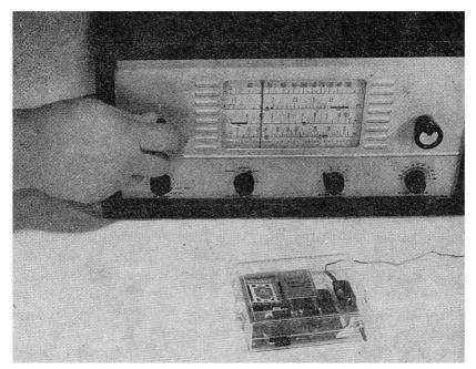
Fig. 8-19.—Checking the dial calibration of a communications receiver.
