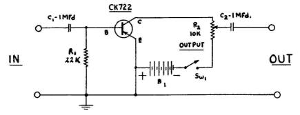
Fig. 9-16.—Schematic of a simple, but useful, test instrument—a Sine Wave Clipper.
