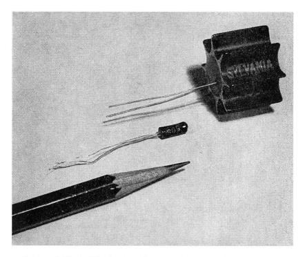
Fig. 1-2.—A TRANSISTRON hearing aid type transistor compared to a SYLVANIA power transistor to show relative sizes. Pencil gives an idea of true size.
