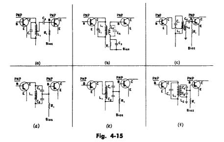
**R. F. AMPLIFIER COUPLING METHODS** — (a) Tapped coil; (b) Transformer coupling; (c) Tapped-primary transformer coupling; (d) "Tapped" capacitor; (e) Tapped coil and tapped capacitor; (f) Transformer coupling with tapped capacitor. In all the circuits shown, it is assumed that the grounded-emitter configuration has been employed; however, similar techniques could be used for the other configurations.
