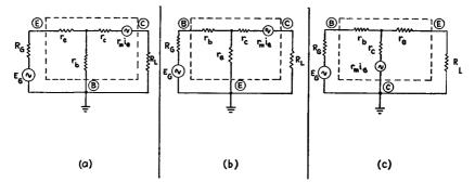
Fig. 12-4.—The three fundamental transistor circuit configurations shown as their operating T network equivalent circuits. The emitter, base, and collector connections are identified outside the dotted box, which represents the transistor proper. The grounded-base configuration is shown at (a), the grounded-emitter configuration at (b), and the groundedcollector configuration at (c).
