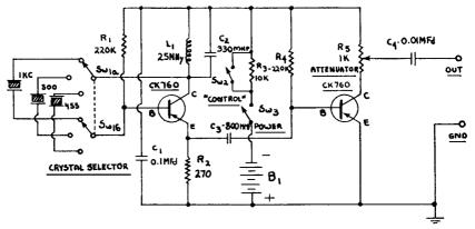
Fig. 9-4.—Schematic diagram of an R.F. Alignment Generator.
