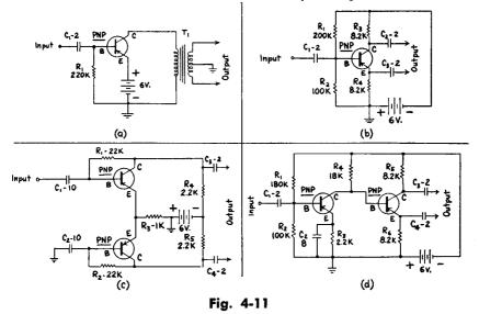
**PRACTICAL PHASE INVERTERS** — (a) Transformer type; (b) Split-load type; (c) Emitter-coupled type; (d) Split-load type direct-coupled to a groundedemitter amplifier.
