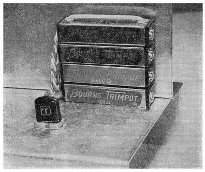
Fig. 9-23.—Range calibration potentiometers used in a transistorized meter circuit.
