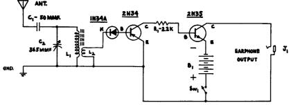
Fig. 8-5.—Schematic diagram of a Pocket Receiver using a two-stage complementary amplifier.
