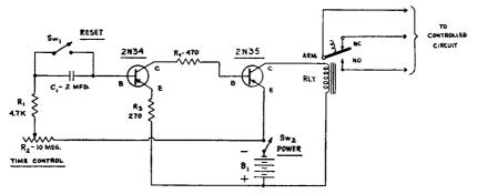
Fig. 10-2.—A "Precision" transistorized Timer circuit—no electrolytic capacitors are used.
