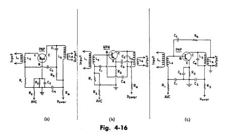
**NEUTRALIZATION METHODS**—(a) Grounded-base amplifier; (b) Groundedemitter amplifier with primary feedback; (c) Grounded-emitter amplifier with secondary feedback. In all three circuits, it is assumed that the transistors are used as receiver R.F. or I.F. amplifiers and hence a source of AVC current is indicated; however, similar techniques may be used with power amplifiers.
