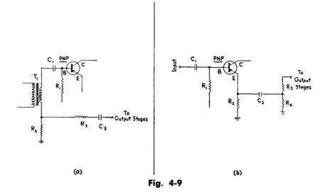
**OVERALL FEEDBACK** — (a) Series type base-coupled; (b) Emitter-coupled. As with vacuum tube audio amplifiers, the over-all frequency response may be improved and distortion reduced if inverse feedback is used between the output and input stages of a multi-stage transistor amplifier.
