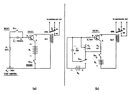
Fig. 10-1.—Two simple transistorized Timers: Circuit (a) operates on the "charge" cycle of a capacitor, circuit (b) on the "discharge" cycle.
