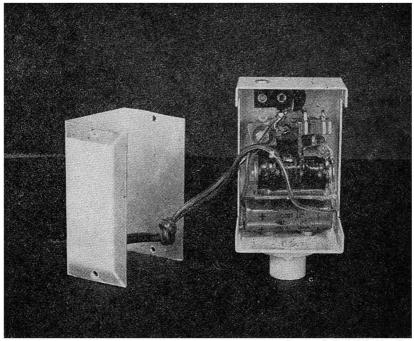
Courtesy Radio & Television News Fig. 10-23.—Interior view of the CdS Photocell Relay.
