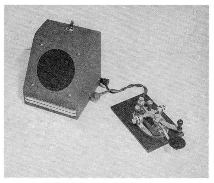
Fig. 10-14.-Loudspeaker type Code Practice Oscillator.
