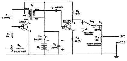
Fig. 9-13.—Circuit of a transistorized Pulse Generator delivering both positive-going and negative-going pulses.
