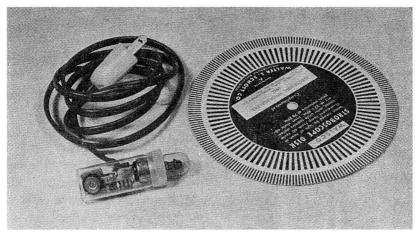
Fig. 10-25.-A 60 Cycle Stroboscope . . . shown with the disk with which it is used.
