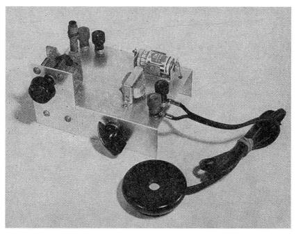
Fig. 8-4.—Author's model of the Regenerative Receiver. Transistors are mounted below chassis.
