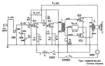
Fig. 7-23.—Circuit of a high quality transistorized Phonograph Amplifier. This unit might also be used as a Guitar or similar "Music" amplifier, or even as a low power P.A. system.
