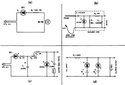
Fig. 10-24.—General semiconductor applications: (a) 60 Cycle Stroboscope; (b) Signal Tracing Probe; (c) Zener Oscillator; (d) Clipper.
