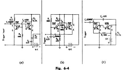
**MONOSTABLE CIRCUITS** — (a) Collector-Coupled; (b) Emitter-Coupled; (c) "Complementary Symmetry" Collector-Coupled. All three circuits are direct adaptations from corresponding multivibrator circuits.
