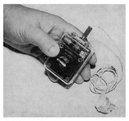
Fig. 8-6.—Exterior view of the Pocket Receiver . . . assembled in a small plastic box!
