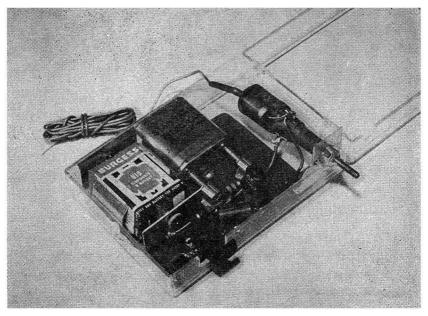
Fig. 8-20.—Interior view of the Crystal Calibrator.
