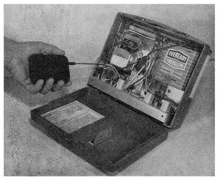
Fig. 9-9.—Using The Signal Squirter to service a transistorized receiver.
