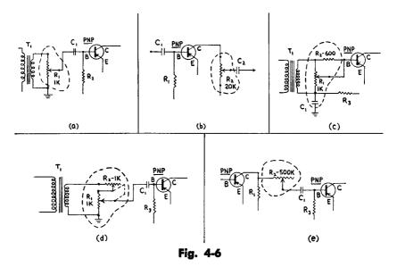
**GAIN CONTROLS** — An input gain control is shown at (a); an output gain control at (b); two types of "constant impedance" controls at (c) and (d); a series type gain control at (e). The actual control circuits are enclosed by dotted lines.
