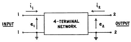
Fig. 12-1.—Basic four-terminal network representation shown as a "black box." Input and output terminals and input and output voltages and currents are identified. Arrows show conventional flow.
