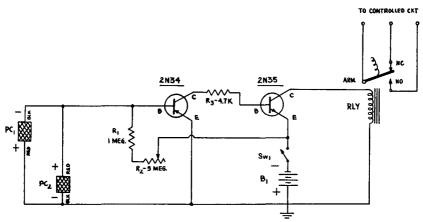
Fig. 10-7.—Schematic of a transistorized "ON-OFF" Light Control circuit.
