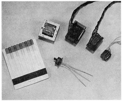
Fig. 3-4.—Subminiature iron-core audio transformers and choke.
