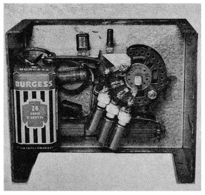
Fig. 9-6.-Interior view of the R.F. Alignment Generator-note crystal mounting.
