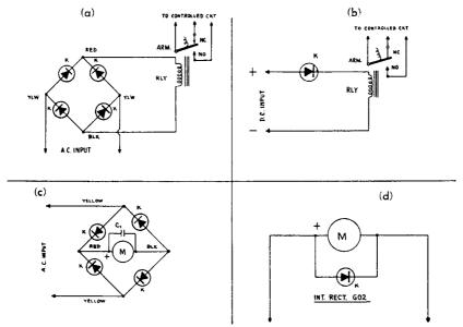
Fig. 10-27.—Semiconductor diode Relay and Meter applications: (a) Sensitive A.C. Relay; (b) Polarized Relay; (c) A.C. Meter; (d) Meter Protection Circuit.
