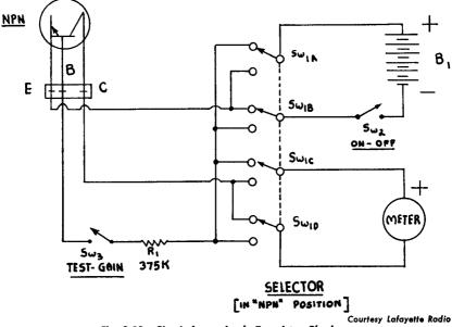
Fig. 9-18.—Circuit for a simple Transistor Checker.
