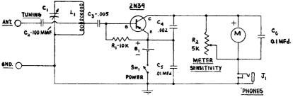
Fig. 8-22.-Circuit for a transistorized R.F. Frequency Meter.
