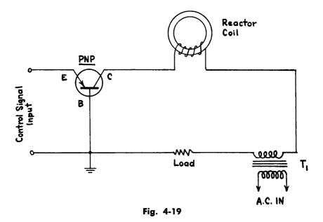
**TRANSISTORIZED MAGNETIC AMPLIFIER** — A number of approaches are open to the designer wishing to transistorize a magnetic amplifier circuit. One such arrangement is shown. Here, a transistor is connected in the grounded-base configuration. In some other application, a grounded-emitter or grounded-collector configuration might be preferred, although a different circuit arrangement would be required.
