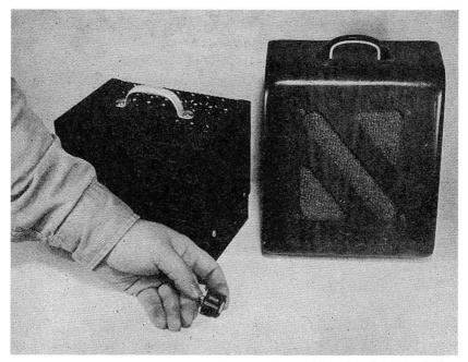
Fig. 7-20.—The transistorized P.A. System, less microphone. The loudspeaker is in the floor baffle to the right, the amplifier itself in the case to the left. The type of power transistor used is shown.
