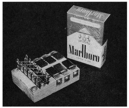
Fig. 10-29.—Easily assembled "Sun Battery" . . . will power a simple receiver, an audio amplifier, or a Code Practice Oscillator, or even a low-power transmitter in full sunlight.
