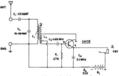
Fig. 8-15.—Circuit for a Wireless Code Practice Oscillator.
