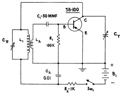
Fig. 8-26.—Schematic of a High Frequency Oscillator featuring a "Surface Barrier" transistor.
