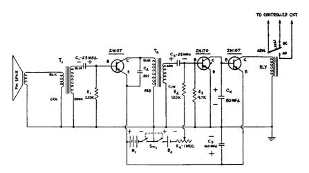
Fig. 10-11.—Circuit of a transistorized Sound Switch or voice-controlled relay.
