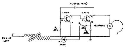
Fig. 8-21.—Schematic of an easily built Ham Station Monitor.
