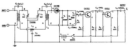
Fig. 8-8.—Diagram of a Hi Fi AM Tuner featuring a transistorized preamplifier.
