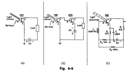
**BASIC PHOTOTRANSISTOR CIRCUITS**—(a) Simple Diode Circuit; (b) Diode with Direct-Coupled Amplifier; (c) Triode Circuit. The grounded-emitter configuration is used in all three circuits. In circuit (a), the phototransistor is used as a simple photoconductive diode; the Load may be a meter or a D'Arsonval type relay.
