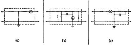
Fig. 12-2.—Three basic equivalent circuits which may be represented as fourterminal networks. (a) T Network; (b) Pi Network; (c) H Network.
