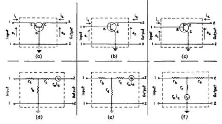
Fig. 12-3.—The three fundamental transistor circuit configurations together with their T network equivalent circuits. The grounded-base configuration is shown at (a) and (d); the grounded-emitter configuration is shown at (b) and (e); the grounded-collector configuration is shown at (c) and (f).
