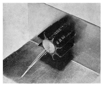
Fig. 2-10.—High-power transistor mounted on a chassis for maximum heat dissipation.
