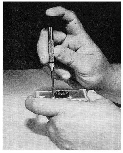
Fig. 2-2.—Proper technique for using a jeweler's screwdriver.
