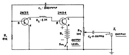
Fig. 9-7.—Circuit for The Signal Squirter.
