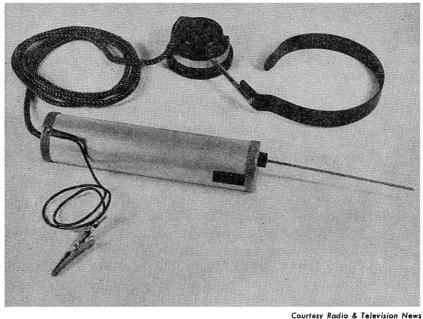
Fig. 9-28.—Author's model of the Signal Tracer.
