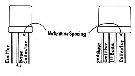
(a) (b) Fig. 2-7.—Pin connections for standard triode (a) and tetrode junction (b) transistors.
