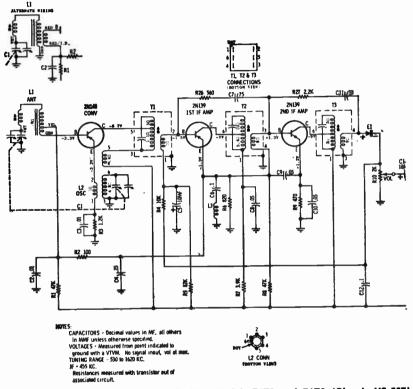
Fig. 14-16.—Circuit diagram of MOTOROLA Models 76T1 and 76T2 (Chassis HS-507). Note that a variety of output connections are used in various production runs af this seven-transistor radio. Manufacturers will frequently make minor circuit changes during production.
