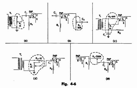
**GAIN CONTROLS** — An input gain control is shown at (a); an output gain control at (b); two types of "constant impedance" controls at (c) and (d); a series type gain control at (e). The actual control circuits are enclosed by dotted lines.
