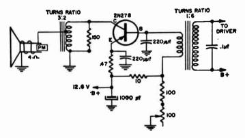
Fig. 14-2.—Typical audio output using a single power transistor. Depending on the transistor used, this type of circuit can deliver from 0.5 to as high as 4.5 watts.
