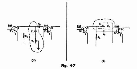
**TONE CONTROLS** – (a) Treble "losser" control; (b) Bass "losser" control. In both circuits, the tone control network is enclosed by a dotted line. In circuit (a), coupling capacitor Cc has a normal value,  $C_1$  may have a value as low as 0.01 mfd to as large as 0.5 mfd, depending on circuit requirements, and  $R_1$  may have a value from 5K to 50K.
