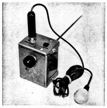
Fig. 7-6.—Exterior view of the electronic "Stethoscope"
