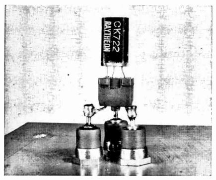
Fig. 2-5.—Detail of transistor socket mounting.
