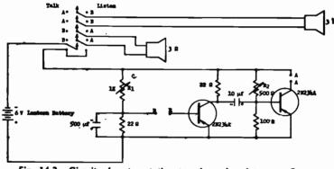
Fig. 14-3.—Circuit of a two-station transformerless Intercom, Output level is approximately 1/5 watt.
