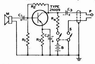
Fig. 14-1.—Single-stage microphone preamplifier — used with a magnetic cartridge or small loudspeaker, this circuit provides an output level comparable to that obtained from a carbon microphone.
