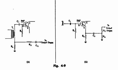
**OVERALL FEEDBACK** — (a) Series type base-coupled; (b) Emitter-coupled. As with vacuum tube audio amplifiers, the over-all frequency response may be improved and distortion reduced if inverse feedback is used between the output and input stages of a multi-stage transistor amplifier.
