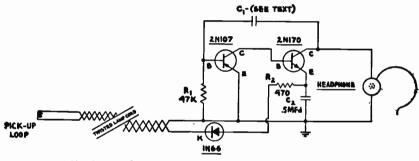
ig. 8-21.—Schematic of an easily built Ham Station Monitor.
