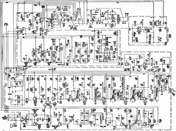
Fig. 14-18.—Circuit of PHILCO'S "Safari" portable television receiver. This fully transistorized set uses a small cathode ray tube and employs a special optical system to enlarge the image. It may be operated either from an A.C. line or from its own rechargeable batteries.
