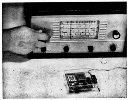
rig. 6-19.—Checking the dial calibration of a communications receiver.
