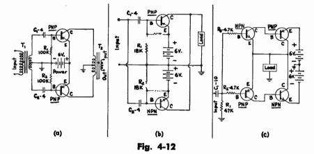
**PUSH-PULL CIRCUITS** – (a) Conventional; (b) Complementary Symmetry; (c) Cascaded Complementary Symmetry. Circuit (a) is a conventional transformer-coupled push-pull amplifier employing transistors of the same type. The general arrangement is quite similar to its vacuum tube counterpart. D.C. stabilization is not provided in the circuit shown, although it is recommended in power applications (see Fig. 4-4).
