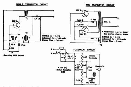
Fig. 14-25.—Schematic diagrams of typical transistorized photoflash circuits. Basically, the transistar serves in a D.C. to D.C. CONVERTER, charging a high-voltage capacitor fram a low-voltage source.
