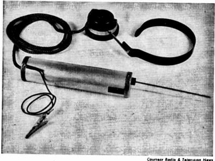
Fig. 9-28.—Author's model of the Signal Tracer.
