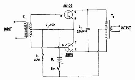
Fig. 7-2.-Basic Push-Pull Power Amplifier.
