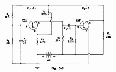
WIEN BRIDGE (R-C) OSCILLATOR – A transistorized version of a standard vacuum tube Wien Bridge audio oscillator is shown. Only the basic circuit is illustrated and, therefore, no provision has been made for D.C. stabilization, output amplitude stabilization, or for minimizing waveform distortion at different frequencies. However, such refinements would be desirable in a commercial version of the circuit. The grounded-emitter configuration is employed.
