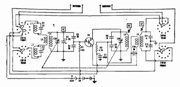
Fig. 14-21.—Circuit of REGENCY'S Model RC-103 FM TeleVerter. This interesting device permits the reception of FM Broadcast Band stations through any standard TV set.
