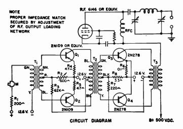
Fig. 14-20.—Wiring diagram of a 25 watt modulator designed for use in a tubeoperated Radiotelephone transmitter. As power R.F. transistor become available in quantity, fully transistorized radio trasmitters will become feasible.
