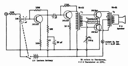
Fig. 14-4.—Schematic diagram of a phonograph amplifier. Designed for use with a crystal or ceromic pick-up, this omplifier delivers good room volume, but requires relatively little bat(ery power, insuring long battery life.
