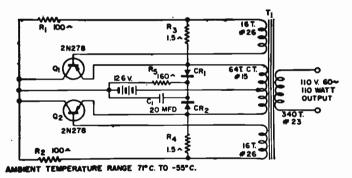
Fig. 14-22.—Schemotic of a typicol tansistorized INVERTER. This type of unit converts D.C., obtained, say, from a storage battery, to A.C. for the operation of line-powered equipment.
