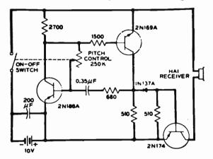
Fig. 14-19.—Schematic diagram of BELL LABS' "Electronic Larynx," a special device for individuals who have last their vacal cards through accident ar diseases.
