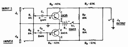
Fig. 7-17.—A transistorized 2-Channel Audio Mixer.
