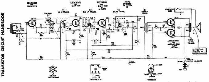
Fig. 14-14. — Circuit of WESTINHOUSE Models H-655P5 and H-656P5 receivers. These five-transistor sets feature a push-pull output stage, and a reflexed I.F. amplifier.
