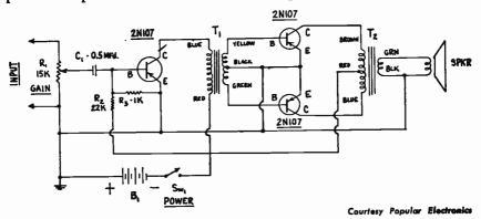
Fig. 7-10.—Circuit of the Geigamp . . . a Geiger Counter amplifier.
