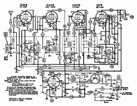
Fig. 14-9.—Wiring diogram of the PONTIAC Model 988671 outomobile rodio. A "hybrid" receiver using five tubes and a single transistor, this set was manufactured by DELCO.
