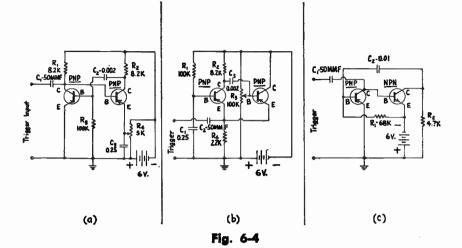
**MONOSTABLE CIRCUITS** — (a) Collector-Coupled; (b) Emitter-Coupled; (c) "Complementary Symmetry" Collector-Coupled. All three circuits are direct adaptations from corresponding multivibrator circuits.
