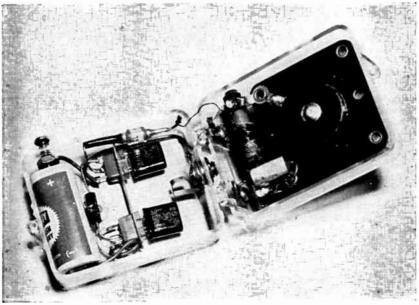
Fig. 8-7.—Interior view of the Pocket Receiver.
