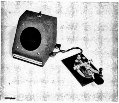
Fig. 10-14.—Loudspeaker type Code Practice Oscillator.
