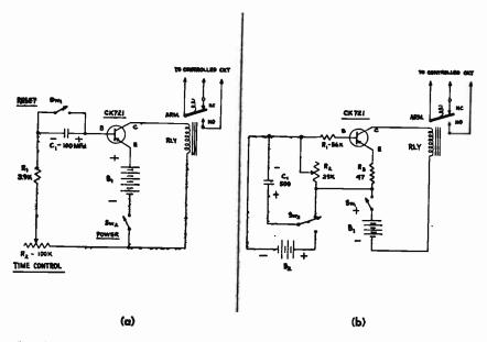
Ry. 10-1.—Two simple transistorized Timers: Circuit (a) operates on the "charge" cycle of a capacitor, circuit (b) on the "discharge" cycle.
