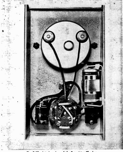
Fig. 9-20.—Interior view of the Transistor Checker.
