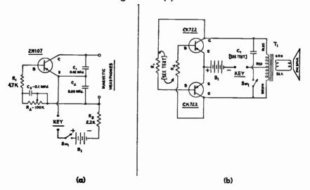
Hy. 10-12.—Diagrams for two easily built Code Practice Oscillators—(a) Headphone type; (b) Loudspeaker type.
