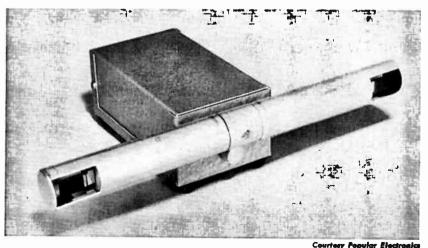
fig. 10-8.—Author's model of the "ON-OFF" Light Control.
