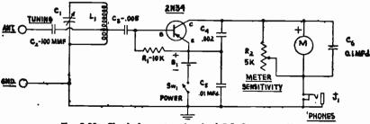
ig. 8-22.—Circuit for a transistorized R.F. Frequency Meter.
