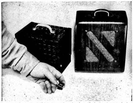
Fig. 7-20.—The transistorized P.A. System, less microphone. The loudspecker is in the floor baffle to the right, the amplifier itself in the case to the left. The type of power transistor used is shown.
