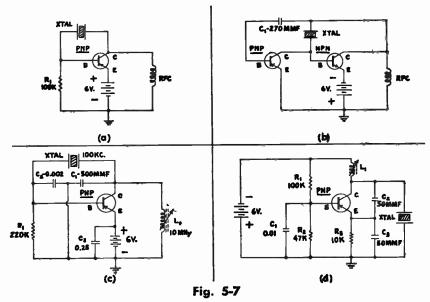
**CRYSTAL-CONTROLLED OSCILLATORS** — (a) Basic circuit; (b) Complementary-Symmetry circuit; (c) Modified grounded-emitter circuit; (d) Groundedbase configuration. The circuits shown represent but four of a large number of possible crystal-controlled transistor oscillators. Almost every vacuum
