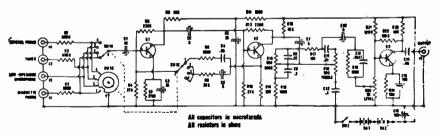
Fig. 14-7.—Schematic diagram of REGENCY'S Model HFT-1 Preamplifier-Equalizer. Designed for use with a High Fidelity power amplifier, this unit has four inputs and provides proper compensation for a variety of phonograph cartridges.
