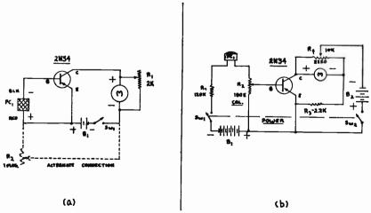
Fig. 9-34.—Two Light Meter circuits—(a) Basic circuit using a selenium photocell and (b) Basic circuit using a Cadmium Sulfide photocell.
