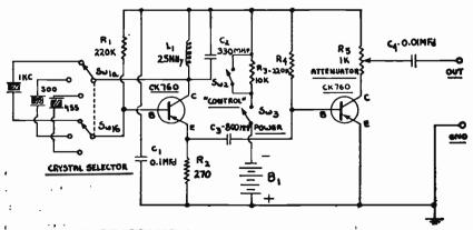
Fig. 9-4.—Schematic diagram of an R.F. Alignment Generator.
