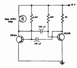
Fig. 14-27.—A transistarized LIGHT FLASHER circuit. Such circuits are used extensively in the manufacture af warning and safety light systems.
