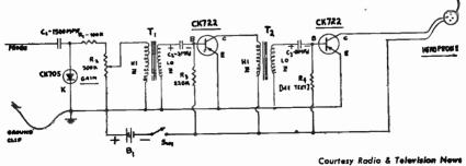
Na. 9-27.-Schematic diagram of a transistorized Signal Tracer.
