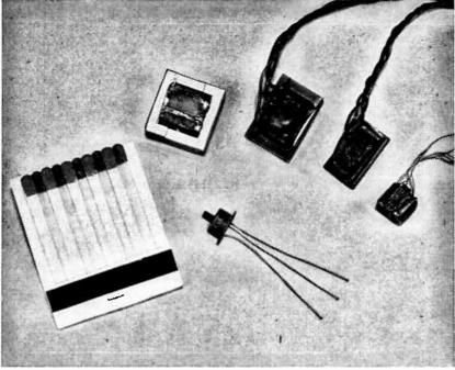
Fig. 3-4.—Subminiature iron-core audio transformers and choke.
