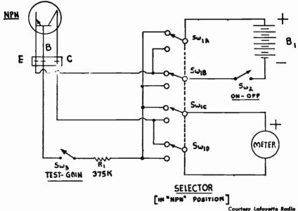
Fig. 9-18.—Circuit for a simple Transistor Checker.
