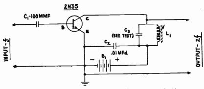
Fig. 8-24.—Diagram of a basic transistorized R.F. Frequency Doubler.
