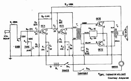
Fig. 7-23.—Circuit of a high quality transistorized Phonograph Amplifier. This unit might also be used as a Guitar or similar "Music" amplifier, or even as a low power P.A. system. designed primarily for use in a portable record player, the amplifier is also suitable for use as a musical instrument amplifier if a suitable pick-up is substituted for the phonograph cartridge. It might also serve as the *audio section of* a transistorized receiver or as a "loudspeaker booster" for a crystal set.
