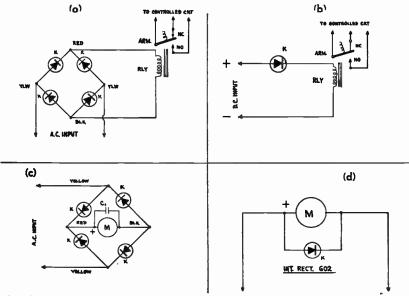
**Fig. 10-27**.—Semiconductor diode Relay and Meter applications: (a) Sensitive A.C. Relay; (b) Polarized Relay; (c) A.C. Meter; (d) Meter Protection Circuit.
