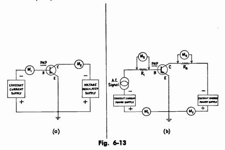
**BETA MEASUREMENT** — (a) Static Measurement; (b) Dynamic Measurement. Beta is the current amplification factor of a transistor in the grounded-emitter configuration and may be defined as the ratio of the change in collector
