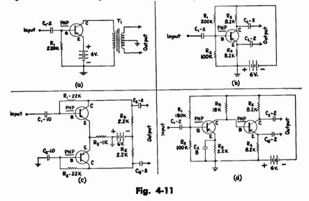
**PRACTICAL PHASE INVERTERS** — (a) Transformer type; (b) Split-load type; (c) Emitter-coupled type; (d) Split-load type direct-coupled to a grounded-emitter amplifier.
