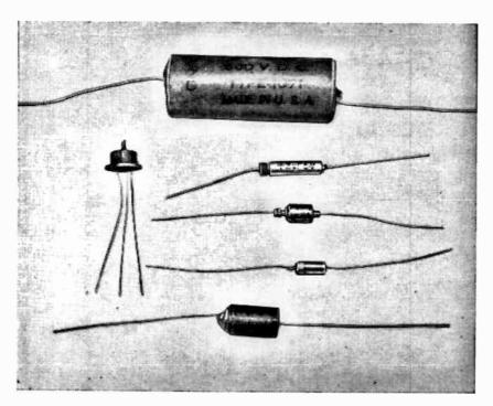
Fig. 3-2.—Subminiature electrolytic capacitors compared to a standard paper unit.
