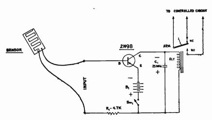
Fig. 10-4.--"Rain Alarm" circuit
