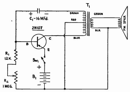
Fig. 10-16.—Schematic diagram of a transistorized Metronome.
