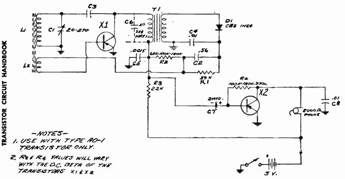
Fig. 14-12.—Schematic of REGENCY'S Model XR-2A Pocket Receiver. This Broadcast Band receiver features a regenerative R.F. stage, reflexed to serve as an audio amplifier.
