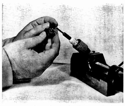
Fig. 2-3.—Some technicians prefer to clamp their soldering instrument in a vise.
