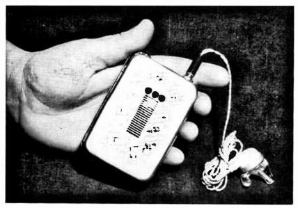
Fig. 7-4.—Hearing Aid assembled in a small metal box
