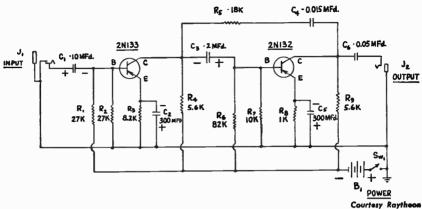
Fig. 7-21.—Circuit of a transistorized Hi Fi Preamplifier
