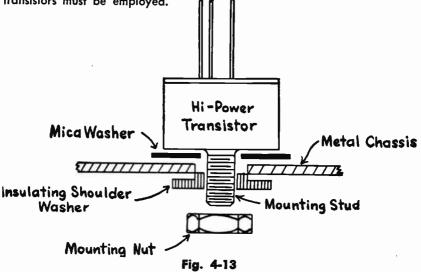
**POWER AMPLIFIERS** – A typical mounting for a "high power" transistor is shown. In order to improve heat dissipation, power transistors are frequently assembled in a metal case which serves as a heat radiator. This case, in turn, may be mounted on a metal chassis to provide a "heat sink".
