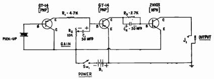
Fig. 7-5.-- A transistorized electronic "Stethoscope".
