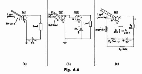
**BASIC PHOTOTRANSISTOR CIRCUITS**—(a) Simple Diode Circuit; (b) Diode with Direct-Coupled Amplifier; (c) Triode Circuit. The grounded-emitter configuration is used in all three circuits. In circuit (a), the phototransistor is used as a simple photoconductive diode; the Load may be a meter or a D'Arsonval type relay.
