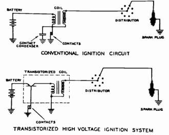
Fig. 14-26: Here, "conventional" and transistorized automobile ignition circuits are compared.
