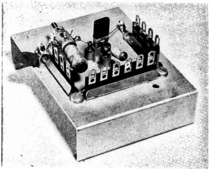
Fig. 8-25.—Breadboarded Frequency Doubler.
