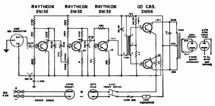
Fig. 14-5.—Circuit of the BOGEN Model BT12 transistorized P.A. Amplifier. With an output of 4 watts, this amplifier is designed for use with a moderate impedance (200 to 500 ohm) microphone.
