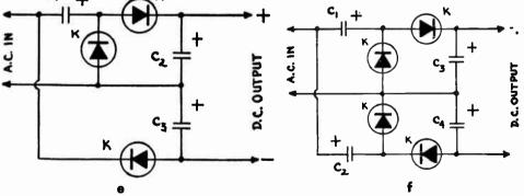
Fig. 10-20.—Basic semiconductor diode Rectifier circuits: (a) Holf-Wave; (b) Full-Wave; (c) Full-Wave Bridge; (d) Voltage-Doubler; (e) Voltage-Tripler; (f) Voltage-Quadrupler.
