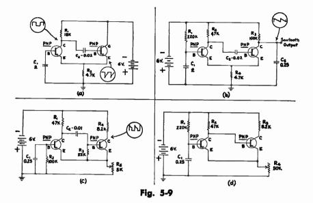
**EMITTER-COUPLED MULTIVIBRATORS** — (a) Basic Emitter-Coupled circuit; (b) Sawtooth waveform circuit; (c) Adjustable stability circuit; (d) Directcaupled circuit. The emitter-coupled transistor multivibrator is roughly analogous to the cathode-coupled vacuum tube multivibrator.
