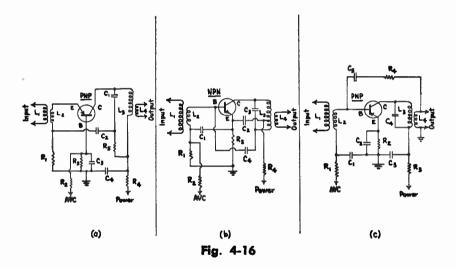
**NEUTRALIZATION METHODS**—(a) Grounded-base amplifier; (b) Groundedemitter amplifier with primary feedback; (c) Grounded-emitter amplifier with secondary feedback. In all three circuits, it is assumed that the transistors are used as receiver R.F. or I.F. amplifiers and hence a source of AVC current is indicated; however, similar techniques may be used with power amplifiers.
