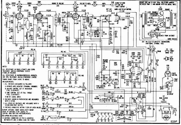
Fig. 14-11.—Circuit diagram of BENDIX'S Model R85BHP car radio. This set was designed for installation in 1958 Lincoln cars and is equipped with a transistorized push-pull power amplifier. As in other hybrid receivers, vacuum tubes are used in the R.F and I.F. stages.
