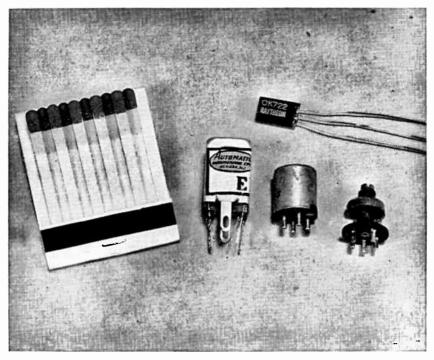
Fig. 3-3.—Subminiature R.F. coils and I.F. transformers.
