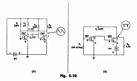
**COLLECTOR-COUPLED MULTIVIBRATORS** — (a) Basic Collector-Coupled Circuit; (b) Complementary-symmetry circuit. Circuit (a) is a transistorized version of the familiar plate-coupled vacuum tube multivibrator, but circuit (b) is unique to transistor circuitry—there is no analogous vacuum tube arrangement, for circuit (b) utilizes the complementary symmetrical characteristics of transistors of different types.
