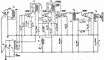
Fig. 8-11.—Schematic diagram of a four-transistor Superheterodyne Receiver.
