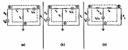
Fig. 12-4.—The three fundamental transistor circuit configurations shown as their operating I network equivalent circuits. The emitter, base, and collector connections are identified outside the dotted box, which represents the transistor proper. The grounded-base configuration is shown at (a), the grounded-emitter configuration at (b), and the groundedcollector configuration at (c).
