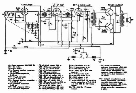
Fig. 14-8.—Circuit of a typical "hybrid" portable receiver. Using both tubes and transistors, this type of receiver was popular until low-cost R.F. transistors became available in quantity.
