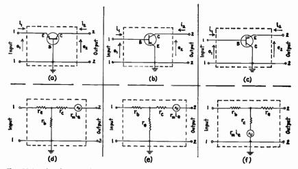
Fig. 12-3.—The three fundamental transister circuit configurations together with their T network equivalent circuits. The grounded-base configuration is shawn at (a) and (d); the grounded-emitter configuration is shown at (b) and (e); the grounded-collector configuration is shown at (c) and (f).
