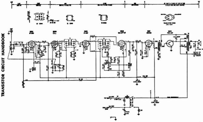
Section 14-10.—Schematic of MOTOROLA'S Model 75MF car radio. Designed for use in 1957 Ford automobiles, this popular hybrid receiver features both manual and push-button tuning.
