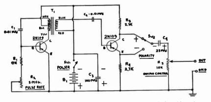
Fig. 9-13.—Circuit of a transistorized Pulse Generator delivering both positive-going and negative-going pulses.
