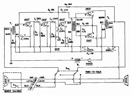
Fig. 7-13 .-- A transistorized two-station intercom.
