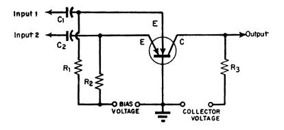
Figure 6-6. A mixer or modulator circuit suitable for use with a point-contact tetrode transistor. The tetrode transistor has two emitter terminals. CREDIT, Circuit Courtesy SYLVANIA.
