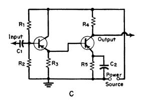
Figure 6-1. Three useful transistor circuits. A d.c. amplifier is shown at A; an R.F. detector or Sine-wave Clipper at B; and a two-stage direct-coupled amplifier at C.
