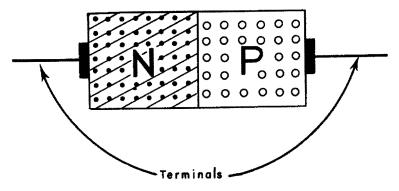
Figure 2-1. Schematic representation of an N-P junction of semi-conductor material Such a junction is made up of a single piece of material (a single crystal), but with the ends having different electrical characteristics.
