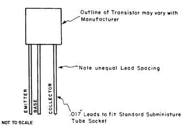
Figure 3-1. The presently accepted "standard" for lead connections of triode transistors. The pin size and spacing is chosen so as to permit the use of a standard 5- or 7-pin "in line" subminiature tube socket. Some manufacturers supply their transistors with long leads to permit the units to be wired directly into a circuit ... these leads are cut short where a socket is employed.
