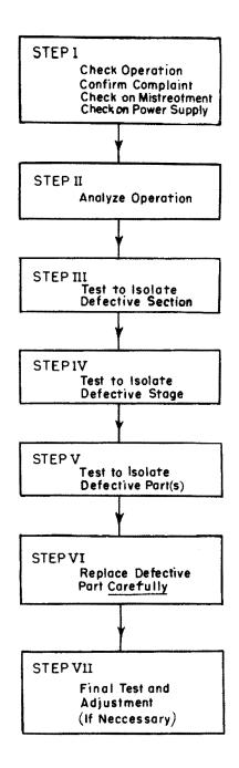
Figure 8-1. A block diagram illustrating the steps to be followed when servicing transistorized equipment. The same steps are followed, generally, when servicing all types of electronic equipment.
