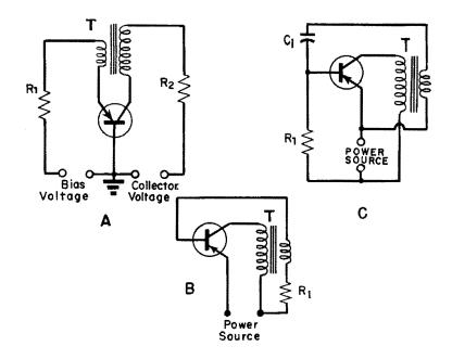
Figure 5-1. Three basic "tickler feedback" transistor oscillator circuits. The grounded base circuit is shown at A; grounded emitter circuits are shown at B and C. Power supply voltage polarities are not shown, as these will depend on the type of transistor employed.
