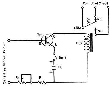
Figure 9-7. A sensitive Relay Circuit. Parts values are as follows:
