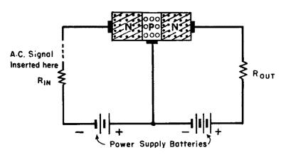
Figure 2-2. Schematic representation of an NPN junction transistor, showing power supply connections and input and output load resistors.
