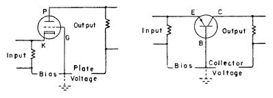
Figure 4-3. Grounded grid triode tube connections (left) and grounded base connections for a transistor (right). Note that these circuits are analogous, but not equivalent.
