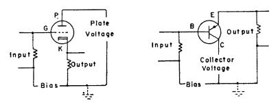
Figure 4-4. Grounded plate(cathode follower) circuit for a triode vacuum tube(left) and the grounded collector circuit for a transistor (right). Both circuits are used primarily for impedance matching.
