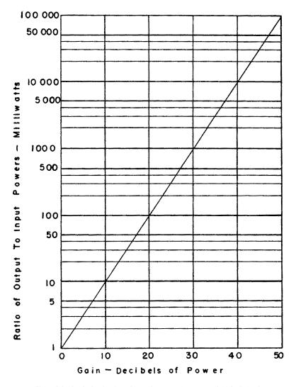
Figure 4-6. Graph showing the relations between gains measured in decibels of power and in ratios of output to input milliwatts. This chart may also be used to compare db gain for other power units.
