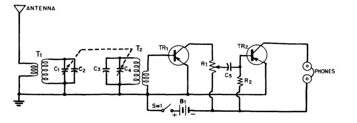
Figure 9-6. A simple broadcast band receiver using two transistors. Parts value are listed below.
