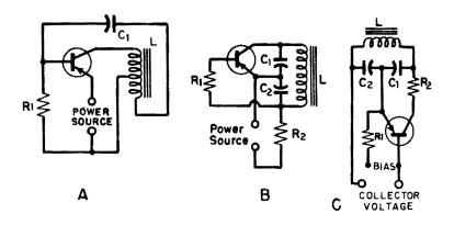
Figure 5-2. Three additional transistor oscillator circuits. The circuit shown at A is somewhat analogous to a vacuum tube " $H_{\rm B}$ rtley" oscillator, while those shown at B and C are similar to the vacuum tube "Colpits" oscillator. Grounded emitter circuits are used at A and B, and a grounded base circuit at C.
