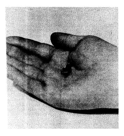
Figure 7-2. A standard "in-line" sub-minature tube socket may be used for all transistors employing the standard lead connections. This photo shows the small size of the socket and transistor... the transistor shown is a point-contact unit.
