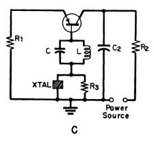
Figure 5-4. Three common base oscillator circuits which are suitable for use with point-contact transistors only. The circuit shown at C is crystal-controlled.
