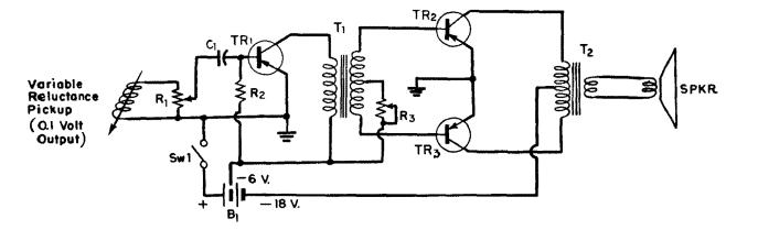
Figure 9-2. A transistor-operated phonograph amplifier. Parts values are as follows:
