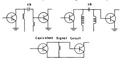
Figure 4-8. Resistance-capacity and impedance coupling techniques, as applied to transistor amplifiers, are illustrated in this sketch. If  $C_b$  is large and offers alow reactance at the signal frequencies, the Equivalent Signal Circuit shown applies. Since no special provision is made for matching the input and output impedances of the coupled stages, the efficiency of such circuits is low.
