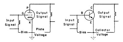
Figure 4-2. Grounded cathode circuit for a vacuum tube (left) and the grounded emitter circuit for a transistor (right). While the plate voltage of the vacuum tube will always be positive with respect to its cathode, the voltage polarities in the transistor circuit will depend on the type of transistor used.
