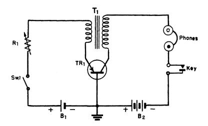
Figure 9-1. A transistor code practice oscillator. Parts values are as follows:
