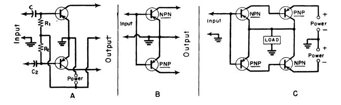
Figure 6-3. Push-pull transistor circuits. The circuits shown at B and C require but a single-ended input signal. The circuit shown at C can drive a low impedance load directly.
