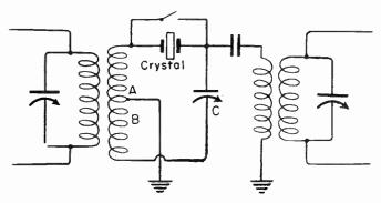
Fig. 27.—Crystal Used in Intermediate-frequency Amplifier.
