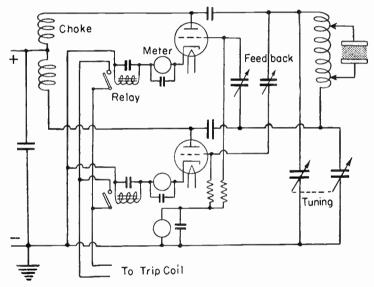
Fig. 3.—Typical Circuit for Electrostatic Heating.
