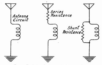
Fig. 2.—Equivalent Resistances in Antenna Circuit.
