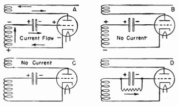
Fig. 1.-Action of Blocking Due to Charge on Grid Condenser.
