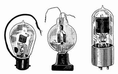
Fig. 1.—Early Experimental Types of Vacuum Tubes
