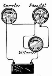
Fig. 1.—Determining Rheostat Resistance with Ohm's Law.
