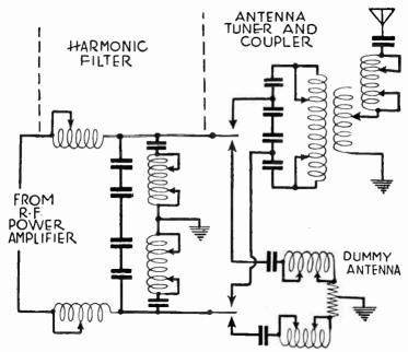
Fig. 10.—Antenna System and Harmonic Filter.
