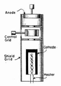
Fig. 1.—Element Arrangement in Heavy-duty Four-element Thyratron.
