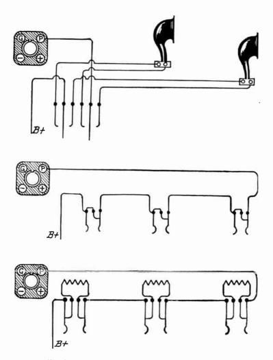
Fig. 6, Jacks for Connection of Several Speakers.
