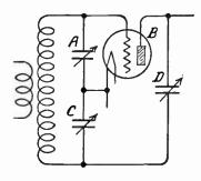
Fig. 7.—The Isofarad Method of Balancing.
