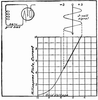
Fig. 1.—Effect of Zero Grid Bias, Distortion.
