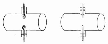
Fig. 2.—Energy Transfer Probes for Cavity Resonator.
