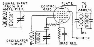
Fig. 25.—Complete Pentagrid Converter Connections.
