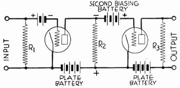
Fig. 2.-Two-Stage Direct Current Amplifier.
