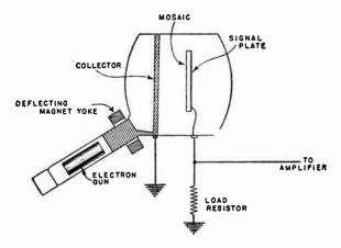
Fig. 4.—Circuit for Signal Current in the Iconoscope.
