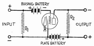
Fig. 1.—Simple Form of Direct Current Amplifier.
