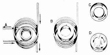
Fig. 1.—Elementary Principle of Induction Heating.
