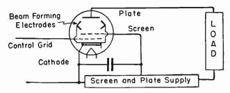
Fig. 3.—Circuit Connections to a Beam Power Tube.
