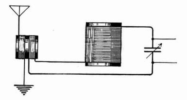
Fig. 2.—Separate Coupling Coil for Antenna Circuit.
