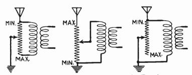
Fig. 13.—Antenna Circuit Volume Controls for Transformers.
