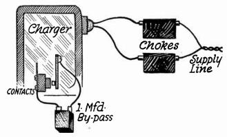
Fig. 5.—Handling Interference of Vibrators and Flashers.
