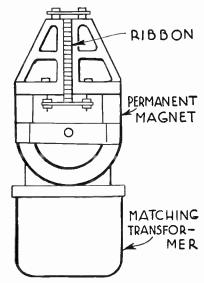
Fig. 1.—Constructional Details of Velocity Microphone,
