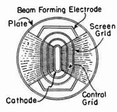
Fig. 1.—Element Arrangement in Beam Power Tube.
