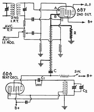
Fig. 10.-Beat Frequency Oscillator Circuit
