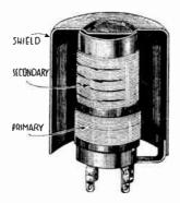
Fig. 2.-Shielded Radio Frequency Transformer.
