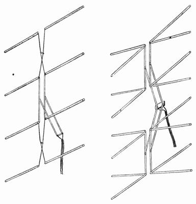
Fig. 13.—Connections for stacked antennas with four bays.
