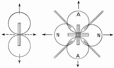
Fig. 4.—Radiation from Loop Antennas.
