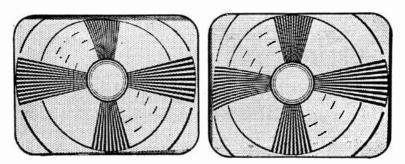
Fig. 34.—Effects of Wrong Adjustment of Linearity Controls.
