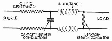
Fig. 4.—Electrical Elements of Transmission Line.
