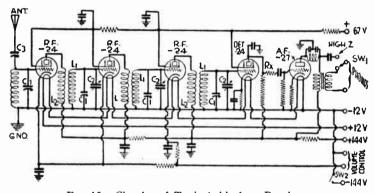
Fig. 15.—Circuits of Typical Airplane Receiver.
