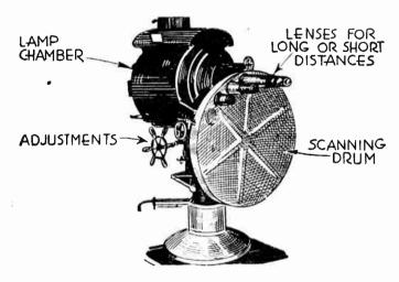
Fig. 6.—Television Scanner Employing an Arc Lamp.
