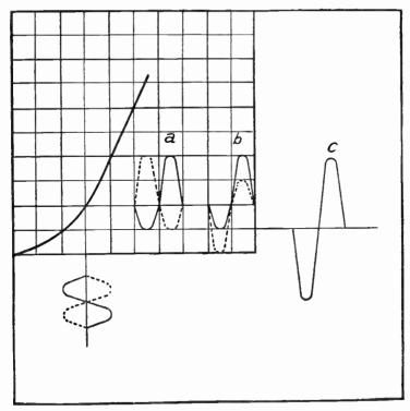
Fig. 4.—Balancing Unequal Changes of Plate Current.
