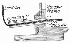
Antenna Lead-in Carried Through Tube.
