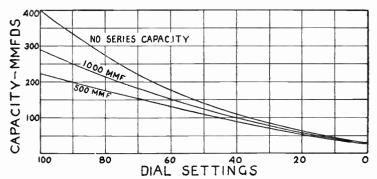
Fig. 22.—How Series Capacities Affect the Tuning.
