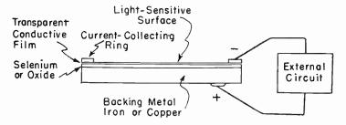
Fig. 1.—Principal Parts of Barrier Layer Photocells.
