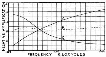
Fig. 4.—Effect of Primary Frequency on Amplification.
