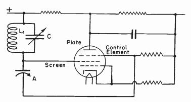
Fig. 8.—Negative Transconductance Oscillator.
