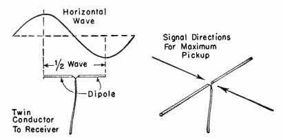
Fig. 14.—Half-wave Dipole Antenna.
