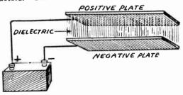
Fig. 2.—The Plates and Dielectric of a Condenser
