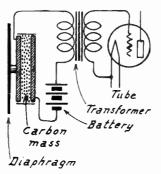
Fig. 1.—Simple Type of Microphone.
