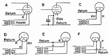
Fig. 2.—Returns for Heater-cathode Type Tubes.
