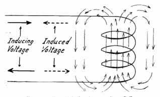
Fig. 1.—Effect of Self-Inductance in a Coil.
