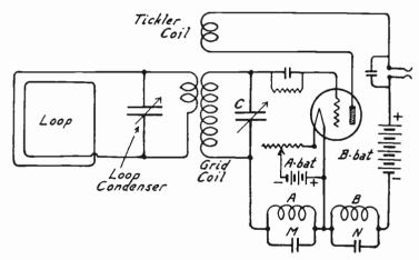
Circuits of Super-Regenerative Single Tube Receiver.
