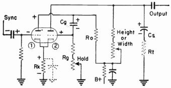
Fig. 27.-Multivibrator Oscillator for Television Sweep Circuits.
