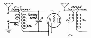
Fig. 1.—Antenna Connections for Testing Radio Stages.
