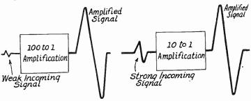
The Effect of Amplification on Signal Strength.
