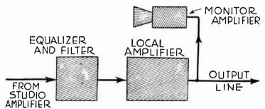
Fig. 4.-Equipment at Repeater Station.
