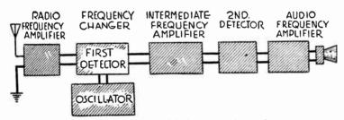
Fig. 3.—Elements of a Modern Superheterodyne.
