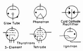
Fig. 1.—Symbols for Gas-filled Tubes.
