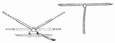
Fig. 15.—Two types of indoor antennas.
