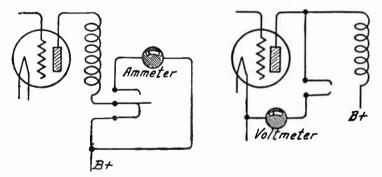
Fig. 4.—Meter Connections Made with Switches.
