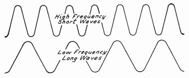
Fig. 2.—Frequency Relation to Wavelength.
