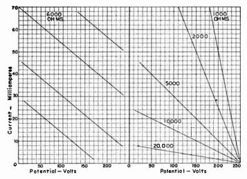
Fig. 2.—Load Lines for 6,000 Ohms Resistance.
