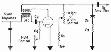
Fig. 26.—Blocking Oscillator Used in Sweep Circuits.
