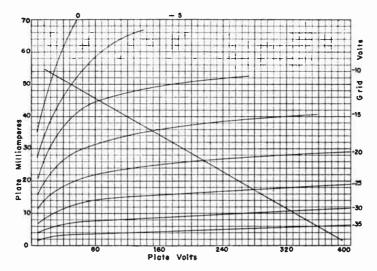
Fig. 5.—Plate Characteristics of a Power-amplifier Pentode. The Load Line 1s for 7,000 Ohms Load Resistance.
