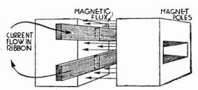
Fig. 8.—Magnetic Action in Light Valve.
