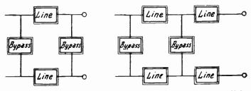
Fig. 11.—Filters Composed of Multiple Line Units and Bypass Units.
