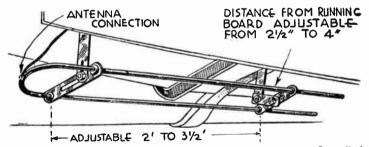
Fis. 4.—Folded Doublet or Di-pole Automobile Antenna Installed under Running Board.
