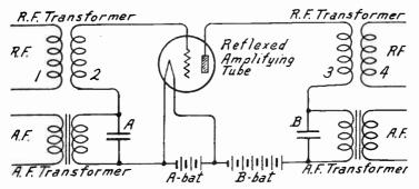
Fig. 2.—Circuits of Reflexed Amplifying Tube.
