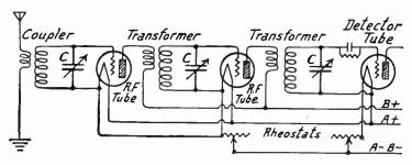
Radio Frequency Circuits of Tuned Radio Frequency Receiver.
