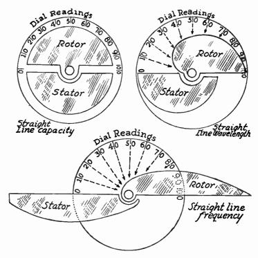
Fig. 5.—Basic Forms of Condenser Rotor Plates.
