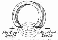
Fig. 1.—The Poles and Field of a Magnet.
