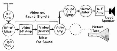
Fig. 23.—Path of Signal in Intercarrier Sound System.
