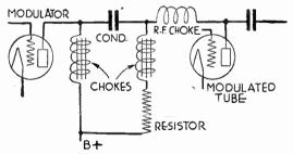
Fig. 13.—Separate Chokes for Modulator and Oscillator.
