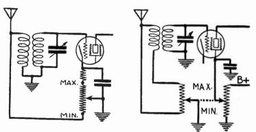
Fig. 20.—Dual Control with One Fig. 21.—Twin Control for Antenna Potentiometer. and Screen Voltage.
