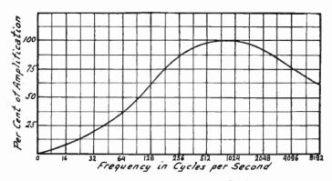
Fig. 3.--Amplification Curve of a Poor Audio Transformer.
