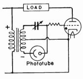
Fig. 10.—Phase-shift Control by Means of a Vacuum Triode Connected to a Bridge Rectifier.
