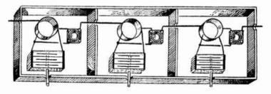
Fig. 5.—Amplifying Stages Enclosed in Individual Shields.
