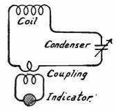
Fig. 1.—The Simplest Frequency Meter Circuit.
