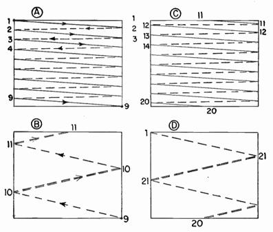
Fig. 3.—Travel of Electron Beam for Interlaced Scanning.
