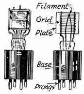
Fig. 1.—Principal Parts of a Triode Having a Filament-cathode.
