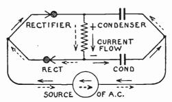
Fig. 2.—Equivalent Circuit for Voltage Doubler.
