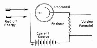
Fig. 3.—The Basic Phototube Circuit.
