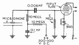
Fig. 2b.—Circuit Connection of Static Velocity Microphone.
