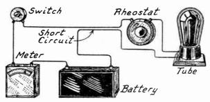
Fig. 2.—Testing for Short Circuit with Voltmeter.
