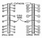
Fig. 2.—Control Grid Spacing in Variable-mu Tube.
