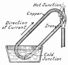
Fig. 1.—Principle of the Thermocouple.
