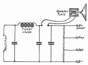
Fig. 6.—Speaker Field Used As a Filter Choke.
