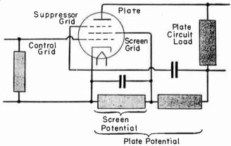
Fig. 2.—Typical Connections for Pentode Voltage Amplification.
