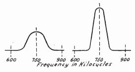
Fig. 3.-Effect of Regeneration on Signal.
