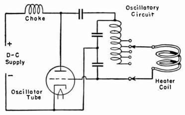
Fig. 2.—Simplified Circuit for Induction Heating.
