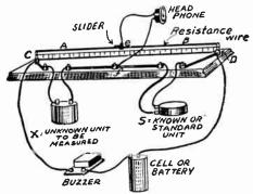
Fig. 5.—Practical Form of Slide Wire Bridge.
