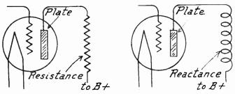
Fig. 2.—Tubes Working into Resistance and Into Reactance for Amplification.
