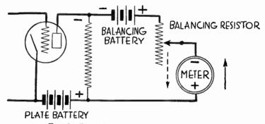
Fig. 3.—Balancing the Plate Resistor Voltage.
