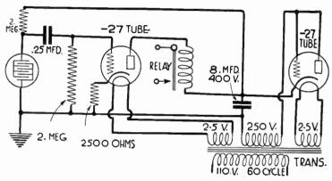
Fig. 7.—Photoconductive Cell Amplifier for Power Line.
