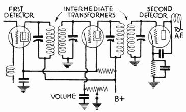
Fig. 14.—Typical Intermediate Frequency Amplifier.
