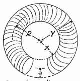
a=winding radius X=inside radius <u>y</u>=2.6 y=outside radius X=2.6 R=mean radius
