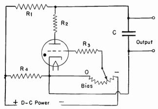
Fig. 6.—Relaxation Oscillator Using Thyratron Tube.
