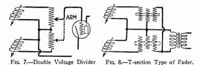
lessens the input voltage to the tube until it is of minimum value. Continued movement of the arm picks up and increases the signal from the lower pickup.
