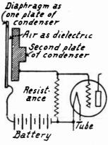
Fig 3.-Condenser Microphone.
