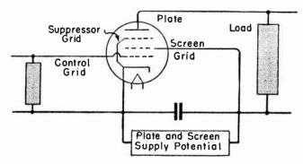
Fig. 3.—Typical Connections for Pentode Power Amplifier,
