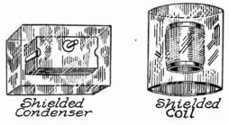
Fig. 4.—Tuning Condenser and Coil Enclosed in Shields.
