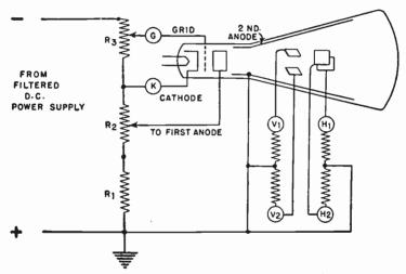
Fig. 4.—Control Circuits for Cathode-ray Tube.
