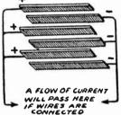
The condition is much the same as if a piece of elastic rubber were either compressed or stretched out between pieces of metal. The strain thus put upon the rubber would cause it to store or contain mechanical energy. This energy in the rubber would tend to return the metal pieces to their original positions as soon as the strain was relieved. The electrostatic strain set up in the material of the dielectric does
