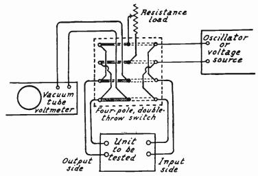
Fig. 8.—Checking Amplifier Unit with VT Voltmeter.
