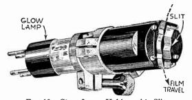
Fig. 10.—Glow Lamp Holder with Slit.
