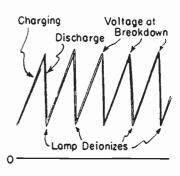
Fig. 4.—Neon Lamp in Relaxation Oscillator.
