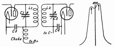
Fig. 3.-Band Selector with Tuned Plate and Tuned Grid Circuits.
