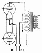
Fig. 3.—D.C. In Output Transformer Primary.
