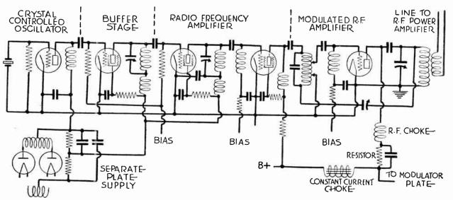
Fig. 8.—Radio Frequency Amplifier at Transmitter.
