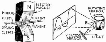
Fig. 2.—Principle of the Duddell Oscillograph.
