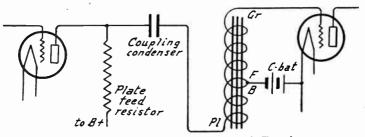
Fig. 11.-Parallel Feed with Resistor and Transformer.
