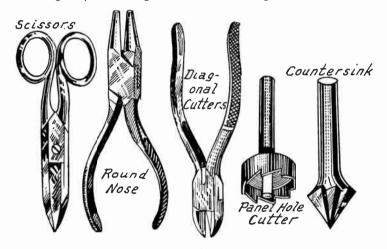
Fig. 2.—Pliers and Cutting Tools.
