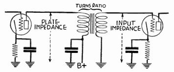
Fig. 2.—Circuit for Transformer Coupling.
