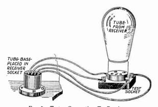
Fig. 7.—Tester Connection To Receiver.
