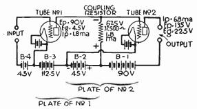
Fig. 1.—Simple Form of Direct Coupled Amplifier.
