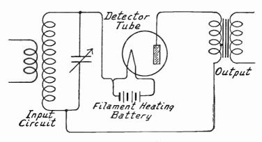
Elementary Principle of Diode Detector.
