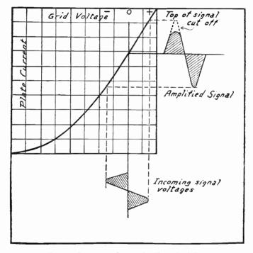
Fig. 2.-Distortion Caused by Zero Grid Bias.
