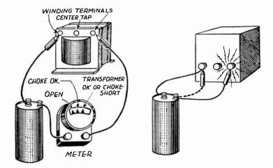
Fig. 14.—Test for Open Circuit or Fig. 15.—Test for Short Circuited Short in Transformer or Choke.
