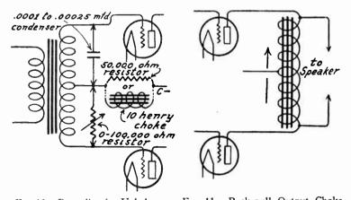
Fig. 10.—Remedies for Unbalance. Fig. 11.—Push-pull Output Choke.
