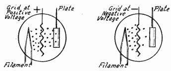
Fig. 3.—Effect of Positive and Negative Grid on Electron Flow.
