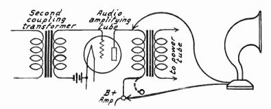
Fig. 5.—Second Test on Audio Amplifier.
