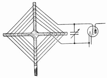
Connections from Spiral Loop to Receiver.
