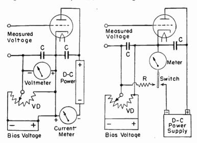
Fig. 3.—Slide Back Instrument Using Two Meters.
