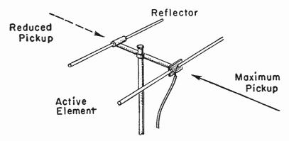
Fig. 15.-Half-wave Dipole with Reflector.
