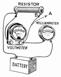
Fig. 18.-Measuring the Resistance of a Resistor.
