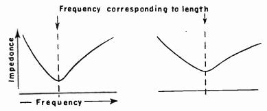
Fig. 3.—Half-wave dipole antennas act like series resonant circuits in their change of impedance with frequency.
