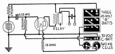
Fig. 6.—Photoconductive Cell Amplifier for Batteries.
