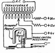
Fig. 2.—Half-wave Vibrating Rectifier.
