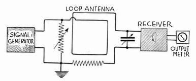
Fig. 12.—Method of Measuring Field Intensity.
