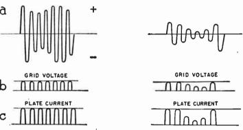
Fig. 4.—How the Limiter Affects a Strong Signal.
