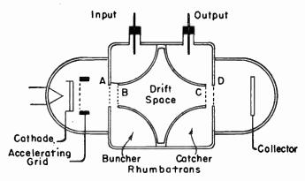
Fig. 1.—Arrangement of Elements in a Klystron.
