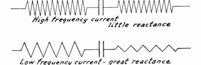
Fig. 5.-Effect of Filter Condensers on High and Low Frequencies.
