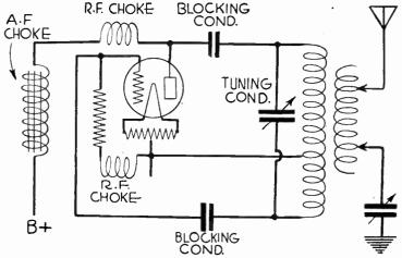
Fig. 3.—Oscillator Coupled to Transmitting Antenna.
