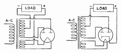
Fig. 3.—Full-wave Filament-cathode Rectifier.
