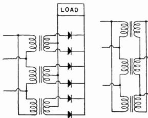
Fig. 4.—Six Elements with Center-tapped Transformer.
