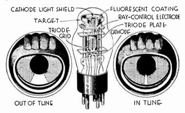
Fig. 13.-Cathode Ray Tuning Meter
