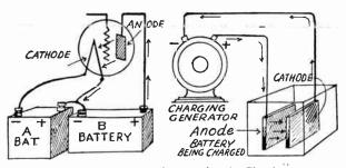
Anodes and Cathodes in Electric Circuits.
