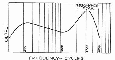
Fig. 9.—Output of Record and Pickup Working Together.
