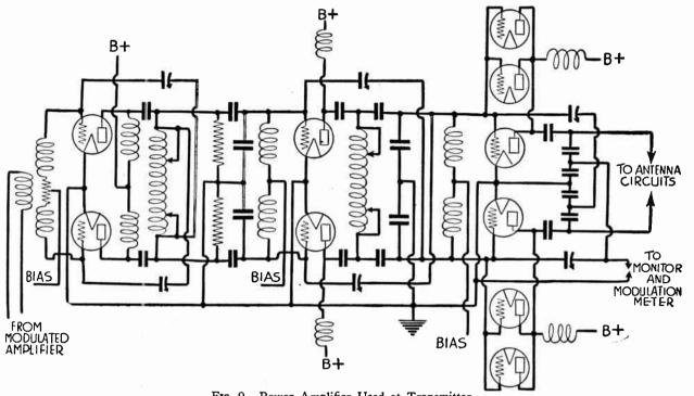
Fig. 9.—Power Amplifier Used at Transmitter.
