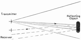
Fig. 3.—The Angle of Reflected Waves Indicates Direction.
