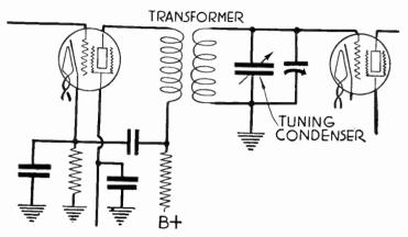
Fig. 1.—Transformer Coupling for Radio Frequencies.
