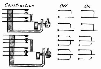
Fig. 2.—Operation of a Jack Switch.
