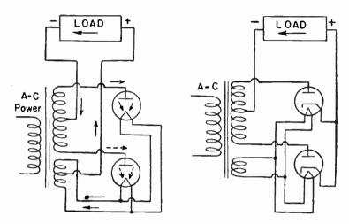
Fig. 1.—Two Filament-cathode Tubes in Full-wave Rectifier.
