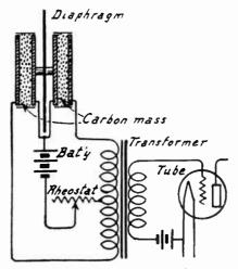
Fig. 2.—Double-button Carbon Microphone.
