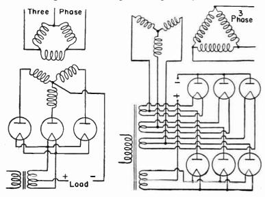
Fig. 1.—Polyphase Half-wave Rectifier.
