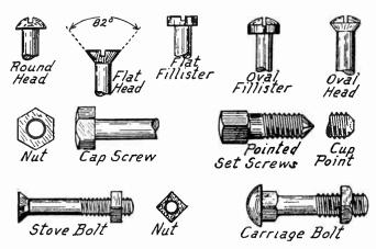
Screws and Bolts Used in Construction Work.
