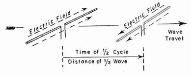
Fig. 1.—Induction of signal currents in a half-wave dipole antenna.
