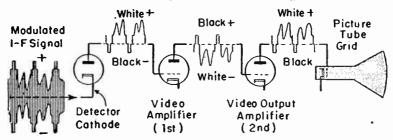
Fig. 21.—Signal Polarities with Two Video Amplifiers.
