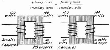
Fig. 7.—A Step-Up Transformer.
