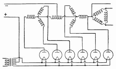
Fig. 3.—Three-phase Double-Y Parallel Rectifier.
