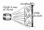
Fig. 2.—Dissipation of Energy in a Conductor Such as a Shield.
