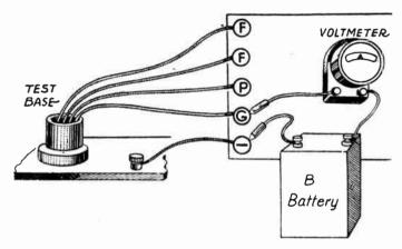
Fig. 10.—Circuit Tests on Receiver.
