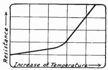
Fig. 3.—Increase of Resistance with Temperature in Iron
