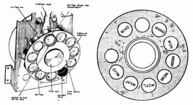
Fig. 6.—Telephone Type Tuning Dial.
