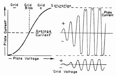
Fig. 3.—The Manner in Which Voltages and Currents Commence and Continue During Oscillation.
