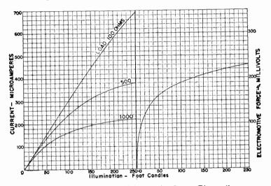
Fig. 2.—Current and Emf in Barrier Layer Photocells.
