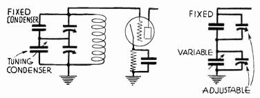
Fig. 21.—Arrangement of Capacities for Oscillator Tuning
