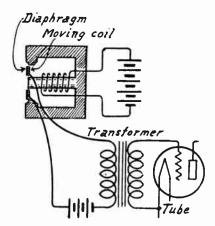
Fig. 4.-Moving Coil Microphone.
