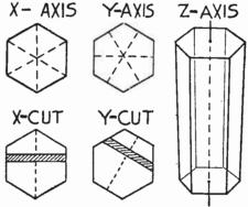
Fig. 2.—Methods of Cutting Quartz Plates.
