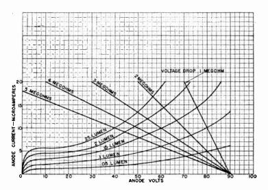
Fig. 9.—Load Lines Showing Phototube Performance.
