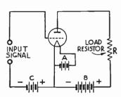
B.—Circuit Connections for Class A Operation.
