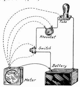
Fig. 2.—Testing Filament Circuit for Opens.
