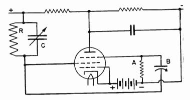
Fig. 9.—Negative Resistance Oscillator Employing Resistancecapacity Circuits.
