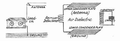
Fig. 2.—The Principle of the Capacity Antenna.
