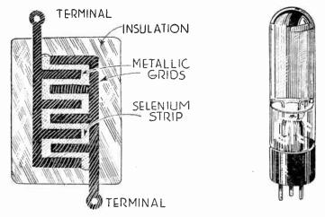
Fig. 1.—Photoconductive Element.
