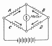
Fig. 5.—Balancing Principle of the Wheatstone Bridge.
