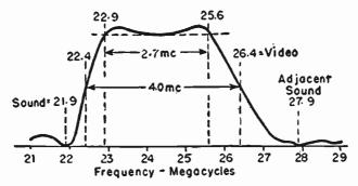
Fig. 13.—Frequency Response of Video I-f Amplifier.
