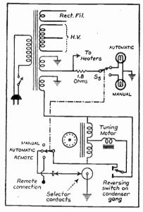
Fig. 2.—Electric Tuning Circuit.
