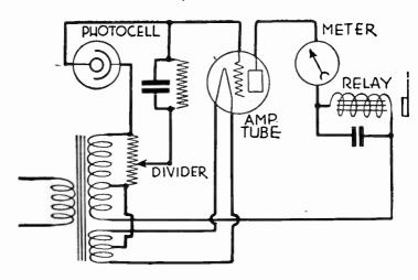
Fig. 11.—The Relay Opens upon Increase of Light.
