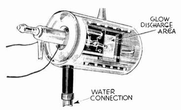
Fig. 7.—High Power Glow Lamp for Television.
