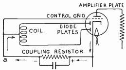
Fig. 2.—Double-diode Triode as Detector and Amplifier.
