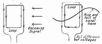
Fig. 2.—Equal Voltages Generated in Both Sides of Loop.
