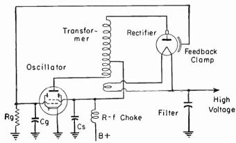
Fig. 38.—High-voltage Supply Using an R-f Oscillator.
