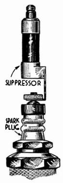
Fig. 10.— Spark Plug Auto Radio Suppressor.
