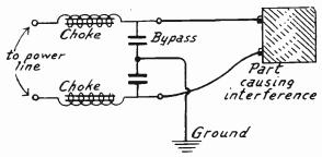
Fig. 8.-Interference Filter with Grounded Center Tap.
