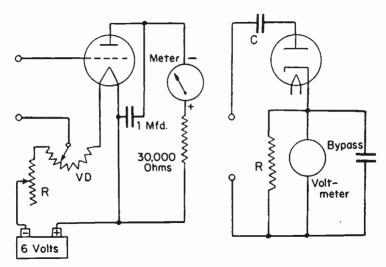
Fig. 5.—Circuit for Moullin Type VT Voltmeter.
