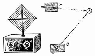
Fig. 1.-Elementary Principle of Radio Compass.
