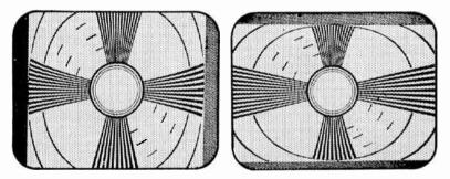
Fig. 31.—Effects of Wrong Adjustment of Height and Width Controls.
