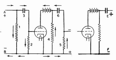
Fig. 2.—Operating Principle of the Multivibrator.
