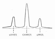
Fig. 7.—Combining the Frequencies in Modulation.
