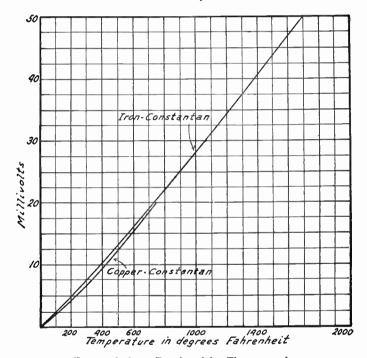
Fig. 2.—Voltage Developed by Thermocouples.
