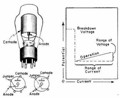
Fig. 1.—Construction and Connections of One Type of Voltage Regulator.
