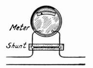
Fig. 4.—Shunt Used with Ammeter.
