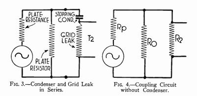
The portion of the first tube's plate voltage variations actually applied to the second tube is called the coupling factor and is found from the following formula:
