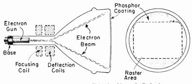
Fig. 5.—Television Picture Tube for Magnetic Deflection.
