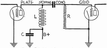
Fig. 1.—Principle of Impedance Coupling.
