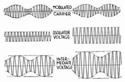
Fig. 12.—How Oscillator Voltage Increases Intermediate Voltage.
