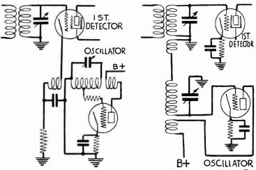
Fig. 10.-Oscillator Coupled to Detector Cathode.
