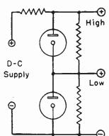
Fig. 3.—Connections Used with Single Regulator Tube.
