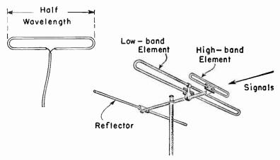
Fig. 16.-Folded Dipole Antenna.
