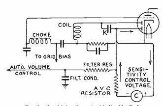
Fig. 5.—Sensitivity Control with Double-diode.
