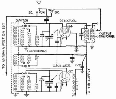
Fig. 8.—Circuit Diagram of Superheterodyne Converter
