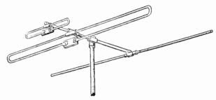
Fig. 11.—High-band and low-band antennas mounted in line with each other.
