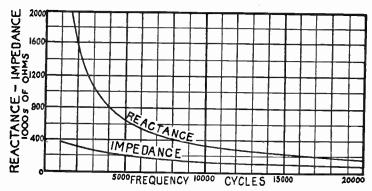
Fig. 8.—Effect of Frequency on Reactance and Impedance.
