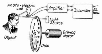
Fig. 1.—Nipkow Disc Scanning at Televisor or Transmitter.
