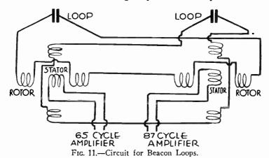
beacon with which are used three modulating frequencies; 65 cycles, 86.7 cycles and 108.3 cycles.
