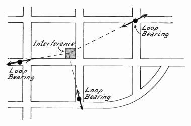
Fig. 2.-Locating Interference with Portable Receiver.
