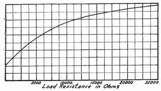
Ftg. 5.—Increase of Power from Tube with Increase of Load When Maintaining Constant Voltage at the Plate Itself.
