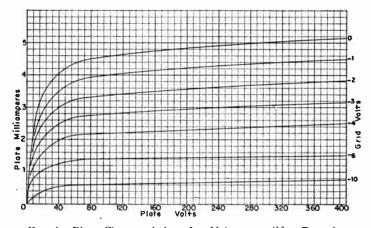
Fig. 4.—Plate Characteristics of a Voltage-amplifier Pentode.
