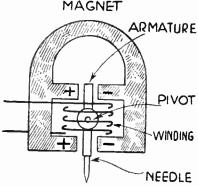
Fig. 7.—Balanced Armature Type of Electromagnetic Pickup.
