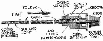
Fig. 5.—Construction at "Dental Cable" Flexible Control Shaft.
