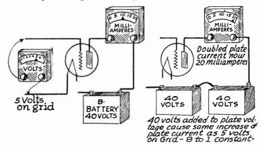
Fig. 1.—The Voltage Amplification of a Vacuum Tube.
