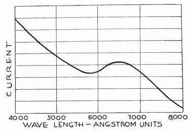
Fig. 5.—Color Sensitivity of Selenium Cell.
