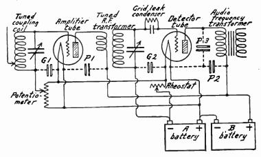
Fig. 2.—Bypass Condensers in a Receiver.
