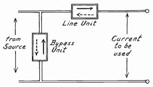
Fig. 10.—Connection of Filter Units in Circuit. Desired Frequencies in Full Line Arrows; Unwanted Frequencies in Broken Line Arrows.
