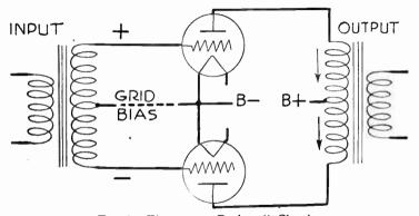
Fig. 1.-Elementary Push-pull Circuit.
