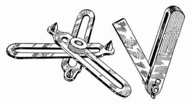
Fig. 1.—Adjustable Template and Adjustable Square.
