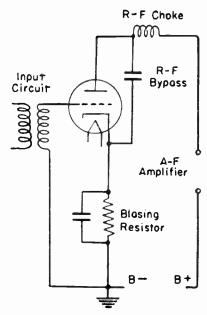
Fig. 2.—Current Change During Plate Current Detection.
