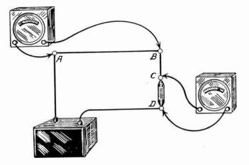
Fig. 1.—Principle of Testing for Open Circuits.
