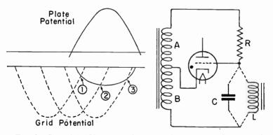
Fig. 6.—Control by Variation of Phase Shift of Grid Potential, with Constant Amplitude.
