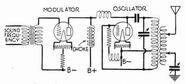
Fig. 6.—Connection of Modulator to Oscillator.
