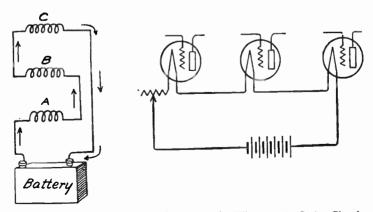
Fig. 1.—A Series Circuit.
