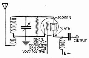
Fig. 7.—Screen Grid Tube as Space Charge Detector
