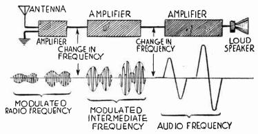
Fig. 1.—The Three Frequencies Used in Superheterodyne Reception.
