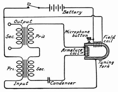
Fig. 2.—Tuning Fork Audio Oscillator.
