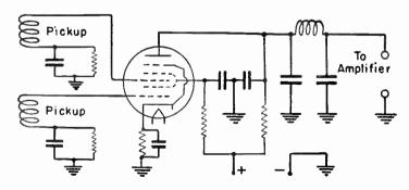
Fig. 2.—Separate Frequencies Combined in Pentagrid Mixer for Output of Beat Frequency Oscillator.
