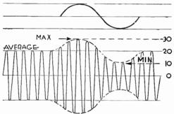
Fig. 10.—Calculating the Percentage Modulation.
