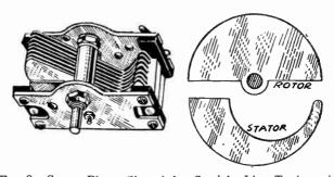
Fig. 8.—Stator Plates Shaped for Straight Line Tuning with Semicircular Rotor Plates.
