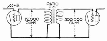
Fig. 3.—Simplified Diagram of Transformer Coupling.
