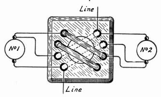
Fig. 1.-Special Form of Series-Parallel Switch.
