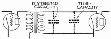
Fig. 7.—Capacities in Transformer Secondary Circuit.
