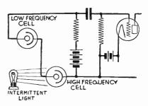
Fig. 14.—Screen Grid Amplifier for Phototube.
