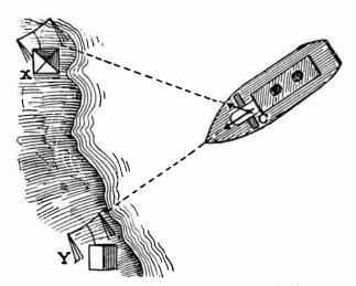
Fig. 2.—Determining Ship's Position with Radio Compass.
