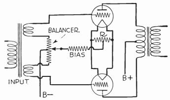
Fig. 8.—Equalizing Plate Currents in Push-pull Tubes.
