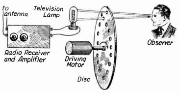
Fig. 2.—Nipkow Disc Reproduction at Television Receiver.
