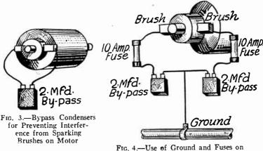
Fig. 4.—Use of Ground and Fuses on Interference Filter.
