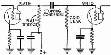
Fig. 1.—Resistance-capacity Coupled Amplifier.
