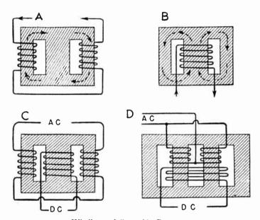
Windings of Saturable Reactors.
