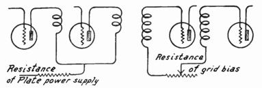
Fig. 1.—Feedback through Plate Supply Resistance to Cause Oscillation.
