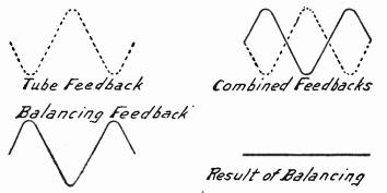
Fig. 1.-Combining the Feedbacks for Balancing.
