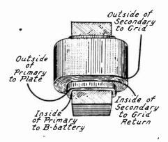
Fig. 6.-Windings and Connections of Audio Frequency Transformer.
