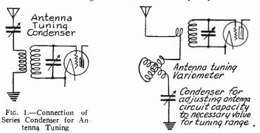
Fig. 2.—Use of Variometer for Antenna Tuning.
