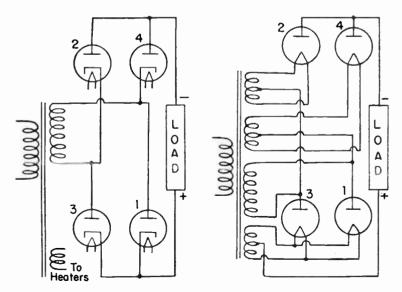
Fig. 7.—Four Tubes in Full-wave Bridge Circuit.
