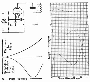
Fig. 6.—Connections and Action of Dynatron Oscillator.
