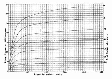
Fig. 1.—Plate Characteristics of a Power Pentode.
