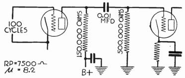
Fig. 5.-Typical Values for Resistance Coupling.
