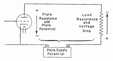
Fig. 5.—Relations of Supply Potential to Potential Drops.
