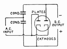
Fig. 1.—Voltage Doubler Connections.
