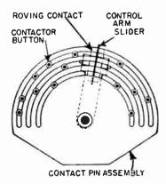
Fig. 3.—Roving Contact Pin Assembly.
