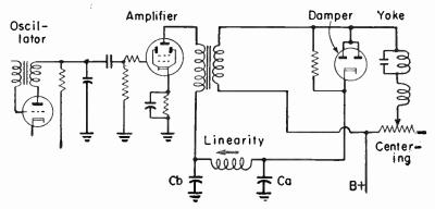
Fig. 28.—Sweep Circuits for Magnetic Deflection.
