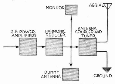
Fig. 3.—High Power Equipment Used at Transmitter.
