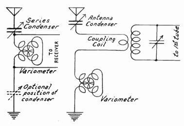
Fig. 4.—Variometer and Series Condenser for Antenna.
