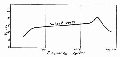
Fig. 5.—Result of Frequency Distortion in Amplifier.
