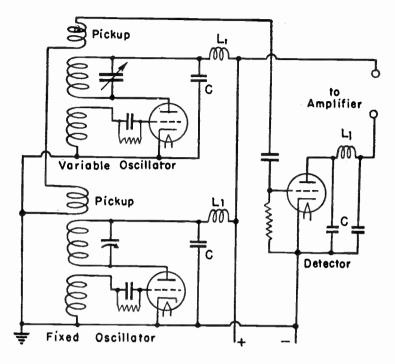
Fig. 1.—Circuits of a Beat Frequency Oscillator.
