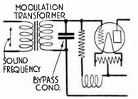
Fig. 4.—Grid Circuit Modulation.
