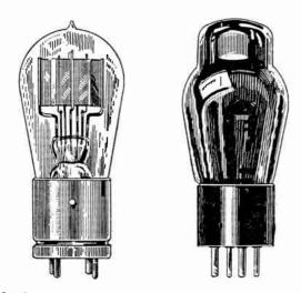
Fig. 2.—Short Prong UV201 of Early Manufacture and Latest Dome Shaped Long Prong UN201A
