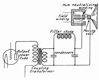
Fig. 5.—Hum Winding and Scratch Filter on Dynamic Speaker.
