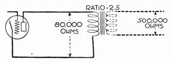
Fig. 4.—Secondary Load as Reflected in Primary.
