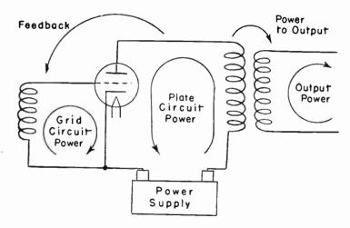
Fig. 1.—Principle of the Feedback Oscillator.
