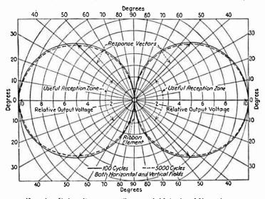
Fig. 4.—Polar Response Curve of Velocity Microphone.
