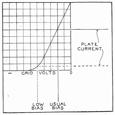
Fig. 5.—Biasing Points on Characteristic Curve.
