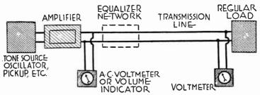
Fig. 5.-Making Measurements for Line Equalizing.
