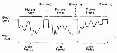
Fig. 6.—Horizontal Blanking Intervals Between Picture Signals.
