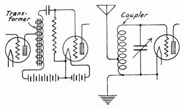
Fig. 3.—Auto-Transformer Interstage Coupling.
