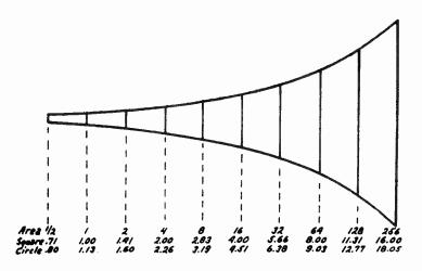
Fig. 3. Design of Exponential Horn,
