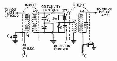
Fig. 15.—Crystal Filter Circuit
