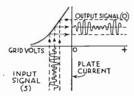
Fig. 1-A.—Class A Operating Characteristics.
