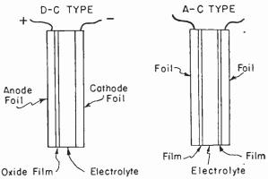
Elements Used in Electrolytic Condensers.
