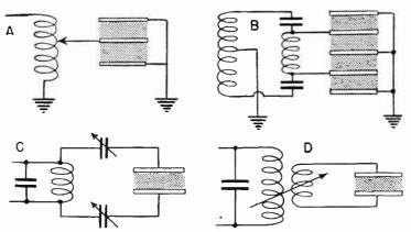
Fig. 2.—Electrode Arrangements for Electrostatic Heating.
