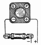
Fig. 1.-Filament Resistor.
