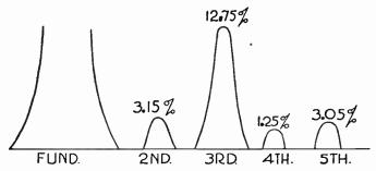
Fig. 6.—Harmonics with Push-pull Amplification.
