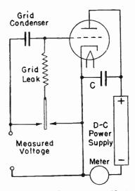
Fig. 1.—Plate Current Detector Used as VT Voltmeter.
