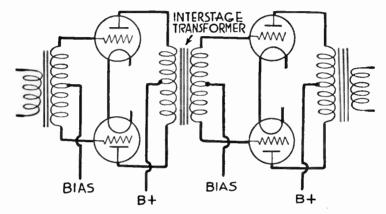
Fig. 12.—Dual Push-pull Amplification.
