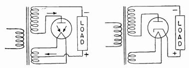
Fig. 1.—Tubes Used as Half-wave Rectifiers.
