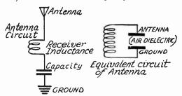
The Antenna Circuit and Its Electrical Equivalent.
