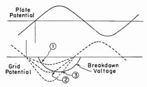
Fig. 5.—Breakdown Control by Variation of Grid Potential Amplitude, with Phase Shift of Grid Potential.
