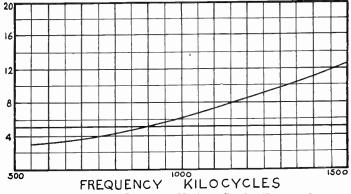
Fig. 5.—Sideband Widths at Various Carrier Frequencies.
