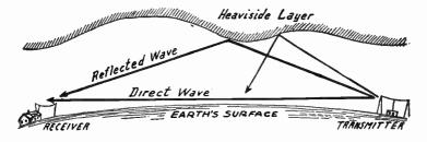
Fig. 1.—Effect of Heavyside Layer on Fading
