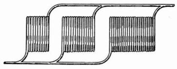
Fig. 4.—Inductance Coils in Parallel.
