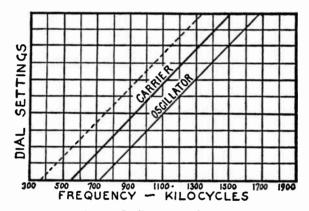
Fig. 5.—Relation of Oscillator and Carrier Frequencies.
