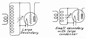
Fig. 4.—Large Secondary Giving Increased Power or Voltage.
