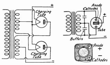
Fig. 3.—Charging Tubes Used as Filament Supply Rectifier.
