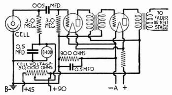
Fig. 14.—Sound Picture Amplifier with Phototube.
