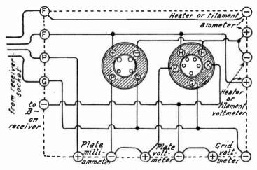
Fig. 9.-Test Board with Sockets.
