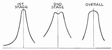
Fig. 15.—Resonance Curves for Intermediate Amplifier.
