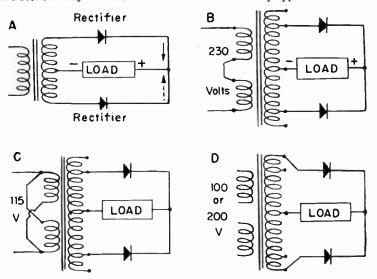
Fig. 5.—Contact Rectifiers in Full-wave Circuits.
