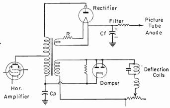
Fig. 37.—Flyback Type of High-voltage Supply.
