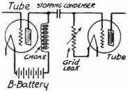
Fig. 2.-The Impedance Coupled Audio Amplifier.
