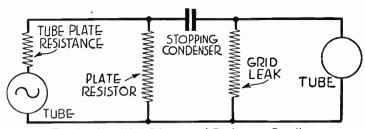
Fig. 2.—Simplified Diagram of Resistance Coupling.
