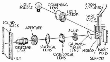
Fig. 5.—Variable Area System of Recording.
