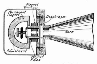
Fig. 1.—Electromagnetic Type of Loud Speaker.
