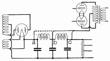
Fig. 7.—Connections of Plate Circuit to Filter.
