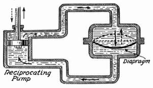
Fig. 5.—Hydraulic Explanation of Condenser Action.
