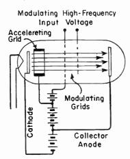
Fig. 1.—The Elements Employed for Velocity Modulation.
