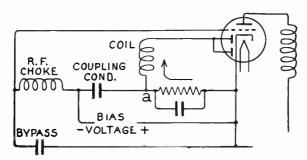
Fig. 4.—Double-diode Half-wave Detector.
