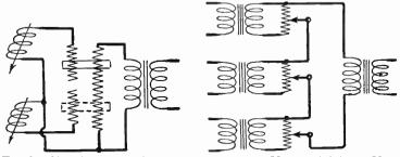
Fig. 9.—Simplified T-section Fader.
