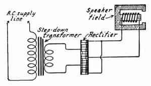
Fig. 7.—Rectifier Field Current Supply.
