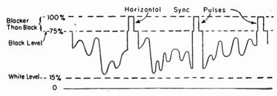
Fig. 7.—Horizontal Sync Pulses During Blanking Intervals.
