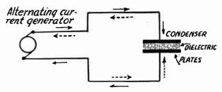
Fig. 6.—Flow of Alternating Current Through a Condenser.
