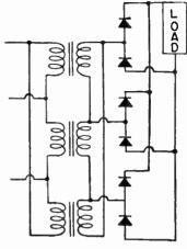
Fig. 5.—Six Elements in a Bridge Circuit.
