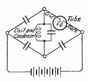
Fig. 6.—Position of Tube Capacity in a Bridge Circuit for Balancing.
