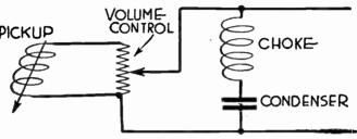
Fig. 10.—Connections for Scratch Filter.
