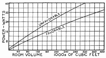
Fig. 12.—Power Requirements According to Room Volume.
