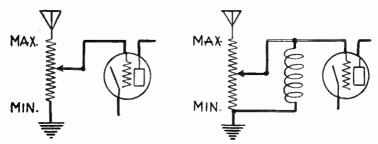
Fig. 14.—Volume Controls for Untuned Antenna Circuits.
