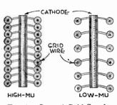
Fig. 1.—Control Grid Spacing and Extent of Fields.
