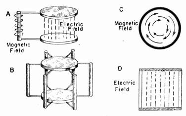
Fig. 1.—Principle of the Cavity Resonator.
