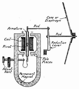
Fig. 2.-Balanced Armature Type of Loud Speaker.
