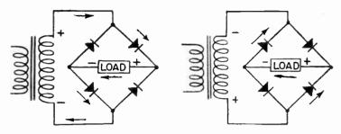
Fig. 6.—Bridge Type Full-wave Rectifier.
