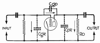
Fig. 7.—Tube Capacities Affecting Amplification.
