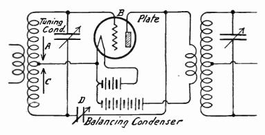
Fig. 4.—Rice Method of Balancing.
