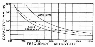
Fig. 19.—Change of Capacity to Maintain Oscillator Frequency.
