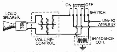
Fig. 10.—Switching and Volume Control at Loud Speaker.
