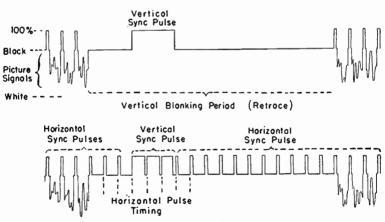
Fig. 8.—Vertical Sync Pulse During Vertical Blanking Period.
