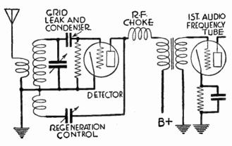
Fig. 4.—Regenerative Detector for Short Wave Reception
