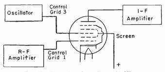
Fig. 26.—Connections for a Pentagrid Mixer.
