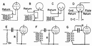
Fig. 3.—Returns for Filament-cathode Type Tubes, Also for Circuits with Grid Condensers.
