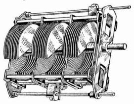
A Ganged Condenser for Tuning Three Circuits.
