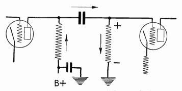
F|c. 6.—Effect of Leakage Through Stopping Condenser.
