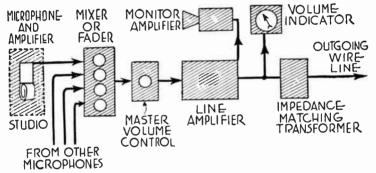
Fig. 1.—Speech Input Equipment for Broadcasting.
