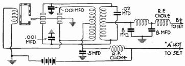
Fig. 8.—Diagram at Synchronous (Rectifying) Type of Vibrator "B" Supply for Automobile Radio Receivers.
