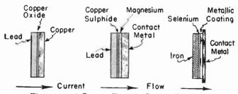
Elements and Current Flow in Contact Rectifiers.
