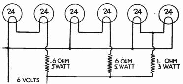
Fig. 1.—Series Parallel Connection of Tube Filaments Used in Early Automobile Receiver Design.
