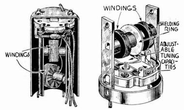
Fig. 16.—Construction of Intermediate Frequency Transformers.
