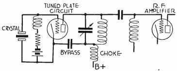
Fig. 3.—Circuit of Crystal Controlled Oscillator.
