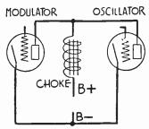
Fig. 5.—Principle of Constant Current Modulation.
