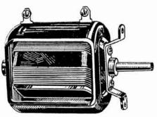
Fig. 2.—Variometer with Rectangular Windings.
