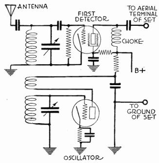
Fig. 6.—Superheterodyne Converter for Short Wave Reception
