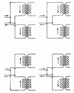
Fig. 11.—Connections of Transformers to Supply Line.
