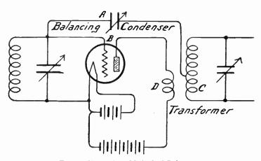
Fig. 2.—Neutrodyne Method of Balancing.
