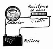
Fig. 2.—Determining Voltage Drop with Ohm's Law.
