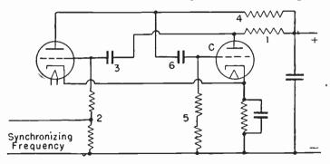
Fig. 3.—Circuit of Multivibrator Oscillator.
