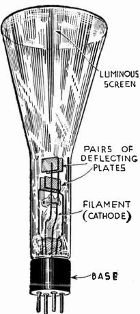
Fig. 1.—A Cathode-ray Tube.
