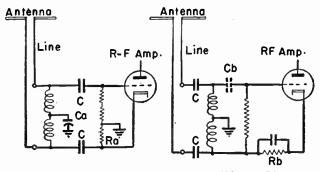
Fig. 17.—Untuned Input Circuits for 300-ohm Lines.
