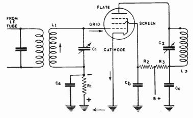
Fig. 3.—Connections for a Typical Limiter.
