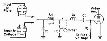
Fig. 19.—Typical Connections for Video Detectors.
