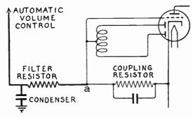
Fig. 3.—Double-diode in Automatic Volume Control.
