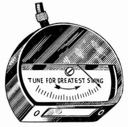
Fig. 11.—Reversed Scale Meter Tuning Indicator
