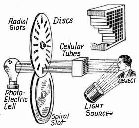
Fig. 3.—Action of Baird Discs in Television.
