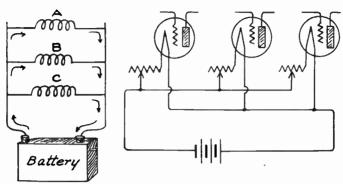
Fig. 1.—Parallel Circuits. Fig. 2.—Tube Filaments in Parallel Circuit.
