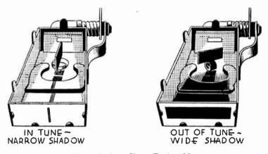
Fig. 12.-Iron Vane Tuning Meter
