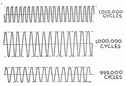
Fig. 9.—The Three Received Frequencies.
