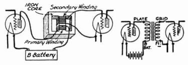
Fig. 1.—Transformer Coupling for Audio Frequency Amplifier.
