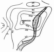
Fig. 11.—Variations in Radio Field Intensity.
