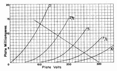
Load Line Used for Computing Voltage Amplification.
