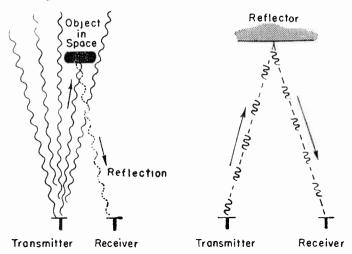
Fig. 1.—Reflection of Radar Waves.
