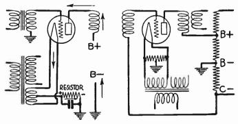
Fig. 7.—Biasing for Filament Tubes.
