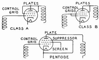
Fig. 6.—Connections for Voltage-amplifier Pentodes.
