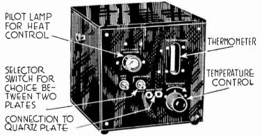
Fig. 4.—Temperature Control Box for Quartz Plates.
