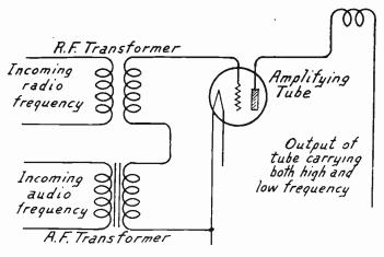
Fig. 1.—Effect of Reflexing on Amplifying Tube.
