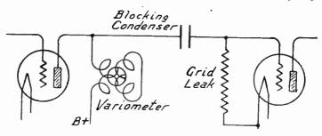
Fig. 1.—Tuned Impedance Coupling with Variometer.
