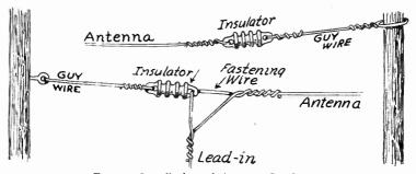
Fig. 1.—Installation of Antenna Insulators.
