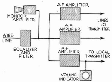
Fig. 5.—Bridging System Used in Chain Broadcasting.
