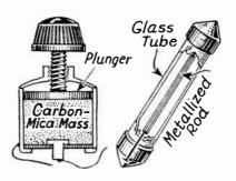
Fig. 2.—Carbon Type and Metallized Type of Resistors.
