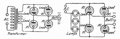
Fig. 8.—Electrolytic Rectifiers in Full-wave Bridge Circuit.
