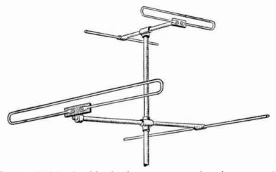
Fig. 10.—High-band and low-band antennas mounted on the same mast.
