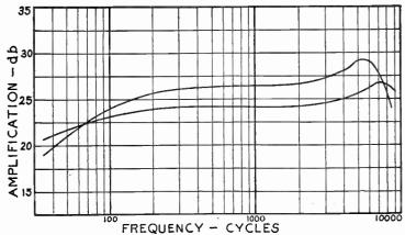
Fig. 8.—Amplification with Transformer Coupling.
