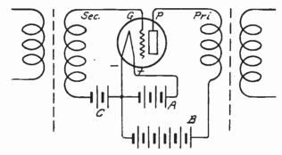
Fig. 6.-Circuits of Amplifying Stage.
