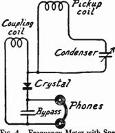
Fig. 3.—Inductively Coupled Indicator Fig. 4.—Frequency Meter with Spe-Circuit for Frequency Meter.
