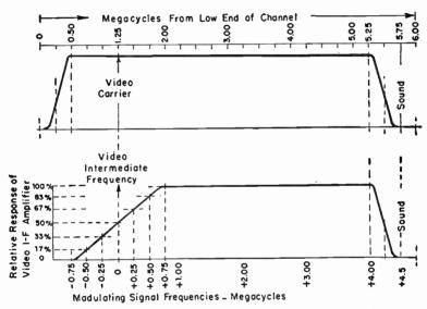
Fig. 12.—Distribution of Transmitted Frequencies and Frequency Response of the Video I-f Amplifier.
