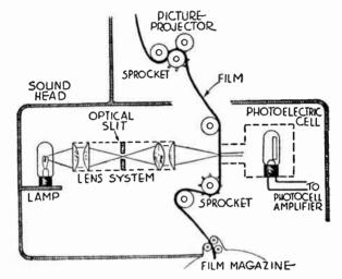
Fig. 12.—Principal Parts of a Sound Head.
