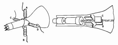
Fig. 2.—Electromagnetic Deflection of the Electron Beam.
