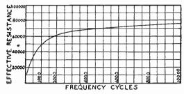
Fig. 6.—Frequency Effect on Apparent Resistance.
