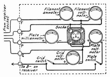
Fig. 8.—Receiver Tester with Attached Meters.
