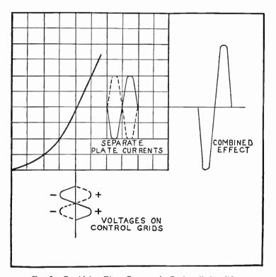
Fig. 2.—Combining Plate Currents in Push-pull Amplifier.
