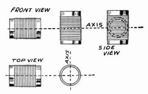
Relative Coil Positions for Minimum Coupling.
