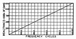
Fig. 5.—Frequency Effect on Inductive Reactance.
