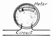
Fig. 1.—Ammeter in Series with Circuit.
