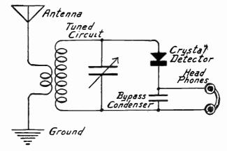
Receiver Circuit with Crystal Detector.
