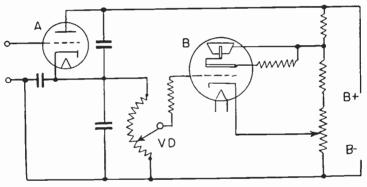
Fig. 7.-Electron-ray Tube Used as the Indicator for VT Volumeter.
