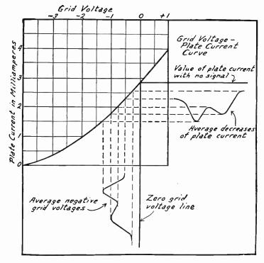
r'ig. 3.—Action of the Grid Leak Detector. Variations of grid voltage cause corresponding variations of plate current, the latter decreasing in value as detection takes place.
