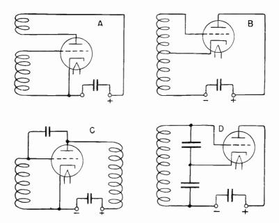
Fig. 2.—Methods of Providing Feedback.
