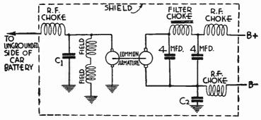
Fig. 6.—Circuit Diagram of Dynamotor Type Automobile "B" Supply.
