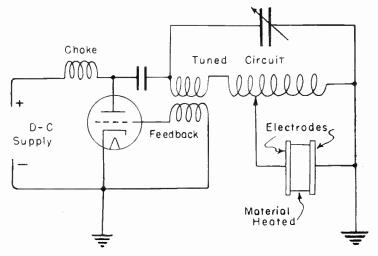
Fig. 1.—Simplified Circuit for Electrostatic Heating.
