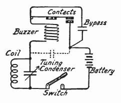
Oscillator Circuit Excited by Buzzer.
