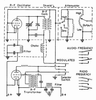
Modulated Oscillator or Signal Generator.
