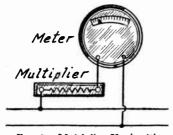
Fig. 3.-Multiplier Used with Voltmeter.
