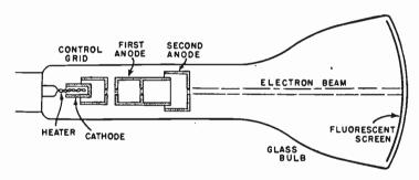
Fig. 1.—Principal Parts of a Cathode-ray Tube.
