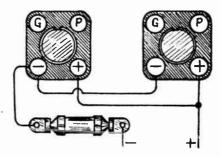
Fig. 2.—Single Filament Resistor for Two Tubes.
