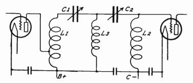
Fig. 7.—Circuit Arrangement of Vreeland Band Selector.
