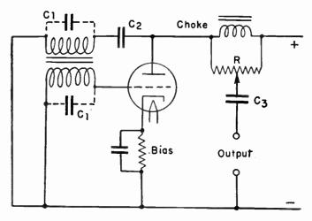
Fig. 1.—Feedback Type of Audio-frequency Oscillator.
