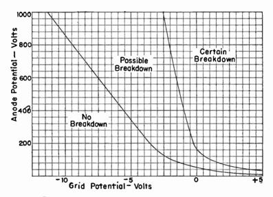
Fig. 1.—Range of Breakdown Potentials for Mercury-vapor Thyratron of Three-element Type.
