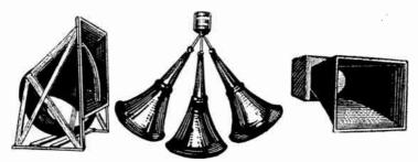
Fig. 9.—Projectors Used for Public Address Work.
