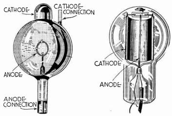
Fig. 1,—Phototube with Wall
