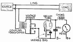
Fig. 2.—Vacuum Tube Type of Volume Indicator.
