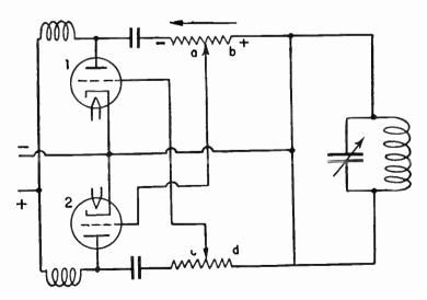
Fig. 10.-Negative Resistance Oscillator with Two Tubes.
