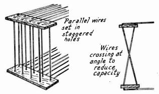
Arrangement of Wire on Loop Framework.
