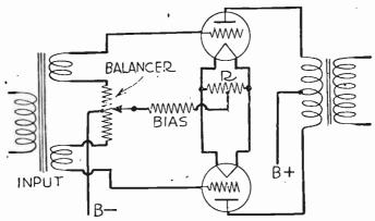
Fig. 8.—Equalizing Plate Currents in Push-pull Tubes.
