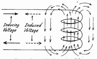
Fig. 1.—Effect of Self-Inductance in a Coil.
