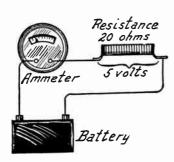
Fig. 2.—Determining Voltage Drop with Ohm's Law.
