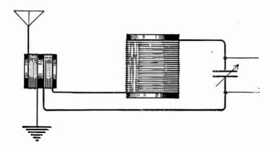
Fig. 2.—Separate Coupling Coil for Antenna Circuit.
