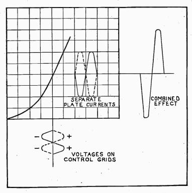
Fig. 2.—Combining Plate Currents in Push-pull Amplifier.
