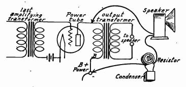
Fig. 3.—First Test on Audio Amplifier with Transformer Speaker Coupling.
