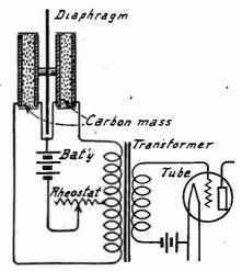
Fig. 2.—Double-button Carbon Microphone.
