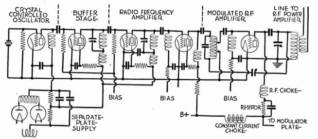
Fig. 8.—Radio Frequency Amplifier at Transmitter.
