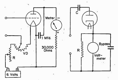
Fig. 5.—Circuit for Moullin Type VT Voltmeter.
