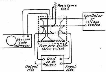
Fig. 8.—Checking Amplifier Unit with VT Voltmeter.
