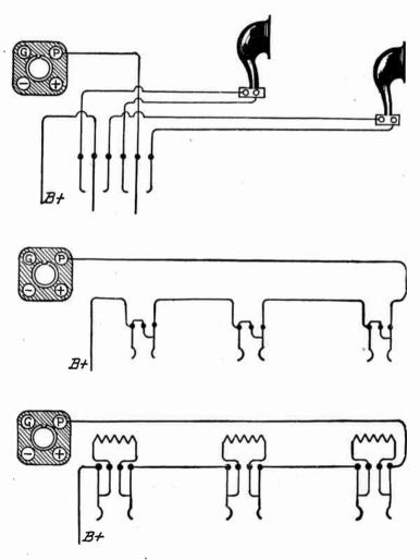
Fig. 6.—Jacks for Connection of Several Speakers.
