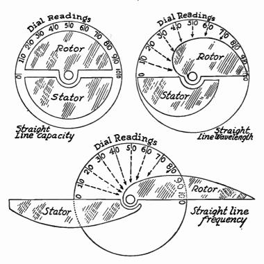
Fig. 5.—Basic Forms of Condenser Rotor Plates.
