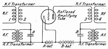
FIG. 2.—Circuits of Reflexed Amplifying Tube.
