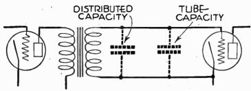
Fig. 7.—Capacities in Transformer Secondary Circuit.
