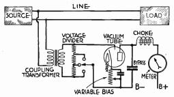
Fig. 2.—Vacuum Tube Type of Volume Indicator.
