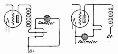
Fig. 4.—Meter Connections Made with Switches.
