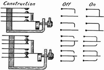
Fig. 2.—Operation of a Jack Switch.
