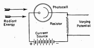
Fig. 3.—The Basic Phototube Circuit.
