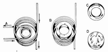
Fig. 1.—Elementary Principle of Induction Heating.
