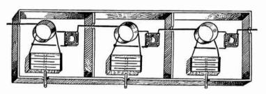
Fig. 5.—Amplifying Stages Enclosed in Individual Shields.
