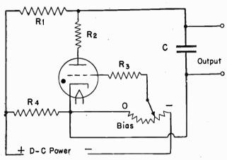
Fig. 6.—Relaxation Oscillator Using Thyratron Tube.
