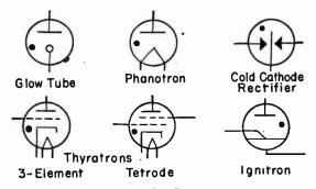
Fig. 1.—Symbols for Gas-filled Tubes.
