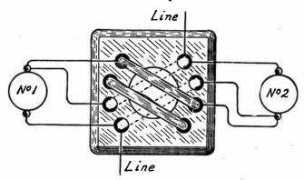
Fig. 1.—Special Form of Series-Parallel Switch.
