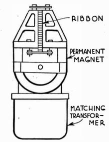
Fig. 1.—Constructional Details of Velocity Microphone.
