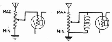
Fig. 14.—Volume Controls for Untuned Antenna Circuits.
