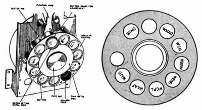
Fig. 6.—Telephone Type Tuning Dial.
