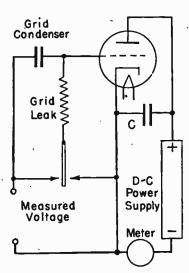
Fig. 2.—Grid Leak Detector Used as VT Voltmeter.
