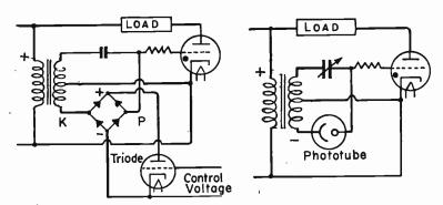
Fig. 10.—Phase-shift Control by Means of a Vacuum Triode Connected to a Bridge Rectifier.
