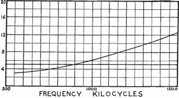
Fig. 5.—Sideband Widths at Various Carrier Frequencies.
