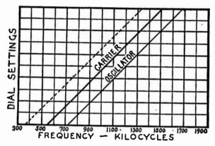
Fig. 5.—Relation of Oscillator and Carrier Frequencies.
