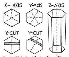
Fig. 2.—Methods of Cutting Quartz Plates.
