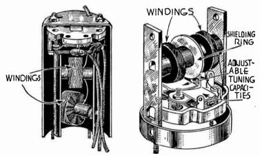
Fig. 16.—Construction of Intermediate Frequency Transformers.
