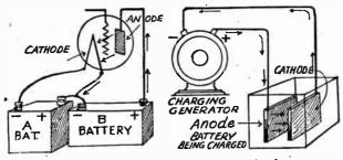
Anodes and Cathodes in Electric Circuits.
