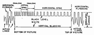
Fig. 4.—Order in Which the Control Signals Are Received.
