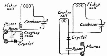
Fig. 3.—Inductively Coupled Indicator Fig. 4.—Frequency Meter with Spe-Circuit for Frequency Meter. cial Coupling for Indicator.
