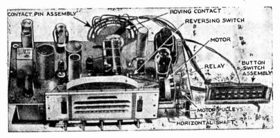
Fig. 1.—General Electric Touch Tuning Chassis.
