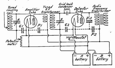
Fig. 2.—Bypass Condensers in a Receiver.
