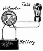
Fig. 3.—Determining Current with Ohm's Law.
