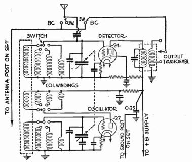
Fig. 8.—Circuit Diagram of Superheterodyne Converter
