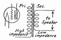
Fig. 2.—Matching Impedances with Special Transformer.
