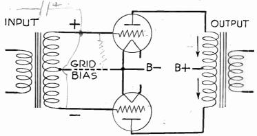
Fig. 1.—Elementary Push-pull Circuit.
