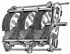
A Ganged Condenser for Tuning Three Circuits.
