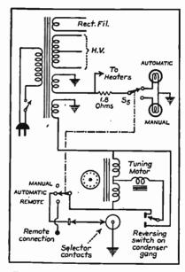
Fig. 2.—Electric Tuning Circuit.
