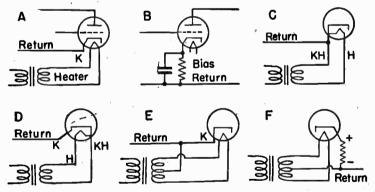
Fig. 2.—Returns for Heater-cathode Type Tubes.
