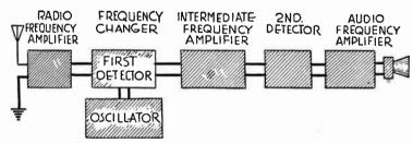
Fig. 3.—Elements of a Modern Superheterodyne.
