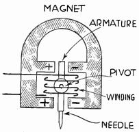
Fig. 7.—Balanced Armature Type of Electromagnetic Pickup.
