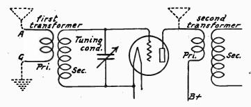
Fig. 1.—Antenna Connections for Testing Radio Stages.
