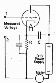
Fig. 1.—Plate Current Detector Used as VT Voltmeter. .
