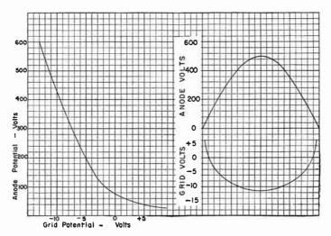
Fig. 1.—Average Breakdown Potentials for a Gas-filled Tube. Fig. 2.—Relations of Grid and Anode Volts for Breakdown.
