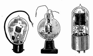
Fig. 1.—Early Experimental Types of Vacuum Tubes
