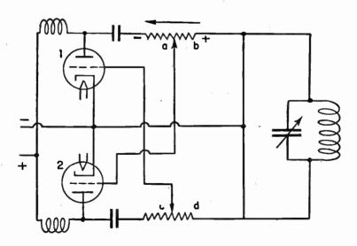
Fig. 10.—Negative Resistance Oscillator with Two Tubes.
