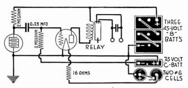
Fig. 6.—Photoconductive Cell Amplifier for Batteries.
