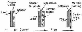
Elements and Current Flow in Contact Rectifiers.
