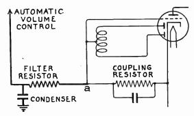
Fig. 3.—Double-diode in Automatic Volume Control.
