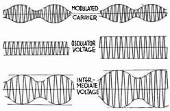
Fig. 12.—How Oscillator Voltage Increases Intermediate Voltage.
