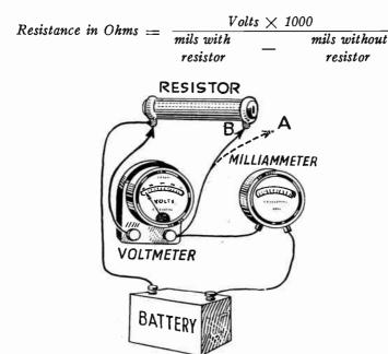
Fig. 18.—Measuring the Resistance of a Resistor.
