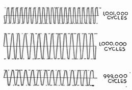
Fig. 9.—The Three Received Frequencies.
