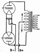
Fig. 3.—D.C. In Output Transformer Primary.
