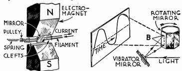
Fig. 2.—Principle of the Duddell Oscillograph.
