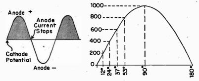
Fig. 5.—Anode Current Flows Only During Positive Halfcycles.
