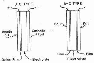
Elements Used in Electrolytic Condensers.
