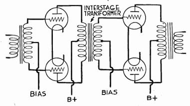
Fig. 12.—Dual Push-pull Amplification.
