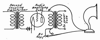
Fig. 5.—Second Test on Audio Amplifier.
