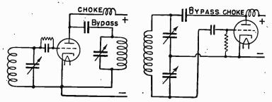
Fig. 5.—Capacity Feedback Oscillator Circuits. Tuned-plate, tuned-grid at left; Colpitts at right.
