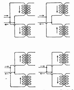
Fig. 11.—Connections of Transformers to Supply Line.
