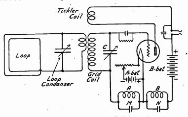
Circuits of Super-Regenerative Single Tube Receiver.
