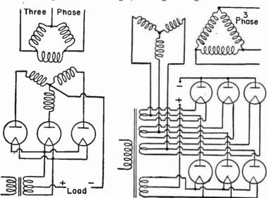
Fig. 1.—Polyphase Half-wave Rectifier.
