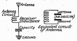
The Antenna Circuit and Its Electrical Equivalent.
