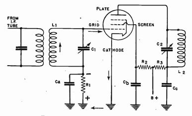
Fig. 3.—Connections for a Typical Limiter.
