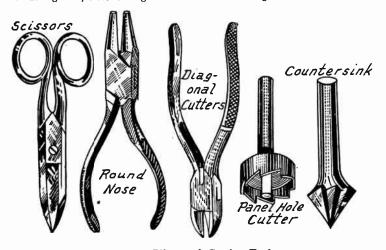
Fig. 2.—Pliers and Cutting Tools.
