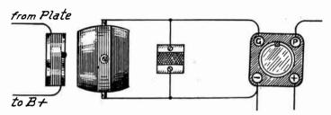
Fig. 3.-Layout of Variometer Used in Tuned Transformer for Coupling.
