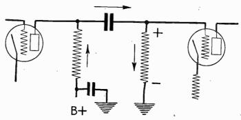
Flg. 6.—Effect of Leakage Through Stopping Condenser.
