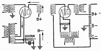
Fig. 7.—Biasing for Filament Tubes.
