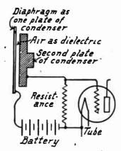
Fig 3.—Condenser Microphone.
