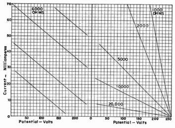
Fig. 2.—Load Lines for 6,000 Ohms Resistance.
