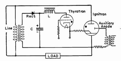
Fig. 4.—Ignitron Control Circuit with Auxiliary Anode Connections.
