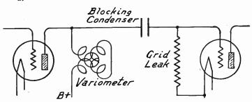
Fig. 1.—Tuned Impedance Coupling with Variometer.
