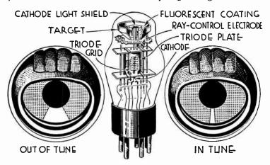
Fig. 13.—Cathode Ray Tuning Meter
