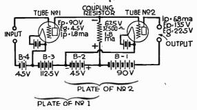
Fig. 1.—Simple Form of Direct Coupled Amplifier.
