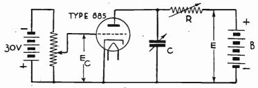
Fig. 11.—Thyratron Sweep Circuit Oscillator.
