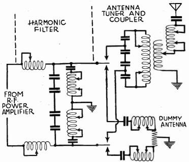
Fig. 10.—Antenna System and Harmonic Filter.
