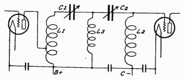
Fig. 7.—Circuit Arrangement of Vreeland Band Selector.
