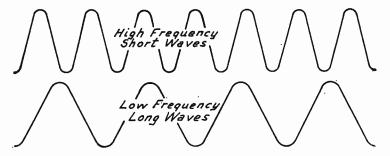
Fig. 2.—Frequency Relation to Wavelength.
