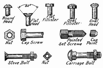
Screws and Bolts Used in Construction Work.
