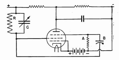
Fig. 9.—Negative Resistance Oscillator Employing Resistancecapacity Circuits.
