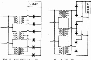
Fig. 4.—Six Elements with Center-tapped Transformer.
