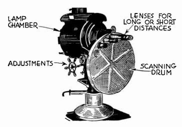
Fig. 6.—Television Scanner Employing an Arc Lamp.
