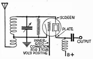
Fig. 7.—Screen Grid Tube as Space Charge Detector
