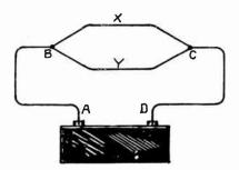
Fig. 1.—Circuits with Resistances in Parallel on Battery.
