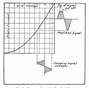
Fig. 2.—Distortion Caused by Zero Grid Bias.
