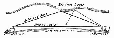
Fig. 1.—Effect of Heavyside Layer on Fading
