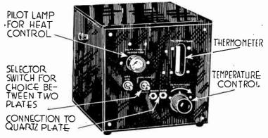
Fig. 4.—Temperature Control Box for Quartz Plates.
