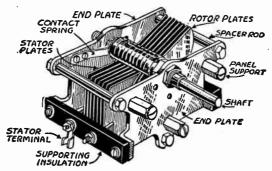
Fig. 1.—The Parts Considered in Design of a Typical Variáble Condenser.
