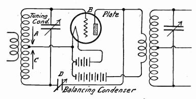
Fig. 4.—Rice Method of Balancing.
