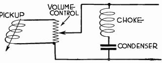
Fig. 10.—Connections for Scratch Filter.
