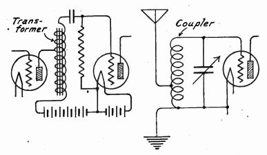
Fig. 3.—Auto-Transformer Interstage Coupling.
