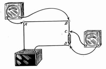
Fig. 1.—Principle of Testing for Open Circuits.
