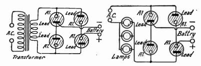
Fig. 8.—Electrolytic Rectifiers in Full-wave Bridge Circuit.
