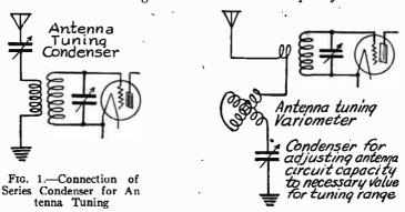
Fig. 2.—Use of Variometer for Antenna Tuning.
