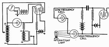
Fig. 14.—Screen Grid Amplifier for Phototube.
