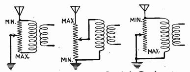
Fig. 13.—Antenna Circuit Volume Controls for Transformers.
