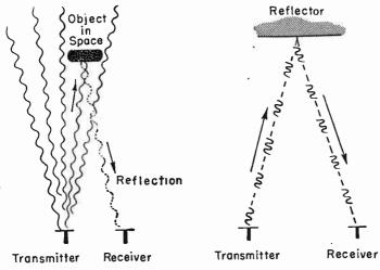
Fig. 1.—Reflection of Radar Waves.
