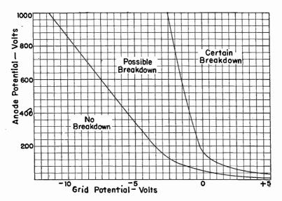
Fig. 1.—Range of Breakdown Potentials for Mercury-vapor Thyratron of Three-element Type.
