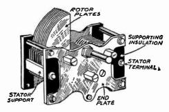
Fig. 3.—Terminal Positions Considered in Condenser Design.
