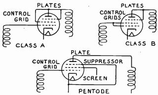
Fig. 6.—Connections for Voltage-amplifier Pentodes.
