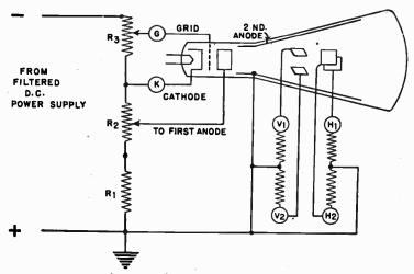
Fig. 4.—Control Circuits for Cathode-ray Tube.
