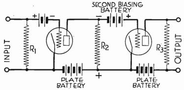
Fig. 2.—Two-Stage Direct Current Amplifier.
