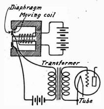
Fig. 4.-Moving Coil Microphone.
