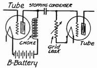
Fig. 2.—The Impedance Coupled Audio Amplifier.
