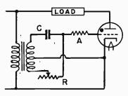
Fig. 8.—Phase Shift with Adjustable Resistor and Fixed Condenser.
