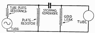
Fig. 2.—Simplified Diagram of Resistance Coupling.
