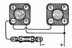
Fig. 2.—Single Filament Resistor for Two Tubes.
