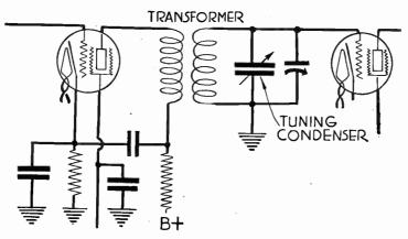
Fig. 1.—Transformer Coupling for Radio Frequencies.
