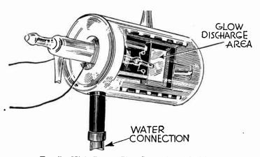
Fig. 7.—High Power Glow Lamp for Television.
