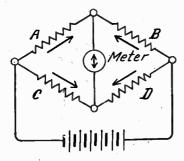
Fig. 5.—Balancing Principle of the Wheatstone Bridge.
