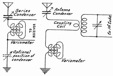
Fig. 4.—Variometer and Series Condenser for Antenna.
