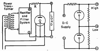
Fig. 3.—Connections Used with Single Regulator Tube.
