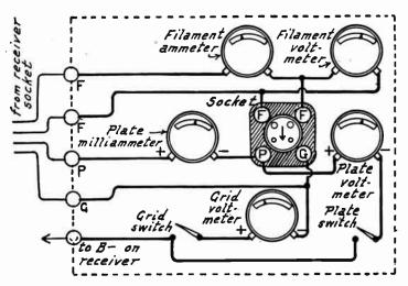
Fig. 8.—Receiver Tester with Attached Meters.
