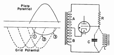
Fig. 6.—Control by Variation of Phase Shift of Grid Potential, with Constant Amplitude.
