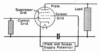
Fig. 3.—Typical Connections for Pentode Power Amplifier.
