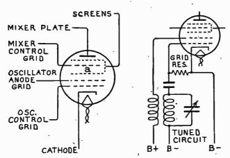
Fig. 23.—The Pentagrid Converter.
