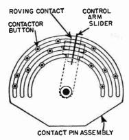
Fig. 3.—Roving Contact Pin Assembly.
