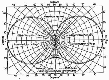
Fig. 4.—Polar Response Curve of Velocity Microphone.
