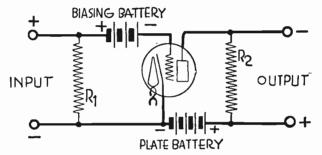
Fig. 1.—Simple Form of Direct Current Amplifier.
