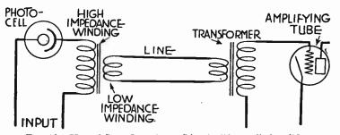
Fig. 13.—Use of Low Impedance Line in Photocell Amplifier.
