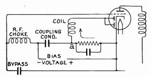
Fig. 4.—Double-diode Half-wave Detector.
