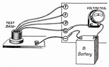
Fig. 10.-Circuit Tests on Receiver.
