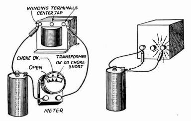
Fig. 14.—Test for Open Circuit or Fig. 15.—Test for Short Circuited Short in Transformer or Choke.
