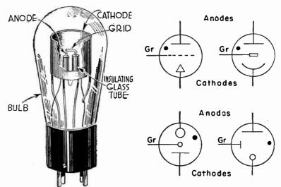
Fig. 1.—Construction of One Style of Grid-glow Tube.
