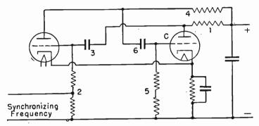
Fig. 3.—Circuit of Multivibrator Oscillator...
