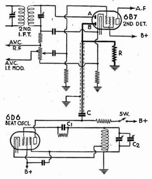
Fig. 10.—Beat Frequency Oscillator Circuit
