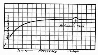
Fig. 4.—Resonance Peak Causing Distortion in Audio Frequency Coupler.
