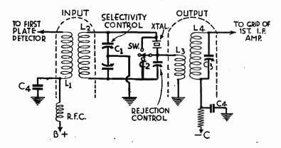
Fig. 15.—Crystal Filter Circuit
