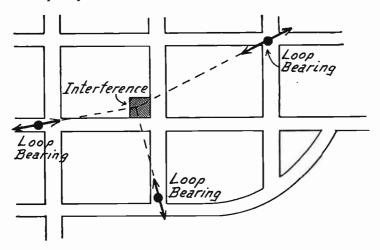
Fig. 2.—Locating Interference with Portable Receiver.
