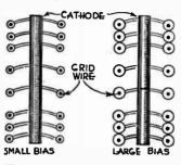
Fig. 2.—Control Grid Spacing in Variable-mu Tube.
