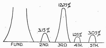
Fig. 6.—Harmonics with Push-pull Amplification.
