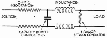
Fig. 4.—Electrical Elements of Transmission Line.
