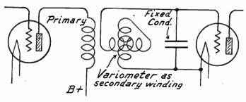
Fro. 2.—Variometer Used as Secondary of Tuned Transformer for Coupling.
