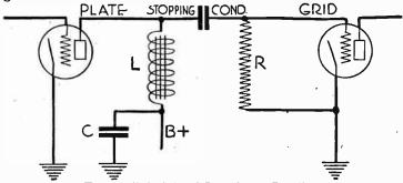
Fig. 1.—Principle of Impedance Coupling.
