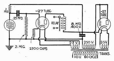
Fig. 7.—Photoconductive Cell Amplifier for Power Line.
