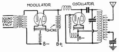
Fig. 6.—Connection of Modulator to Oscillator.
