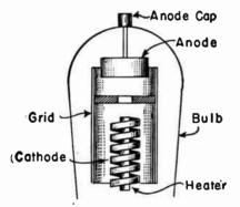
Fig. 1.—Arrangement of Elements in One Style of Thyratron.
