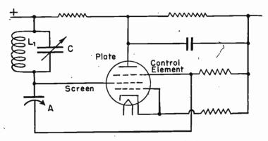
Fig. 8.—Negative Transconductance Oscillator.
