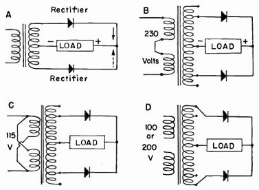
Fig. 5.—Contact Rectifiers in Full-wave Circuits.
