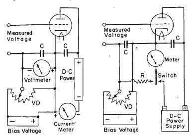
Fig. 3.—Slide Back Instrument Using Two Meters.
