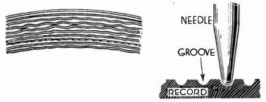
Fig. 3.—Sound Modulated Grooves. Fig. 4.—Cross Section of Record.
