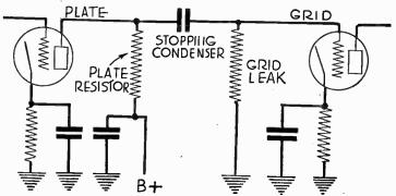
Fig. 1.—Resistance-capacity Coupled Amplifier.
