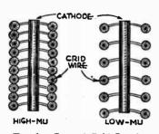
Fig. 1.—Control Grid Spacing and Extent of Fields.
