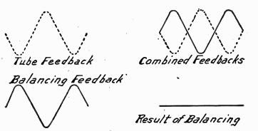
Fig. 1.—Combining the Feedbacks for Balancing.
