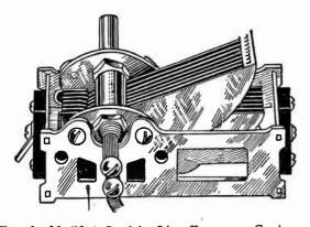
Fig. 6.—Modified Straight Line Frequency Condenser.
