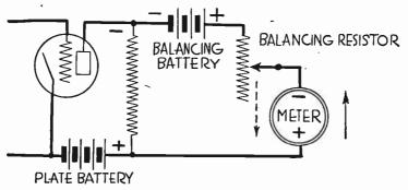
Fig. 3.—Balancing the Plate Resistor Voltage.
