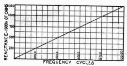
Fig. 5.—Frequency Effect on Inductive Reactance.
