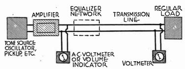
Fig. 5.—Making Measurements for Line Equalizing.
