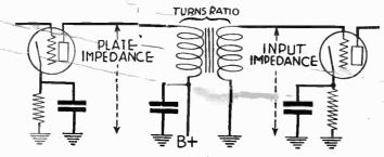
Fig. 2.—Circuit for Transformer Coupling.
