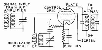
Fig. 25.—Complete Pentagrid Converter Connections.
