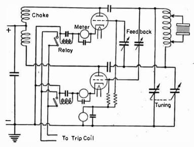
Fig. 3.—Typical Circuit for Electrostatic Heating.
