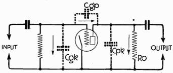
Fig. 7.—Tube Capacities Affecting Amplification.
