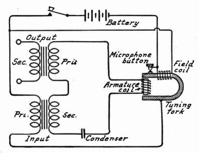
Fig. 2.—Tuning Fork Audio Oscillator.
