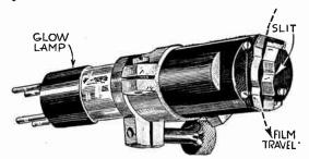
Fig. 10.—Glow Lamp Holder with Slit.
