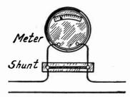
Fig. 4.—Shunt Used with Ammeter.
