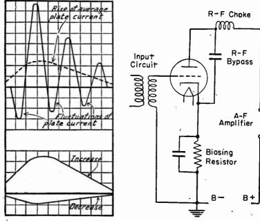
Fig. 2.—Current Change During Plate Current Detection.
