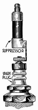
Fig. 10.— Spark Plug Auto Radio Suppressor.
