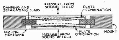
Fig. 1.—Cross Section of Single "Sound Cell."
