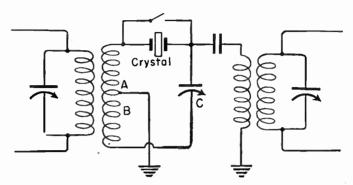
Fig. 27.—Crystal Used in Intermediate-frequency Amplifier.
