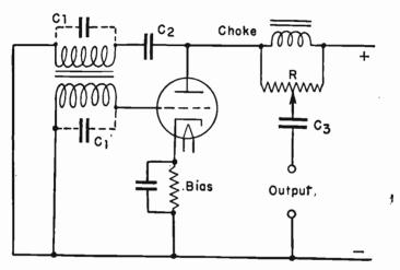
Fig. 1.—Feedback Type of Audio-frequency Oscillator.
