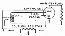
Fig. 2.—Double-diode Triode as Detector and Amplifier.
