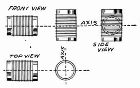
Relative Coil Positions for Minimum Coupling.
