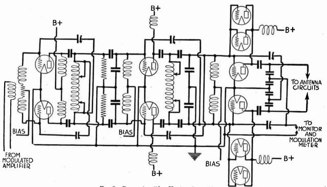
Fig. 9.—Power Amplifier Used at Transmitter.
