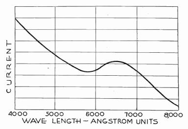
Fig. 5.—Color Sensitivity of Selenium Cell.
