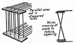
Arrangement of Wire on Loop Framework.
