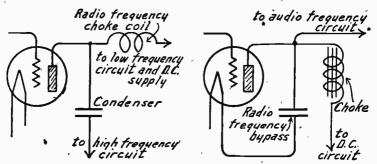
Fig. 1.—Separation of Frequencies with a Choke Coil.
