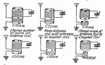
Fig. 1.—Close Coupling and Loose Coupling of Antenna Circuit.
