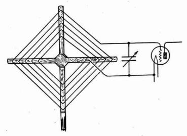
Connections from Spiral Loop to Receiver.
