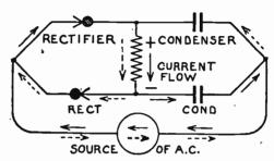
Fig. 2.—Equivalent Circuit for Voltage Doubler.
