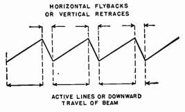
Fig. 5.—A Sawtooth Wave Form.
