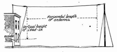
Physical Length of an Antenna and the Height of Its Lead-In.
