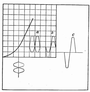
Fig. 4.—Balancing Unequal Changes of Plate Current.
