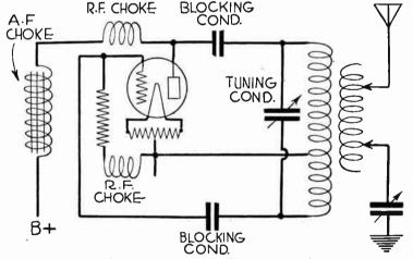
Fig. 3.—Oscillator Coupled to Transmitting Antenna.
