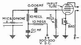
Fig. 2b.—Circuit Connection of Static Velocity Microphone.
