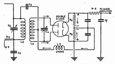
Fig. 6.—The Discriminator Stage of an FM Receiver.
