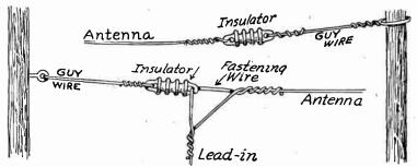
Fig. 1.—Installation of Antenna Insulators.
