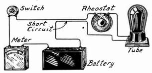
Fig. 2.—Testing for Short Circuit with Voltmeter.
