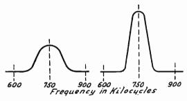
Fig. 3.—Effect of Regeneration on Signal.
