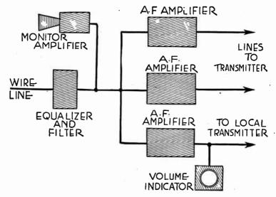
Fig. 5.—Bridging System Used in Chain Broadcasting.
