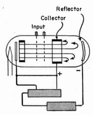
Fig. 2.—Method of Changing Velocity to Intensity Modulation.
