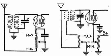
Fig. 20.—Dual Control with One Fig. 21.—Twin Control for Antenna Potentiometer. and Screen Voltage.
