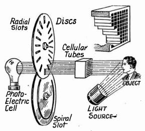
Fig. 3.—Action of Baird Discs in Television.
