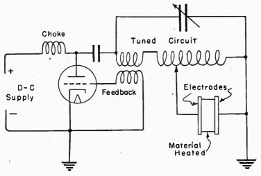
Fig. 1.—Simplified Circuit for Electrostatic Heating.
