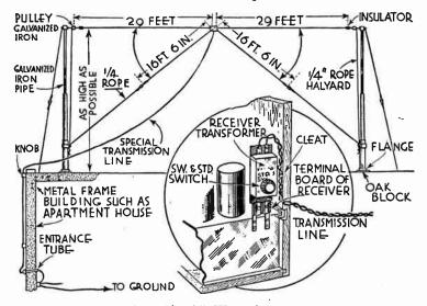
Fig. 14.—All Wave Antenna
