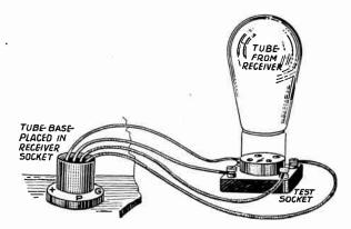
Fig. 7.-Tester Connection To Receiver.
