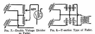
lessens the input voltage to the tube until it is of minimum value. Continued movement of the arm picks up and increases the signal from the lower pickup.
