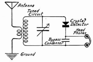
Receiver Circuit with Crystal Detector.
