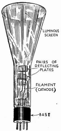
Fig. 1.—A Cathode-ray Tube.
