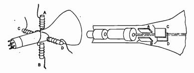
Fig. 2.—Electromagnetic Deflection of the Electron Beam.
