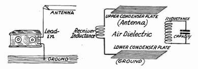
Fig. 2.—The Principle of the Capacity Antenna.
