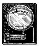
Fig. 5.—Milliammeter Used as Voltmeter.
