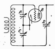
Fig. 7.—The Isofarad Method of Balancing.
