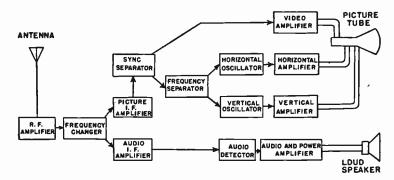
Fig. 3.—Principal Parts of a Television Receiver.
