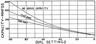
Fig. 22.—How Series Capacities Affect the Tuning.
