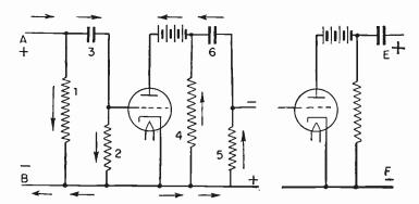
Fig. 2.—Operating Principle of the Multivibrator.
