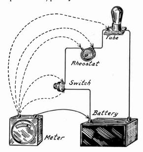
Fig. 2.—Testing Filament Circuit for Opens.
