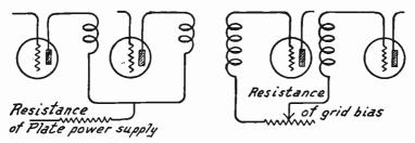
Fig. 1.—Feedback through Plate Supply Resistance to Cause Oscillation.
