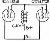
Fig. 4.—Grid Circuit Modulation.
