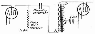
Fig. 11.—Parallel Feed with Resistor and Transformer.
