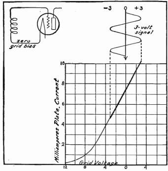
Fig. 1.—Effect of Zero Grid Bias, Distortion.
