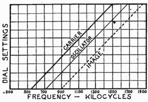
Fig. 17.—Relations Between Image, Oscillator and Carrier Frequencies.
