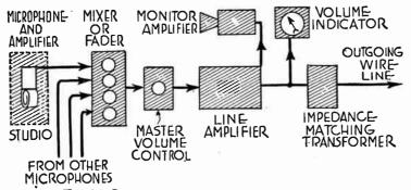
Fig. 1.—Speech Input Equipment for Broadcasting.
