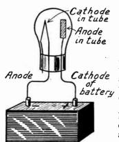
ELECTRODE.—Either one of the terminals of an electric source is called an electrode. The terminal, connection or conductor through which electric current or an electron stream enters or leaves anything is called an electrode. The terminal which the current enters is called the anode, the terminal through which the current leaves being called the cathode. See Anode and Cathode.
