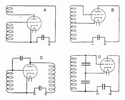
Fig. 2.—Methods of Providing Feedback.
