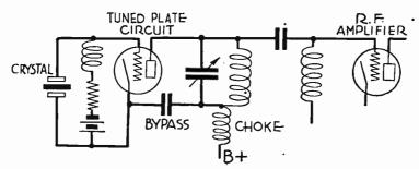
Fig. 3.—Circuit of Crystal Controlled Oscillator.
