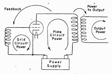
Fig. 1.—Principle of the Feedback Oscillator.
