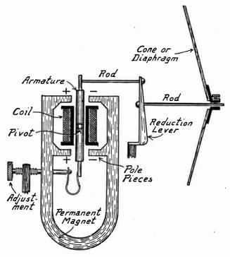
Fig. 2.—Balanced Armature Type of Loud Speaker.
