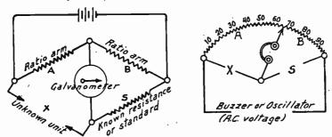
Fig. 3.—Functions of the Arms in a Bridge.
