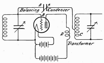
Fig. 2.—Neutrodyne Method of Balancing.
