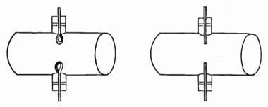
Fig. 2.—Energy Transfer Probes for Cavity Resonator.
