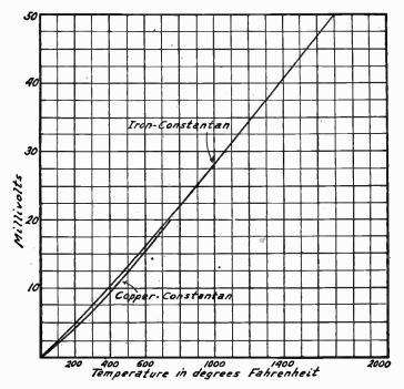
Fig. 2.—Voltage Developed by Thermocouples.
