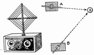
Fig. 1.—Elementary Principle of Radio Compass.
