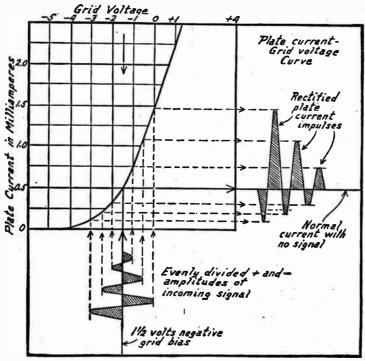
Fro. 1.—Action of Detector Using Grid Bias for Plate Current Rectification.
