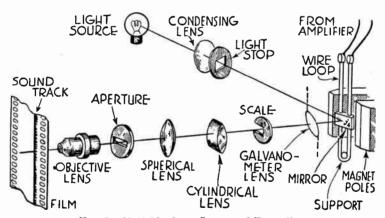
Fig. 5.—Variable Area System of Recording.
