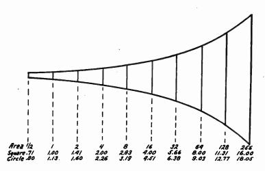
Fig. 3.—Design of Exponential Horn.
