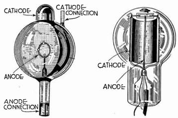
Fig. 1.—Phototube with Wall Type of Cathode.
