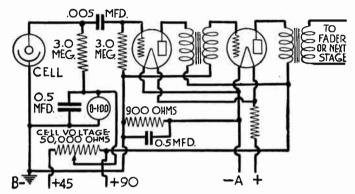
Fig. 14.—Sound Picture Amplifier with Phototube.
