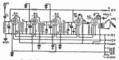
Fig. 15.—Circuits of Typical Airplane Receiver.
