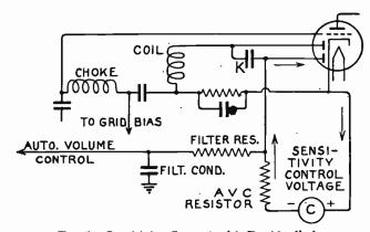
Fig. 5.—Sensitivity Control with Double-diode.
