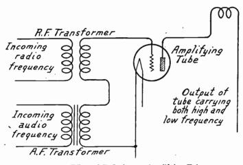
Fig. 1.—Effect of Reflexing on Amplifying Tube.
