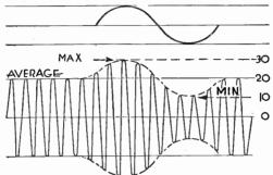
Fig. 10.—Calculating the Percentage Modulation.
