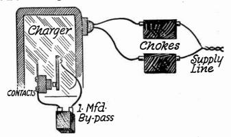
Fig. 5.—Handling Interference of Vibrators and Flashers.
