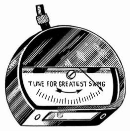
Fig. 11.—Reversed Scale Meter Tuning Indicator
