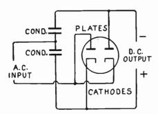
Fig. 1.—Voltage Doubler Connections.
