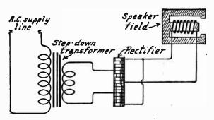
Fig. 7.—Rectifier Field Current Supply.
