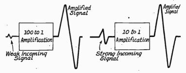
The Effect of Amplification on Signal Strength.
