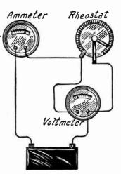
Fig. 1.—Determining Rheostat Resistance with Ohm's Law.
