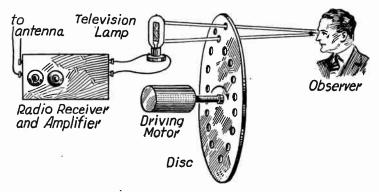
Fig. 2.—Nipkow Disc Reproduction at Television Receiver.
