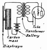
Fig. 1.—Simple Type of Microphone.
