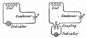
Fig. 1.—The Simplest Frequency Meter Circuit.
