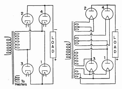
Fig. 7.—Four Tubes in Full-wave Bridge Circuit.
