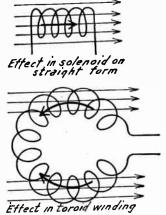
Fig. 3.—Opposing Voltages Set Up in Toroid Winding.
