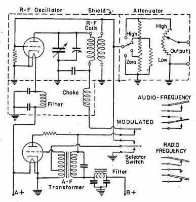
Modulated Oscillator or Signal Generator.
