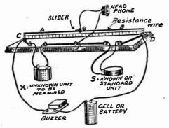
Fig. 5.—Practical Form of Slide Wire Bridge.
