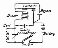
Oscillator Circuit Excited by Buzzer.
