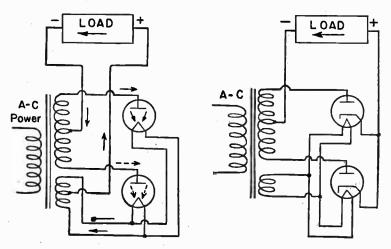
Fig. 1.—Two Filament-cathode Tubes in Full-wave Rectifier.
