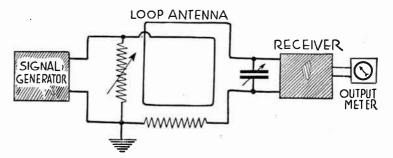
Fig. 12.—Method of Measuring Field Intensity.
