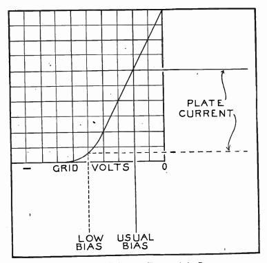
Fig. 5.—Biasing Points on Characteristic Curve.
