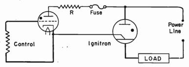
Fig. 2.—Thyratron Used for Control of an Ignitron.
