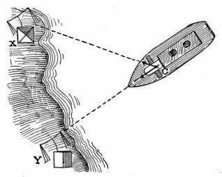
Fig. 2.—Determining Ship's Position with Radio Compass.
