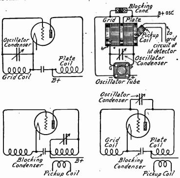
Fig. 6.—Oscillators with Tuned Grid Fig. 7.—Oscillator in Which Grid (above) and Tuned Plate (below). Coil and Plate Coil Are Tuned Together.
