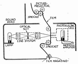
Fig. 12.—Principal Parts of a Sound Head.
