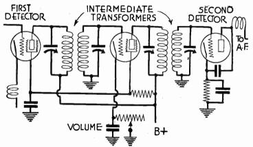
Fig. 14.—Typical Intermediate Frequency Amplifier.
