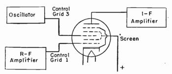
Fig. 26.—Connections for a Pentagrid Mixer.
