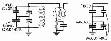
Fig. 21.—Arrangement of Capacities for Oscillator Tuning
