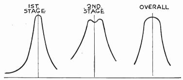
Fig. 15.—Resonance Curves for Intermediate Amplifier.
