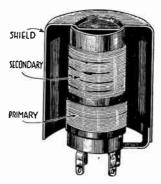
Fig. 2.—Shielded Radio Frequency Transformer.
