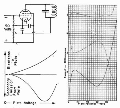
Fig. 6.—Connections and Action of Dynatron Oscillator.
