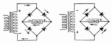
Fig. 6.—Bridge Type Full-wave Rectifier.
