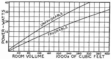
Fig. 12.—Power Requirements According to Room Volume.
