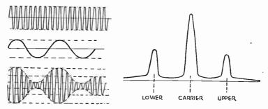
Fig. 7.—Combining the Frequencies in Modulation.
