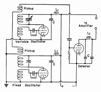
Fig. 1.—Circuits of a Beat Frequency Oscillator.
