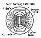
Fig. 1.—Element Arrangement in Beam Power Tube.
