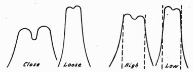
Fig. 5.—Peaks Secured with Changes in Coupling.
