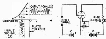
Fig. 1-A.—Class A Operating Characteristics.
