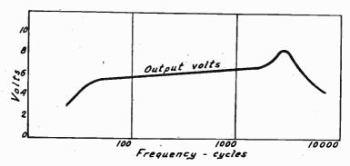
Fig. 5.—Result of Frequency Distortion in Amplifier.
