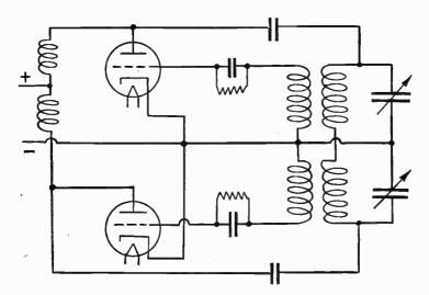
Frc. 12.—Two Oscillator Tubes with Single Resonant Circuit.
