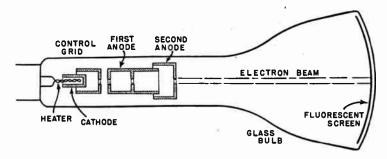
Fig. 1.—Principal Parts of a Cathode-ray Tube.
