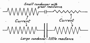
Fig. 4.—Effect of Large and Small Filter Condensers on Alternating Currents.
