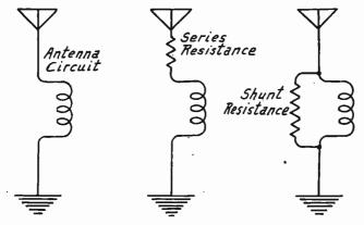
Fig. 2.—Equivalent Resistances in Antenna Circuit.
