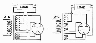
Fig. 3.—Full-wave Filament-cathode Rectifier.
