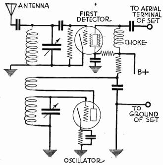
Fig. 6.—Superheterodyne Converter for Short Wave Reception
