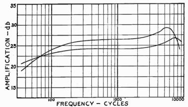
Fig. 8.—Amplification with Transformer Coupling.
