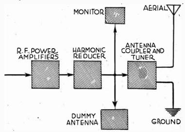
Fig. 3.—High Power Equipment Used at Transmitter.
