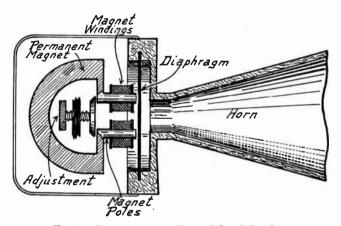
Fig. 1.—Electromagnetic Type of Loud Speaker.
