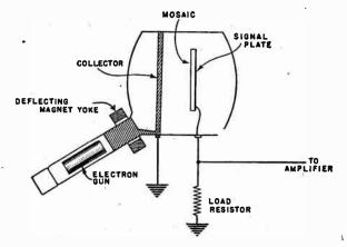
Fig. 1.—The Iconoscope or Camera Tube.
