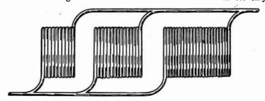
Fig. 4.—Inductance Coils in Parallel.
