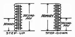
Fig. 1.—Principle of the Auto-Transformer.
