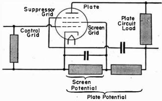
Fig. 2.—Typical Connections for Pentode Voltage Amplification.
