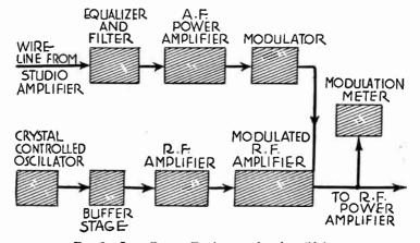
Fig. 2.—Low Power Equipment for Amplifying.
