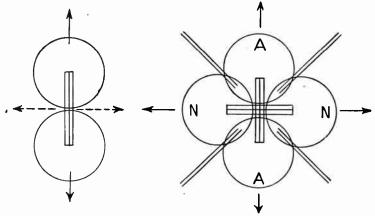
Fig. 4.—Radiation from Loop Antennas.
