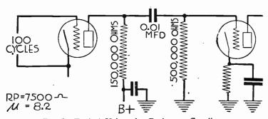
Fig. 5.—Typical Values for Resistance Coupling.
