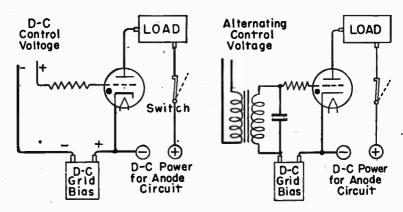
Fig. 3.—D-c Control of D-c Power for Load.
