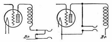
Fig. 3.—Jacks for Plate Current Meter (left) and Voltmeter (right).
