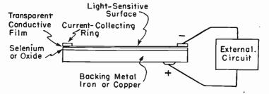
Fig. 1.—Principal Parts of Barrier Layer Photocells.
