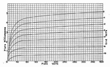
Fig. 4.—Plate Characteristics of a Voltage-amplifier Pentode.
