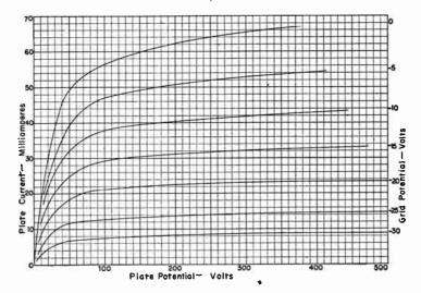
Fig. 1.—Plate Characteristics of a Power Pentode.
