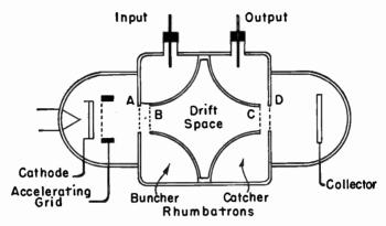
Fig. 1.—Arrangement of Elements in a Klystron.
