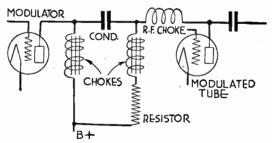
Fig. 13.—Separate Chokes for Modulator and Oscillator.
