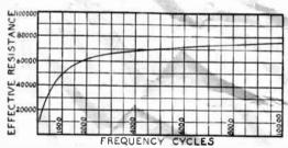
Fig. 6.—Frequency Effect on Apparent Resistance.
