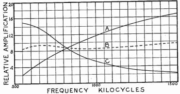
Fig. 4.—Effect of Primary Frequency on Amplification.
