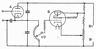
Fig. 7.—Electron-ray Tube Used as the Indicator for VT Voltmeter.
