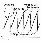
Fig. 4.—Neon Lamp in Relaxation Oscillator.
