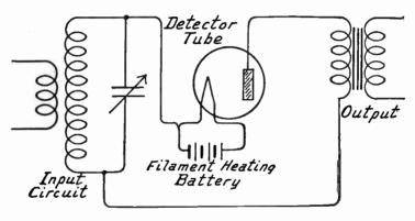
Elementary Principle of Diode Detector.
