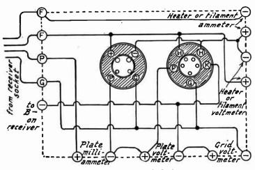
Fig. 9.—Test Board with Sockets.
