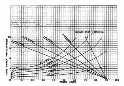
Fig. 9.-Load Lines Showing Phototube Performance.
