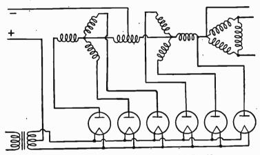
Fig. 3.—Three-phase Double-Y Parallel Rectifier.
