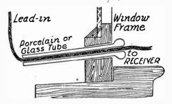
Antenna Lead-in Carried Through Tube.
