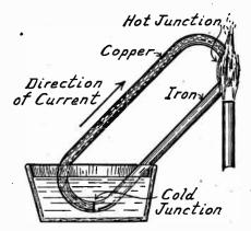
Fig. 1.—Principle of the Thermocouple.
