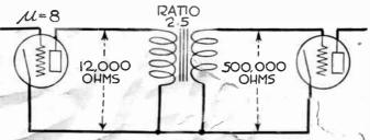
Fig. 3.—Simplified Diagram of Transformer Coupling.
