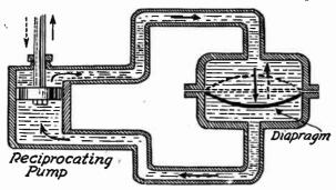
Fig. 5.-Hydraulic Explanation of Condenser Action.
