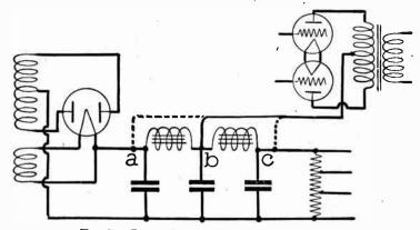
Fig. 7.—Connections of Plate Circuit to Filter.
