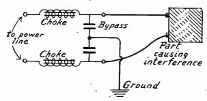
Fig. 8.—Interference Filter with Grounded Center Tap.
