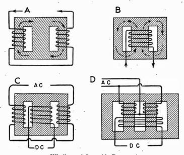
Windings of Saturable Reactors.
