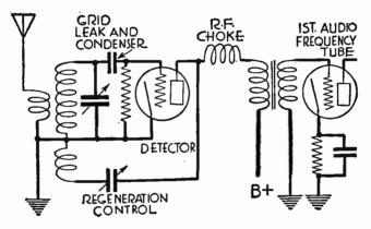
Fig. 4.—Regenerative Detector for Short Wave Reception
