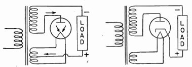
Fig. 1.—Tubes Used as Half-wave Rectifiers.
