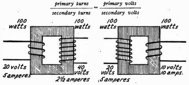
Fig. 7.—A Step-Up Transformer.
