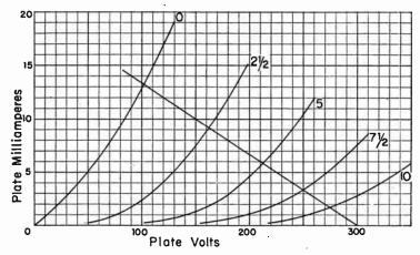
Load Line Used for Computing Voltage Amplification.
