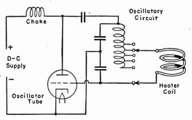
Fig. 2.—Simplified Circuit for Induction Heating.
