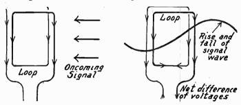
Fig. 2.—Equal Voltages Generated in Both Sides of Loop. Fig. 3.—The Phase Difference Allows a Net Voltage to Be Delivered by a Loop.
