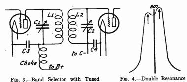
denser C2 and the coil L2. The grid circuit is completed through bypass condenser C4.
