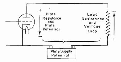
Fig. 5.—Relations of Supply Potential to Potential Drops.
