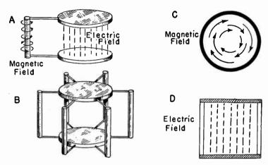
Fig. 1.—Principle of the Cavity Resonator.
