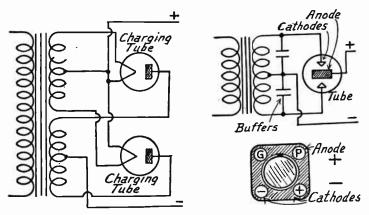
Fig. 3.—Charging Tubes Used as Filament Supply Rectifier.
