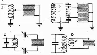
Fig. 2.—Electrode Arrangements for Electrostatic Heating.
