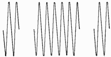
An Interrupted Continuous Wave.
