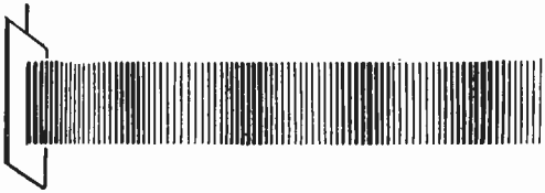
FIG. 1.—Radiation of Sound Waves from Vibrating Body.
