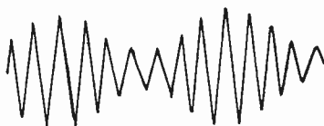
FIG. 3.—A Modulated Radio Wave.
