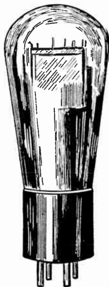
FIG. 4.—Large Type of Power Amplifier Tube.
