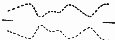
FIG. 4.—The Envelope of the Modulated Carrier.
