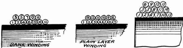
Placing of Turns in Bank and Layer Windings.
