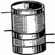
FIG. 5.—Air Core Radio Frequency Transformer.
