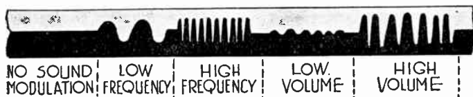
FIG. 4.—Changes in Variable Area Sound Track.
