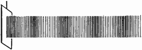
FIG. 1.—Radiation of Sound Waves from Vibrating Body.
