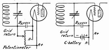
Fig. 4.—Detector Grid Bias with Potentiometer.
