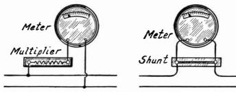
Fig. 3.-Multiplier Used with Voltmeter.
