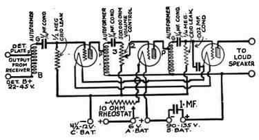
Fig. 1.—Circuits of Step-Up Impedance Coupled Amplifier.
