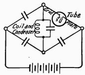
Fig. 6.—Balancing Principle of the Wheatstone Bridge.
