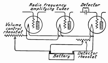
Fig. 1.—Volume Control with Radio Frequency Rheostat.
