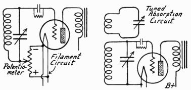
Fig. 15.—Potentiometer in Grid Return to Control Regeneration.
