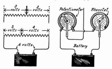
Fig. 2.—Division of Voltage with a Fig. 3.—Rheostat for Fine Control Potentiometer.
