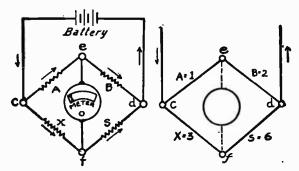
Fig. 1.—Principle of the Fig. 2.—Obtaining a Balance Wheatstone Bridge.
