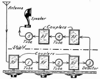
Fig. 3.—Shielding Between Radio Frequency and Audio Frequency Parts. and the couplers are evenly spaced. It is bad electrically and will usually be difficult to operate with any degree of satisfaction.
