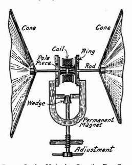
Fig. 4.—Speaker Mechanism Operating Two Cones.
