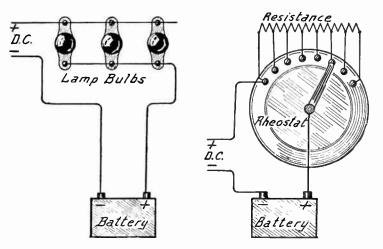
Fig. 1.—Direct Current Battery Charging with Lamp Resistance.
