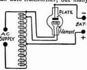
Fig. 1.—Bulb Type Battery arate winding, de Charger with Auto-Transformer. transformer design.
