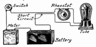
Fig. 2.—Testing for Short Circuit with Voltmeter.
