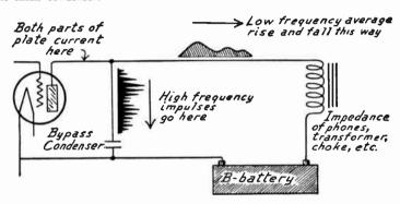
Separation of High and Low Frequencies with Detector Plate Bypass.
