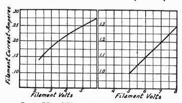
Fig. 1.—Effect of Filament Voltage on Filament Current.
