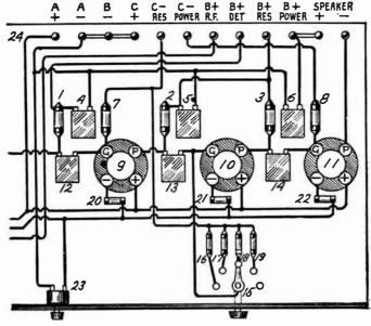
AUDIO AMPLIFIER WITH THREE-STAGE RESISTANCE COUPLING
