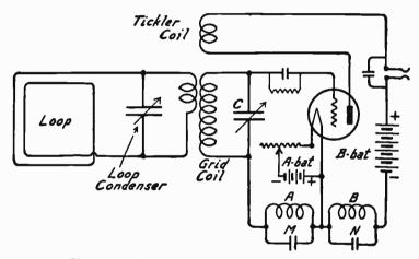
Circuits of Super-Regenerative Single Tube Receiver.
