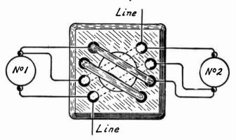
Fig. 1.—Special Form of Series-Parallel Switch.
