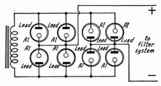
Fig. 5.—Electrolytic Rectifier with Cells in Parallel.
