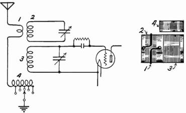
Circuits of Four-Circuit Receiver.
