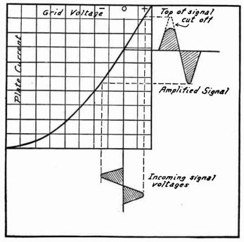
Fig. 2.—Distortion Caused by Zero Grid Bias.
