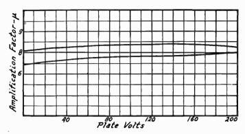
Fig. 16,-Effect of Plate Voltage on Amplification Factor.
