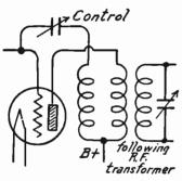
Fig. 21.—Roberts Circuit with Balancing Condenser Used as Regeneration Control.
