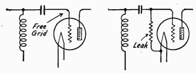
Fro. 3.—Grid Isolated by Condenser With No Leak in Use.
