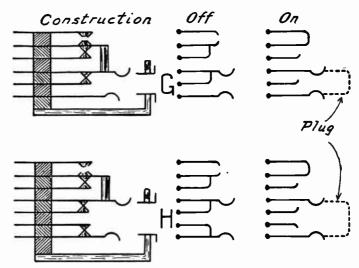
Fig. 3.—Jacks with Three Filament Control Contacts.
