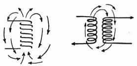
Fig. 7.—Electromagnetic Lines of Force Around a Coil.
