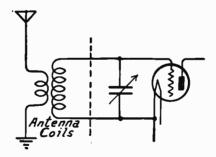
Fig. 2.—Loop Replaced with Antenna Coils.
