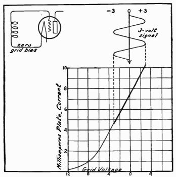
Fig. 1.—Effect of Zero Grid Bias, Distortion.
