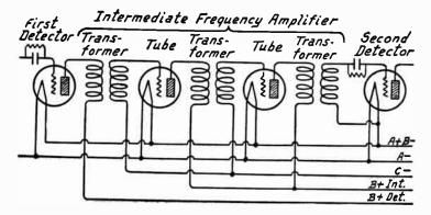
Fig. 4.—Two-Stage Intermediate Amplifier of Superheterodyne.
