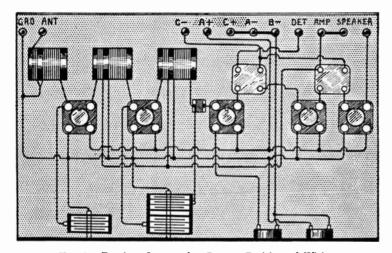
Fig. 3.—Receiver Layout for Correct Position of Wiring.
