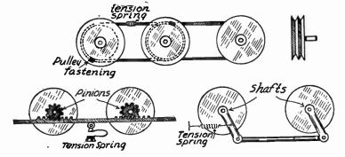
Fig. 3.—Single Control for Side-by-Side Tuning Units.
