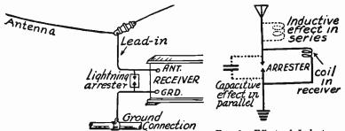
Fig. 1.—Connection of Lightning Arrester to Antenna and Ground.
