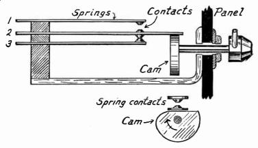
Fig. 4.—Operating Parts of a Jack Switch.
