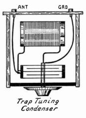
Fig. 2.—Layout of Impedance Wave Trap Unit.
