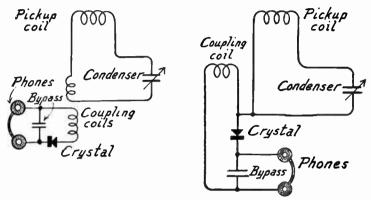
Fig. 7.—Inductively Coupled Indicator Circuit for Frequency Meter.
