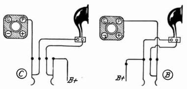
Fig. 21.—Jack for Completely Disconnecting Speaker.
