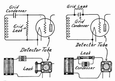
Fig. 1.—Grid Leak Connected to Detector Tube Terminals.
