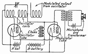
Fig. 3.-Modulation by Variation of Input Power.
