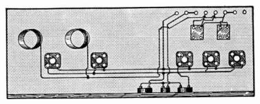
Fig. 14.—Filament and Plate Supply Wiring Arranged for Cabling in Receiver Construction.
