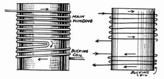
Bucking Coils or Bucking Windings.
