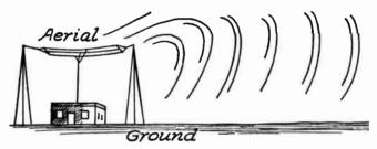
Fig. 1.—Radio Waves from an Aerial.
