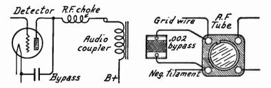
Fig. 12.—Radio Frequency Choke and Fig. 13.—Bypass in Grid Circuit of Bypass on Detector for Prevention Tube for Prevention of Oscillation.
