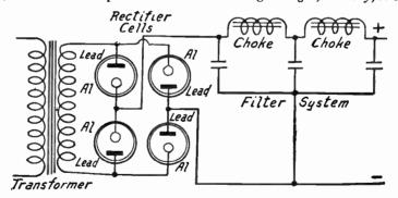
Fig. 4.—Power Unit with Electrolytic Rectifier.
