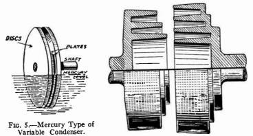
Fig. 6.-Dovetail Type of Variable Condenser.
