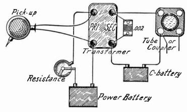
Fig. 6 .-- Using a Battery with Phonograph Pick-up Unit.
