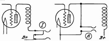
Fig. 17.—Jack for Plate Milliammeter.
