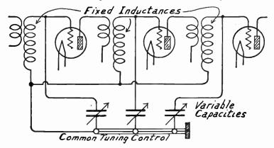
Fig. 1.—Single Control with Variable Condensers.
