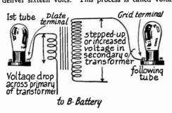
Fig. 1.-Voltage Amplification in a Transformer.
