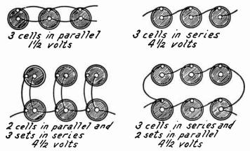
Dry Cell Connections for Increasing Voltage and for Increasing Allowable
