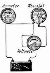
Fig. 1.—Determining Rheostat Resistance with Ohm's Law.
