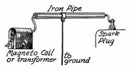
Fig. 6.—Shielding of Ignition Circuits to Prevent Interference.
