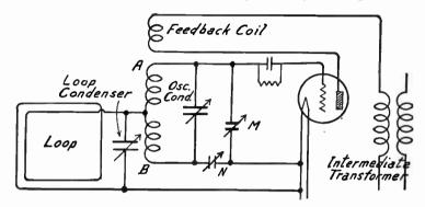
Fig. 8.-Autodyne Combination of Detector and Oscillator Tube.
