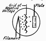
Fig. 9.—Effect of Negative Grid Voltage on Electron Flow.
