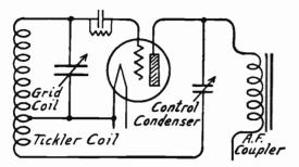
Fig. 9.—Condenser Control of Close Coupled Tickler.
