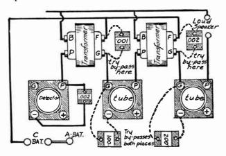
Fig. 7.—Bypassing Radio Frequency Currents in an Audio Amplifier.
