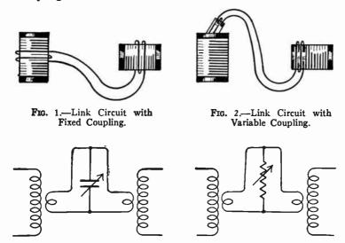
Fig. 3.—Variable Units in Shunt with Link Circuits.
