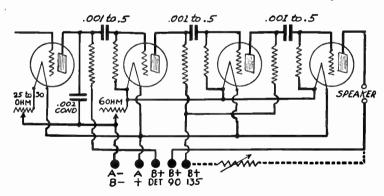
Fig. 4.—Circuit Diagram of Three-Stage Resistance Amplifier.
