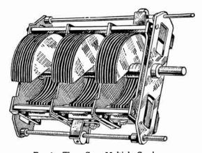
Fig. 3.—Three-Gang Multiple Condenser.
