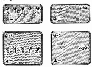
Terminal Arrangements on Dry Cell B-Batteries.
