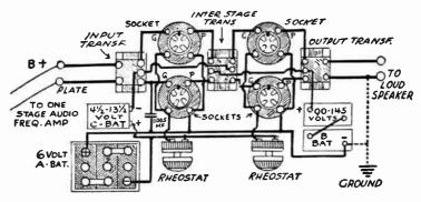
Fig. 3.—Two Stages of Push-Pull Amplification.
