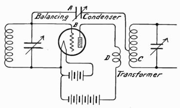
Fig. 3.—Neutrodyne Method of Balancing.
