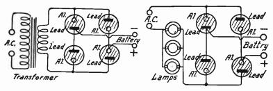
Fig. 2.—Electrolytic Battery Charging Rectifier with Transformer. Fig. 3.—Lamp Resistance with Electrolytic Battery Charging Rectifier.
