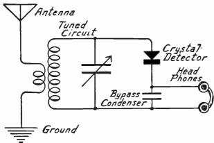
Fig. 2.—Simple Crystal Detector Circuit.
