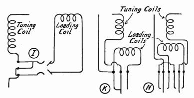
Fig. 28.—Jack for Insertion of Loading Coil.
