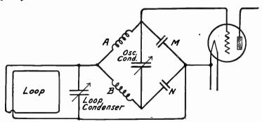
Fig. 9.—Bridge Circuit Equivalent of Autodyne Circuit.
