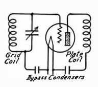
Fig. 1.-Grid and Plate Coils Entering into Regeneration.
