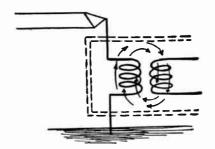
Fig. 9.—Coupled Coils as First Circuit in Receiver.
