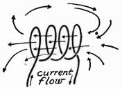
Fig. 3.—Electromagnetic Lines of Force around a Helix.
