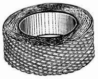
Fig. 1.—A Honeycomb Coil.
