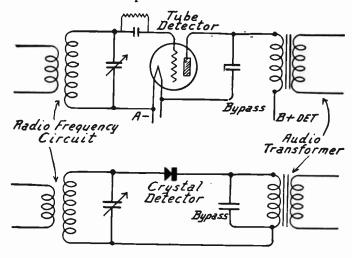
Fig. 5.—Substitution of Crystal for Tube Detector.
