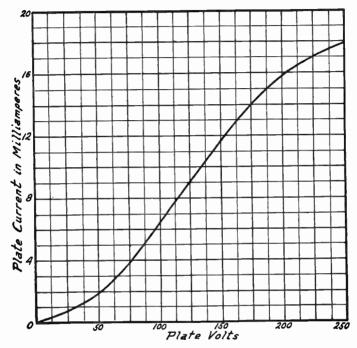
Fig. 11,-Effect of Plate Voltage on Plate Current.
