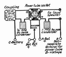
Fig. 1.—Connections for Tube in Power Amplifier.
