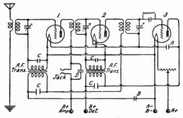
Fig. 5 .- Three-Tube Reflex Receiver.
