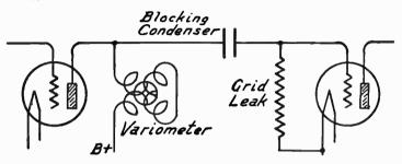
Fig. 1.—Tuned Impedance Coupling with Variometer.
