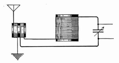
Fig. 2.—Separate Coupling Coil for Antenna Circuit.
