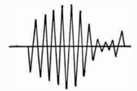
Fig. 6.—Equal Amplitudes of Modulated Carrier Wave Coming to Detector.
