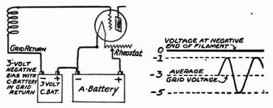
Fig. 4.—Negative Bias with C-Battery Alone.
