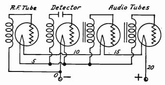
Fig. 9.—Grid Biasing with Five-Volt Tubes in Series.
