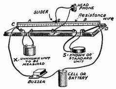
Fig. 5.—Practical Form of Slide Wire Bridge.
