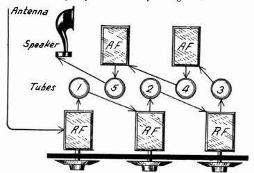
Fig. 4.—A Construction Which Is Poor Electrically.
