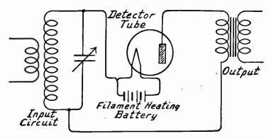
Fig. 3.—Two Element Rectifier Used as Detector.
