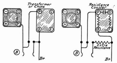
Fig. 1.—Jack for Phones or Speaker Fig. 2.—Jack for Insertion of Phones or Speaker with Resistance Coupling.
