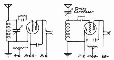
Fig. 1.—Single Circuit Receiver with Fig. 2.—Single Circuit Receiver with Parallel Condenser.
