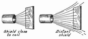
Fig. 7.-Effect of Distance Between Partial Shield and a Coil.
