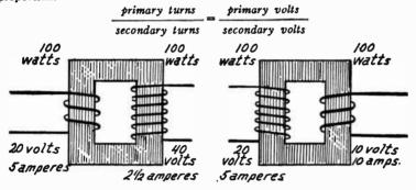
Fig. 7.—A Step-Up Transformer.
