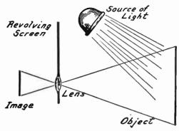
Fig. 1.—Producing the Image in Television.
