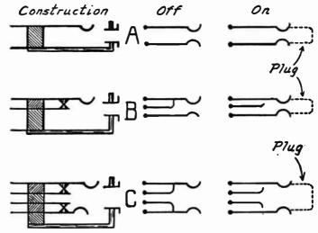
Fig. 1.—Operation of Jacks and Jack Switches.
