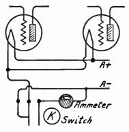
Fig. 15.—Switch for Filament Ammeter.
