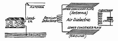
Fig. 2.—The Principle of the Capacity Antenna.
