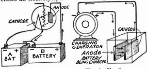
Anodes and Cathodes in Electric Circuits.
