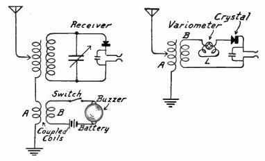
Fig. 3.—Circuit for Adjusting Crystal Contact.
