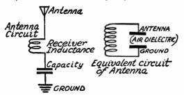
The Antenna Circuit and Its Electrical Equivalent.
