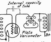
Fig. 17.—Regeneration with Plate Variometer.
