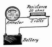
Fig. 2.—Determining Voltage Drop with Ohm's Law.
