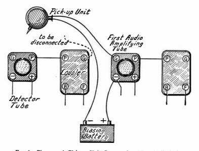
Fig. 3.—Phonograph Pick-up Unit Connected to First Audio Tube.
