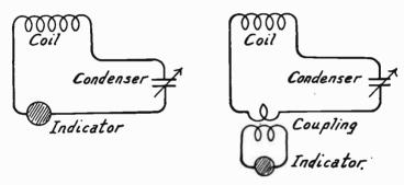
Fig. 1.—The Simplest Frequency Meter Circuit.
