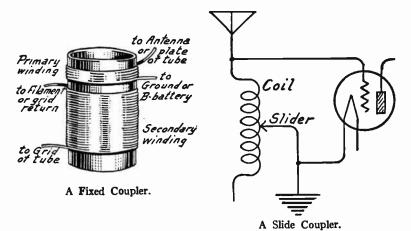
COUPLER, SLIDE.—A slide coupler consists of a coil of wire with which contact may be made at different points along the length of the coil by means of a slide contact. A slide coupler is used to insert more or less inductance in a tuned circuit. See also Coil, Slide Contacts on.
