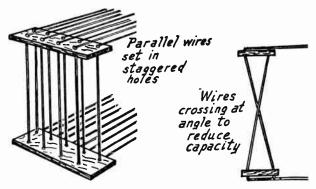
Arrangement of Wire on Loop Framework.
