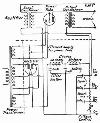
Fig. 1.—Complete Power Amplifier with Full Wave Rectifier.
