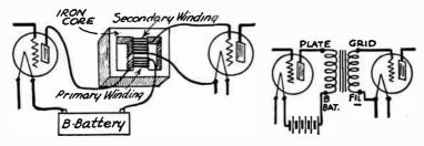
Fig. 1.—Transformer Coupling for Audio Frequency Amplifier.
