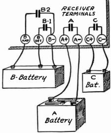
Fig. 3.—Connections of Bypass Condensers to Receiver Terminals. ties greater than those mentioned may be used for either radio frequency or audio circuits and for either grid or plate returns.
