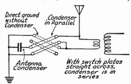
Series-Parallel Switch for Antenna Condenser.
