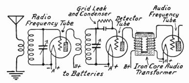
Fig. 22.—Audio Frequency Coupling with Iron-Core Transformer.
