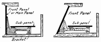
Fig. 12.—Sub-Panel Construction for Receivers.
