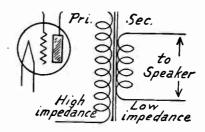
Fig. 2.—Matching Impedances with Special Transformer.
