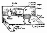
Coil with Proper Spacing Around All Sides.
