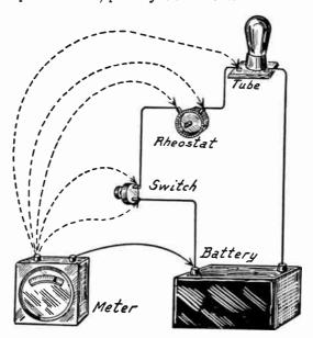
Fig. 2.—Testing Filament Circuit for Opens.
