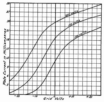
Fig. 5.-Effect of Grid Voltage on Plate Current.
