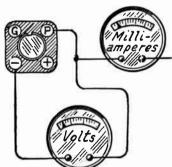
Fig. 3.—Testing Plate Voltage and Plate Current.
