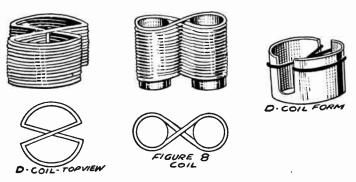
Fig. 2.—Coils of the Closed Field Type.
