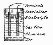
Fig. 1.—Parts of an Electrolytic Condenser.
