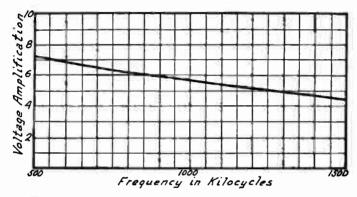
Fig. 3.—Decrease of Amplication with Increase of Frequency.
