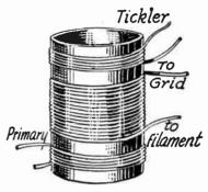
Fig. 5.—Construction of Fixed Tickler Coil for Regeneration.
