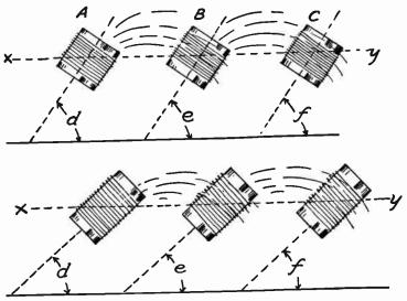
Fig. 4.—Coils at Angle at Minimum Coupling.
