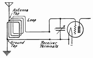
Fig. 1.—Using Antenna and Ground with a Loop.
