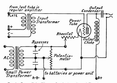
Fig. 7.—Power Tube Filament Supply from Tapped Transformer.
