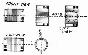
Fig. 2.—Coils Properly Aligned for Minimum Coupling Angle.
