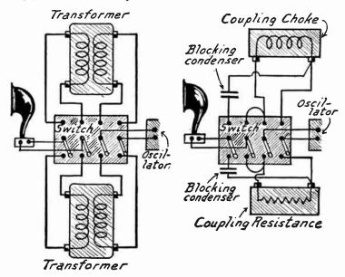
Fig. 1.—Comparative Test of Ampli- Fig. 2.—Comparative Test of Chokes fying Transformers with Audio or Resistances with Audio Oscillator.
