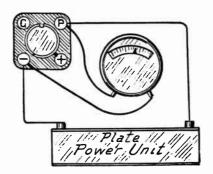
Measuring Applied Plate Voltage.
