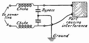
Fig. 8.—Interference Filter with Grounded Center Tap.
