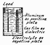
Fig. 2.—Electrolytic Condenser for Direct Current.
