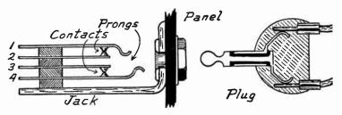
Fig. 1.—Construction of Jack and Plug.
