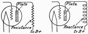
Fro. 2.—Tubes Working into Resistance and Into Reactance for Amplification.
