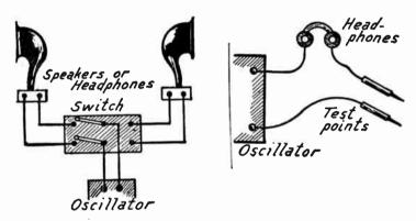
Fig. 3.—Comparison of Speakers or Headphones with Audio Oscillator.
