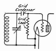
Fig. 5.—Grid Return Through Leak Across Grid Circuit.
