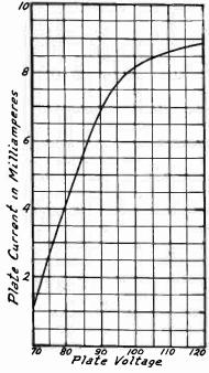
Fig. 4.—Limiting Plate Current by Lack of Emission.
