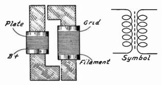
An Iron-Core Untuned Radio Frequency Transformer.
