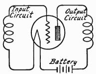
Fro. 3.—Tube Connected to Input and Output Circuits.
