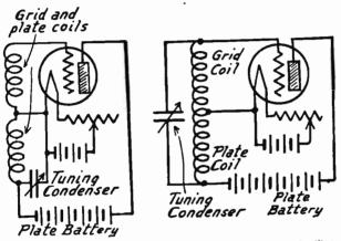
Fig. 1.—Radio Frequency Fig. 2.—Radio Frequency Oscillator with One Condenser for Both Oscillator with Tuned Coils. Plate Coil.
