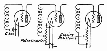
Fig. 2.—Grid Returns to C-Battery and Resistances.
