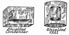
Fig. 4.—Tuning Condenser and Coil Enclosed in Shields.
