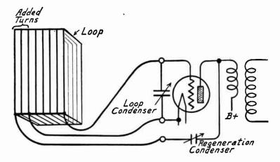
Fig. 19.—Regeneration Applied to a Loop.
