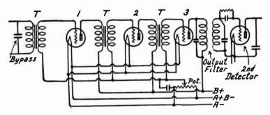
Frg. 12.—Intermediate Amplifier with Output Filter.
