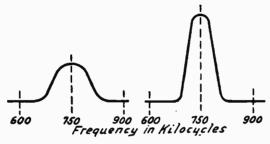
Fig. 3.—Effect of Regeneration on Signal.
