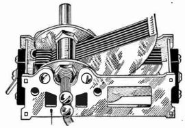
Fig. 7.—Modified Straight Line Frequency Condenser.
