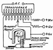
Fig. 2.—A Half-Wave Vibrating Battery Charger.
