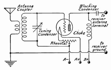
Fig. 3.—Circuit of Added Radio Stage Without Balancing.
