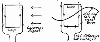
Fro. 2.—Equal Voltages Generated in Both Sides of Loop.
