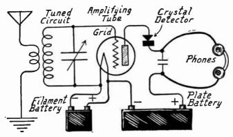
Fig. 17.—One-Tube Receiver with Crystal Detector.
