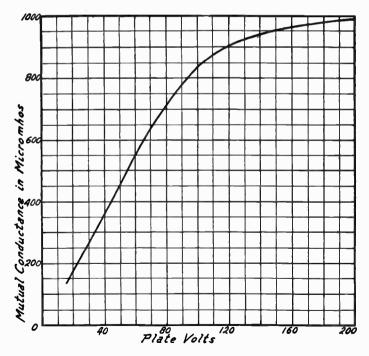
Fig. 17.—Effect of Plate Voltage on Mutual Conductance.
