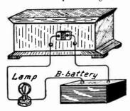
Incandescent Lamp for Protecting Tube Filaments.
