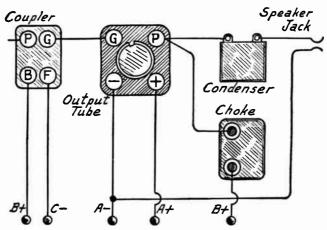
Fig. 4.—Connection of Condenser and Choke for Speaker.
