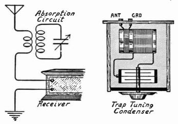
Fig. 1.—Circuit of Absorption Wave Trap.
