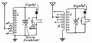
Fig. 1.—Simplest Type of Crystal Receiver.
