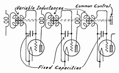
Fig. 2.—Single Control with Variable Inductances or Variometers.
