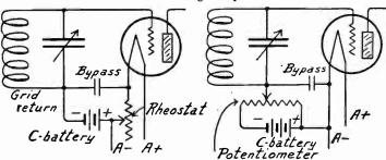
Fig. 6.—Detector Grid Bias with C-battery and Rheostat.
