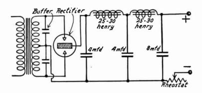
Fig. 5.—Full Wave Rectifying Tube for Filament Supply.
