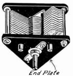
Fig. 4.—Condenser Designed with Dielectric End Plates.
