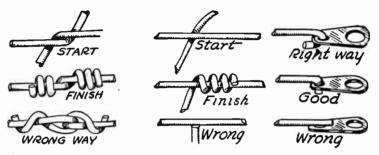
Fig. 1.—Making Joint Between Two Wire Ends in Soldering.
