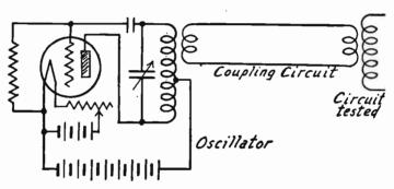
Fig. 3.-Link Circuit for Radio Oscillator Coupling.
