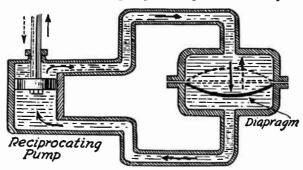
Fig. 5.—Hydraulic Explanation of Condenser Action.
