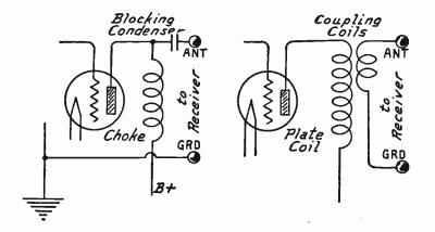
Fig. 5.—Output Choke and Blocking Condenser for Added Radio Stage.
