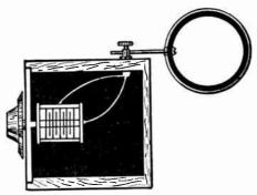
Fig. 11.-Frequency Meter with Shielded Cabinet.
