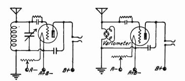
Fig. 1.—One-Tube Single Circuit Receiver.
