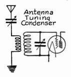
Fig. 1.—Connection of Series Condenser for Antenna Tuning.
