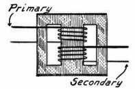
Fig. 3.—Shell Type Transformer.
