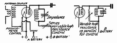
Fig. 2.—Oscillation Control for Radio Amplifier with Potentiometer and with Resistance in Plate Circuit.
