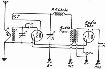
Fig. 2.—Second Type of Short Wave Receiver.
