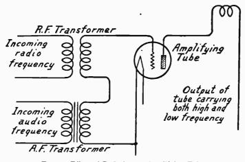
Fig. 1.—Effect of Reflexing on Amplifying Tube.
