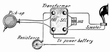
Fig. 7.—Phonograph Pick-up Connected Through Transformer to a Speaker.
