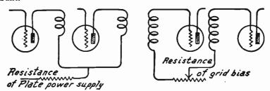
Fig. 3.—Feedback through Plate Sup- Fig. 4.—Feedback through Grid Bias Resistance to Cause Oscillation. ply Resistance to Cause Oscillation.
