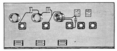
Fig. 15.—Regeneration Controls Kept Away from Panel in Receiver Construction.
