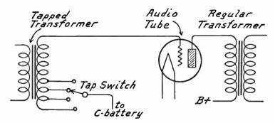
Fig. 5.—Volume Control with Tapped Secondary in Transformer.
