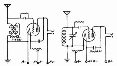
Fig. 3.—Single Circuit Receiver with Variometer Tuning.
