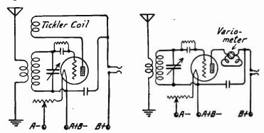
Fig. 3.—One-Tube Receiver with Tickler Coil Regeneration.
