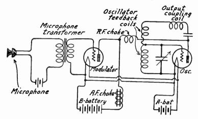
Fig. 2.—Absorption Method of Modulation.
