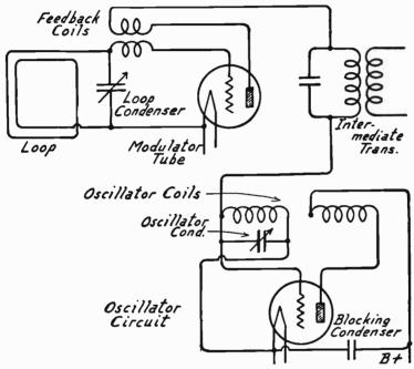
Fig. 10.—Circuits of Ultradyne Frequency Changer.
