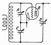
Fig. 8.—The Isofarad Method of Balancing.
