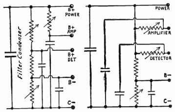
Fro. 1.—Obtaining Grid Biasing Voltage from Plate Supply Unit in Complete Receiver Supply Type of Power Unit.
