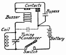
Fig. 1.—Circuits of Buzzer Type Oscillator.
