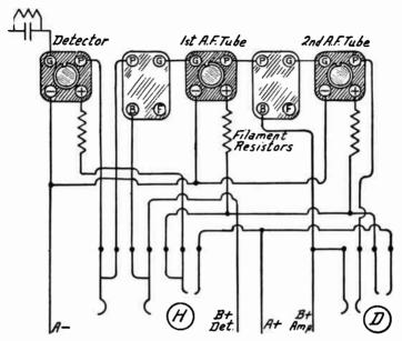
Fig. 9.—Filament Control Jack Following Detector Tube.
