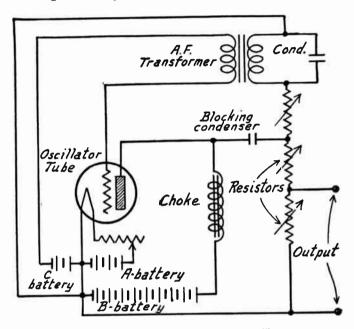
Fig. 2.—Circuits of Practical Audio Oscillator.
