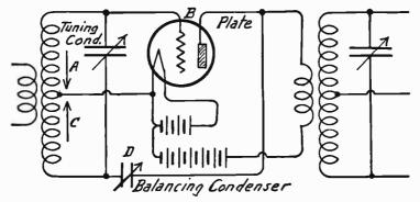
Fig. 5.—Rice Method of Balancing.
