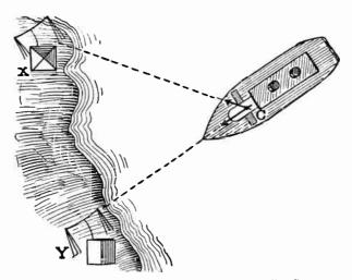
Fig. 2.—Determining Ship's Position with Radio Compass.
