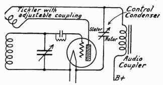
Fig. 7.—Variable Bypass Condenser for Regeneration Control.
