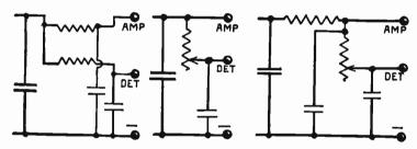
Fig. 1.—Plate Voltage Control Resistors in Series with Receiver Lines.
