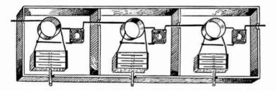
Fig. 5.—Amplifying Stages Enclosed in Individual Shields.
