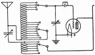
Fig. 1.—Tuner of the Reinartz Type.
