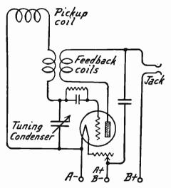
Fig. 10.—Circuits of Autodyne Frequency Meter.
