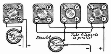
Fig. 1.—Rheostat in Negative Line (Left) and Single Rheostat for Three Tubes in Parallel (Right).
