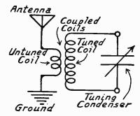
Fig. 11.-Tuned Circuit Coupled to Antenna Circuit.
