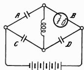
Fig. 9.—The Isofarad Balanced Circuit in Bridge Form.
