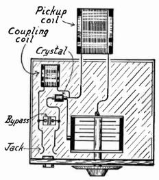
Fig. 9.—Layout for Frequency Meter with Special Indicator Coupling. energy may be introduced into the coupled circuit by mounting a metal plate about two by three inches or three inches square near the stator plates of the frequency meter condenser and connecting this plate to a point in the coupled circuit. This circuit was designed at the Bureau of Standards.
