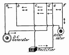
Fig. 2.—Three Electric Circuits with a Common Return.
