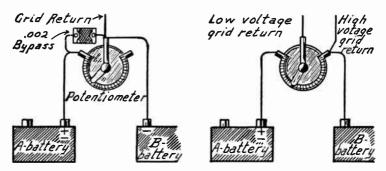
Fig. 7.—Single Biasing Voltage from Potentiometer.
