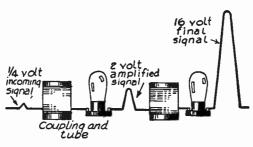
Fig. 2.—The Action of Voltage Amplification.
