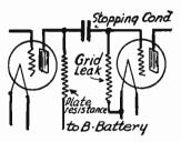
Fig. 2.—Circuits of Resistance Coupled Amplifier.
