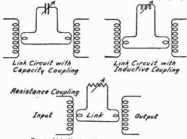
Fig. 4.—Link Circuits with Adjustable Couplings.
