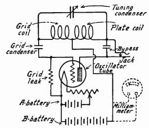
Fig. 4.—Circuits of Radio Frequency Oscillator.
