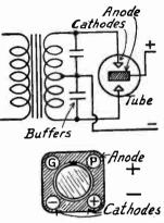
Fig. 8.—Connections for Raytheon Rectifier.
