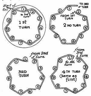
Fig. 2.—First Four Turns of a Basket Winding.
