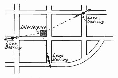
Fig. 2.—Locating Interference with Portable Receiver.
