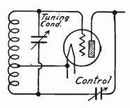
Fig. 22.—Rice Circuit with Regeneration Control.
