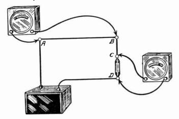
Fig. 1.—Principle of Testing for Open Circuits.
