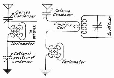
Fig. 4.—Variometer and Series Condenser for Antenna.
