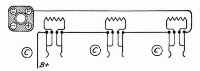
Fig. 25.—Plug-In Outlets with Compensating Resistances.
