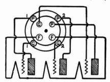
Fig. 2.—Internal Connections of Multiple Element Tube.
