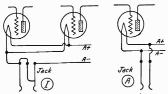
Fig. 13.—Jack for Filament Ammeter.
