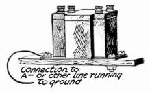
Fig. 8.—Grounding the Shield of an Audio Amplifying Transformer.
