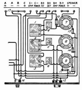
AUDIO AMPLIFIER WITH THREE-STAGE AUTOFORMER COUPLING.
