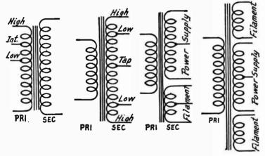
Fig. 2.—Types of Tapped Transformers for Power Units.
