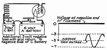
Fig. 3.—Negative Bias with C-Battery and Resistor.
