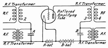
Fig. 2.—Circuits of Reflexed Amplifying Tube.
