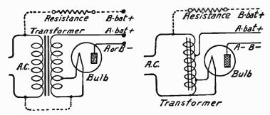
Fig. 2.—Bulb Type Battery Charger with Double Winding Transformer.
