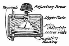
Fig. 1.—Screw Type of Variable Condenser.
