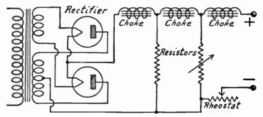
Fig. 4.—Filament Supply with Resistors in Filter System.
