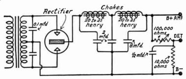
Fig. 6.-Full Wave Rectifier with Two Chokes in Filter.
