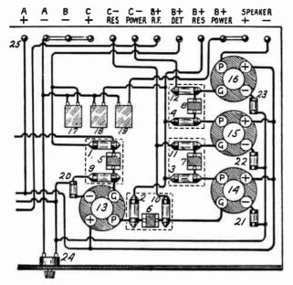
AUDIO AMPLIFIER WITH FOUR-STAGE RESISTANCE COUPLING
