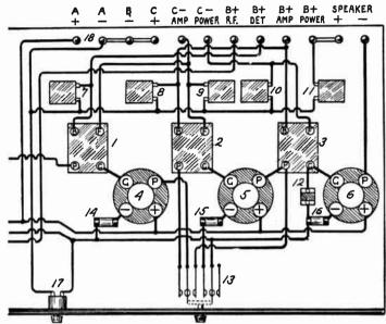
AUDIO AMPLIFIER WITH THREE TRANSFORMER STAGES AND SWITCH CONTROL
