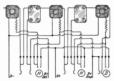
Fig. 10.—Filament Control Jacks for All Stages.
