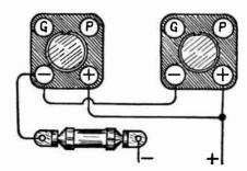
Fig. 2.—Single Filament Resistor for Two Tubes.
