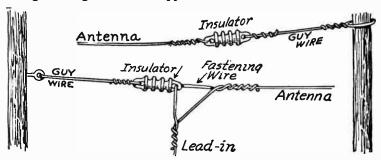
Fig. 1.—Installation of Antenna Insulators.
