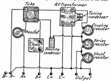
Fig. 3.—Layout for Practical Audio Oscillator.
