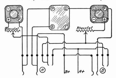
Fig. 6.—Filament Control Jacks on Two Stages.
