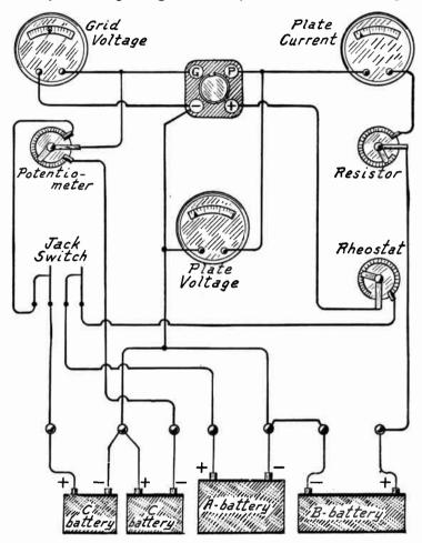
Fig. 4.—Tube Tester with Three Meters.
