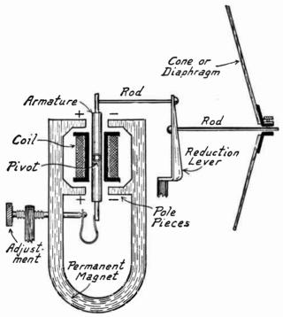
Fig. 3.-Balanced Armature Type of Loud Speaker.
