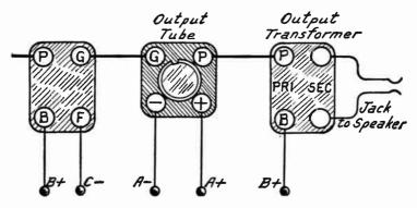
Fig. 8.—Connection of Output Transformer for Speaker.
