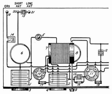
BROWNING-DRAKE RECEIVER (With 3-volt radio frequency tube)
