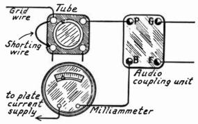
Fig. 14.—Testing Plate Current for Oscillation.
