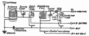
Fig. 4.—Circuits of Impedance Coupled Radio Amplifier.
