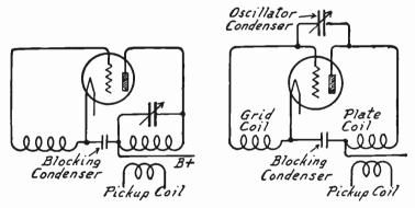
Fig. 6.—Oscillator with Tuned Plate Fig. 7.—Oscillator with Tuning Con-Circuit in Superheterodyne.
