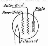
Four-Element Tube with Two Grids.
