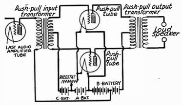
Fig. 1.—Circuits of the Push-Pull Amplifier.
