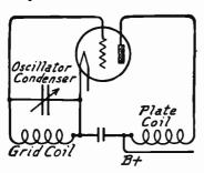
Fig. 2.—Simple Form of Oscillator Used in Superheterodyne.
