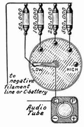
Fig. 4.—Resistor Units for Volume Control.
