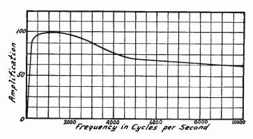
Fig. 5.—Curve for Poor Audio Transformer Drawn on Arithmetical Scale.
