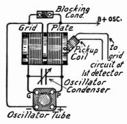
Fig. 14.—Oscillator Coupler for Superheterodyne.
