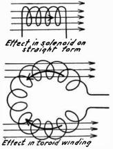
Fig. 3.—Opposing Voltages Set Up in Toroid Winding.
