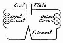
Fig. 4.—Tube Elements Represented as Capacity.
