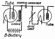
Fig. 1.—The Impedance Coupled Audio Amplifier.
