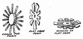
Fig. 1.-Forms for Spiderweb Coil Windings.
