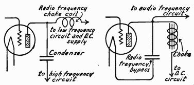
Fro. 1.—Separation of Frequencies with a Choke Coil.
