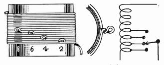
Construction of a Tapped Coil.
