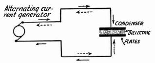
Fig. 6.-Flow of Alternating Current Through a Condenser.
