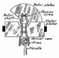
Fig. 2.—Cam Vernier for Moving Condenser Rotor Plates.
