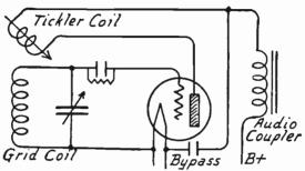
Fig. 1.—Regeneration Obtained with Movable Tickler Coil.
