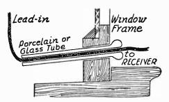
Antenna Lead-in Carried Through Tube.
