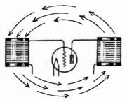
Fig. 7.—Feedback Coupling between Parallel Coils Causing Oscillation.
