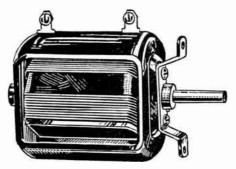
Fig. 2.—Variometer with Rectangular Windings.
