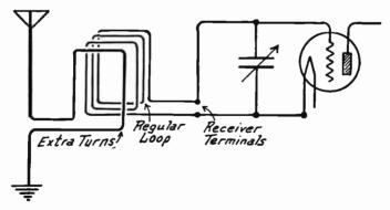
Fig. 2.-Additional Turns for Antenna with Loop.
