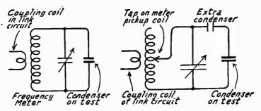
Fig. 3.—Matching Fixed Condensers with Radio Oscillator.
