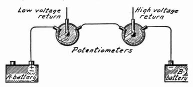
Fig. 9.—Two Variable Biases from Potentiometers.
