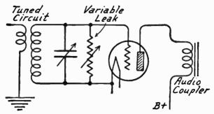
Fig. 14.—Variable Grid Leak Controlling Regeneration.
