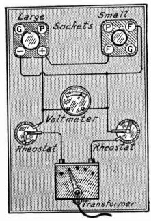
Fig. 1.—Tube Restorer with Transformer.
