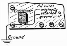
Fig. 3.—Connection of Ground Condenser.
