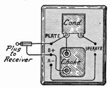
Fig. 5.—Condenser and Choke Unit for Speaker Connection.
