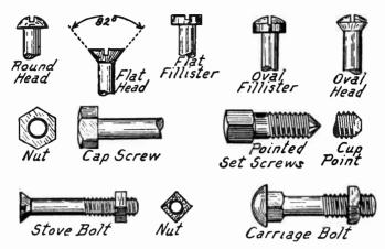
Screws and Bolts Used in Construction Work.
