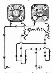
Fig. 8.—Filament Control with Two Tubes in Operation.
