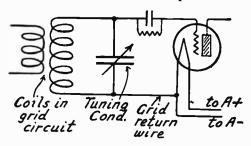
Fig. 1.—Negative Grid Return for Gas Content and Soft Detector Tubes.
