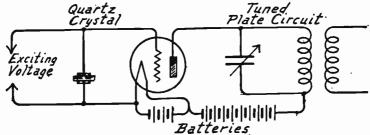
Fig. 2.—Crystal Control of Grid Circuit Frequency.
