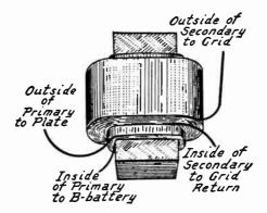
Fig. 6.-Windings and Connections of Audio Frequency Transformer.
