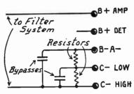
Fig. 11.—Two Grid Biases from Single Plate Voltage Supply.
