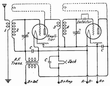
Fig. 4.—Reflex Receiver with Tube Detector.
