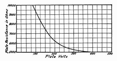
Fig. 15.—Plate-Voltage, Plate-Resistance Curve with Changing Grid Bias.
