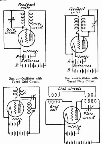
Fig. 5.—Oscillator with Part of Plate Coil in Tuned Circuit.
