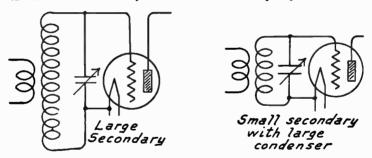
Fig. 4.—Large Secondary Giving Increased Power or Voltage.
