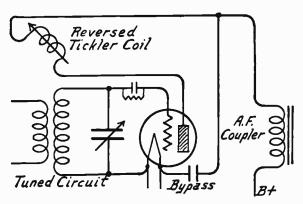
Fig. 3.—Reversed Feedback for Regeneration Control.
