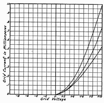
Fig. 10.—Grid Voltage Effect on Grid Current.
