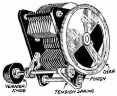
Fig. 3.—Geared Vernier for Tuning Condenser.
