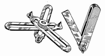
Fig. 1.—Adjustable Template and Adjustable Square.
