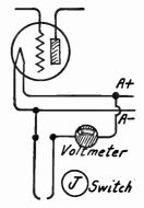
Fig. 16.—Switch for Filament Voltmeter.
