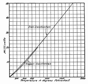
Fig. 2.—Voltage Developed by Thermocouples.
