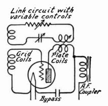
Fig. 10.—Link Circuit Control of Regeneration.
