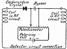
Fig. 5.—Use of Polarizing Battery with Crystal Detector.
