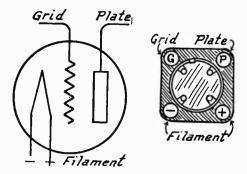
Fig. 5.—Symbol for Tube and Terminals on Socket.
