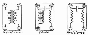
Fig. 5.—Similarity of Terminal Connections with Various Couplers.
