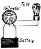
Fig. 3.—Determining Current with Ohm's Law.
