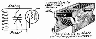
Connections to Rotor and Stator of Condenser.
