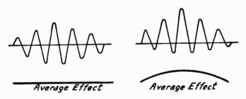
Fig. 19.—Voltages as Received by Detector Tube.
