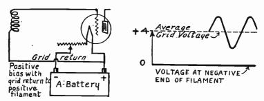
Fig. 6.—Obtaining Positive Grid Bias.
