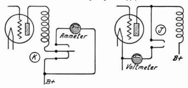
Fig. 19.—Switch for Plate Milliammeter.
