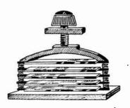
Fig. 3.—Compression Type of Variable Condenser.
