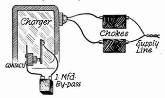
Fig. 5.—Handling Interference of Vibrators and Flashers.
