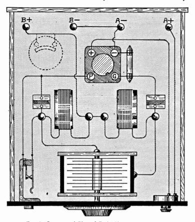
Fig. 5.—Layout and Plan of Radio Frequency Oscillator.
