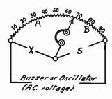
Fig. 3.—Functions of the Arms in a Bridge.
