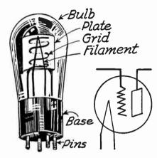
Fig. 15.—The Vacuum Tube and Its Symbol.
