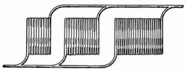
Fig. 4.—Inductance Coils in Parallel.
