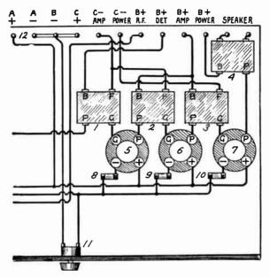
AUDIO AMPLIFIER WITH DOUBLE IMPEDANCE COUPLING.
