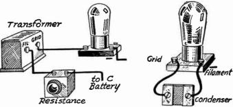
Fig. 5.—Resistance for Securing Uniform Amplification and Reducing Distortion.
