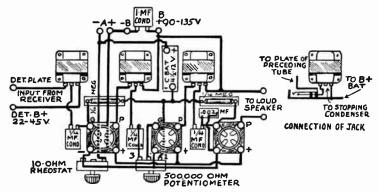
Fig. 2.—Layout of Step-Up Impedance Amplifier.
