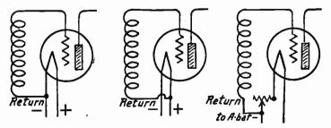
Fig. 1.—Grid Returns to Filament or Battery Lines.
