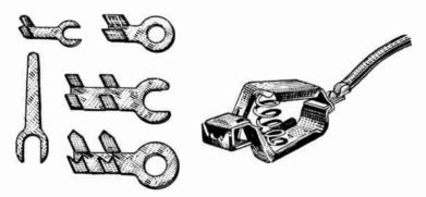
Fig. 5.—Wiring Terminals.
