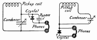
Fig. 5.—Frequency Meter with Direct Coupled Indicator Circuit.
