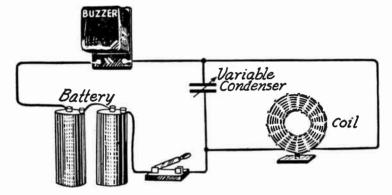
Fig. 2.—Layout of Buzzer Oscillator.
