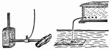
Fig. 1.—Cold Water Pipe Receiver Ground.
