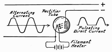
Fig. 1.—Action of Half-Wave Rectifying Tube.
