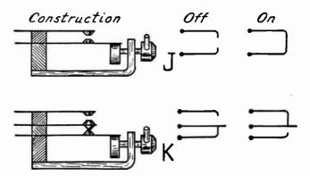
Fig. 5.—Single Pole Jack Switches.
