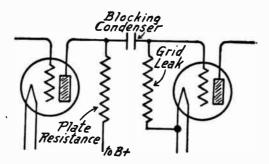
Fig. 6.—Grid Return Through Leak with Resistance Coupling.
