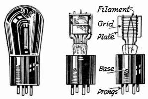
Fig. 1.-- A Vacuum Tube and Its Principal Parts.
