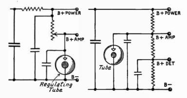
Fro. 3.—Voltage Regulator Tube on Intermediate Plate Voltage.
