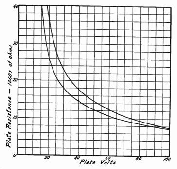
Frc. 13.-Effect of Plate Voltage on Plate Resistance in Amplifier Tubes.
