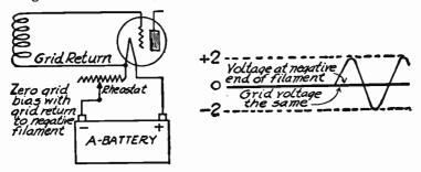
Fig. 1.—Zero Bias with Grid Return to Negative of Filament.
