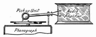
Fig. 2.—Phonograph Pick-up Unit Connected to an Amplifier.
