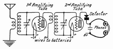
Fig. 18.—Two Stages of Amplification Before the Detector.
