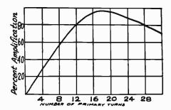
Fig. 2.—Effect of Primary Turns on Radio Frequency Amplification.
