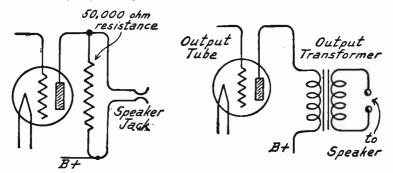
Fig. 6.—Bypassing Resistance for Speaker Connection.
