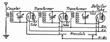
Radio Frequency Circuits of Tuned Radio Frequency Receiver.
