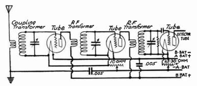
Fig. 7.—Circuits of Two-Stage Tuned Transformer Radio Amplifier.
