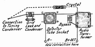
Fig. 6.-Using Crystal in Place of Tube Detector.
