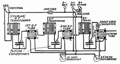
Fig. 6.—Arrangement of Parts in Two-Stage Tuned Transformer Type of Radio Amplifier.
