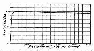
Fig. 4.—Curve for Good Audio Transformer Drawn on Arithmetical Scale.
