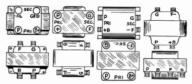
Fig. 2.—Terminal Arrangements on Audio Transformers for Amplifiers.
