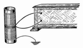
Resonance Wave Coil for Antenna.
