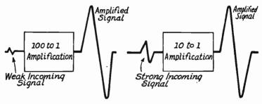
The Effect of Amplification on Signal Strength.
