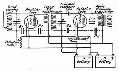
Fig. 2.—Bypass Condensers in a Receiver.
