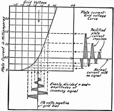
Fig. 1.—Action of Detector Using Grid Bias for Plate Current Rectification. one-half milliampere. Assuming that the grid biasing voltage, or the grid's voltage with no signal coming in, is one and one-half volts negative, the steady plate current that flows under this condition is one-half milliampere.
