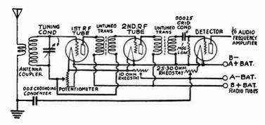
Radio Frequency Amplifier with Untuned Transformers.
