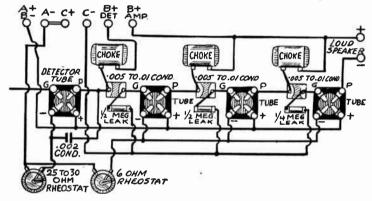
Fig. 2.—Three-Stage Impedance Amplifier Starting with the Detector.
