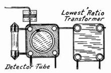
Fig. 3.—High Impedance Couplers Should Follow the Detector for Matching.
