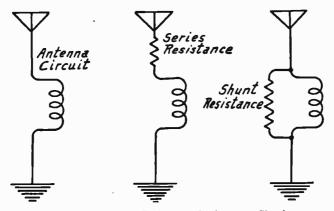
Fig. 2.—Equivalent Resistances in Antenna Circuit.
