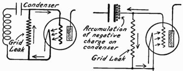
Fig. 4.—Path of Grid Current in Detector with Grid Condenser.
