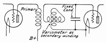
Fig. 2.—Variometer Used as Secondary of Tuned Transformer for Coupling.
