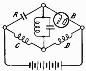
Fig. 10.—The Neutrodyne Balanced Circuit in Bridge Form.
