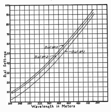
Fig. 1.—Calibration Curves for Wavelength.
