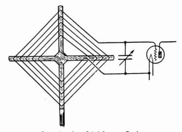
Connections from Spiral Loop to Receiver.
