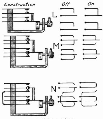
Fig. 6.—Double Pole Jack Switches.
