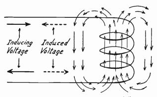
Fig. 1.—Effect of Self-Inductance in a Coil.
