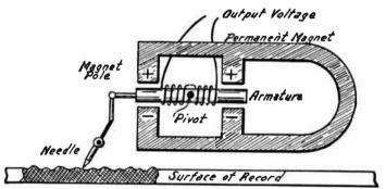
Fig. 1.—Principle of the Phonograph Amplifier Unit.
