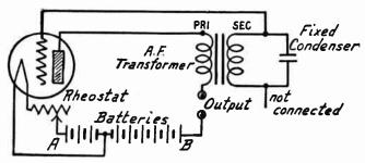
Fig. 1.—Simple Form of Audio Oscillator.
