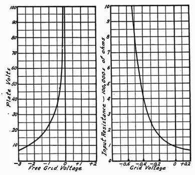
Fig. 8.—Effect of Plate Voltage on Free Grid Voltage.
