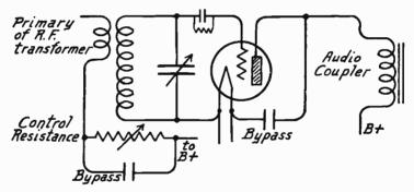
Fig. 11.—Regeneration Control with Plate Circuit Resistance.
