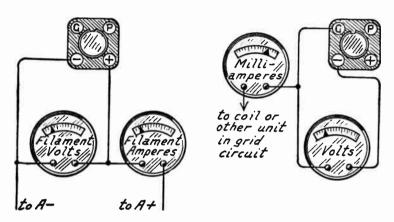
Fig. 1.—Testing Filament Voltage and Amperage.
