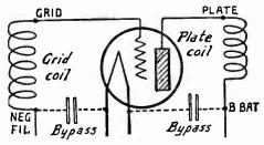
Fig. 1.—Grid Circuit and Plate Circuit Bypass Condensers.
