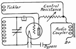
Fig. 6.—Fixed Tickler Control with Shunt Resistance.
