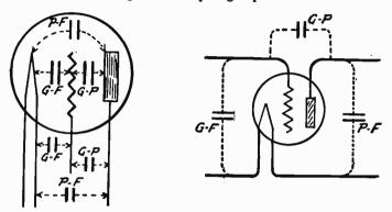
Fig. 1.—Internal Capacities of a Tube.
