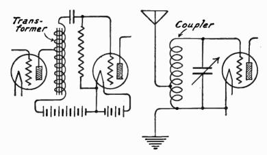
Fig. 3.—Auto-Transformer Interstage Coupling.
