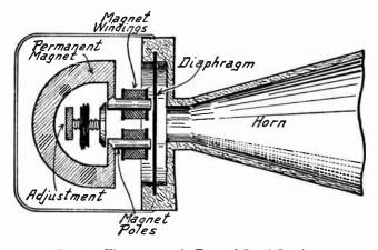
Fig. 2.—Electromagnetic Type of Loud Speaker.
