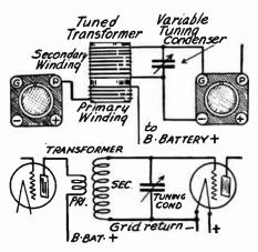
Fig. 1.—Tuned Transformer Coupling for Radio Amplifier.
