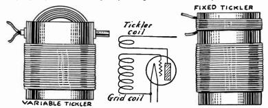
Fig. 1.—Connection of a Tickler Coil.
