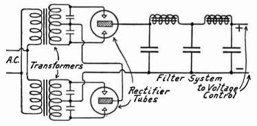
Fig. 9.—Two Standard Rectifiers and Transformers in Series for High Voltage
