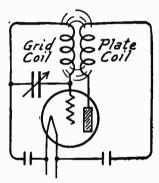
Frg. 2.-Feedback from Plate Circuit to Grid Circuit Causing Regeneration.
