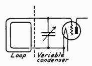
Fig. 1.—Tuned Loop Connected to Amplifying Tube.
