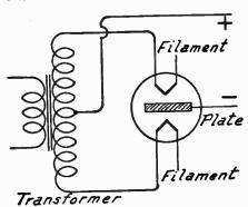
Fig. 2.—Connections of Full-Wave Rectifying Tube.
