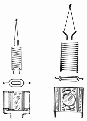
Fig. 1.—Design of an Early Type of Amplifier Tube.
