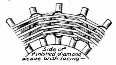
Fig. 3.—Lacing the Finished Diamond Weave Spiderweb Coil.
