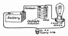
Fig. 1.—Electrolytic Battery Charging Rectifier.
