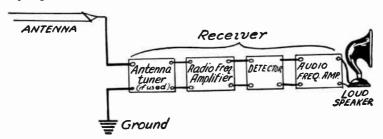
Position of the Radio Frequency Amplifier in a Receiver.
