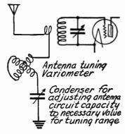
Fig. 2.—Use of Variometer for Antenna Tuning.
