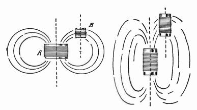
Fig. 3.—Field Lines of Force Passing at Right Angles Through a Coil. the two coils must intersect at right angles and the second point is that the center lines must intersect at the center of the length of the winding on one coil.
