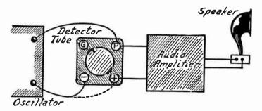
Fig. 5.—Testing Complete Audio Amplifier with Audio Oscillator.
