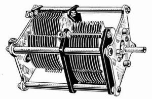
Fig. 1.-- A Two-Part Tandem Multiple Condenser.
