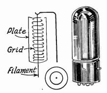
Fig. 4.—Construction of Dry Cell Tube.
