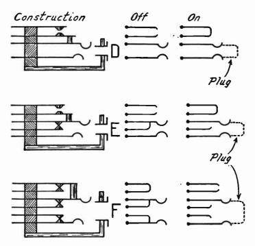
Fig. 2.- Jacks with Two Filament Control Contacts.
