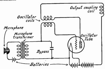
Fig. 1.—Grid Modulation of Oscillator Tube.
