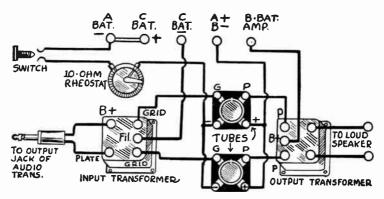
Fig. 2.—Layout for Single Stage of Push-Pull Amplification.
