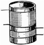
FIG. 5.—Air Core Radio Frequency Transformer.
