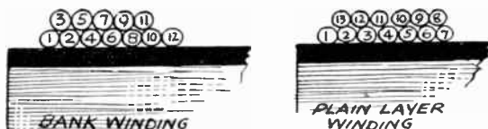
FIG. 1.—Bank Winding of Two-Layer Coil.
