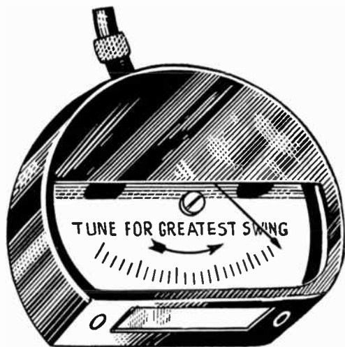
FIG. 11.—Reversed Scale Meter Tuning Indicator
