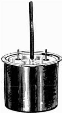
FIG. 6.— Developmental "tin can" Vacuum Tube
