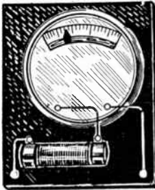
FIG. 5.—Milliammeter Used as Voltmeter.
