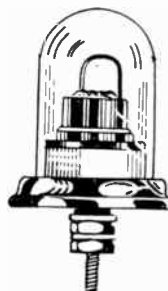
FIG. 4.—Crystal Detector with Fixed Cat Whisker.
