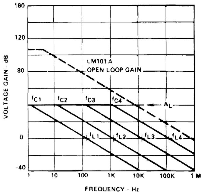
$A_L$  (VOLTAGE GAIN BELOW BREAK FREQUENCY)
