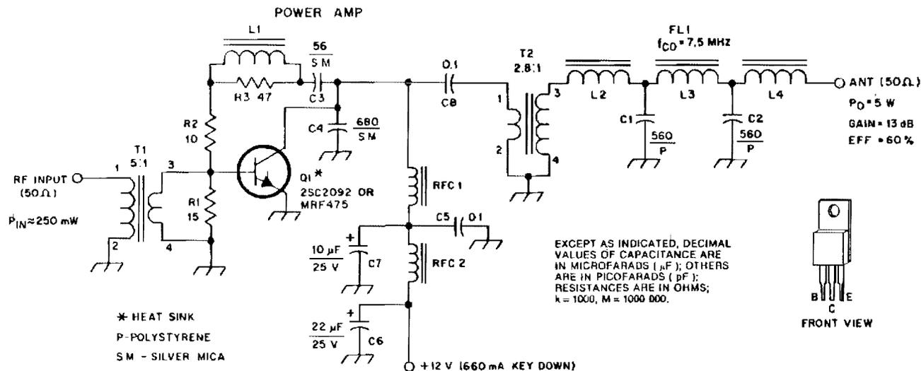
L1—0.22- $\mu\text{H}$  inductor. Small RF choke or 8 turns of no. 24 enam wire on an Amidon T-37-6 toroid.
