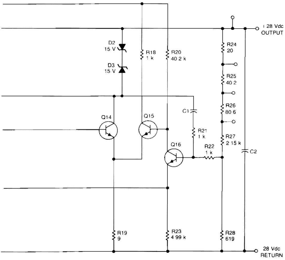
through Q16. The other input of the amplifier is connected to a radiation-hardened zener diode, D1. Local feedback using R21 and C1 produces gain to phase shift that are independent of individual component parameters, which provides stable operation into the required loads.
