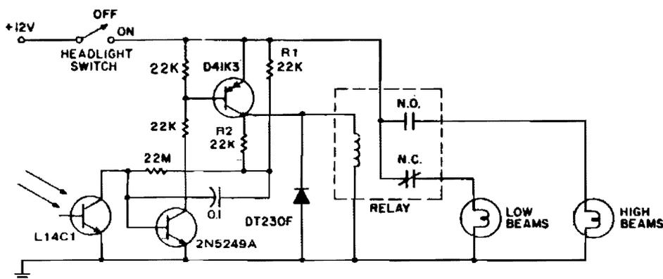
**RELAY:** 12V, 0.3A COIL; 20A, FORM C, CONTACTS OR SOLID-STATE SWITCHING OF 16A STEADY-STATE 150A COLD FILAMENT SURGE, RATING.
