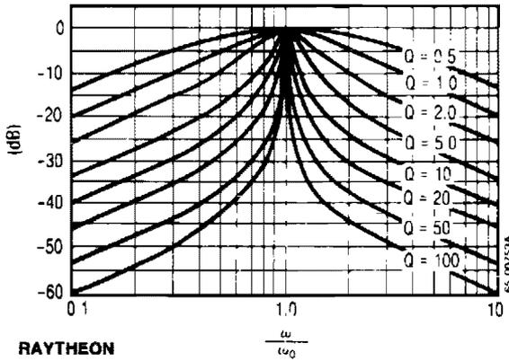
$$V_{BP} = \frac{\frac{\omega}{\omega_0} \frac{1}{Q}}{\sqrt{\left[1 - \left(\frac{\omega}{\omega_0}\right)^2\right]^2 + \left(\frac{1}{Q} \frac{\omega}{\omega_0}\right)^2}} V_{IN}$$
