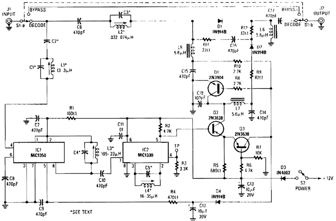
—FOR THE OUTBAND DECODER shown here to work, the cable company must provide at least a 1 millivolt signal. Values for C1–C5 and L1–L4 are found in Table 1.
