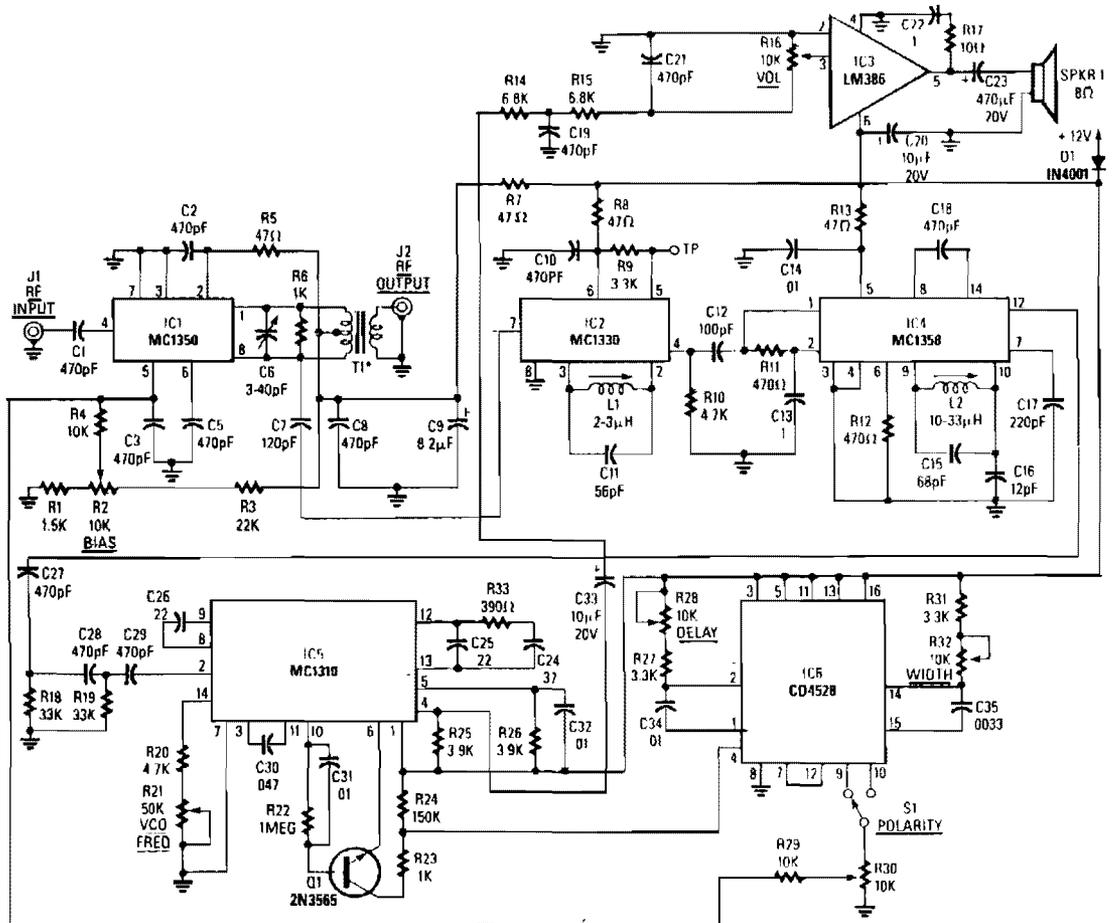
—DESCRAMBLE GATED-PULSE SIGNALS using this easy-to-build circuit. Information for winding transformer T1 and coil L1 can be found in the text.
