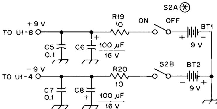
EXCEPT AS INDICATED, DECIMAL VALUES OF CAPACITANCE ARE IN MICROFARADS ( $\mu\text{F}$ ); OTHERS ARE IN PICOFARADS ( $\text{pF}$ ); RESISTANCES ARE IN OHMS;  $k = 1000$ ,  $M = 1000\ 000$ .
