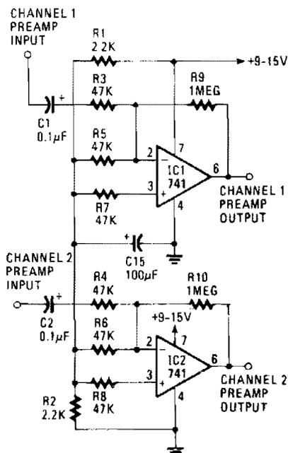
**-THE PREAMP.** If you wish to amplify low-level signals, such as the output of a turntable, the signal will first have to be fed to the preamp shown here.
