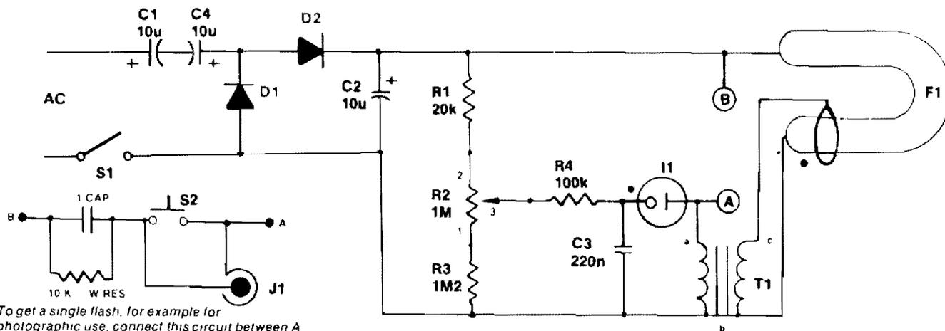
To get a single flash, for example for photographic use, connect this circuit between A and B in the main circuit. With R2 in the position for slowest flash rate (ie no flashes!) S2 will provide the desired single flash. Alternatively J1 can be used to allow the camera's flash contacts to trigger the strobe
