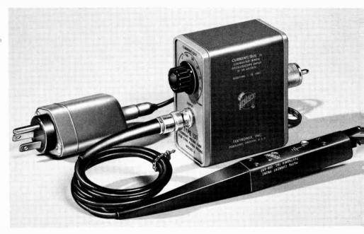
FIGURE 20.2 CURRENT PROBE AND AMPLIFIER
