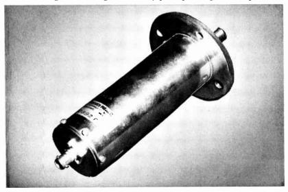
FIGURE 20.4 A COMMERCIAL NON-INDUCTIVE CURRENT SHUNT
