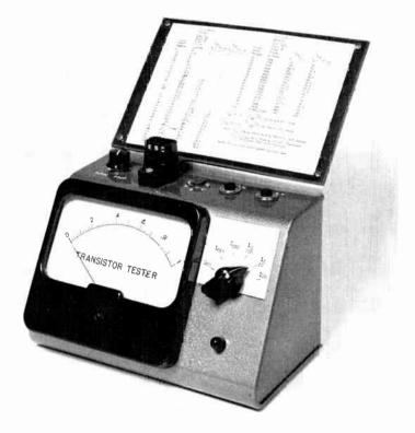
TRANSISTOR TESTER SHOWING READOUT CHART Figure 15.27
