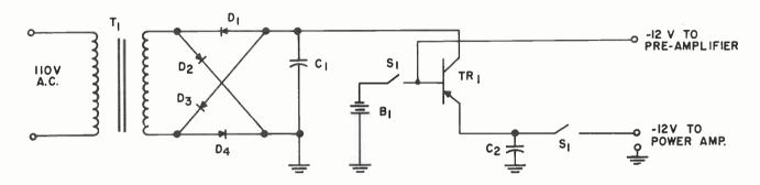
TRI - POWER TRANSISTOR (MOUNT ON HEAT SINK) C.B.S. 2N256, 2N156 OR EQUIVALENT.
