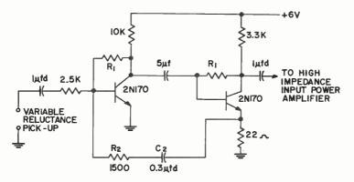
RI (IOOK-500K) SHOULD BE CHOSEN TO MAKE COLLECTOR VOLTAGE 2.5 TO 3.5 VOLTS
