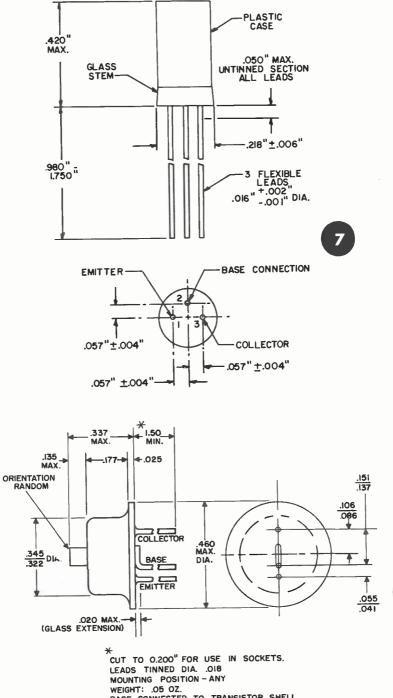
BASE CONNECTED TO TRANSISTOR SHELL. DIMENSIONS IN INCHES.
