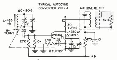
ANTENNA-DELTA COIL<sup>#</sup>I-IO5A OR EQUIVALENT OSCILLATOR COIL – E. STANWYCH CO.<sup>#</sup>II29 (MODIFIED) OR EQUIVALENT CAPACITOR-RADIO CONDENSER<sup>#</sup>242 OR EQUIVALENT I.F. TRANSFORMER-AUTOMATIC 725 (EXO-3926) OR EQUIVALENT
