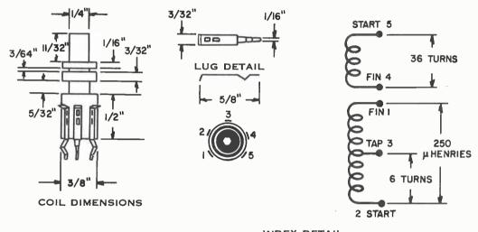
SPECIFICATIONS: 1. Wire To Be #5/44 Heavy Easysol Bonded
