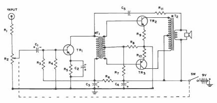
MAXIMUM POWER OUTPUT : .35 WATTS MAXIMUM POWER OUT AT 10% HARMONIC DISTORTION : .25 WATTS SENSITIVITY FOR 50 MILLIWATTS REFERENCE POWER OUTPUT : .2 VOLTS FOR USE WITH MAGNETIC CARTRIDGE OMIT RI, IN THIS CONDITION SENSITIVITY: 5 MILLIVOLTS 220,000 OHM VOLUME CONTROL 10,000 OHM R<sub>2</sub>, 1/2 W AUDIO TAPER 68,000 OHM R3, R4, MHO 000,01 R<sub>5</sub>, - 470 OHM - 220 OHM - 1800 OHM Rg,-- 33 OHM ALL RESISTORS .5W
