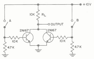
(A) GATE USING NPN TRANSISTORS
