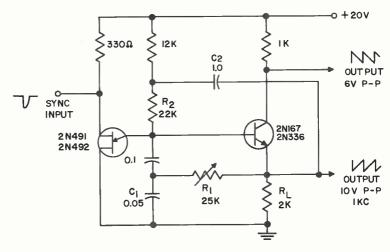
SAWTOOTH GENERATOR WITH HIGH LINEARITY FIGURE 13.12
