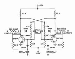
NON-SATURATED FLIP-FLOP FIGURE 11.2 (B)
