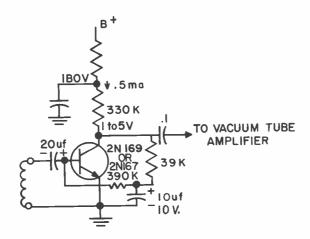
NPN PREAMPLIFIER FOR MAGNETIC PICKUPS
