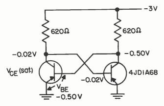
DIRECT COUPLED TRANSISTOR LOGIC (DCTL) FUP-FLOP FIGURE 10.9
