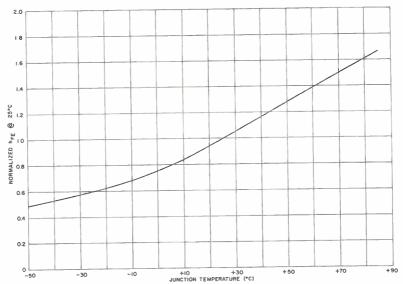
CURRENT GAIN (hFE) VS TEMPERATURE NORMALIZED TO 25°C
