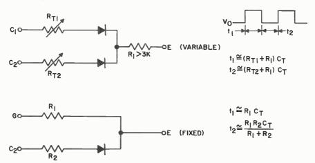
The timing capacitor  $C_T$  will be charged through the resistor  $R_{T1}$  or  $R_{T2}$  which is connected to the positive collector. The diodes will isolate the other resistor from the
