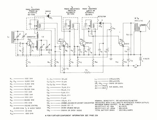
FOUR TRANSISTOR SIX VOLT REFLEX RECEIVER
