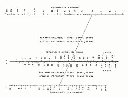
Nomogram for calculating frequency of relaxation oscillation FIGURE 13.10
