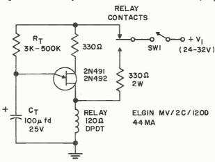
TIME DELAY CIRCUIT WITH RELAY FIGURE 13.14
