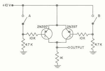
(B) GATE USING PNP TRANSISTORS
