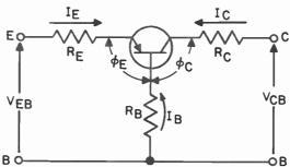
PARAMETERS USED IN LARGE SIGNAL EQUATIONS
