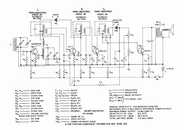
FOUR TRANSISTOR NINE VOLT REFLEX RECEIVER
