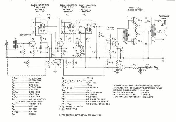
SIX TRANSISTOR SIX VOLT BROADCAST RECEIVER FIGURE 8.23
