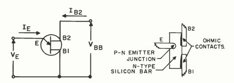
Symbol for unijunction transistor with indentification of principle voltages and currents
