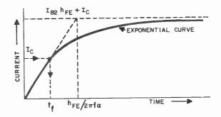
GRAPHICAL ANALYSIS OF FALL TIME THE INTERCEPT OF IC AND THE CURVE GIVES  $\ensuremath{t_{\mathrm{f}}}\xspace$  .
