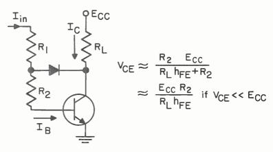
Collector current clamp without bias supply FIGURE 10.11(A)
