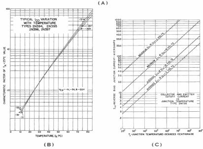
The different electrical properties of the base, emitter and collector regions tend to disappear at high temperatures with the result that transistor action ceases. This temperature usually exceeds  $85^{\circ}$ C and  $150^{\circ}$ C in germanium and silicon transistors respectively.
