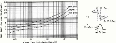
Recovery time of unijunction transistor relaxation oscillator vs. capacity FIGURE 13.11
