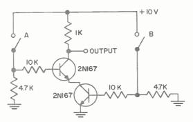
(A) GATE USING NPN TRANSISTORS
