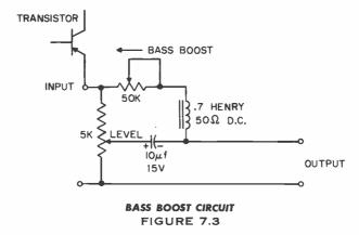
to compensate for listening levels, or deficiencies in program material, pick-up, speakers, etc. This bass boost circuit gives the operator independent control of the level, or amount of bass boost desired, or the level control can be used as a loudness control.
