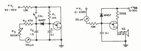
TEST CIRCUIT FOR INTRINSIC STANDOFF RATIO  $(\eta)$
