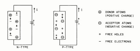
CONDUCTION IN N-TYPE AND P-TYPE SEMICONDUCTORS FIGURE 1.3
