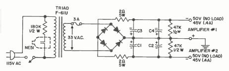
CI - 1500 µf, 50 VOLTS C2-1500 µf, 50 VOLTS C3-1500 µf, 50 VOLTS C4-1500 µf, 50 VOLTS SILICON BRIDGE-FOUR-INIII5
