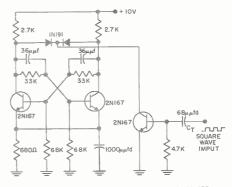
COLLECTOR TRIGGERING WITH TRIGGER AMPLIFIER FOR IMC TRIGGER RATE LESS THAN I VOLT TRIGGER AMPLITUDE REQUIRED.
