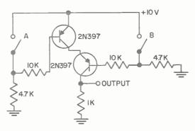
(B) GATE USING PNP TRANSISTORS
