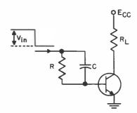
Stored charge neutralization by capacitor FIGURE 10.12
